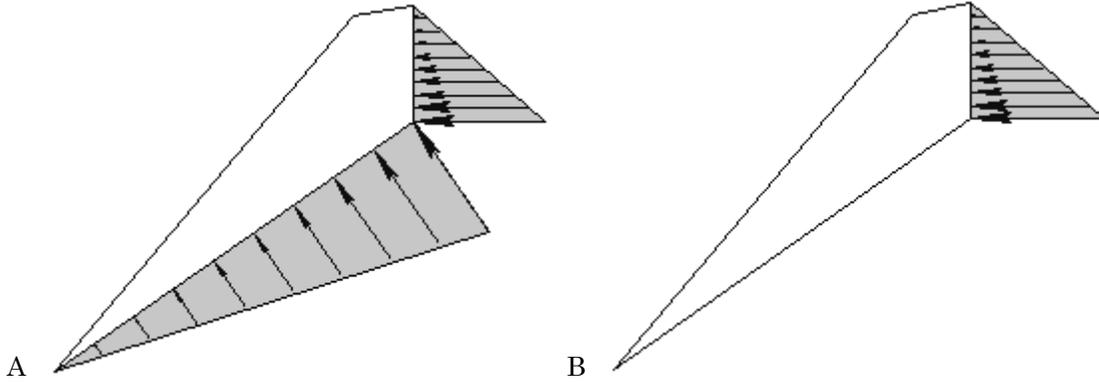
Peak Pressure Tension Crack Base option. Pressure on both tension crack and failure plane (A) and pressure on tension crack only (B).
