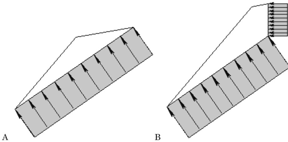
Custom Pressure water pressure option, without tension crack (A) and with tension crack (B).
