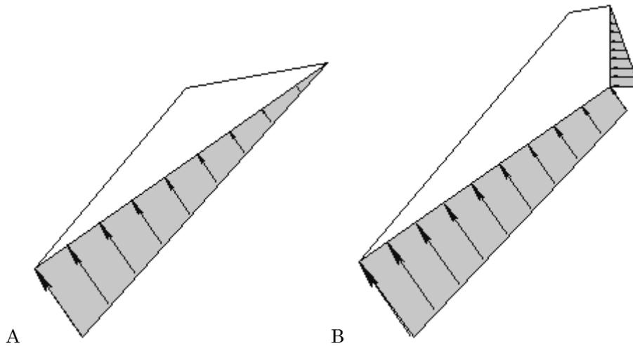
Peak Pressure Toe water pressure option, without tension crack (A) and with tension crack (B).
