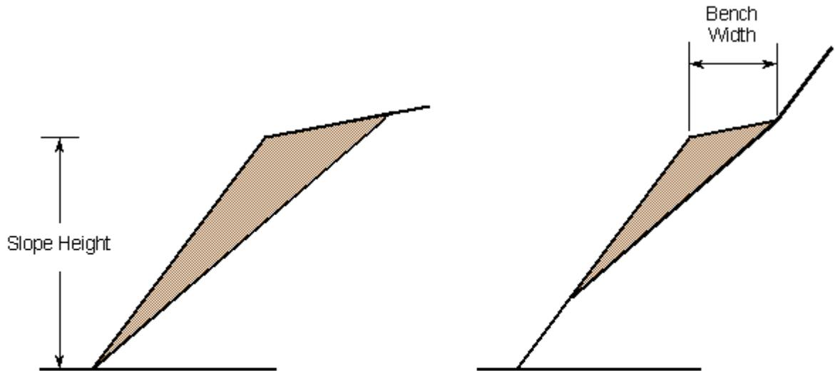
Sliding block in the analysis of a complete slope. The block is scaled to the height of the slope by assuming that the failure plane passes through the slope toe.
