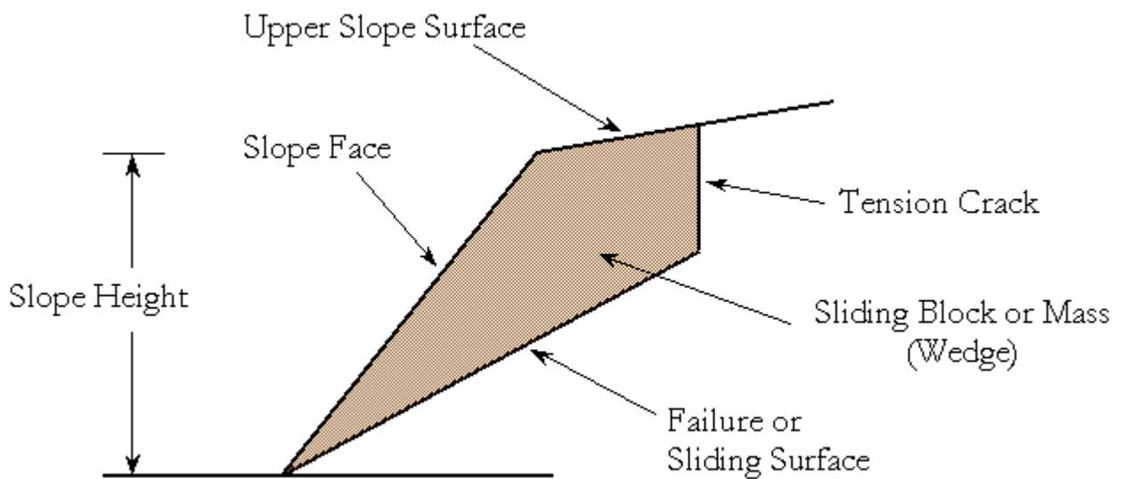
Typical planar geometry of a ROCPLANE model. Basic terminology used in the program is also shown on the figure.
