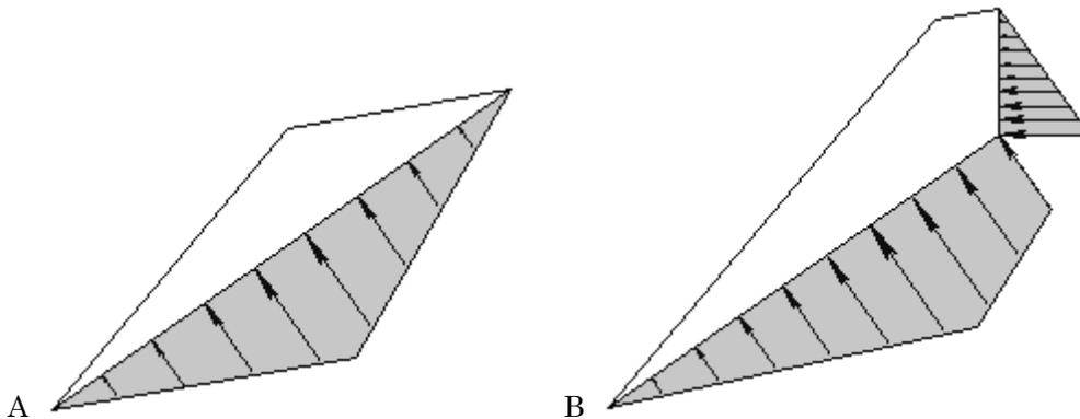
Peak Pressure Mid Height water pressure option, without tension crack (A) and with tension crack (B).
