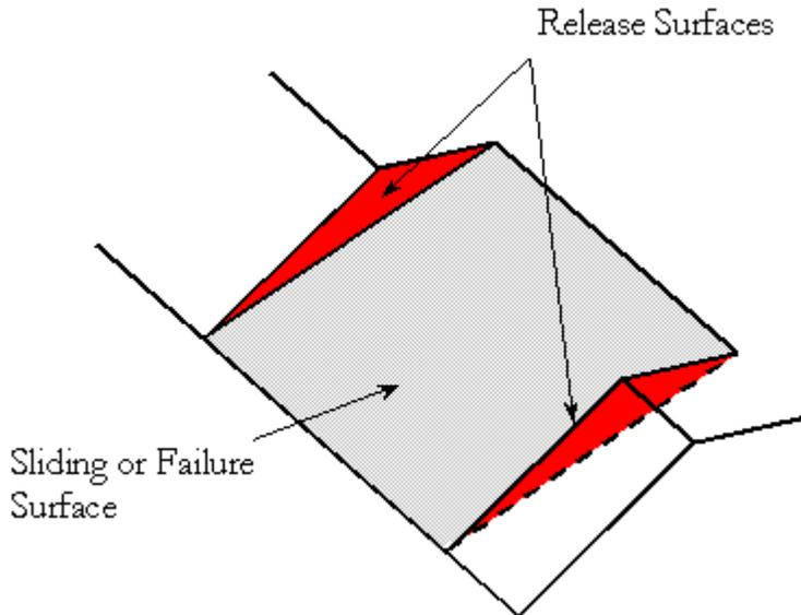
The release surfaces of a sliding block.
