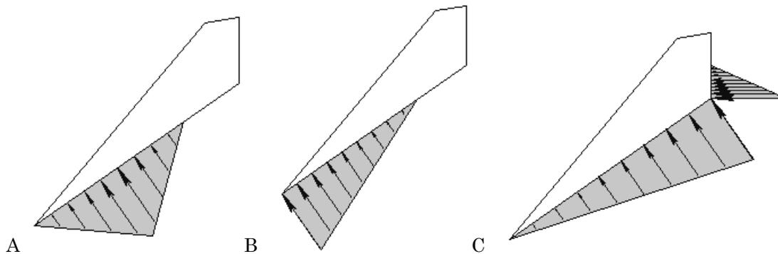
Percent Filled = 50% for Peak Pressure Mid Height (A), Peak Pressure Toe (B) and Peak Pressure TC Base (C).
