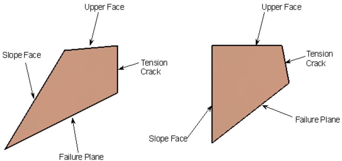
Examples of valid wedge geometries involving tension cracks.
