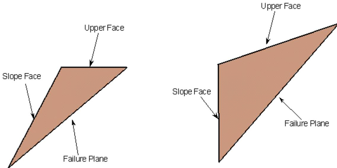
Examples of valid sliding block geometries, when no tension crack is involved.
