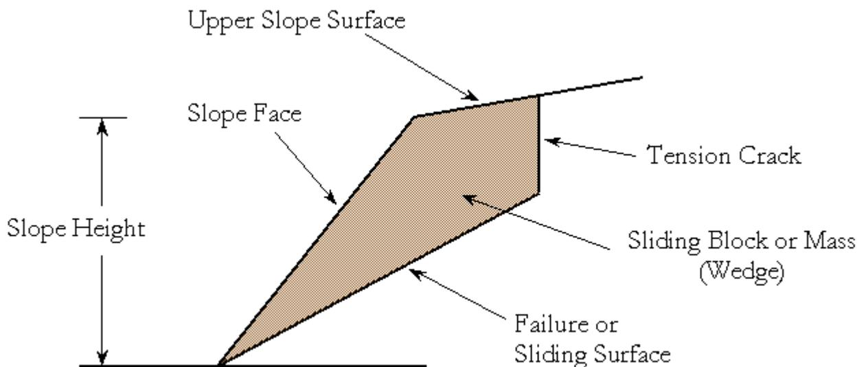
Typical planar wedge geometry for ROCPLANE analysis.
