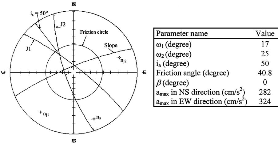
**Fig. 14a,b.** Case 4: **a** the wedge failure occurred northeast of Kızıllı Village (Dinar) after the 1995 earthquake; **b** the kinematical analysis and the geometrical characteristics of the wedge
