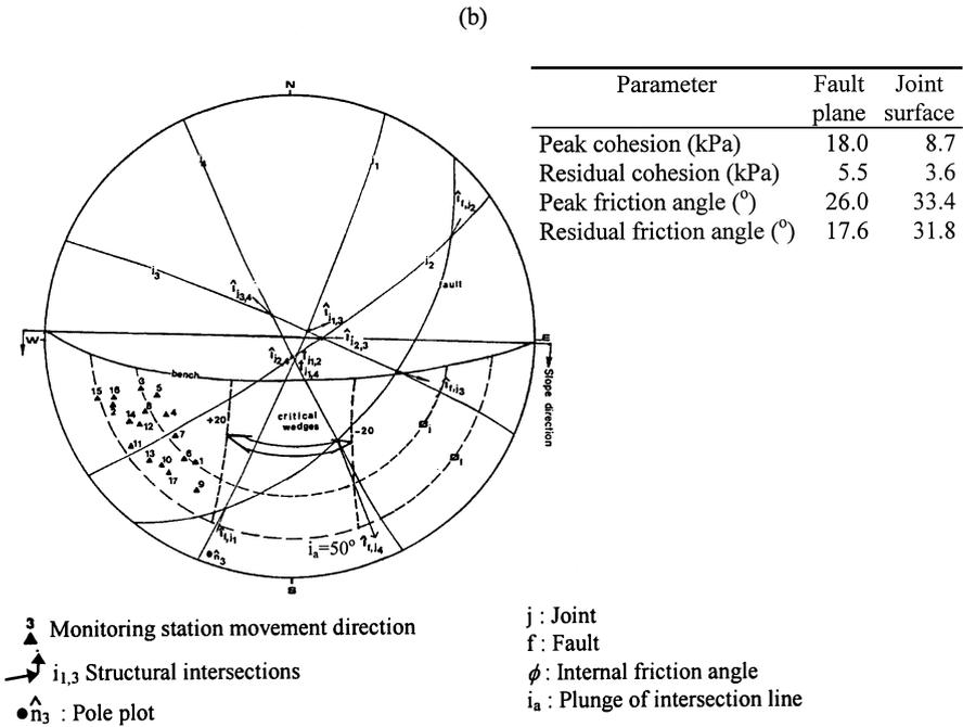
**Fig. 11a,b.** Case 1: **a** general view of the wedge failure and the geometrical characteristics of the wedge; **b** kinematical analysis of possible lines of intersection and plots of monitoring data for Case 1 and shear strength parameters of the discontinuities involved by the wedge (after Ulusay, 1991)
