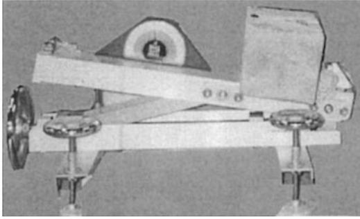
**Fig. 3.** Perspective view of the tilting test on a wedge model
