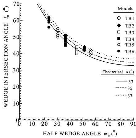
Fig. 9. Comparison of the submerged-static model test results with theoretical solutions
