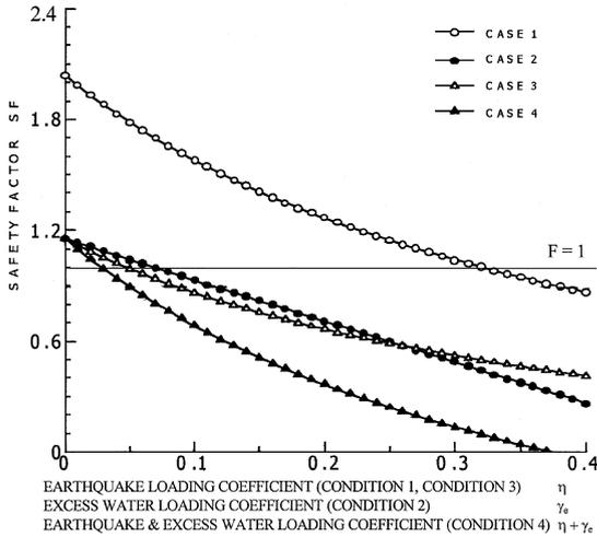
Fig. 17. Comparison of different case results for the wedge failure at Mt. Mayuyama
