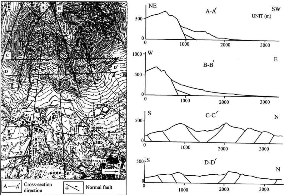
Fig. 15. Present topography and cross-sections of the close vicinity of Mt. Mayuyama (after Misawa et al., 1993)
