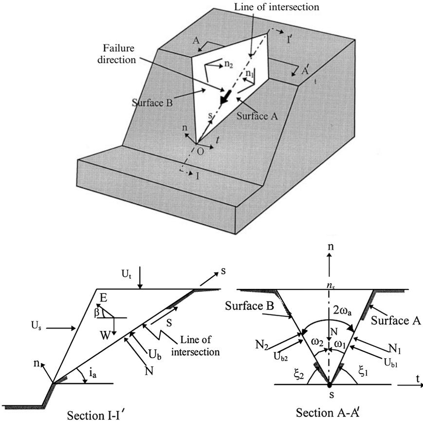
Fig. 7. Forces acting on a wedge block
