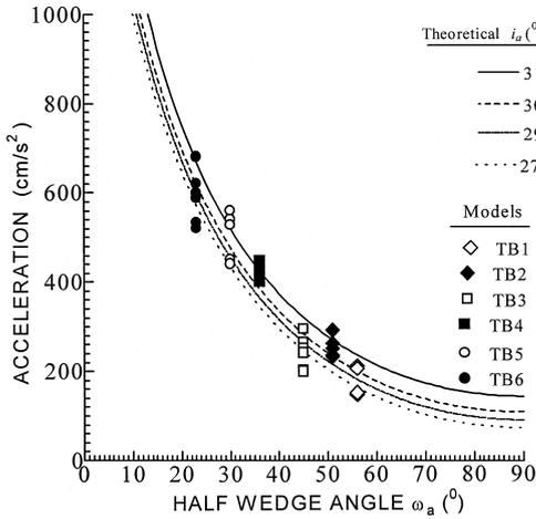
Fig. 10. Comparison of the dynamic model test results with theoretical solutions
