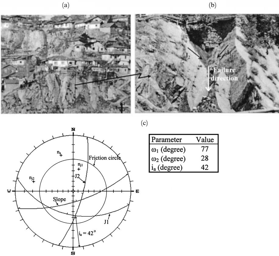
**Fig. 13a–c.** Case 3: **a** view of the wedge failure near Ankara Castle; **b** close up view from the wedge near Ankara Castle; **c** the kinematical analysis and the geometrical characteristics of the wedge
