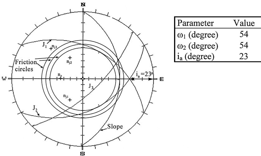
Fig. 16. Kinematical analyses of the wedge blocks at Mt. Mayuyama and the geometrical characteristics of the wedge
