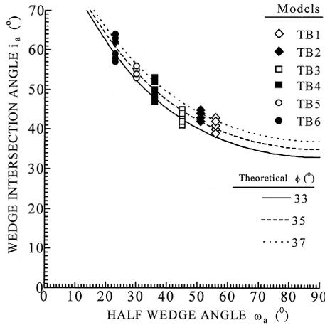
Fig. 8. Comparison of the dry-static model test results with theoretical solutions
