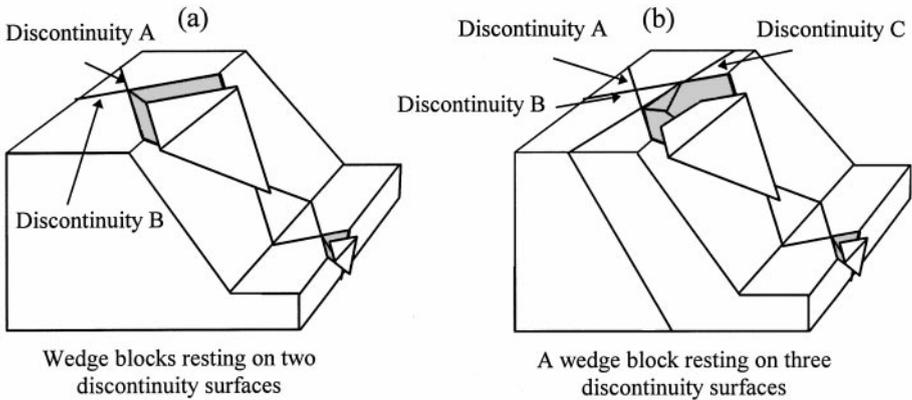
Fig. 1. Types of wedge failure
