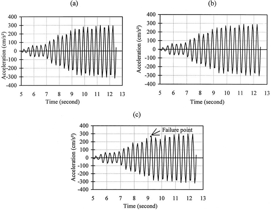
**Fig. 6a–c.** Example records of acceleration of the dynamic stability test on the wedge block numbered TB1C: **a** records on the shaking table; **b** records on the base block; **c** records on the wedge block
