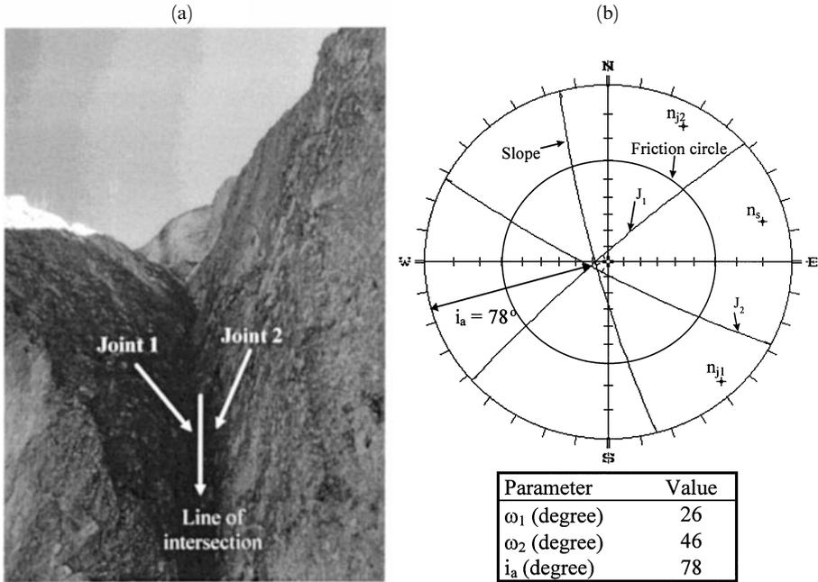
**Fig. 12a,b.** Case 2: a a wedge failure in Zelve at Cappadocia; b its kinematical analysis and geometrical characteristics
