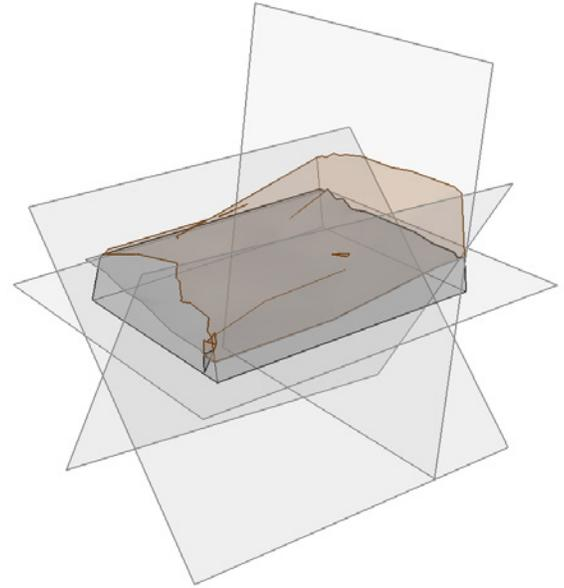
The top layer in the model is MSW, and the layer of leachate just before failure is shown in blue. The landfill rests on a shale bedrock, and there is a thin layer of native soil at the interface. A multiplanar search analysis was conducted on the slope using the searching planes shown in the
