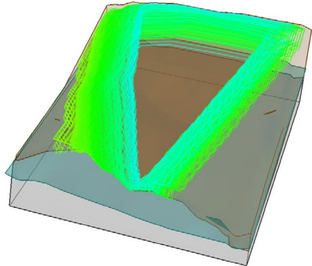
The right figure above shows the range of slip surfaces that were generated and analyzed in the search. This model demonstrates the utility of multiplanar searching in predicting the critical slip surfaces of slopes that commonly experience planar failures.
