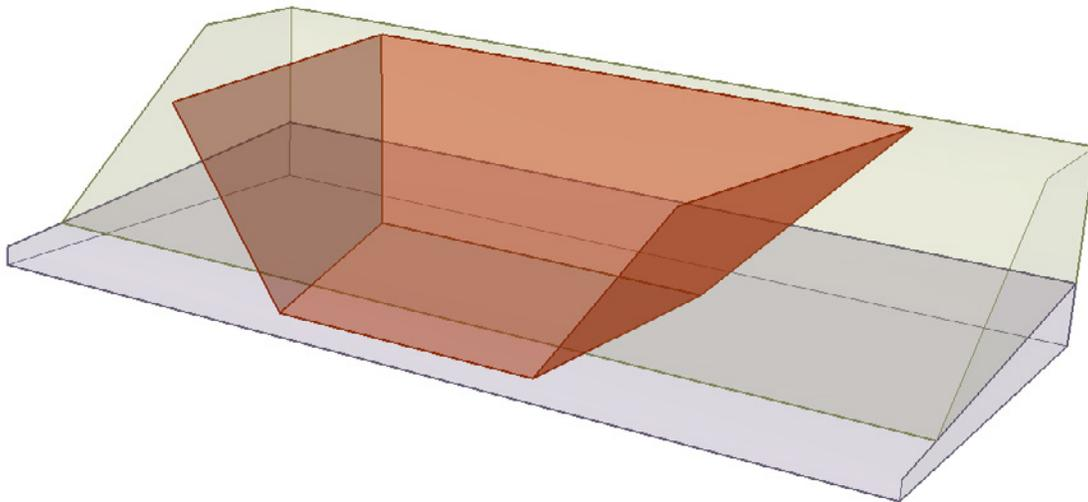
The set of planes used to form the multiplanar slip surface can each be expressed using the infinite plane equation presented below:
