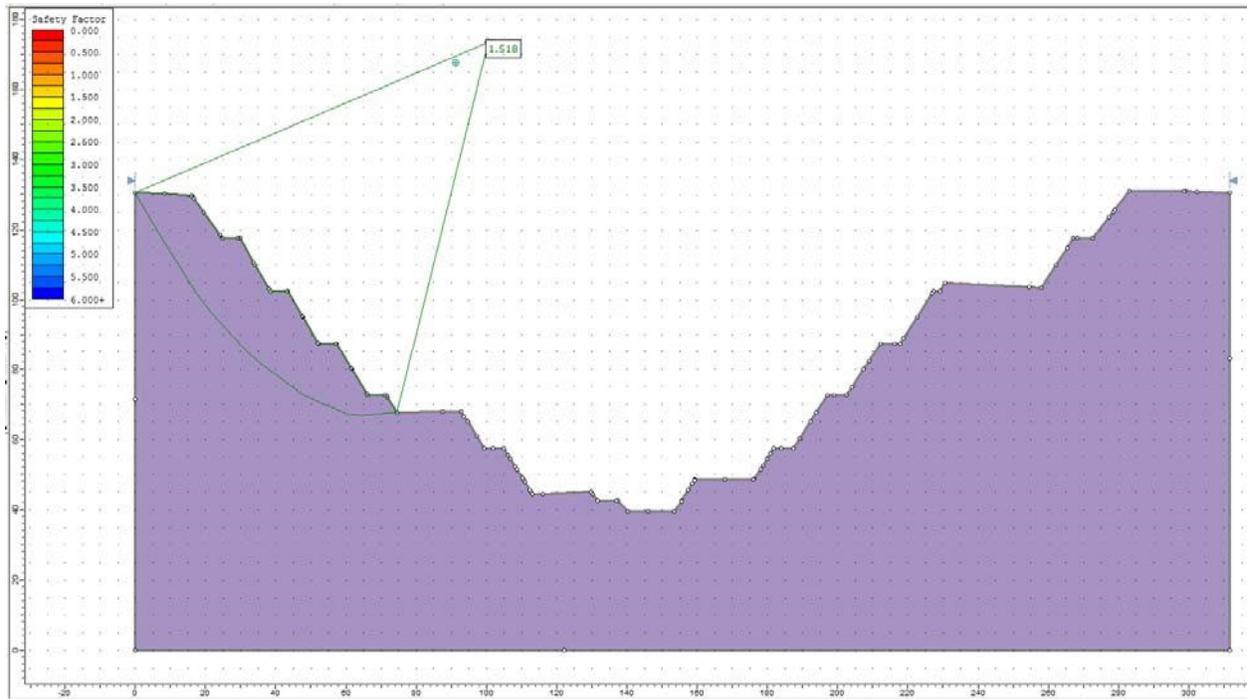
Figure 3.2 – Slide2 Solution Using the Bishop Method
