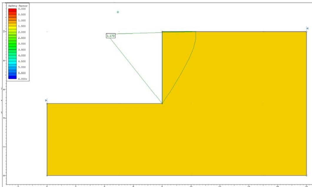
**Figure 18.4.2 – Slide Solution Using the Bishop Method**
