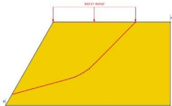
*Bearing capacity test slope, homogeneous ( $\phi=0$ ), weightless, strength (m-c), distributed load, predefined slip surface*
