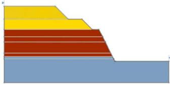
*Excavated slope, (4) materials, multi strength (m-c, undrained (f-depth)), circular (auto-refine), tension crack, clay, imperial units*
