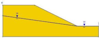
*Slope, homogeneous (c-phi material), strength (m-c), groundwater (dry, ru, water table), circular surface, imperial units*
