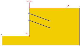
*Retaining wall, homogeneous, strength (undrained, constant cohesion), support (soil nails), planar failure, non-circular (block search), shotcrete, line load, reinforced wall*
