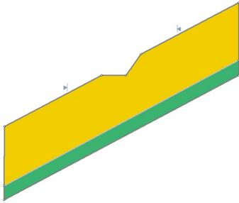
*Excavated slope, homogeneous (c-phi material), strength (m-c), finite element groundwater seepage analysis, matric suction/unsaturated shear strength, circular (auto refine search)*
