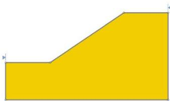
*Slope, homogeneous (c-phi material), strength (m-c), circular (auto refine search), non-circular (path search + optimization)*
