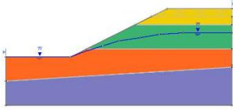
*Slope, (4) materials, strength (m-c), water table, tension crack, seismic, circular (1 surface)*
