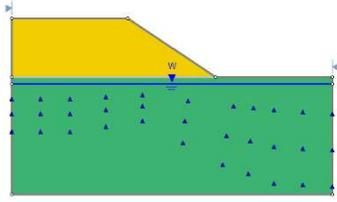
*Embankment, multi (2) materials, embankment, strength (m-c), pore pressure grid, water table, circular (grid search)*
