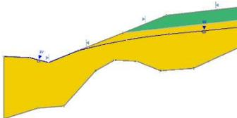
*Slope, (2) materials, strength (m-c), tension crack, water table (auto Hu), unsaturated unit weight, imperial units, bedrock, circular (1 surface, auto refine search)*
