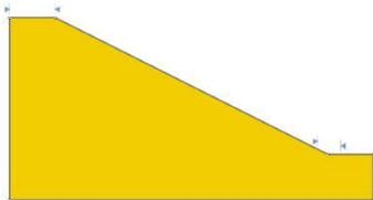
*Slope, homogeneous (c-phi material), strength (m-c), ru pore pressure, non-circular (path search + optimization)*
