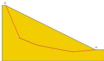
*Slope, homogeneous, strength (power curve), sensitivity analysis, non-circular (1 surface)*
