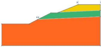
*Slope, (3) material, strength (m-c), dry, seismic, non-circular (path search + optimization)*
