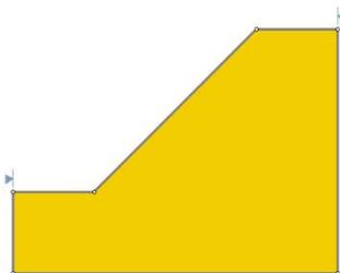
*Slope, homogeneous (c-phi material), strength (m-c), probabilistic analysis (overall slope), ru pore pressure, reliability index, circular (grid search)*
