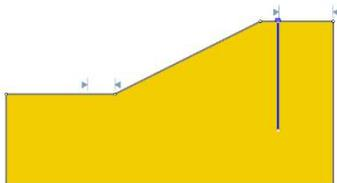
*Slope, homogeneous (c-phi material), strength (m-c), micro pile, circular (grid search)*
