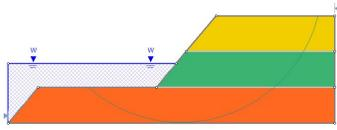
*Embankment, (3) materials, strength (undrained, constant cohesion), ponded water, circular (1 surface), imperial units*
