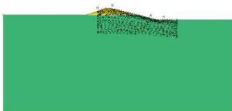
*Dam, (2) materials, end of construction (empty), steady state (full), rapid drawdown, finite element groundwater seepage, ponded water, strength (m-c), strength (discrete strength function), non-circular (path search + optimization)*
