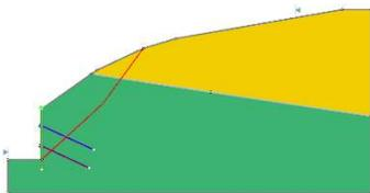
*Retaining wall, (2) materials, strength (m-c), grouted tiebacks, soldier piles, non-circular (1 surface), imperial units*
