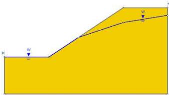
*Slope, homogeneous (c-phi material), strength (m-c), water table, circular (auto refine search), non-circular (path search + optimization)*
