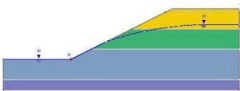
*Slope, (4) materials, strength (m-c), water table, tension crack, circular (grid search), non-circular (block search, path search)*
