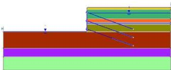
*Retaining wall, (8) materials, strength (m-c), grouted tieback, piezo line, circular (grid search), imperial units, water table*
