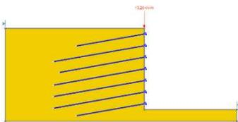
*Retaining wall, homogeneous (c-phi material), strength (m-c), support (soil nails), planar failure, non-circular (6 surfaces), shotcrete, line load, reinforced wall*
