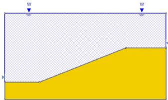
*Submerged slope, homogeneous, strength (m-c), water table, ponded water, circular (auto refine), imperial units*
