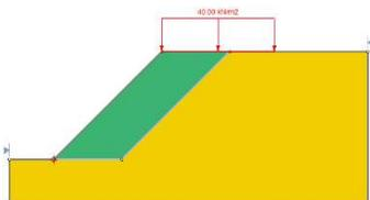
*Slope, homogeneous (c=0), strength (m-c), support (back analysis of required support force and length), distributed load, circular (grid search)*
