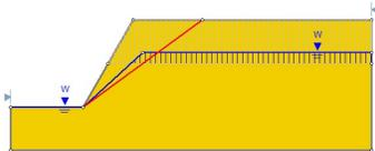
*Slope, homogeneous (c-phi material), strength (m-c), piezo line, water table, tension crack, planar failure, non-circular (1 surface), RocPlane comparison, sensitivity analysis*
