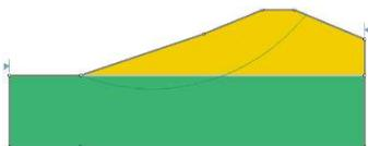
*Embankment dam, (2) materials, strength (m-c), circular (1 surface), imperial units*
