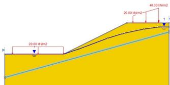
*Slope, (2) material, weak layer, piezo line, distributed load, non-circular (block search, optimization)*
