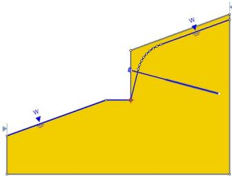
*Retaining wall, homogeneous ( $c=0$  material), strength ( $m-c$ ), grouted tieback, water table, circular (grid search), imperial units*
