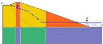
*Embankment dam, (2) materials, strength (m-c), water table, ponded water, circular (1 surface), imperial units*
