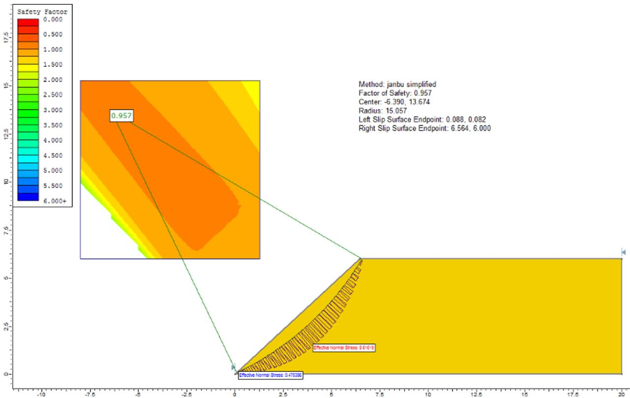
Figure 44.4: Mohr-Coulomb criterion with iterations, Janbu simplified
