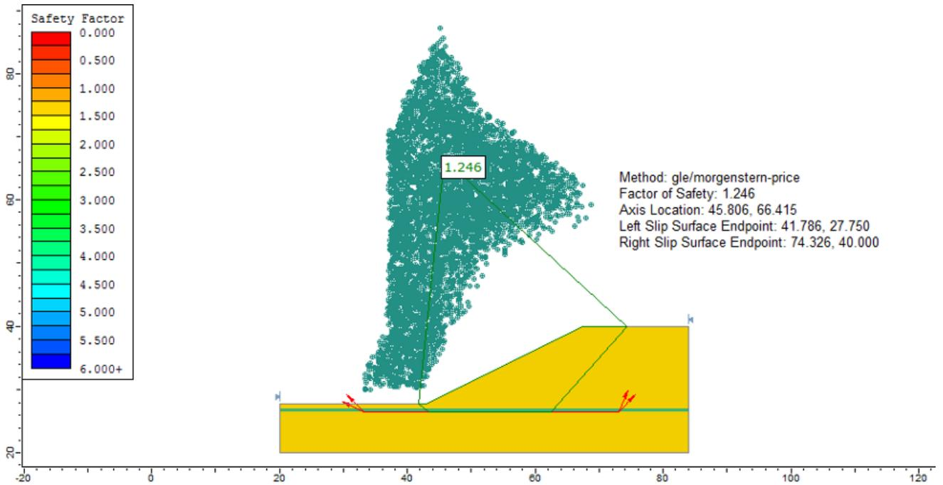
Figure 7.3: Solution, using the GLE method
