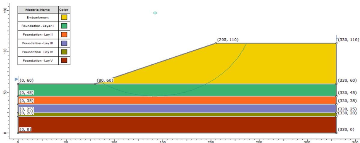
Figure 80.1: An Embankment Resting on A Stratified Soil Foundation
