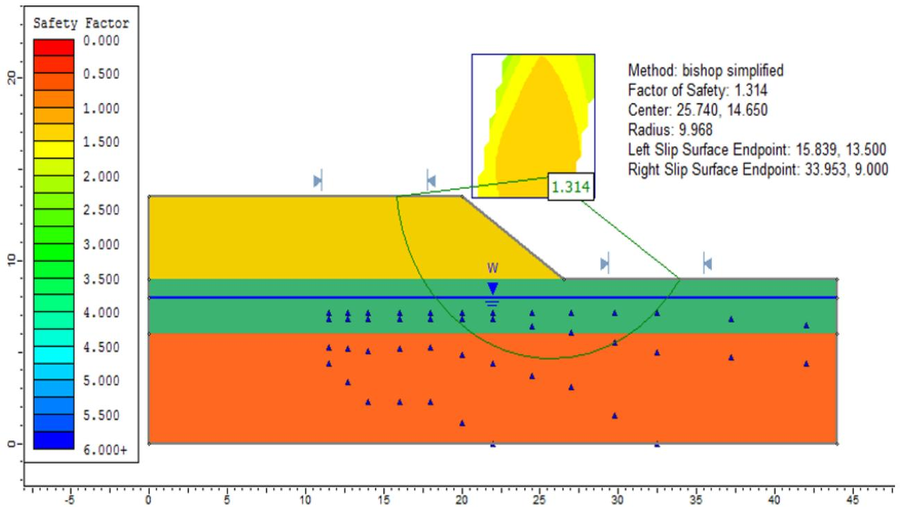
Figure 13.2: Solution, using the Bishop simplified method
