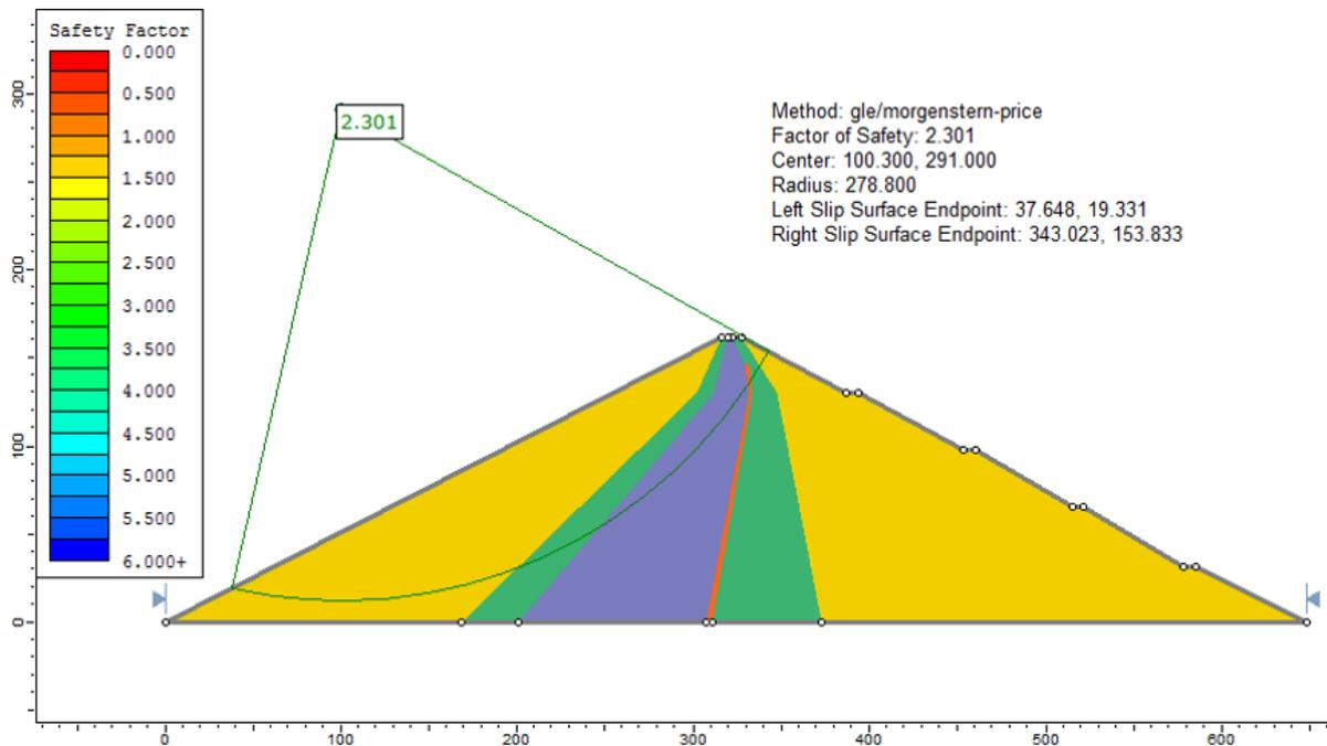
Figure 6.5: Solution, using the GLE method
