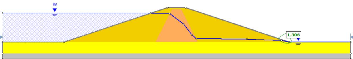
Figure 72.4: Solution to Case 1(b) (Circular), using the Bishop method
