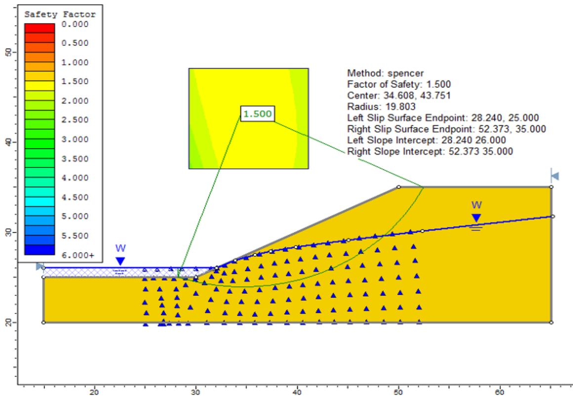
Figure 10.4: Solution, using the Spencer method
