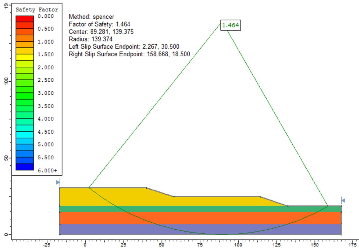
Figure 75.2: Solution to Case 1, using the Spencer method (Circular)
