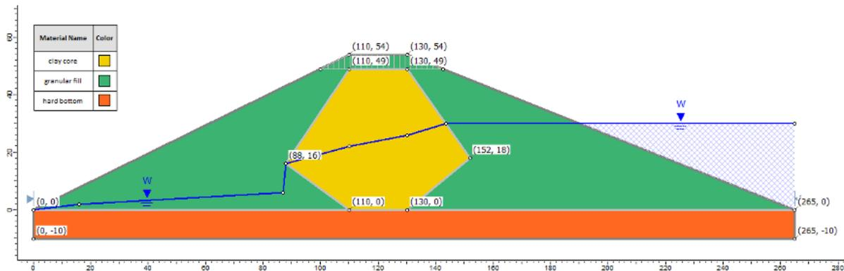
Figure 42.1: Geometry Setup in Slide
