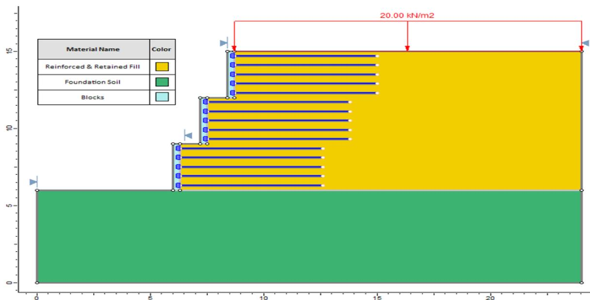
Figure 93.1: A Three-tiered Wall in **Slide**
