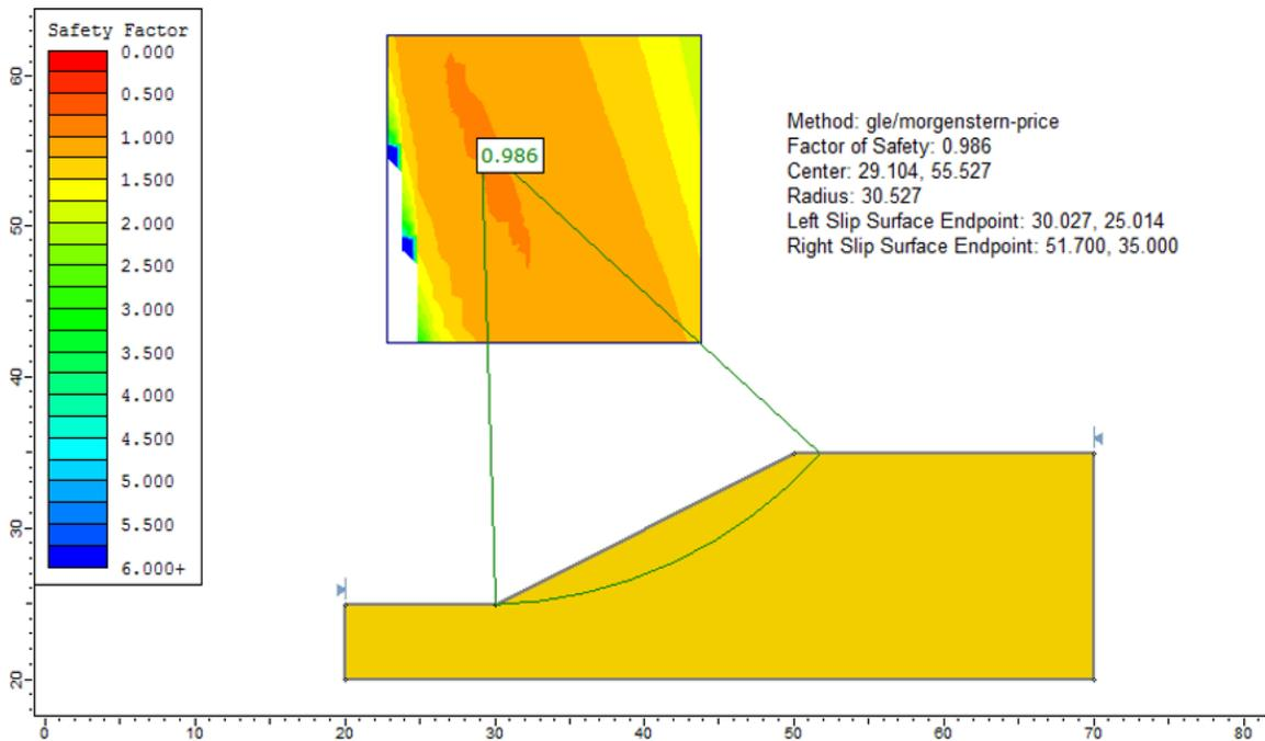
Figure 1.4: Solution, using the GLE method
