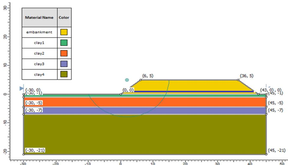
Figure 31.1: Geometry Setup in **Slide**
