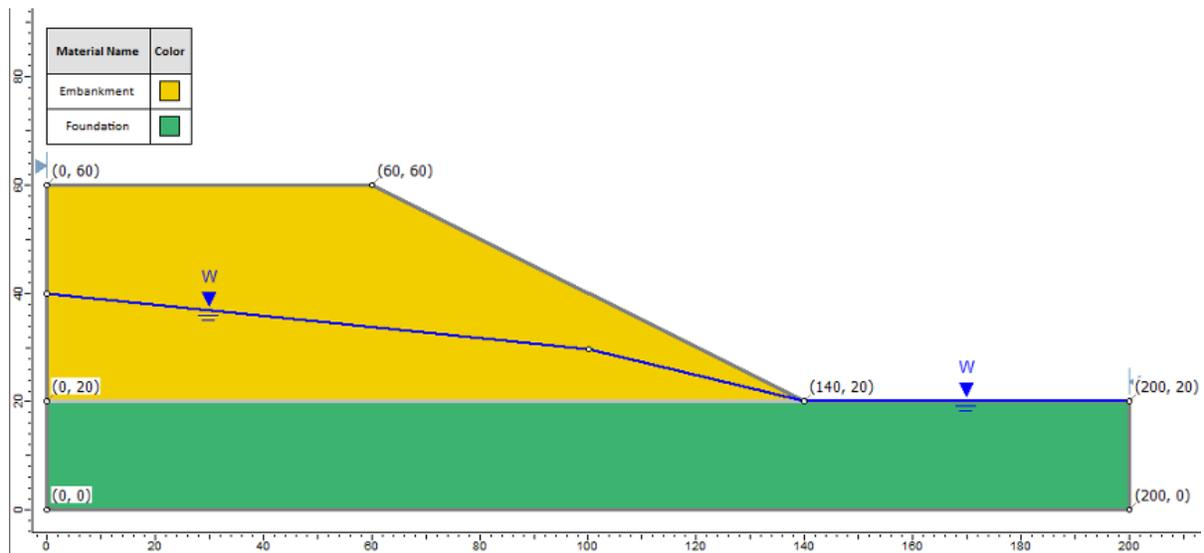
Figure 82.1: Geometry Setup in **Slide**
