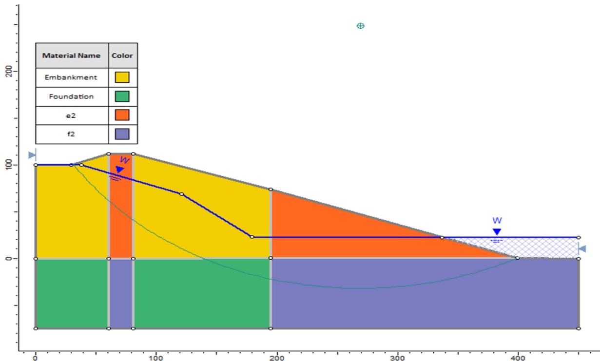
Figure 69.1: Geometry Setup in Slide
