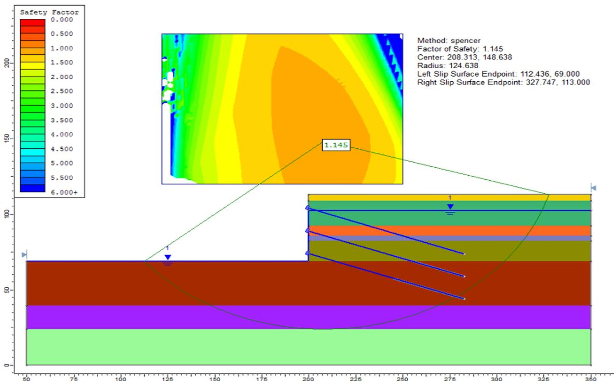
Figure 58.2: Circular failure surface, using the Spencer method
