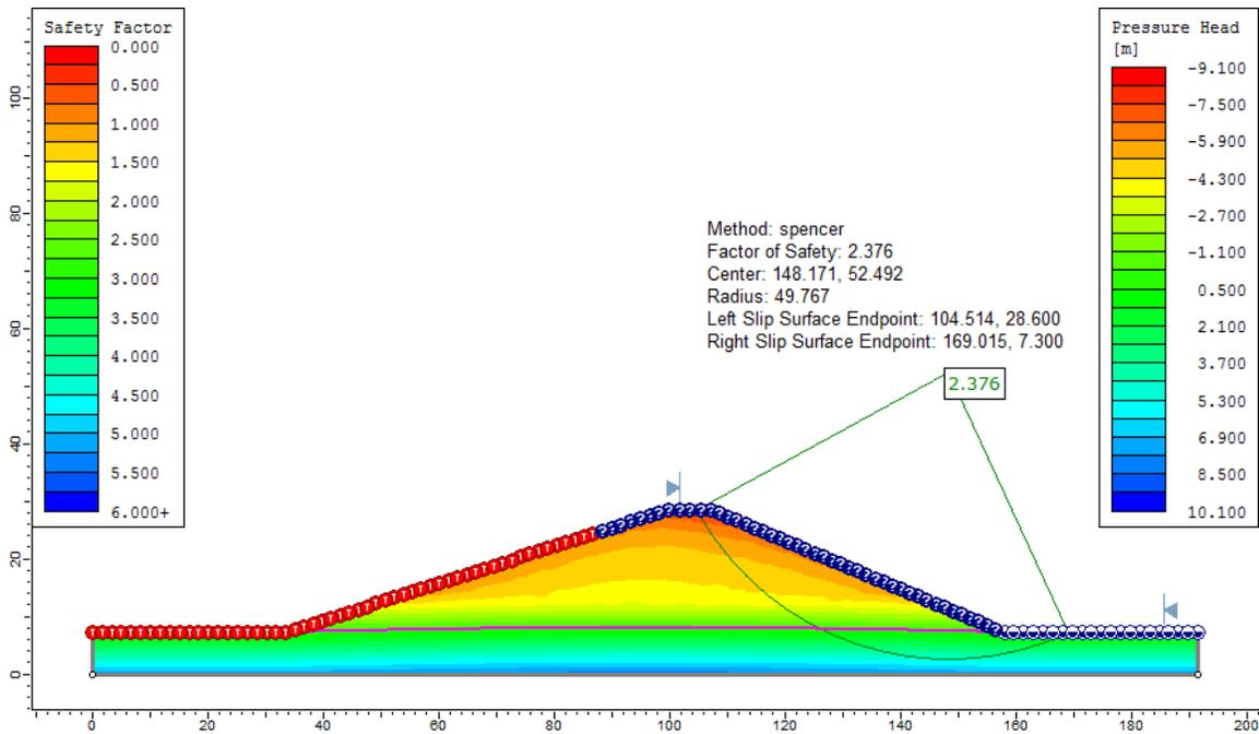
Figure 102.8: **Slide** Results for  $\phi^b = 0^\circ$  at 1500 h, using the Spencer method
