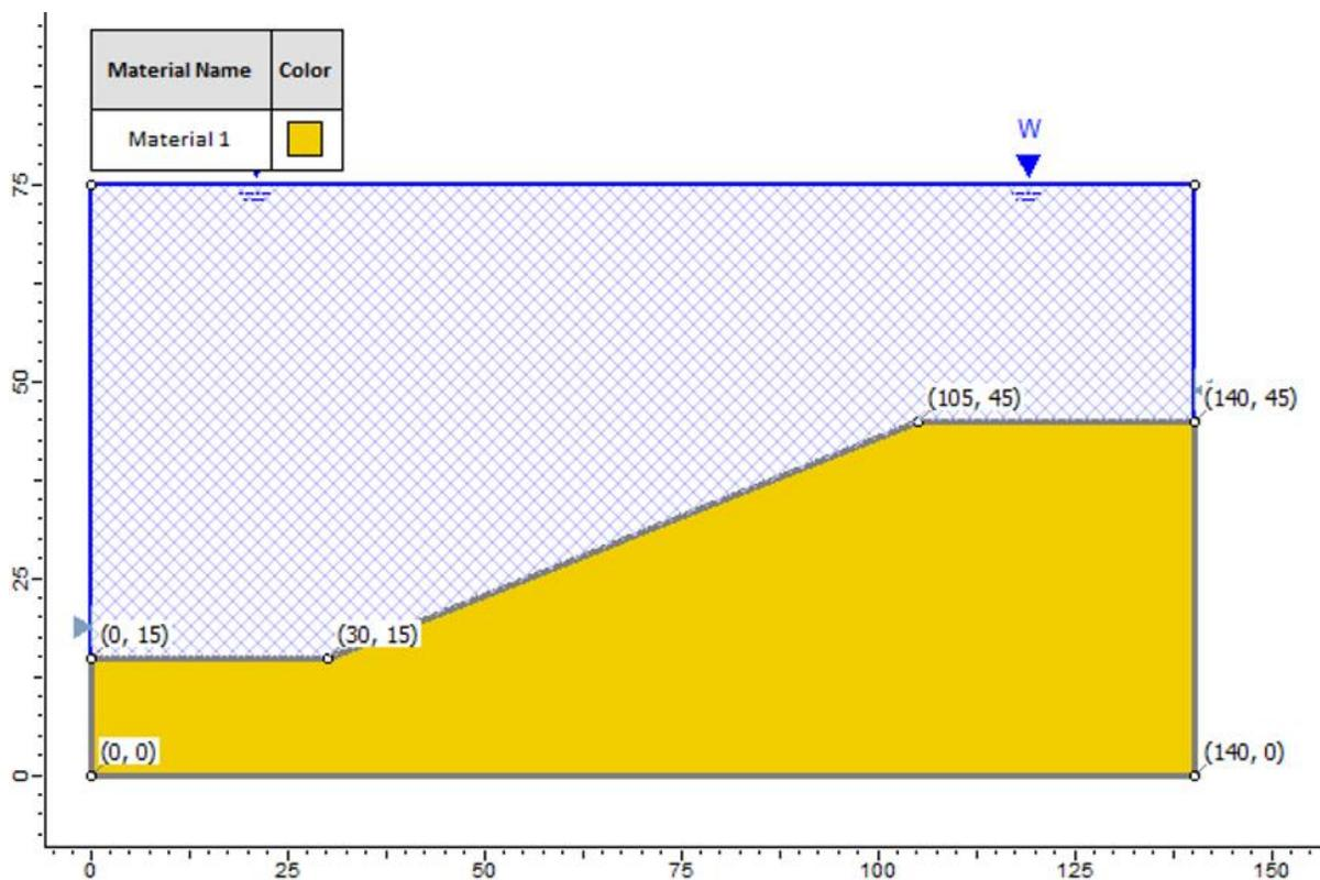
Figure 70.1: Water Table at 30' above the Crest (Case 1)
