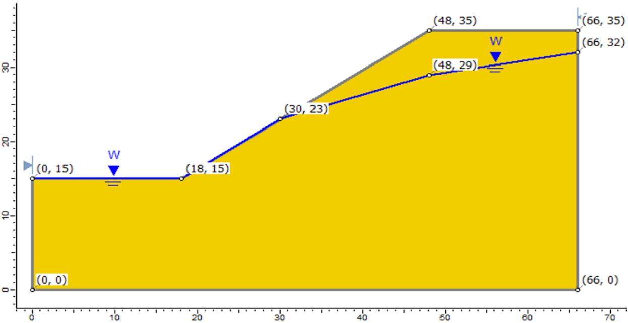
Figure 16.1: Geometry Setup in Slide
