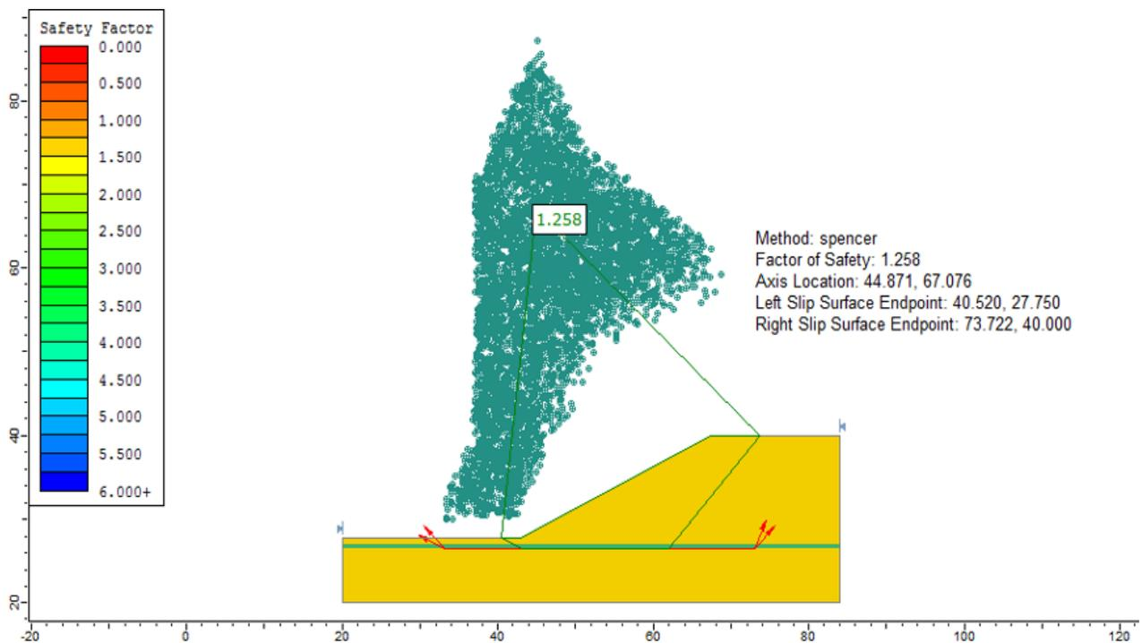
Figure 7.2: Solution, using the Spencer method
