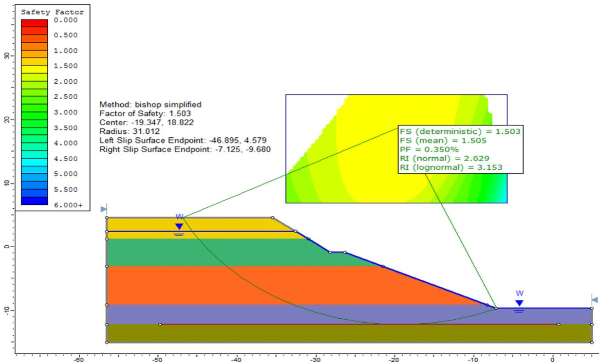
Figure 28.10: Critical slip circle tangential to lower boundary of clay layer 3
