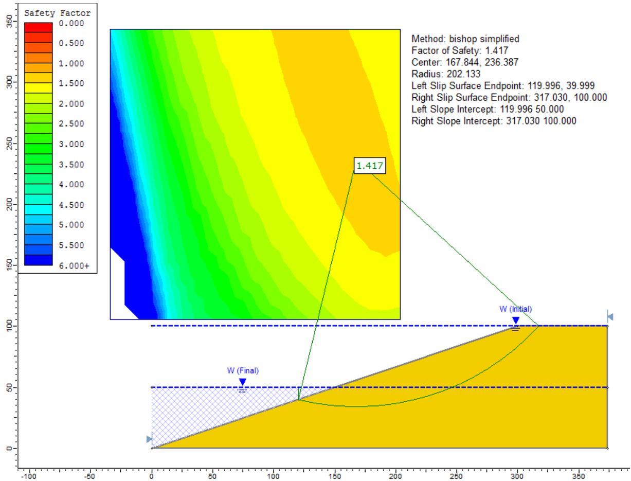
Figure 101.2: Solution, using the B-Bar rapid drawdown method
