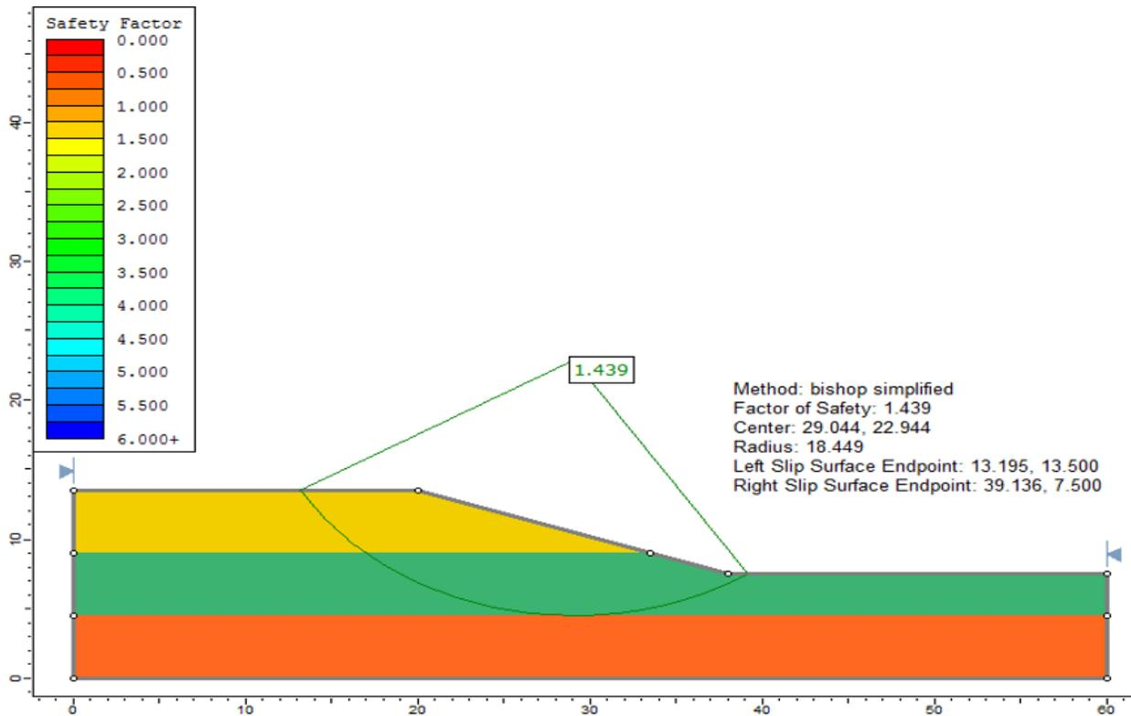
Figure 24.2: Circular failure surface, using the Bishop simplified method
