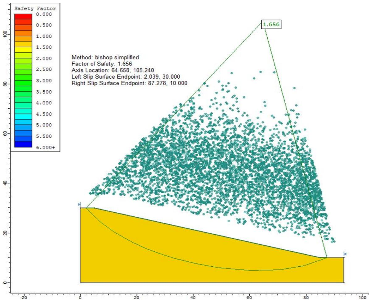
Figure 41.2: Solution, using the Bishop simplified method
