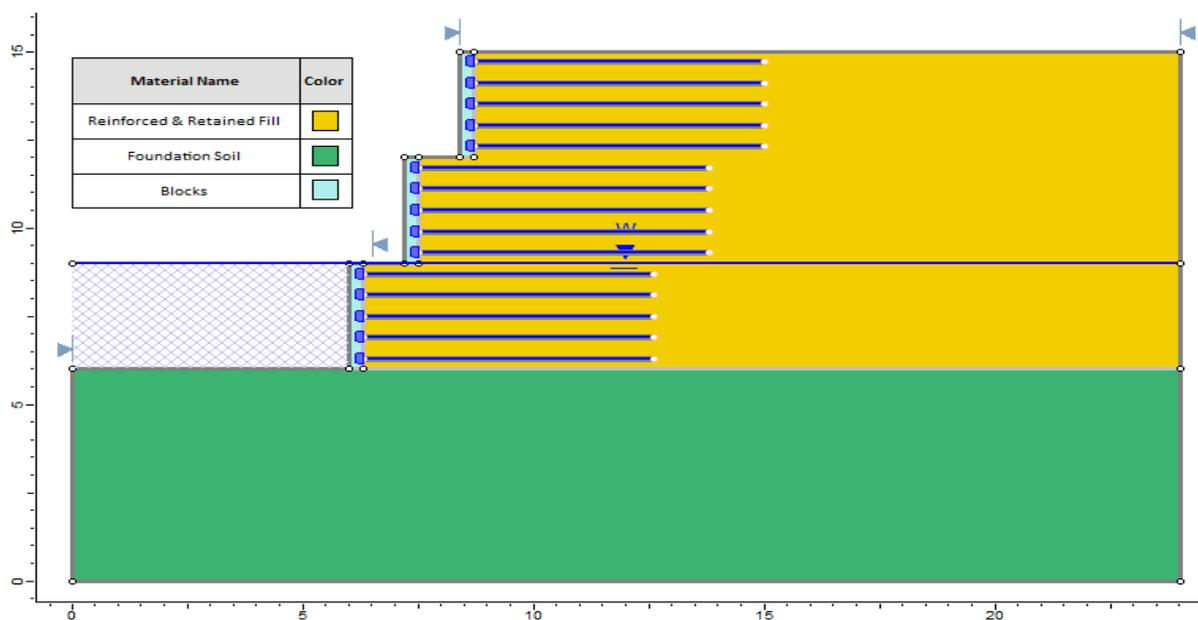
Figure 92.1: A Three-Tiered Wall in **Slide**
