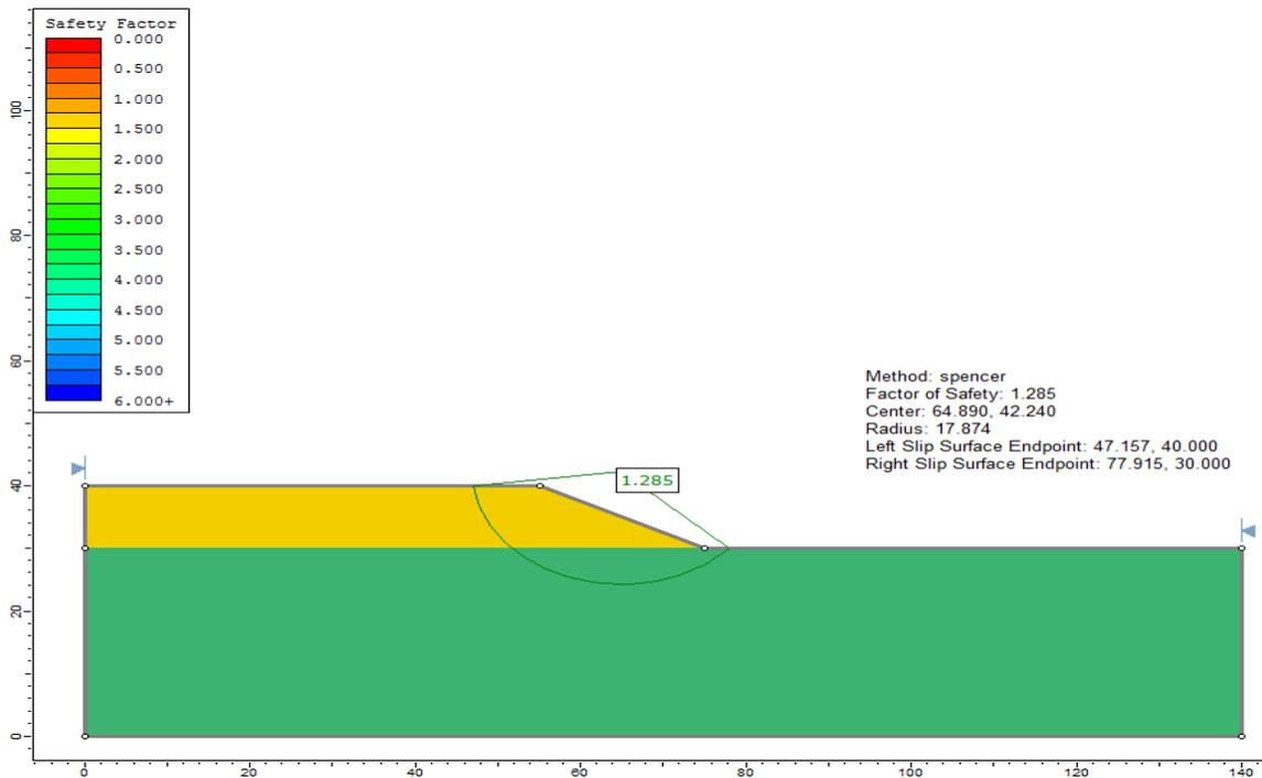
Figure 83.3: Solution to Case 1, using the Spencer method
