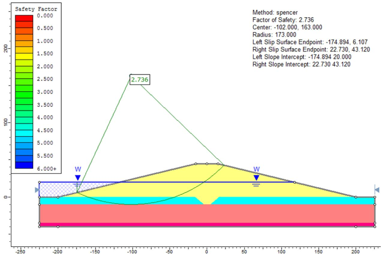
Figure 65.2: Solution, using the Spencer method
