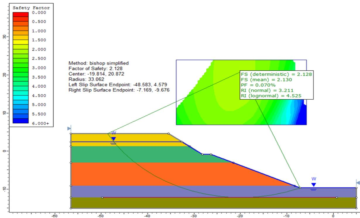
Figure 28.8: Critical slip circle tangential to lower boundary of clay layer 3
