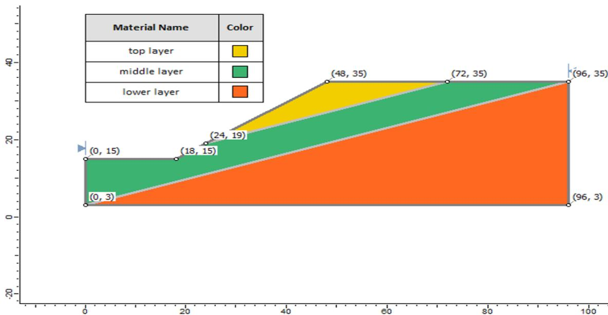
Figure 15.1: Geometry Setup in Slide
