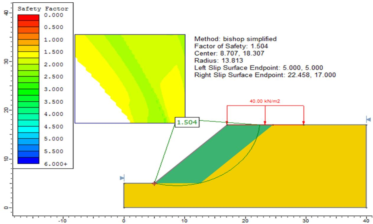
Figure 37.4: Critical Surface (with reinforced zone)
