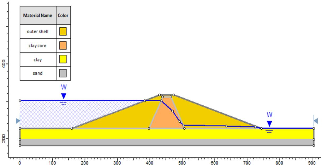
Figure 72.2: Piezometric Line Approximation
