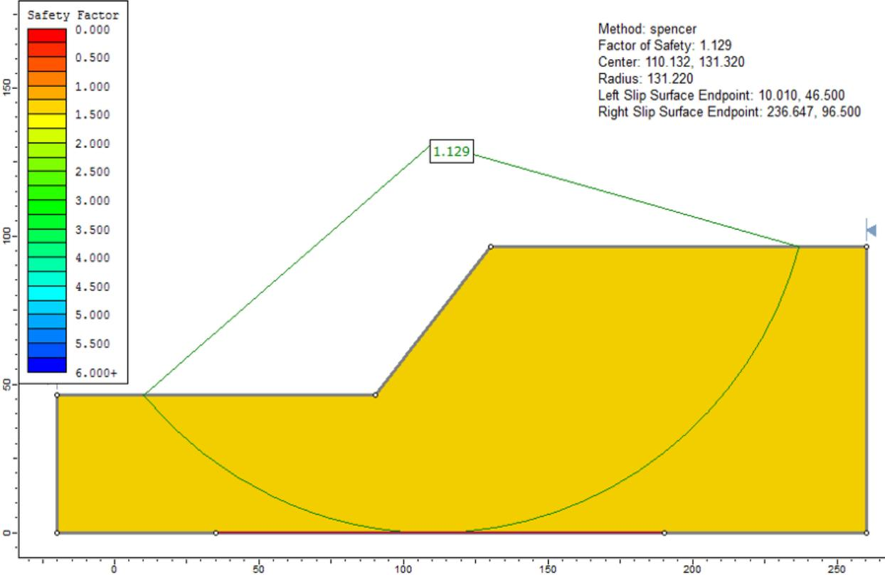
Figure 78.5: Solution to Case 2(b), using the Spencer method
