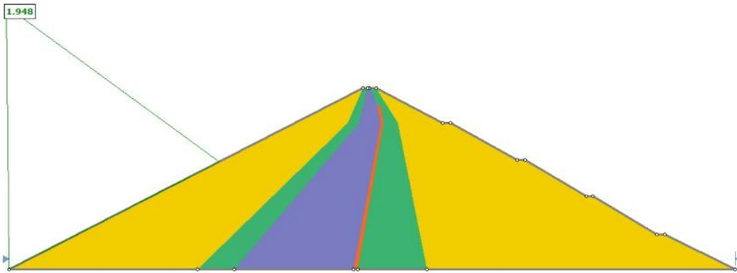
Figure 5.5: Solution, using the GLE method
