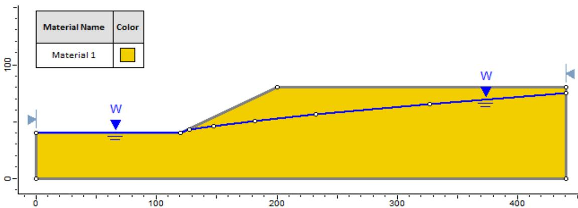
Figure 71.2: Piezometric Line Approximation (Case 2)
