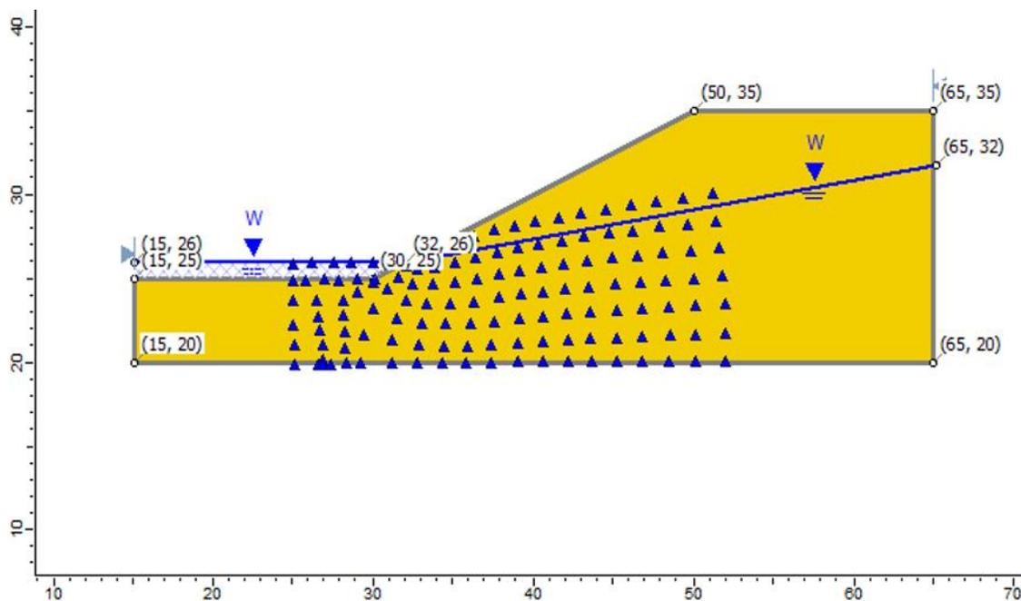
Figure 10.1: Geometry Setup in **Slide**
