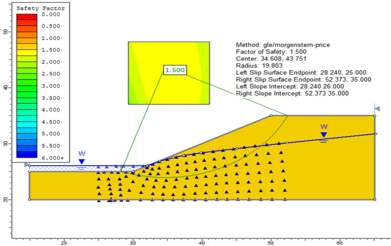
Figure 10.5: Solution, using the GLE method
