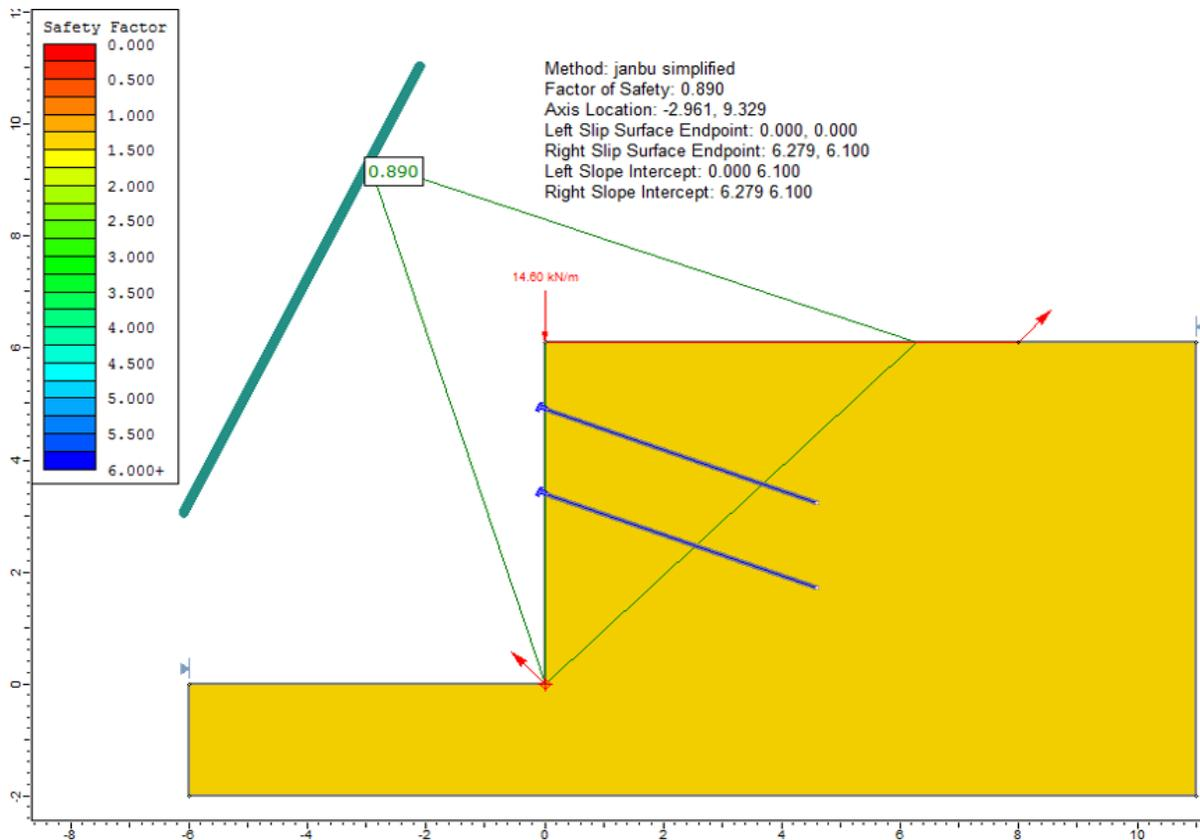
Figure 47.2: Critical failure surface, using the Janbu simplified method
