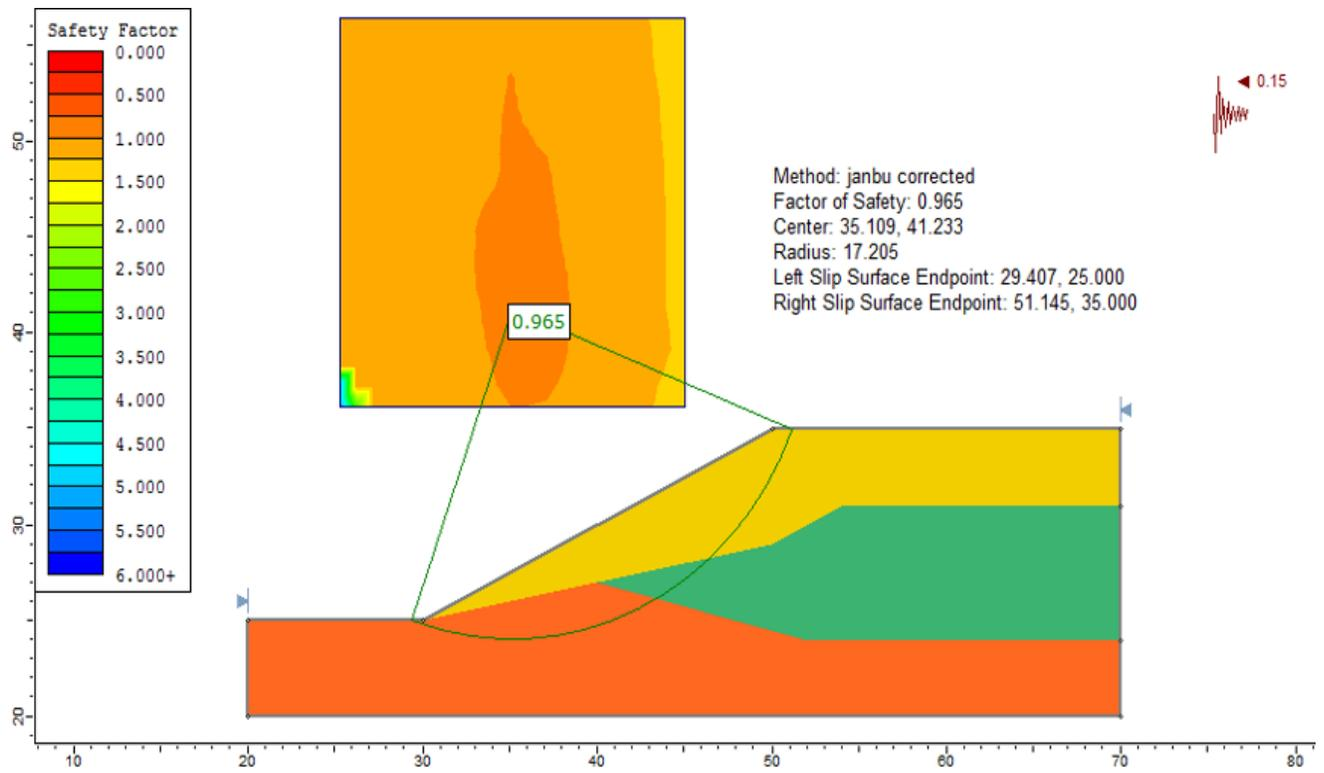
Figure 4.5: Solution, using the Janbu corrected method
