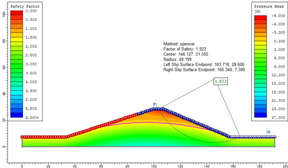
Figure 102.9: **Slide** Results for  $\phi^b = 37^\circ$  at 80 h, using the Spencer method
