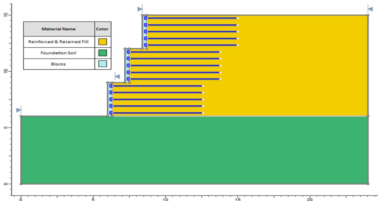
Figure 87.1: A Three-tiered Wall in **Slide**
