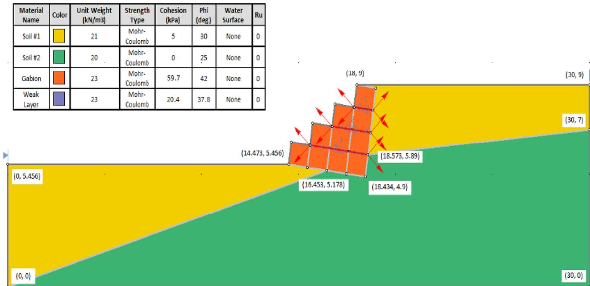
Figure 109.1: Gabion Wall Model in in Slide
