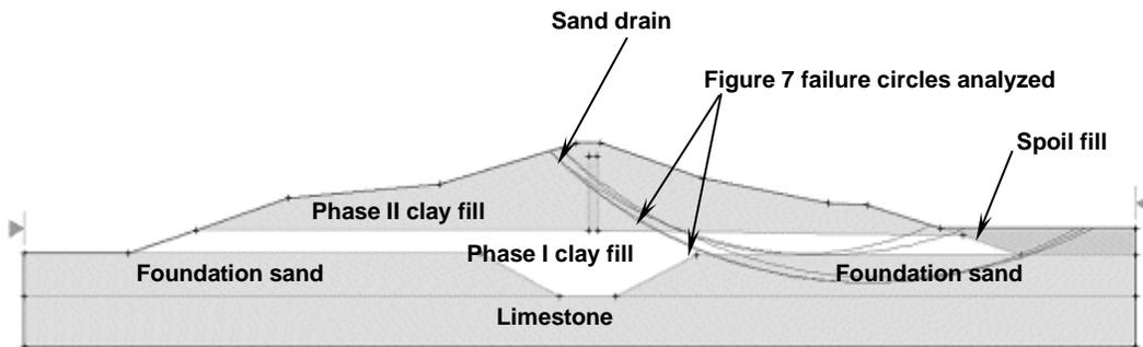
Figure 35.3 Slide Setup for the original Figure 7
