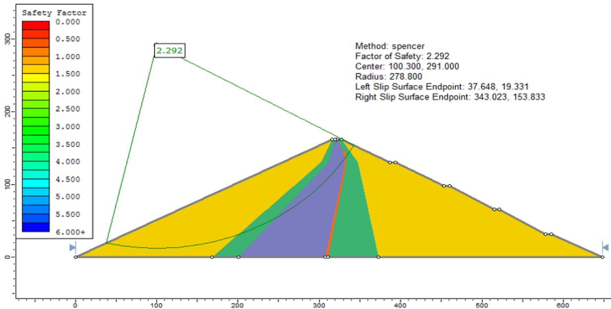
Figure 6.4: Solution, using the Spencer method
