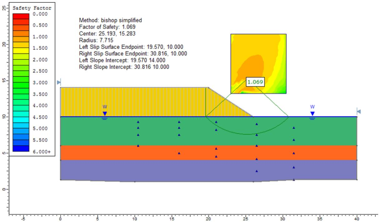
Figure 12.2: Solution, using the Bishop simplified method
