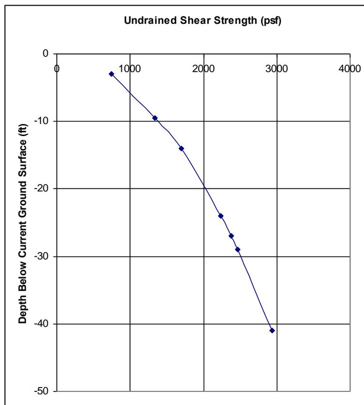
Figure 73.1: Approximation of Undrained Shear Strength Profile Based on Undrained Shear Strength Profile from Skempton and LaRochelle (1965)
