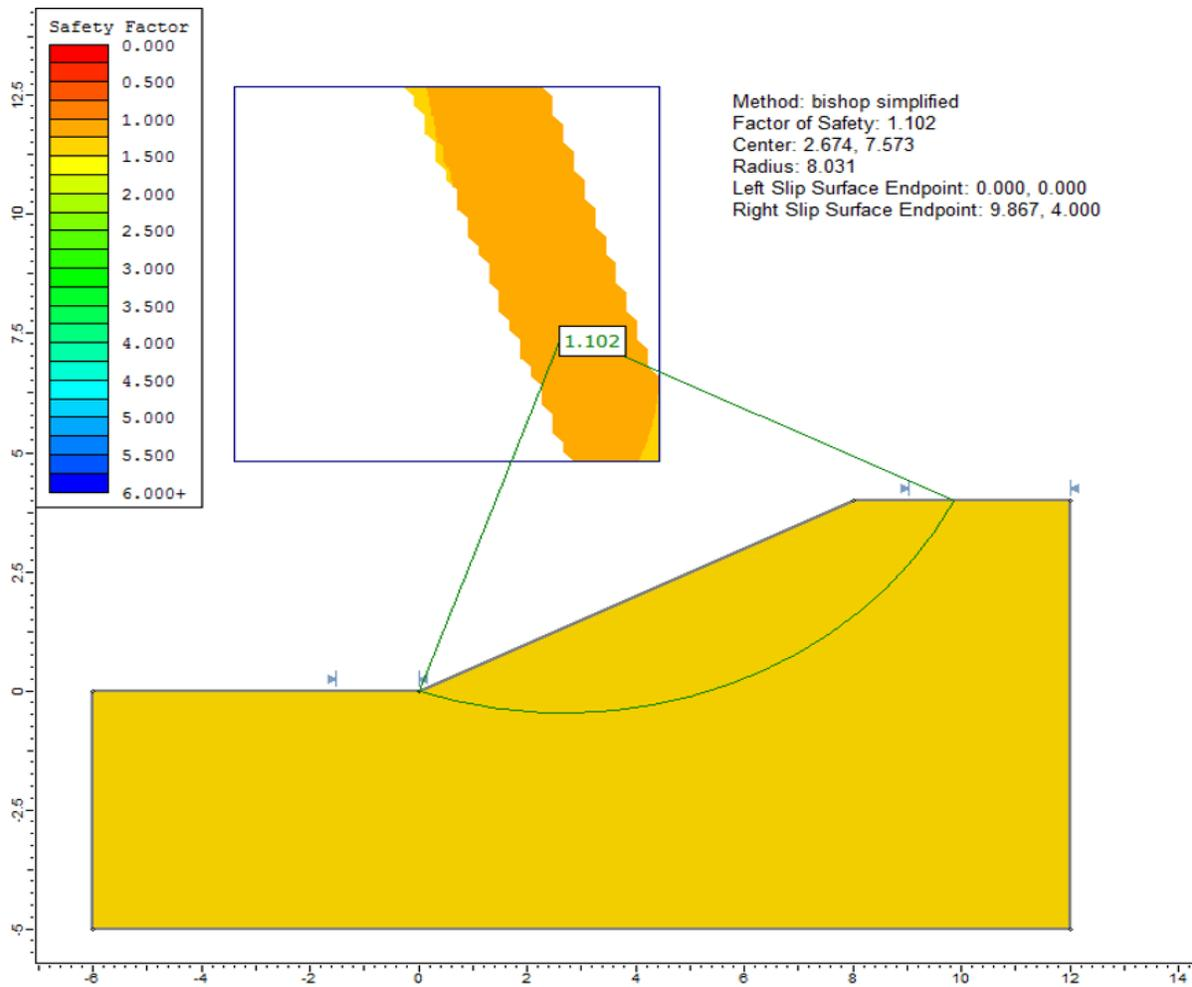
Figure 54.2: Circular failure surface, no pile
