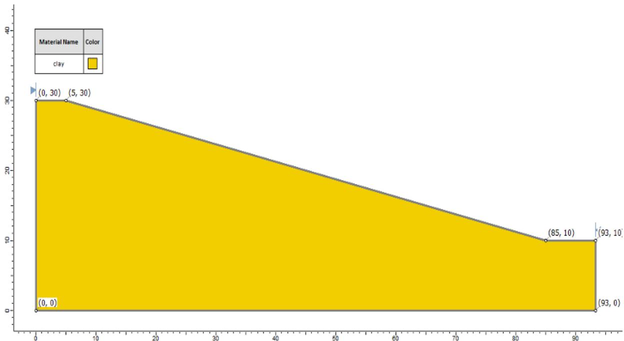
Figure 41.1: Geometry Setup in **Slide**
