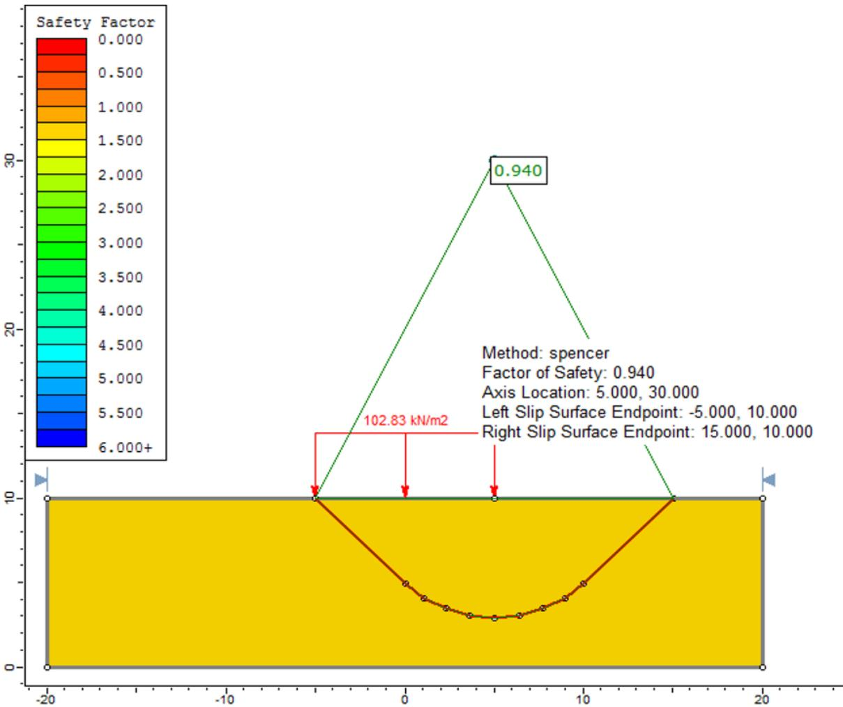
Figure 26.2: Non-Circular failure surface, by using the Spencer method
