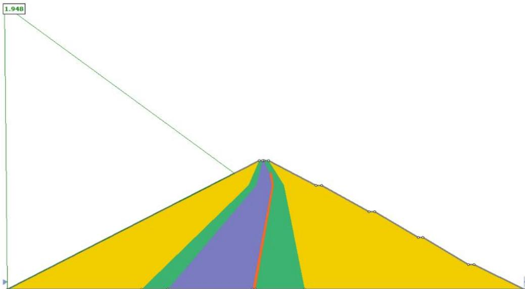
Figure 5.6: Solution, using the Janbu corrected method
