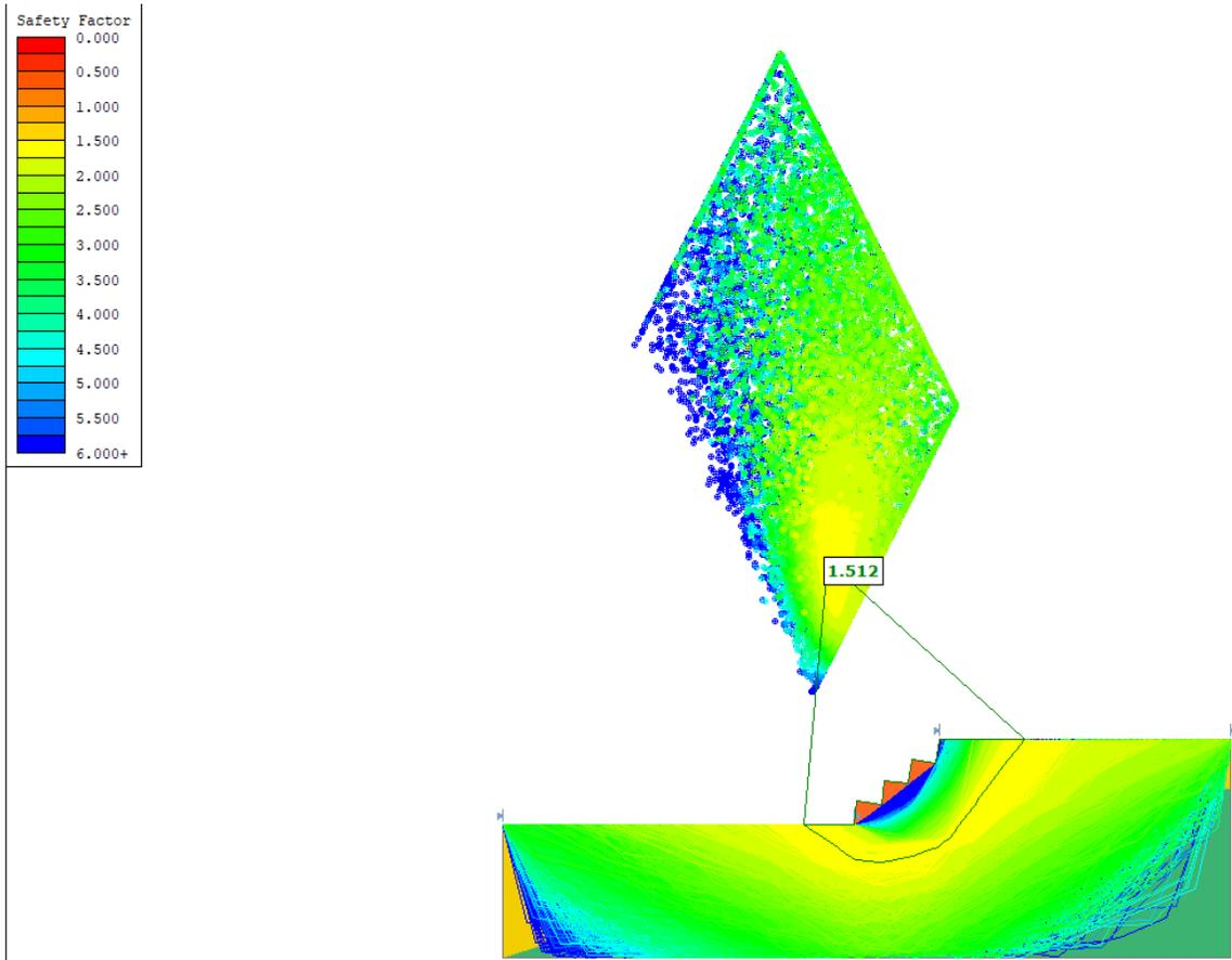
Figure 108.4: Solution for Equivalent Cohesion Method Using Cuckoo Search and Bishop Method
