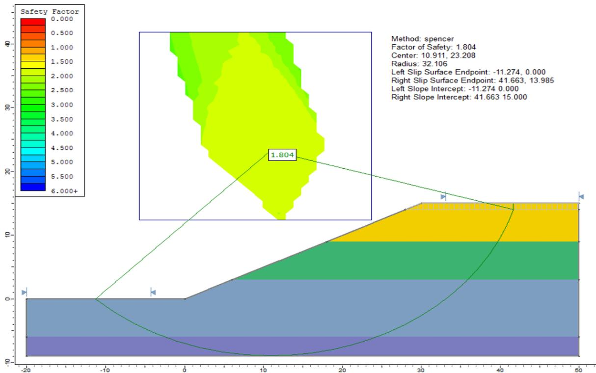
Figure 52.4: Surface 3(dry condition), using the Spencer method
