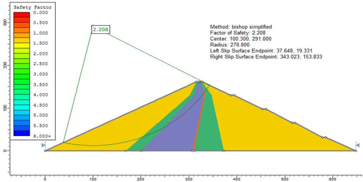
Figure 6.3: Solution, using the Bishop simplified method
