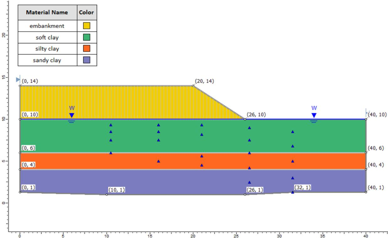
Figure 12.1: Geometry Setup in Slide
