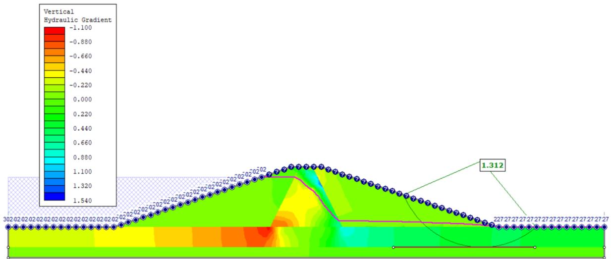
Figure 72.5: Solution to Case 2(a), using the Spencer method
