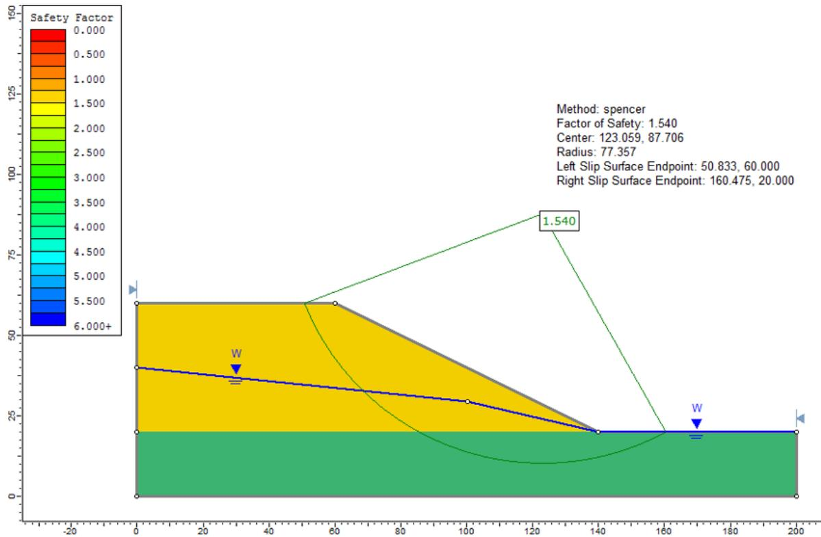
Figure 82.2: Solution, using the Spencer method
