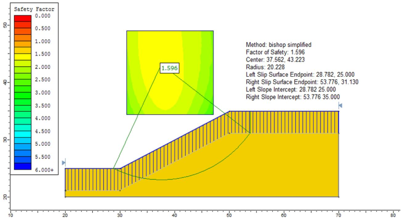
Figure 2.2: Solution, using the Bishop simplified method
