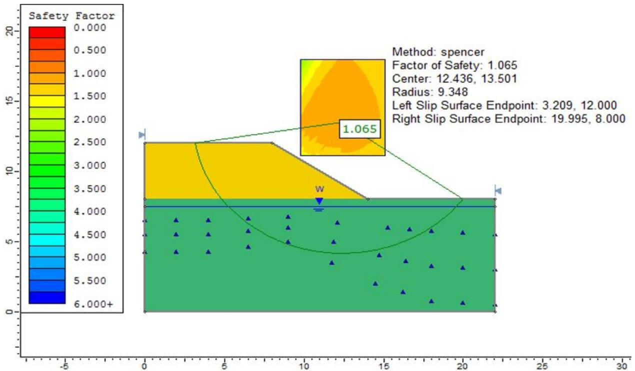
Figure 11.3: Solution, using the Spencer method
