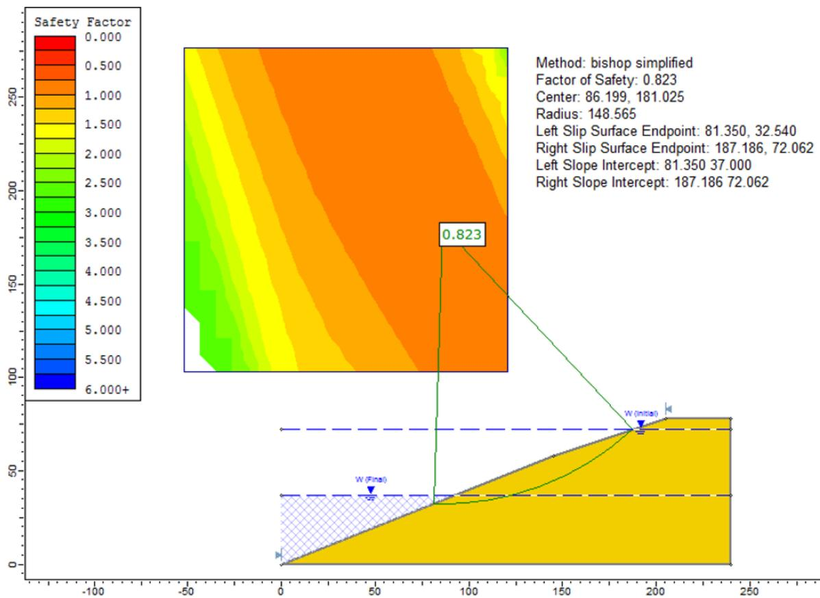
Figure 97.2: Solution, using the Army Corp. Eng. 2-stage rapid drawdown method
