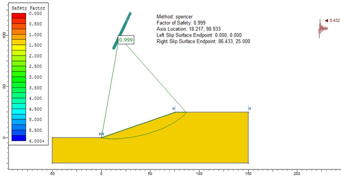
Figure 62.3: Non-circular slip surface, using the Spencer method
