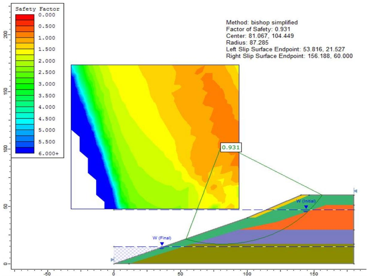
Figure 98.2: Solution, using the Army Corp. Eng. 2-stage rapid drawdown method
