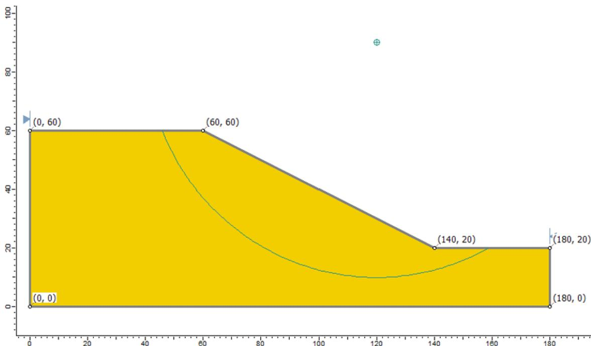
Figure 21.1: Geometry Setup in **Slide**
