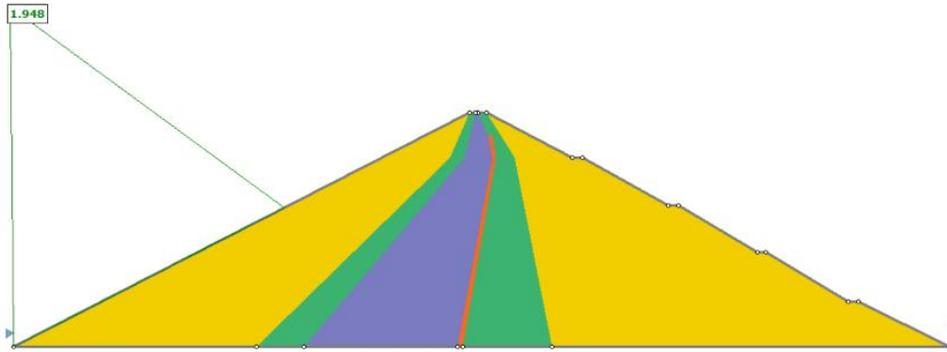
Figure 5.4: Solution, using the Spencer method
