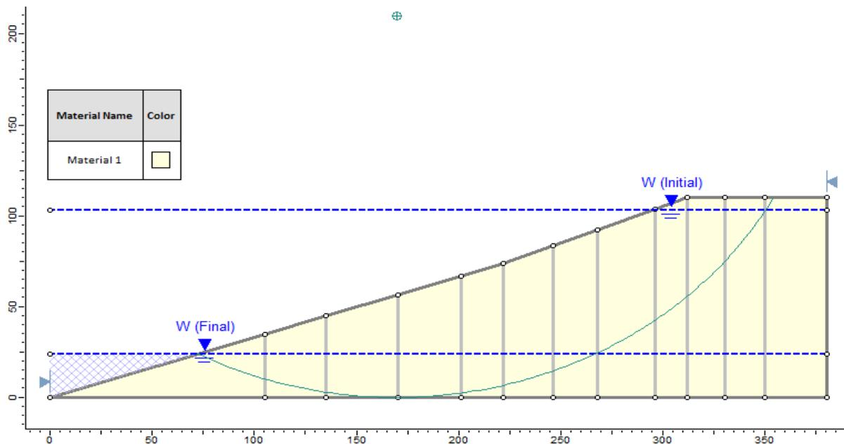
Figure 95.1: Slope Subjected to Rapid Drawdown in **Slide**
