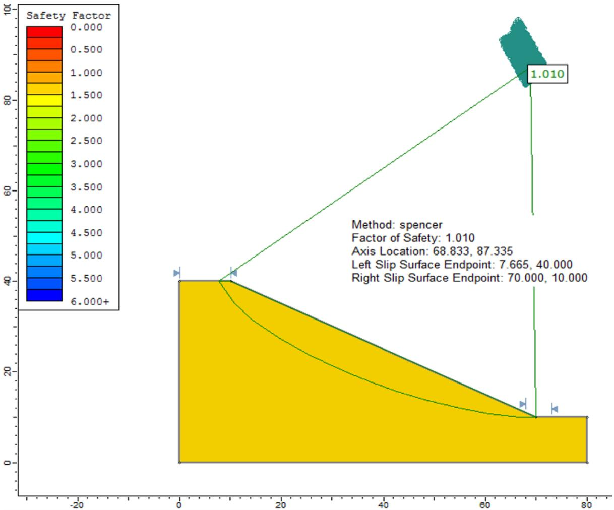
Figure 18.2: Noncircular failure surface, using the Spencer method
