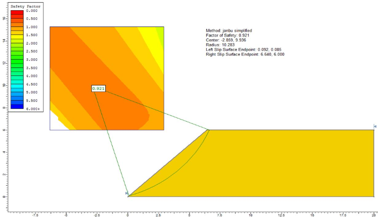
Figure 44.2: Critical failure surface, using the power curve criterion, Janbu simplified
