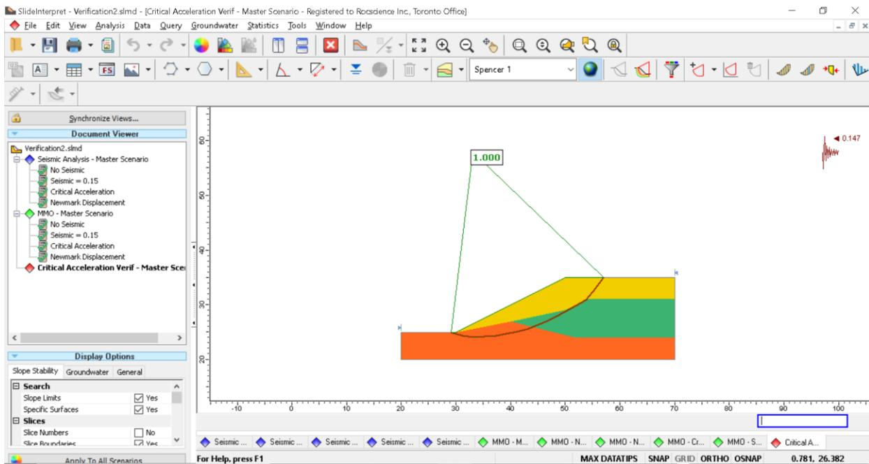
Figure 104.2:  $K_y = 0.147$  applied to corresponding surface found using MMO
