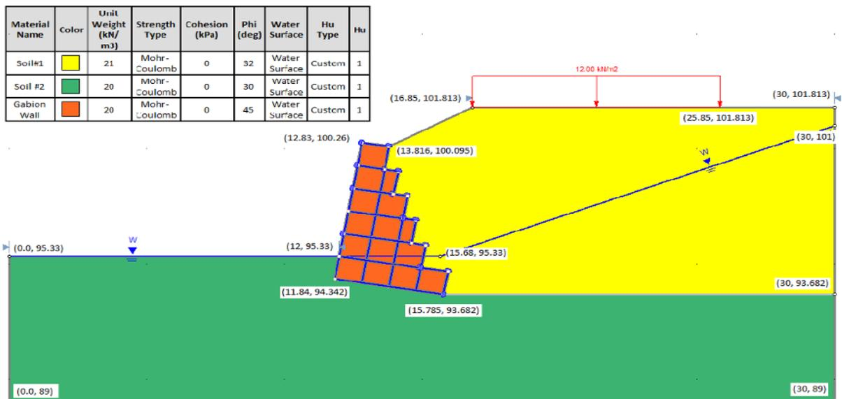
Figure 107.4: Gabion Wall Model in **Slide** (mesh method)
