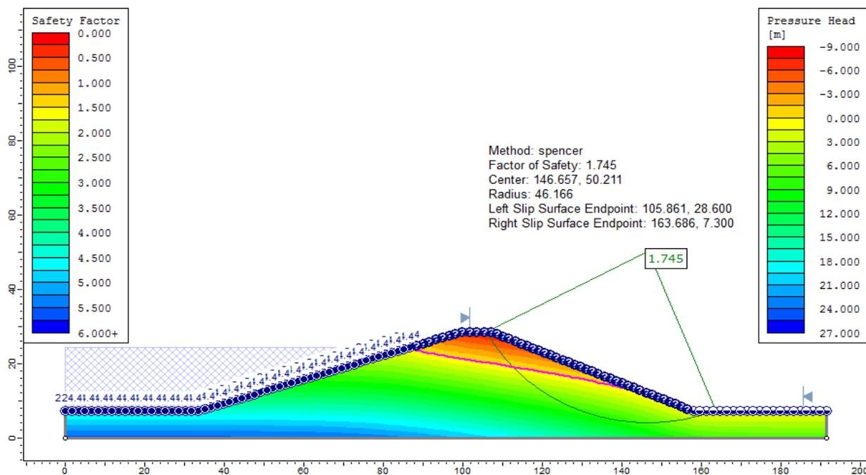
Figure 102.3: **Slide** Results for Initial Conditions, using the Spencer method
