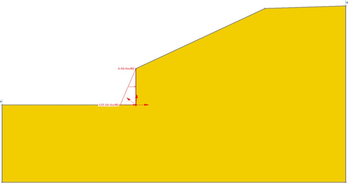
Figure 110.2: Triangular distributed load used for verification
