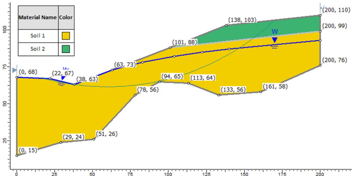
Figure 27.1: Geometry Setup in *Slide*
