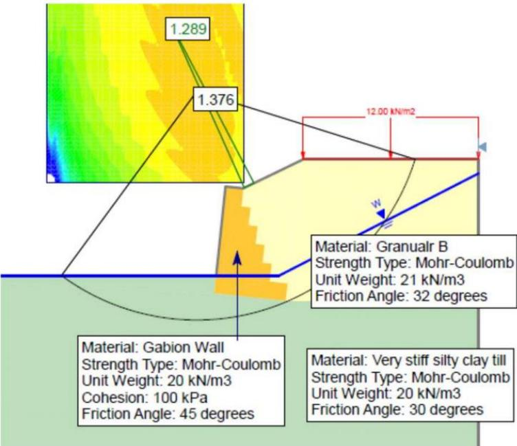
Figure 107.2: Slide model of gabion wall provided by Cao et Al. (2016)
