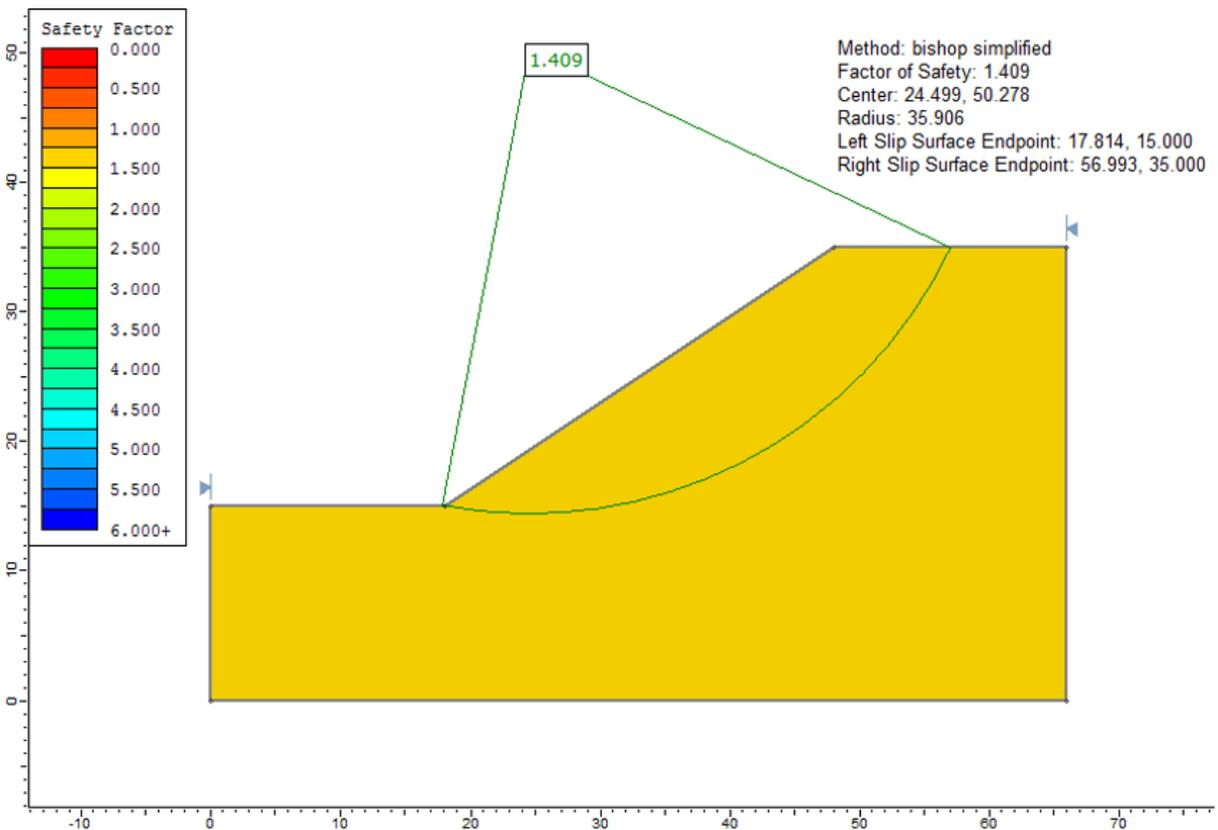
Figure 14.2: Solution, using the Bishop simplified method
