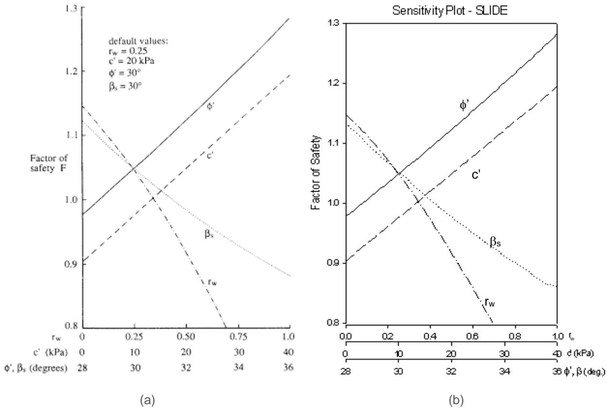
Figure 53.2 Comparison for sensitivity results in  $r_w$ ,  $c'$ ,  $\phi'$  and  $\beta_s$ : (a) Reference's results from Priest (1993); (b) results from **Slide**
