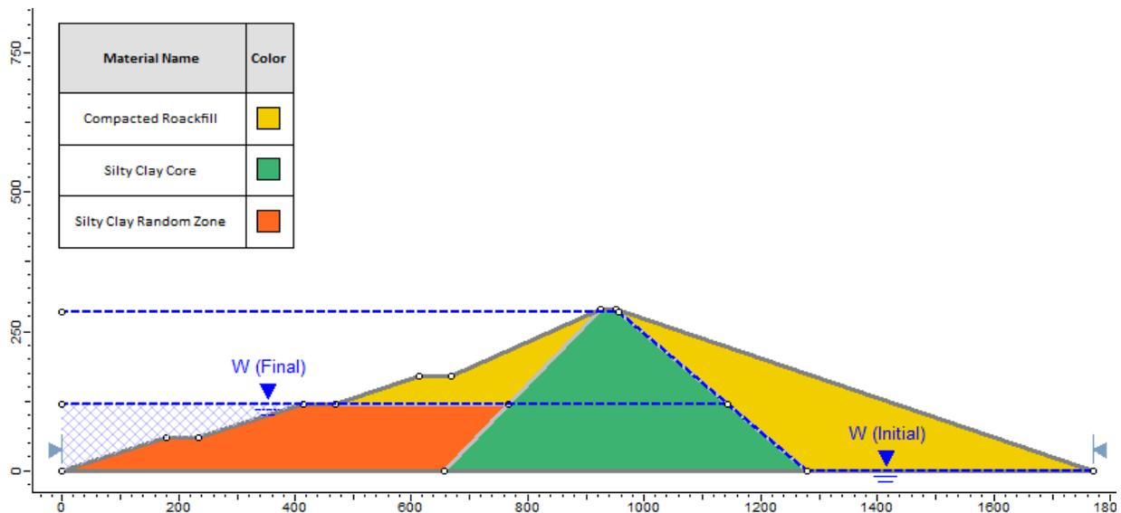
Figure 99.1: Pumped Storage Project Dam Model
