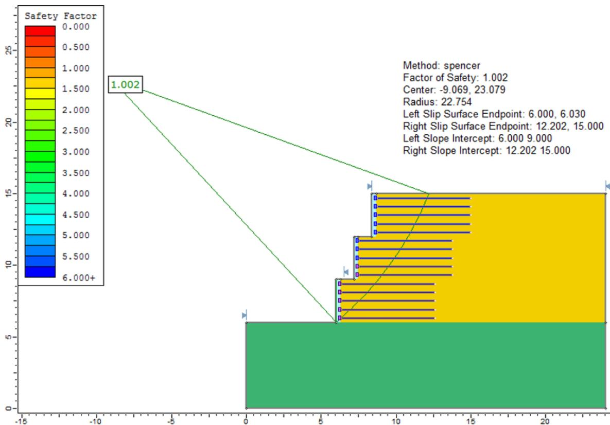
Figure 90.2: Solution, using the Spencer method
