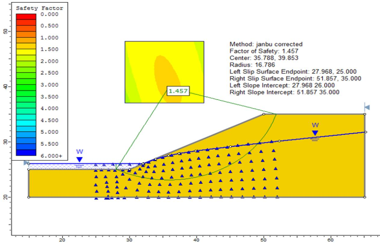
Figure 10.6: Solution, using the Janbu corrected method
