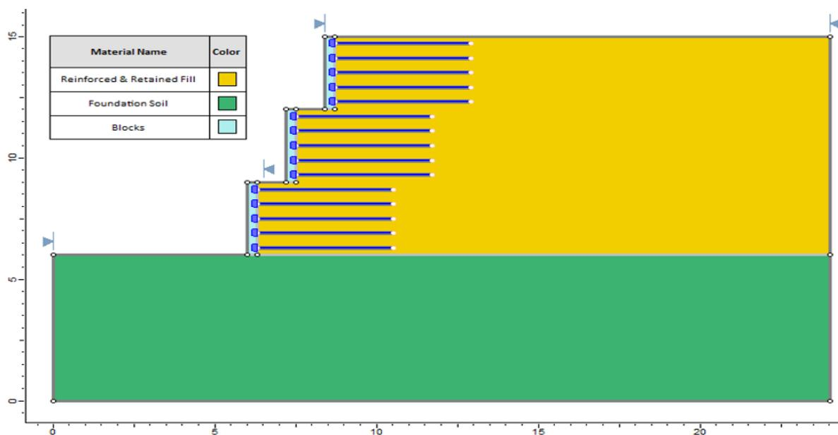
Figure 89.1: A Three-tiered Wall in **Slide**
