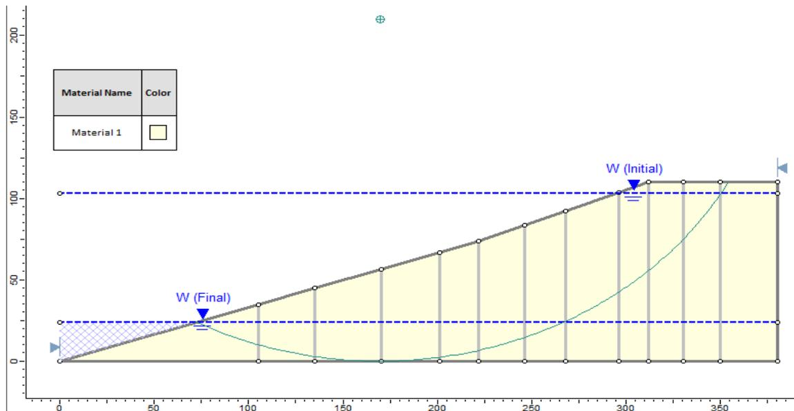
Figure 96.1: Slope Subjected to Rapid Drawdown
