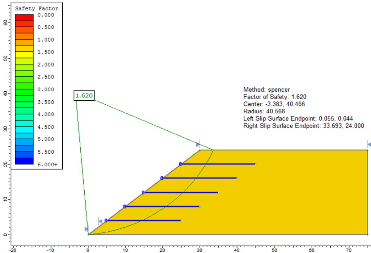
Figure 86.2: Solution, using the Spencer method
