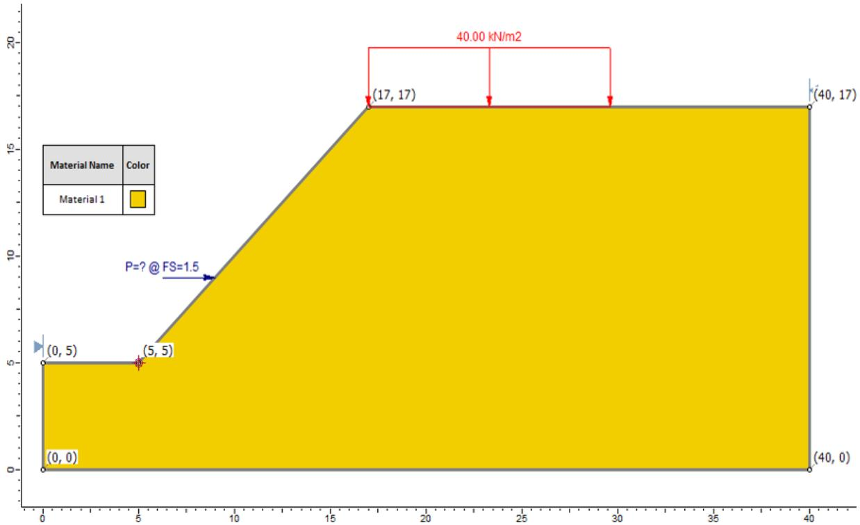
Figure 37.1: Geometry Setup in **Slide** (back analysis)
