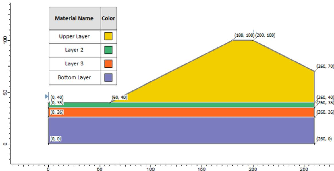
Figure 19.1: Geometry Setup in **Slide**
