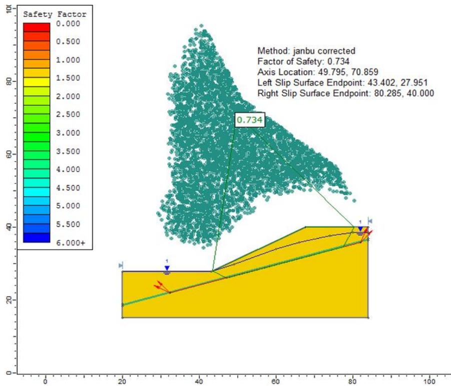
Figure 9.4: Solution, using the Janbu correction method
