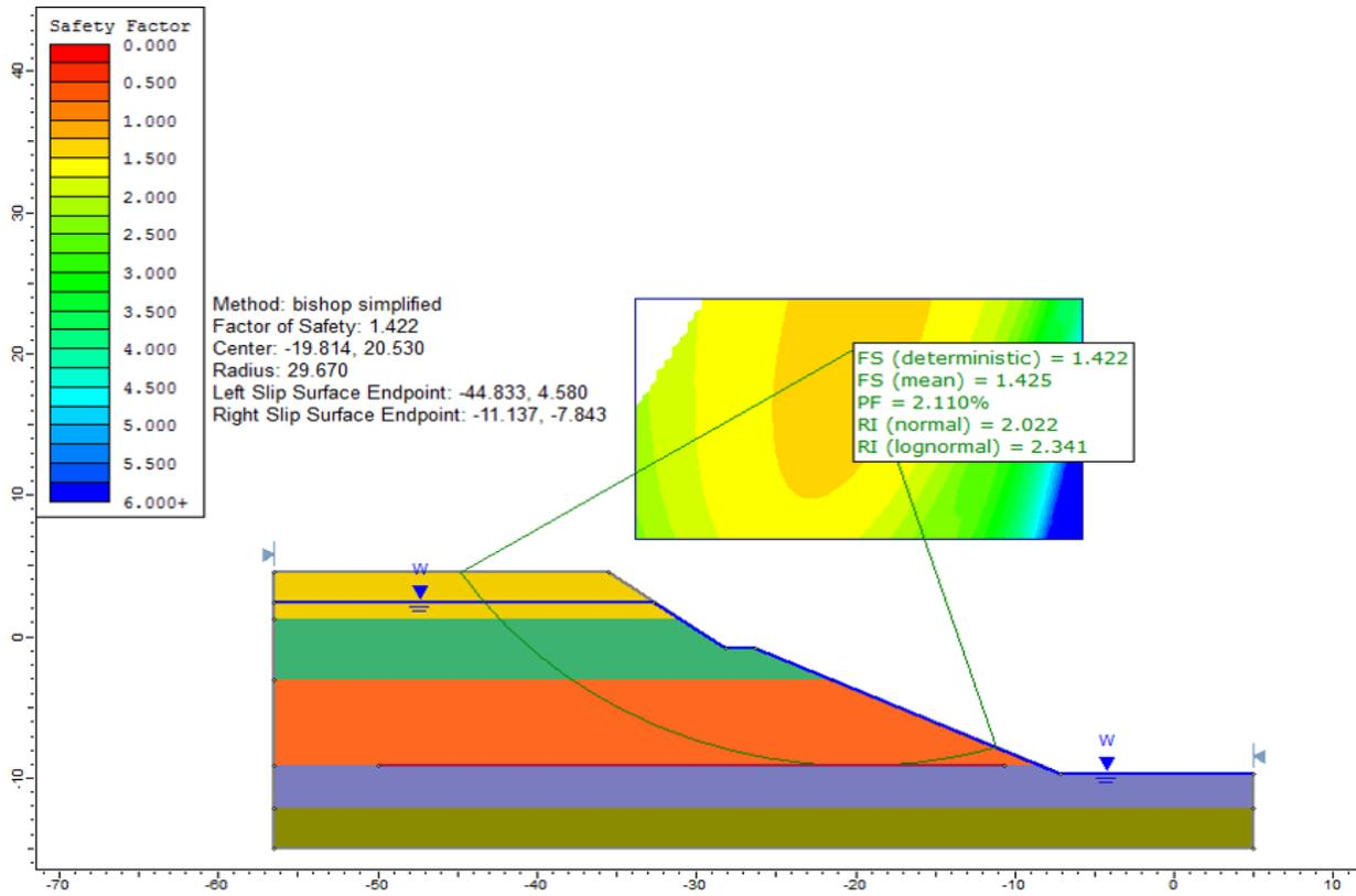
Figure 28.9: Critical slip circle tangential to lower boundary of clay layer 2
