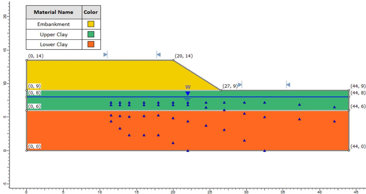
Figure 13.1: Geometry Setup in **Slide**
