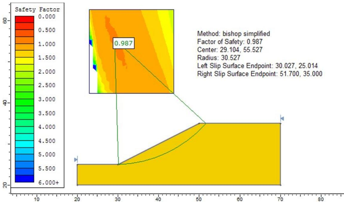
Figure 1.2: Solution, using the Bishop simplified method
