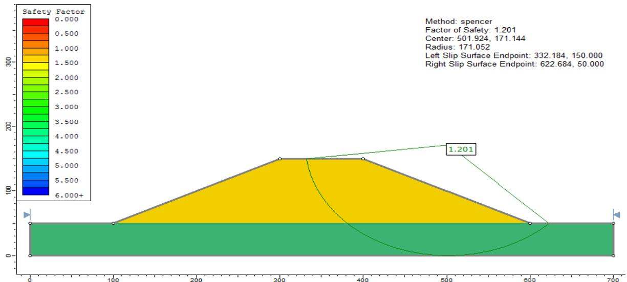
Figure 74.2: Solution, using the Spencer method (Circular)
