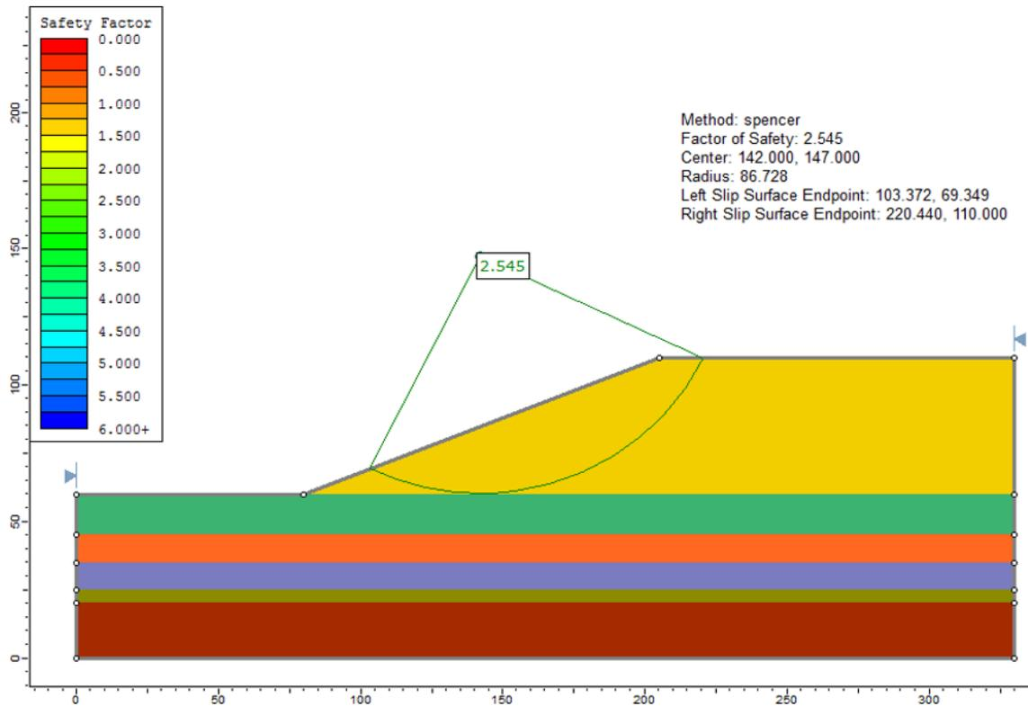
Figure 80.2: Solution to Case 1, using the Spencer method
