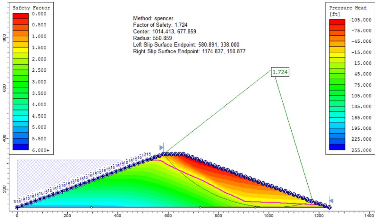
Figure 77.3: Solution to Case 1, using the Spencer method
