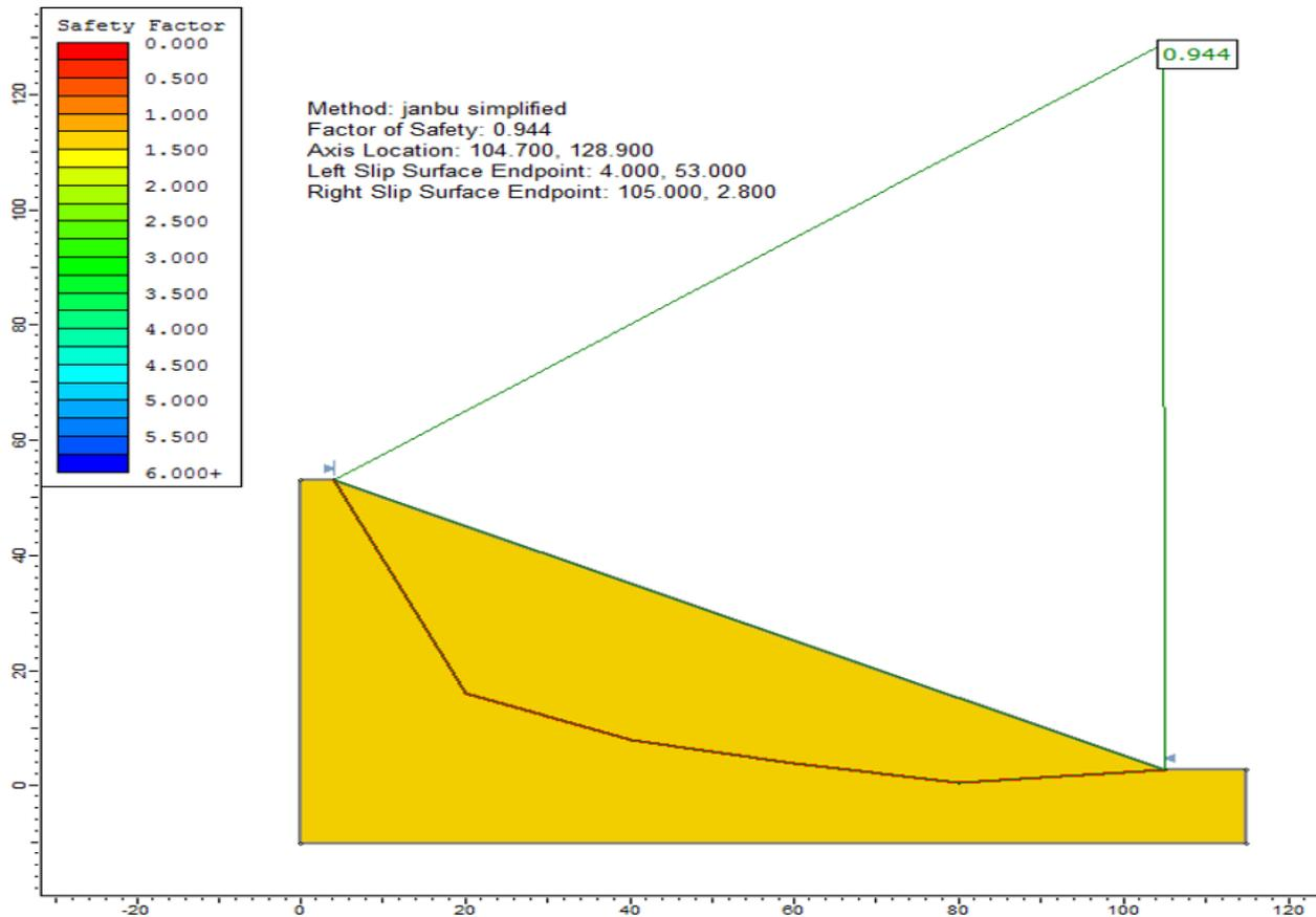
Figure 40.2: Solution, using the Bishop simplified method
