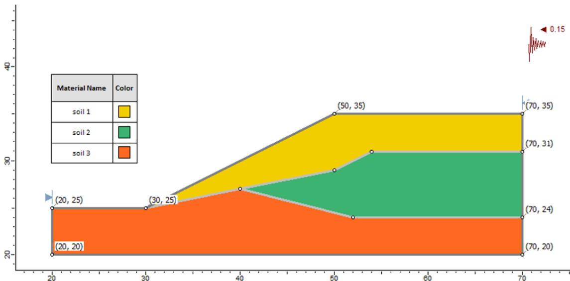
Figure 4.1: Geometry Setup in Slide
