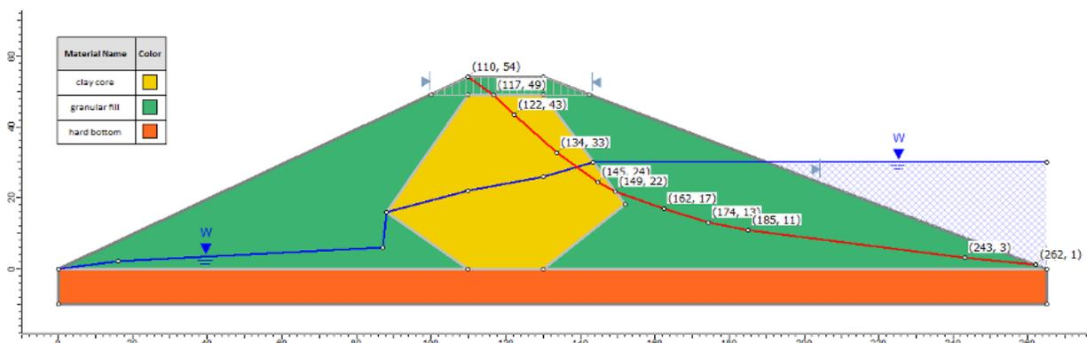
Figure 42.2: Location of noncircular failure surface
