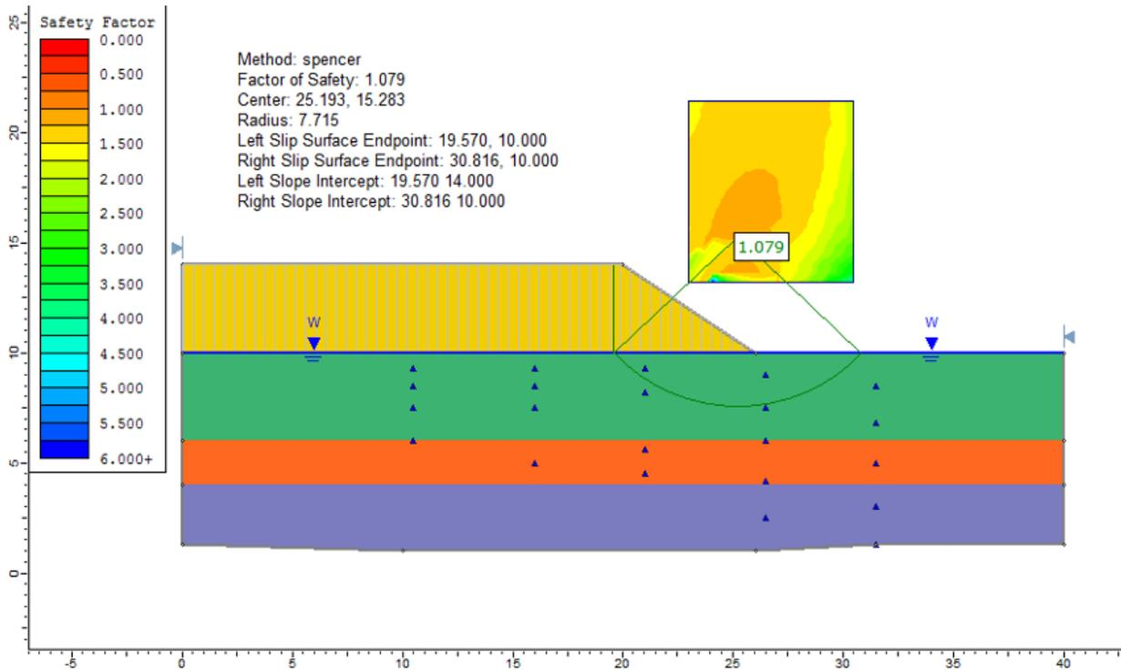
Figure 12.3: Solution, using the Spencer method
