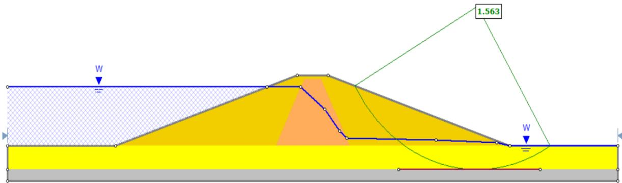
Figure 72.6: Solution to Case 2(b), using the Bishop method
