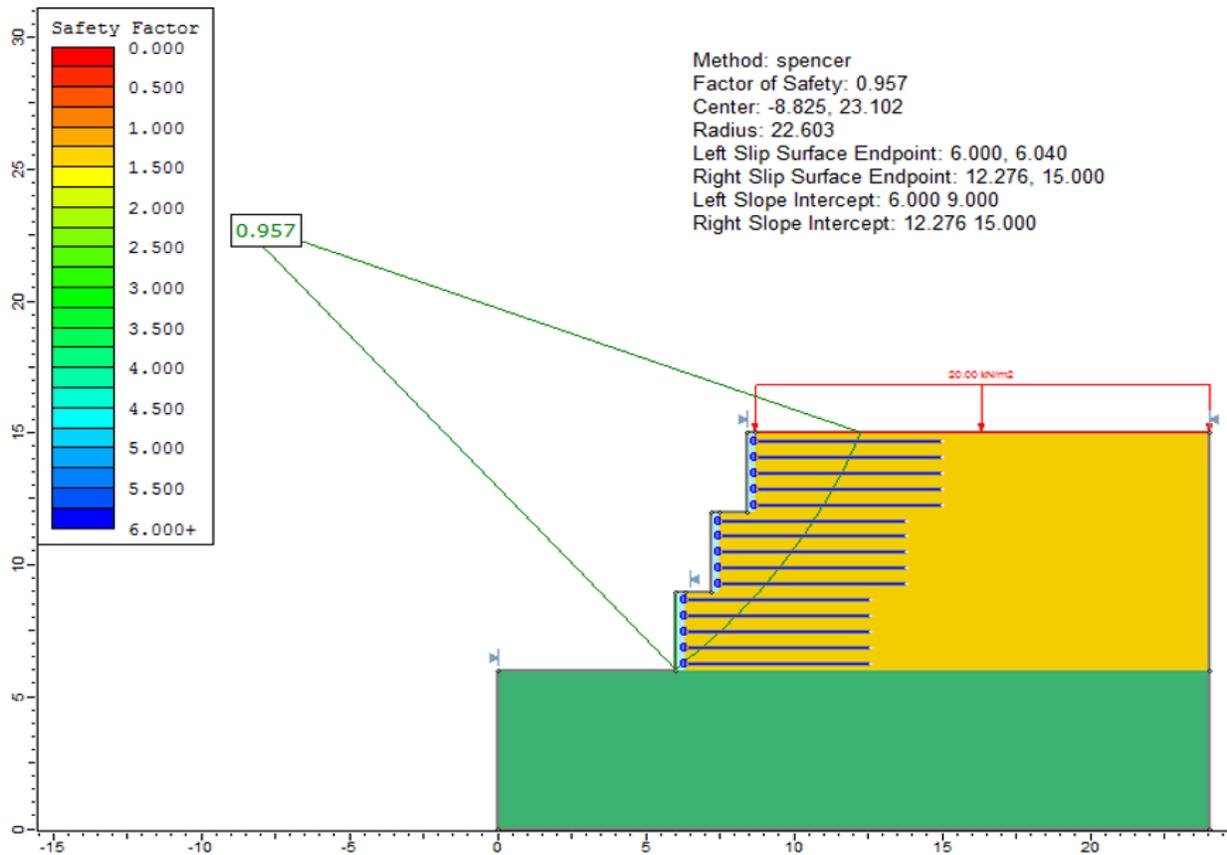
Figure 93.2: Solution, using the Spencer method
