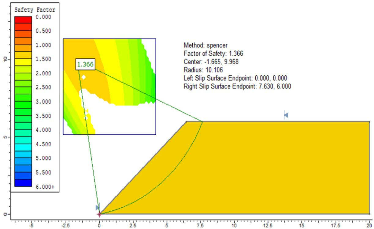
Figure 61.3: Circular critical surface with Mohr-Coulomb criteria, Spencer method
