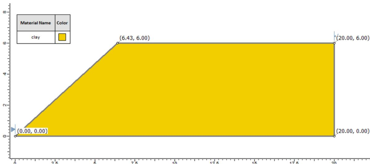
Figure 44.1: Geometry Setup in **Slide**
