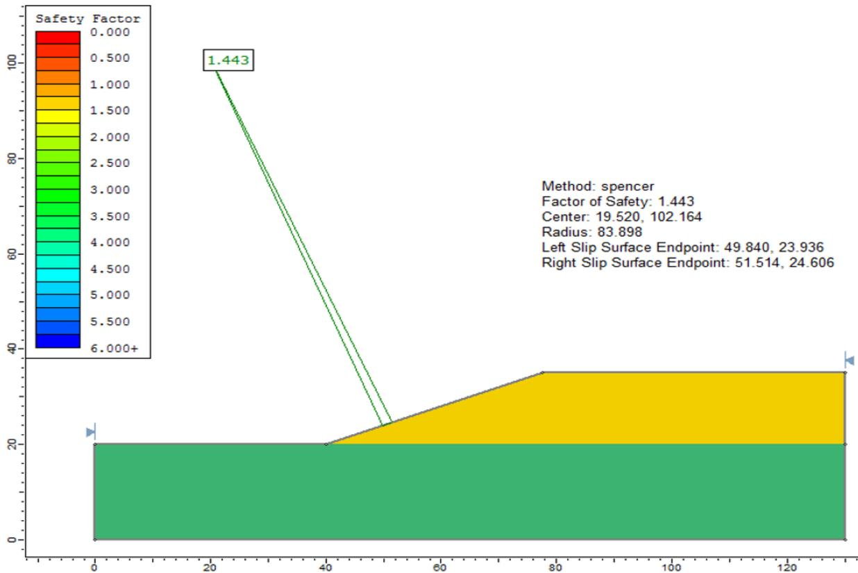
Figure 79.3: Solution to Case 2, using the Spencer method
