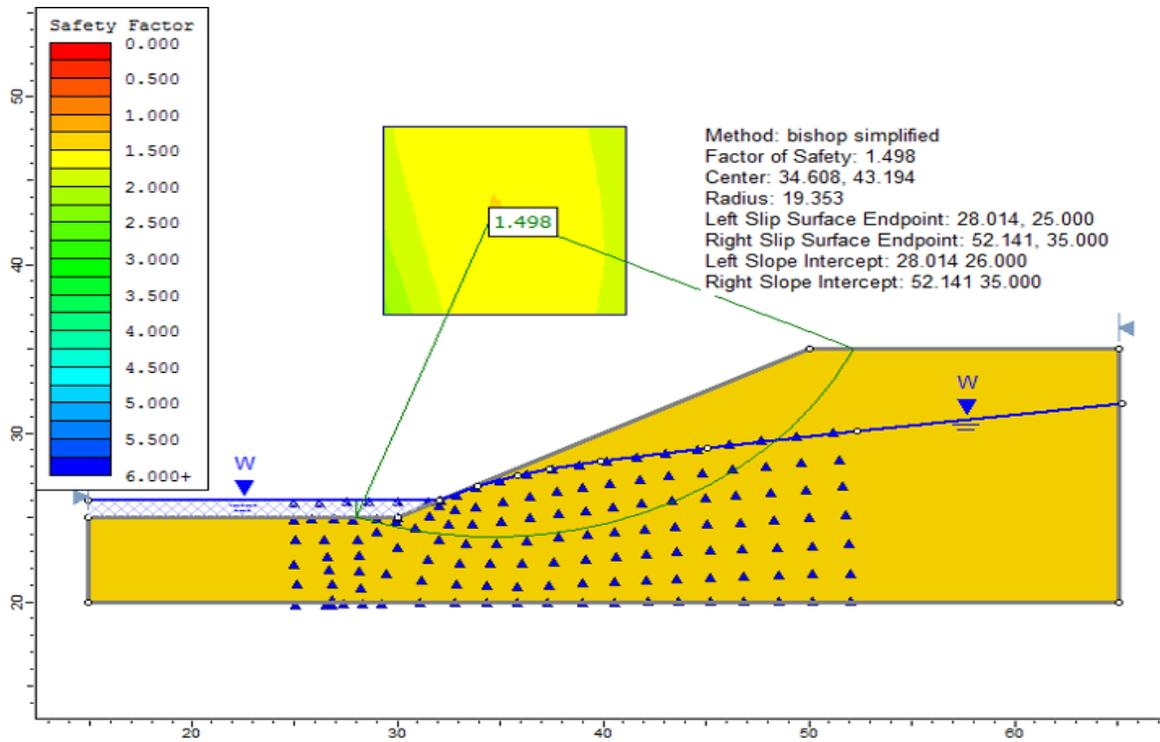
Figure 10.3: Solution, using the Bishop simplified method
