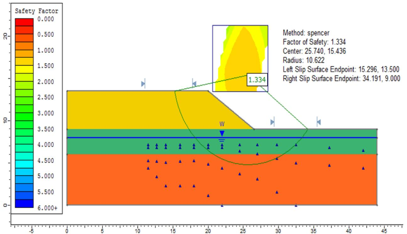
Figure 13.3: Solution, using the Spencer method
