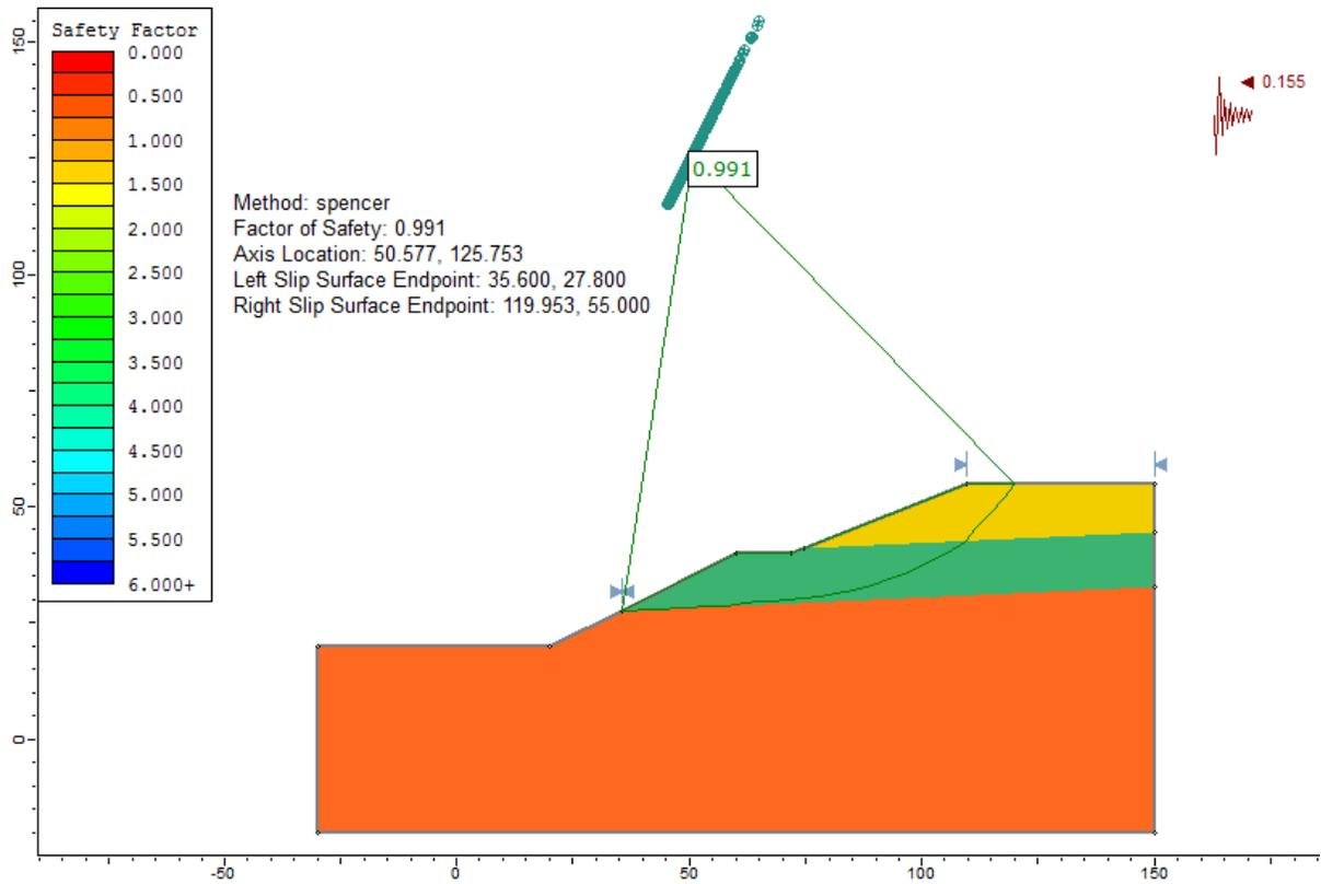
Figure 63.2: Critical slip surface, using the Spencer method
