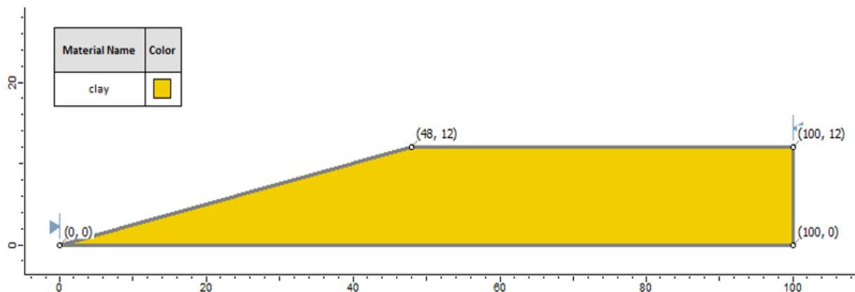
Figure 45.1: Geometry Setup in **Slide**
