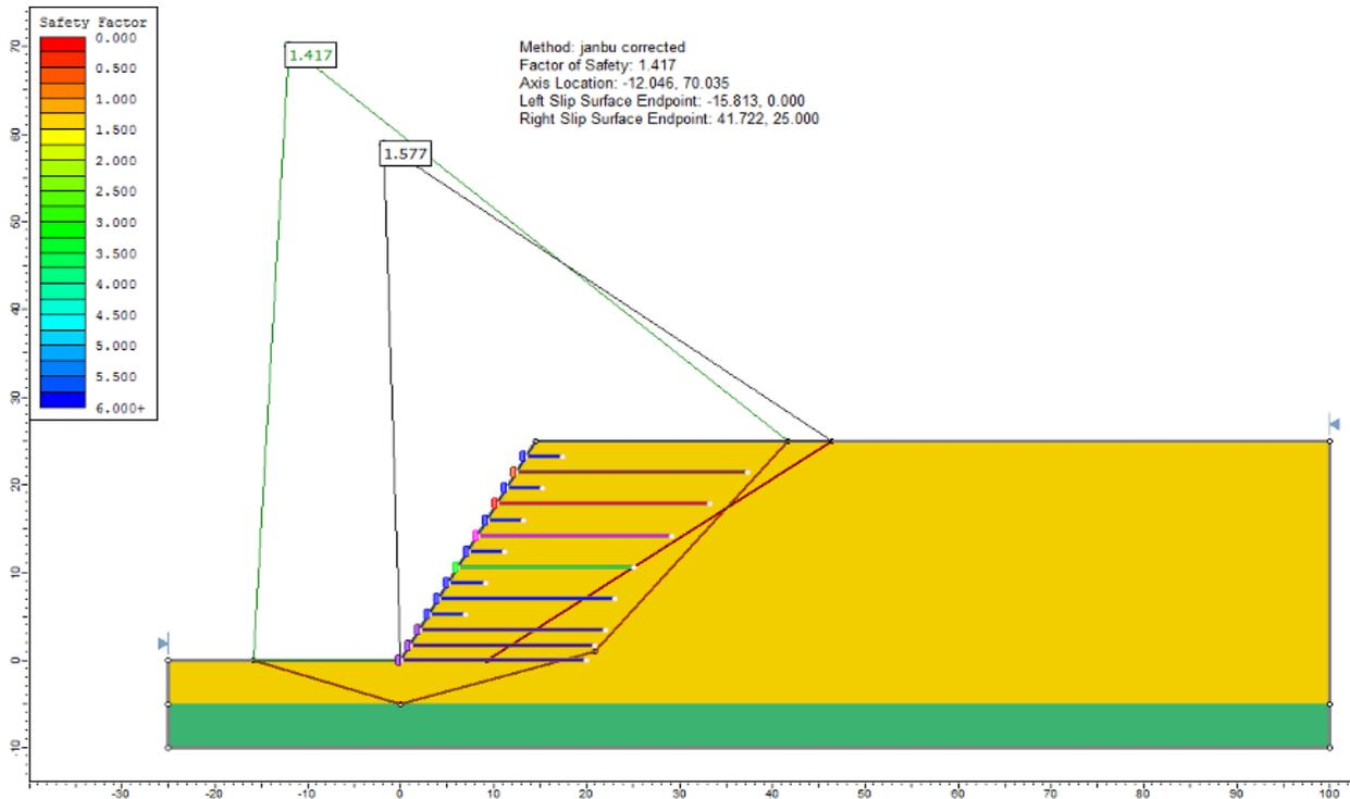
Figure 50.2: Safety factors for the given failure surfaces
