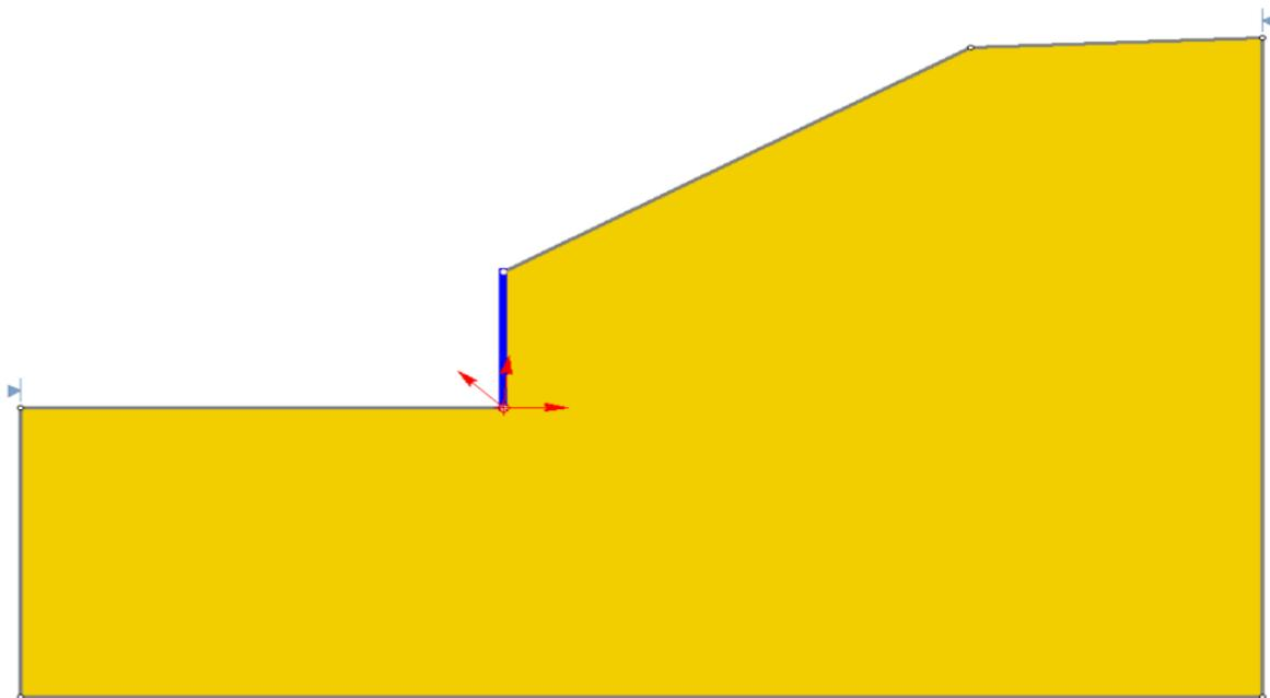
Figure 110.1: Cantilevered Retaining Wall (triangular pressure profile)
