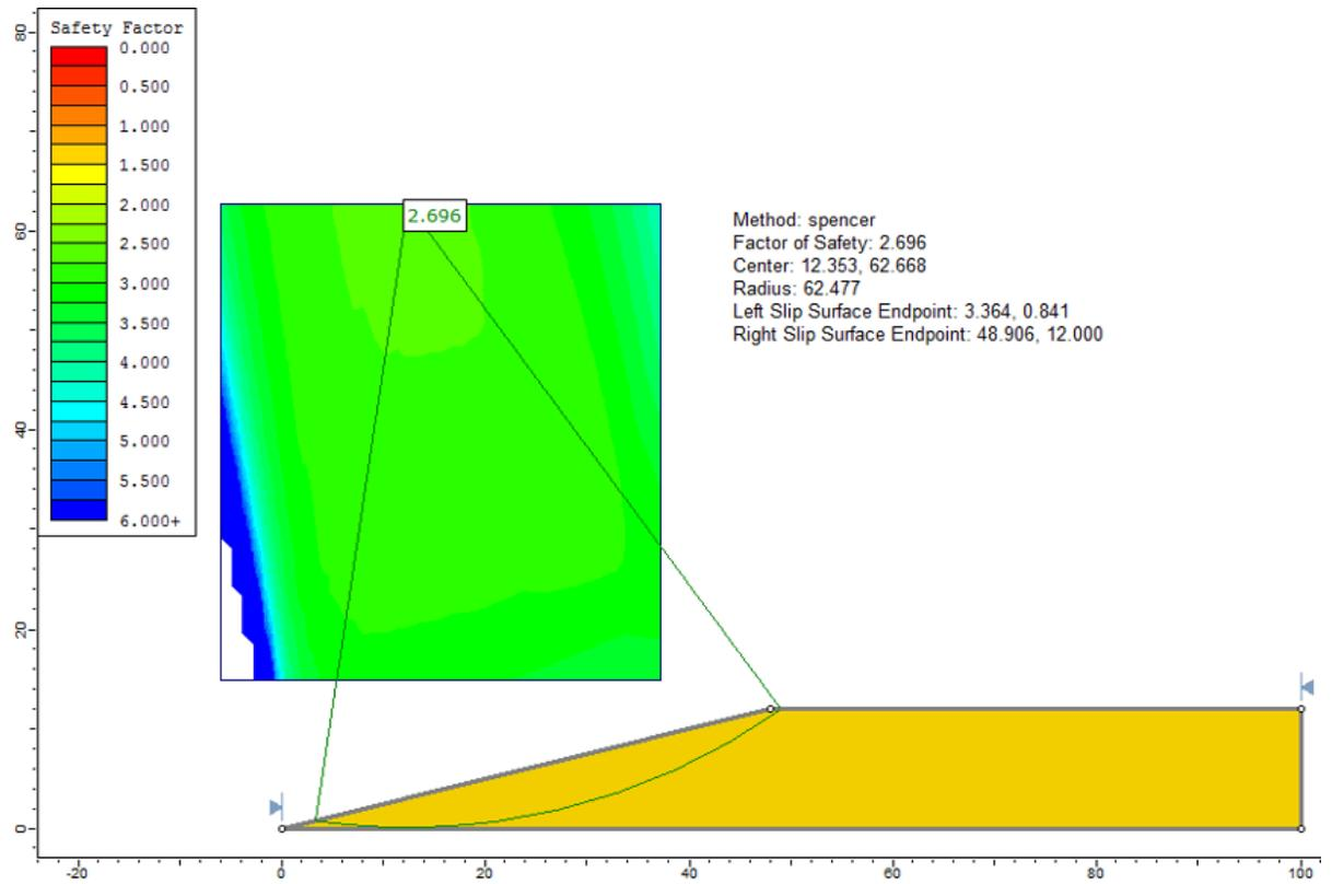
Figure 45.4: Mohr-Coulomb criterion with iterations, Spencer
