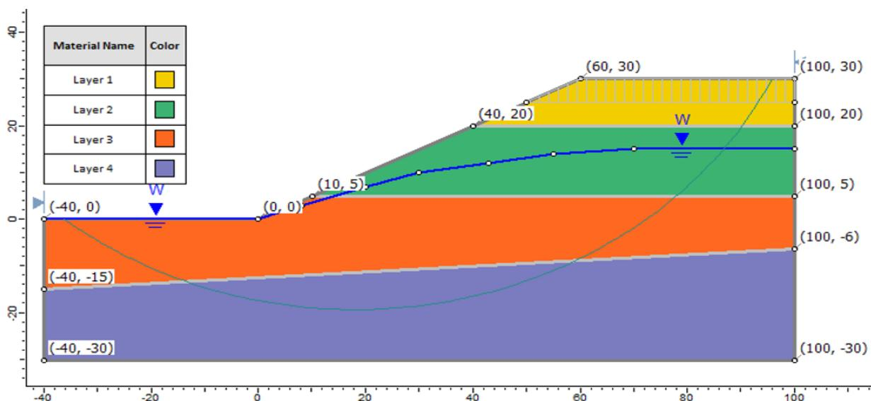
Figure 51.1: Geometry Setup in **Slide**
