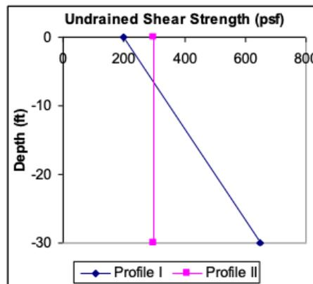
Figure 83.1: Undrained Shear Strength Profiles from Duncan and Wright (2005)
