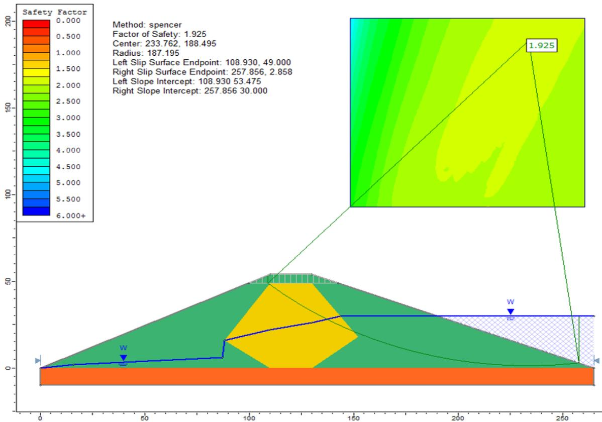
Figure 42.3: Safety map featuring global minimum zone using Spencer method
