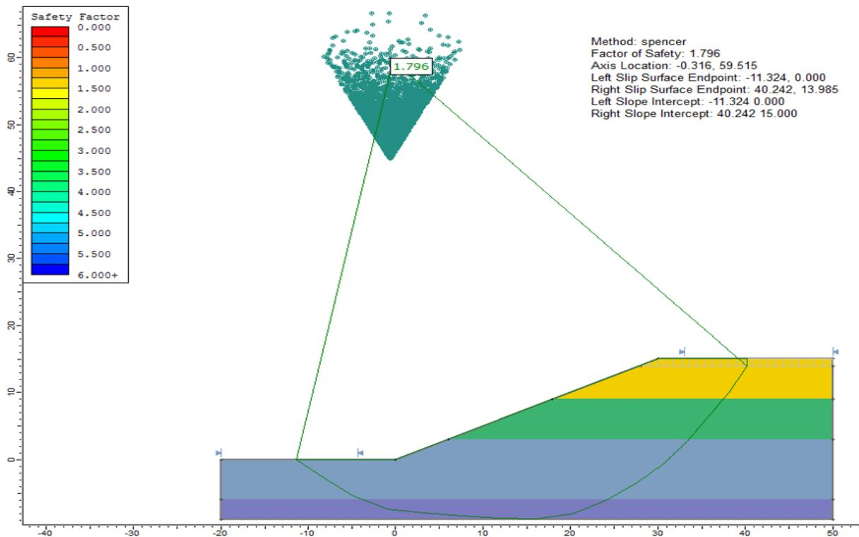
Figure 52.5: Surface 4 (dry condition), using Spencer method
