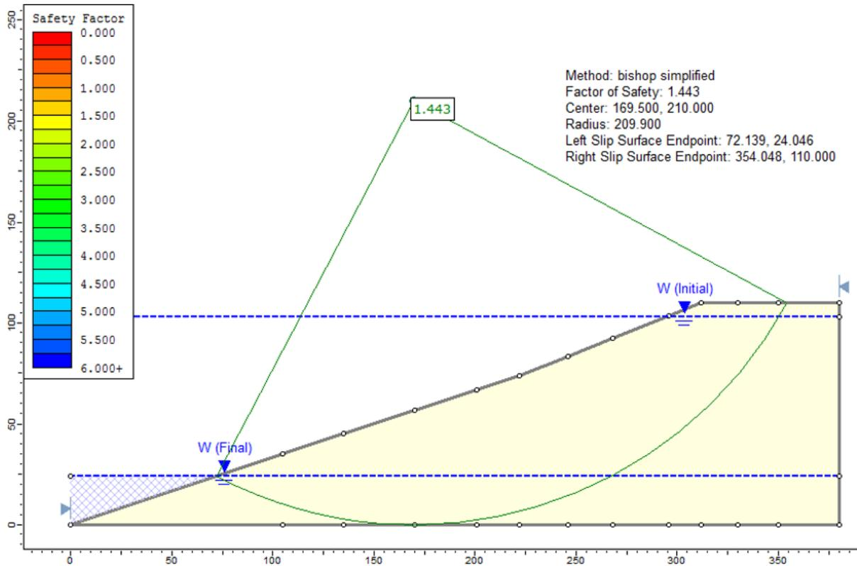
Figure 96.2: Solution, using the Duncan, Wright and Wong 3-stage rapid drawdown method
