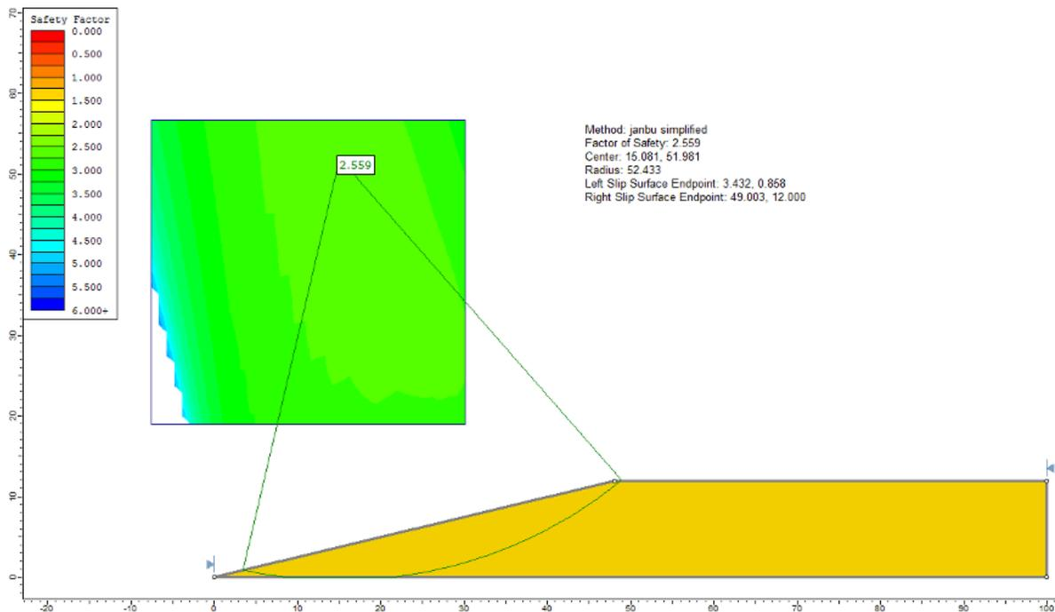
Figure 45.2: Critical failure surface, using the power curve criterion, Janbu simplified
