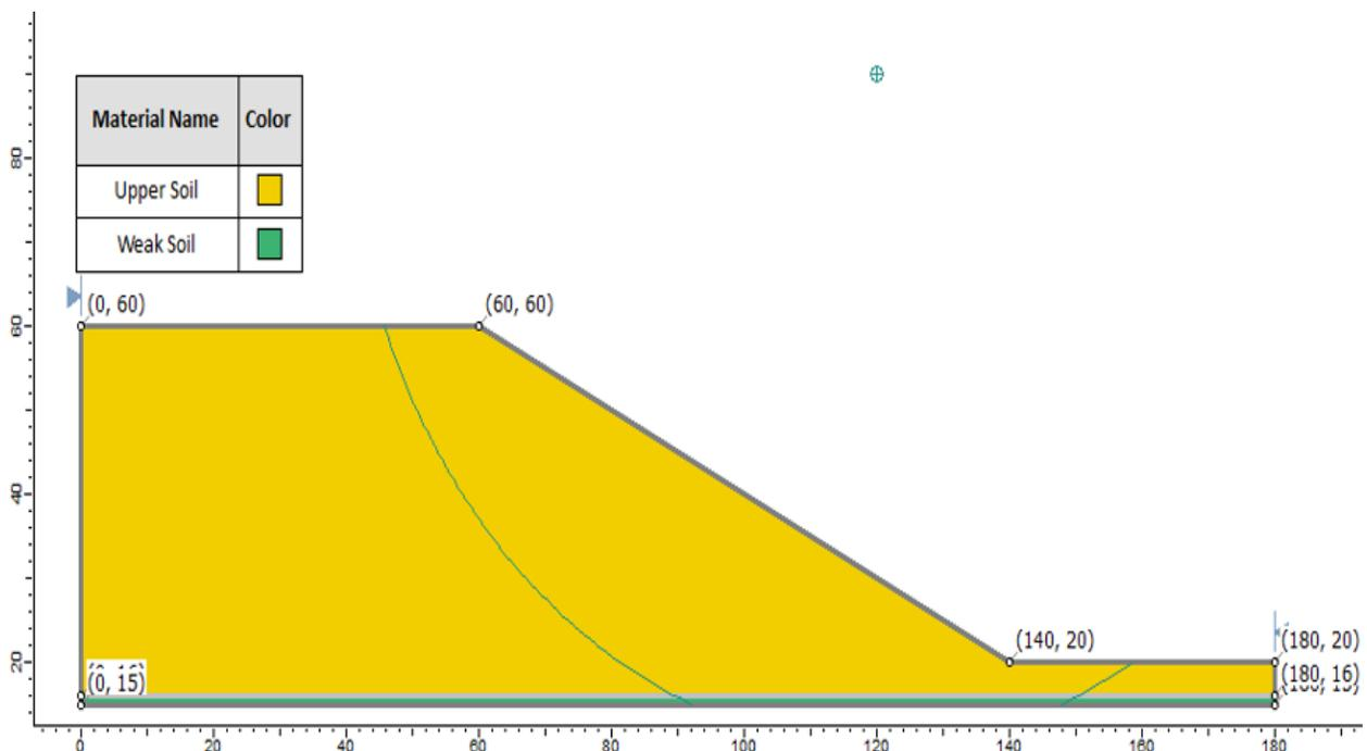
Figure 22.1: Geometry Setup in **Slide**
