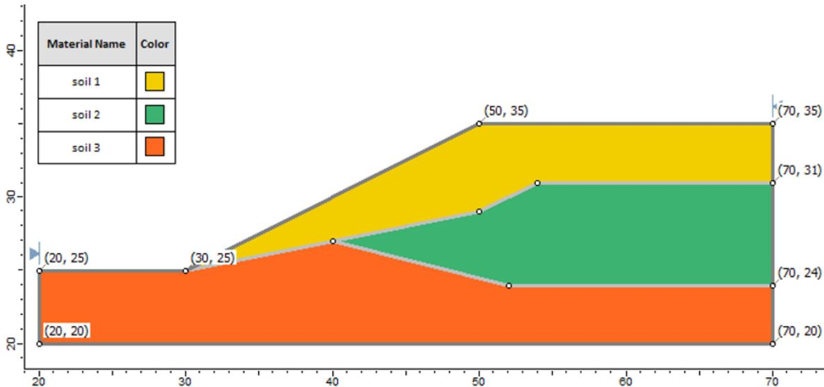
Figure 3.1: Geometry Setup in Slide
