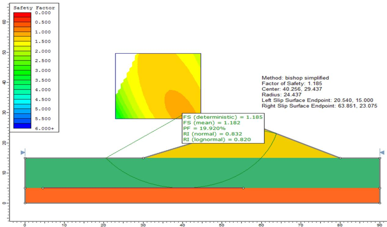
Figure 28.12: Critical slip circle tangential to lower boundary of soft foundation layer
