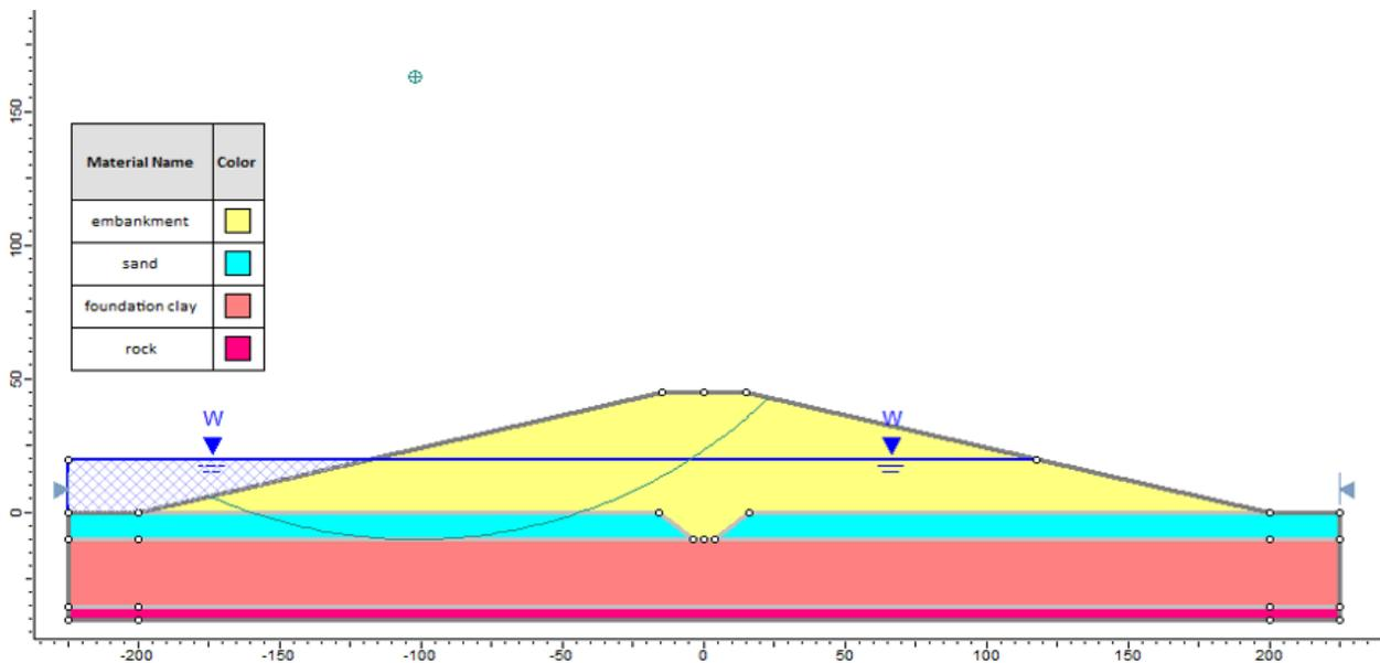
Figure 65.1: Geometry Setup in **Slide**
