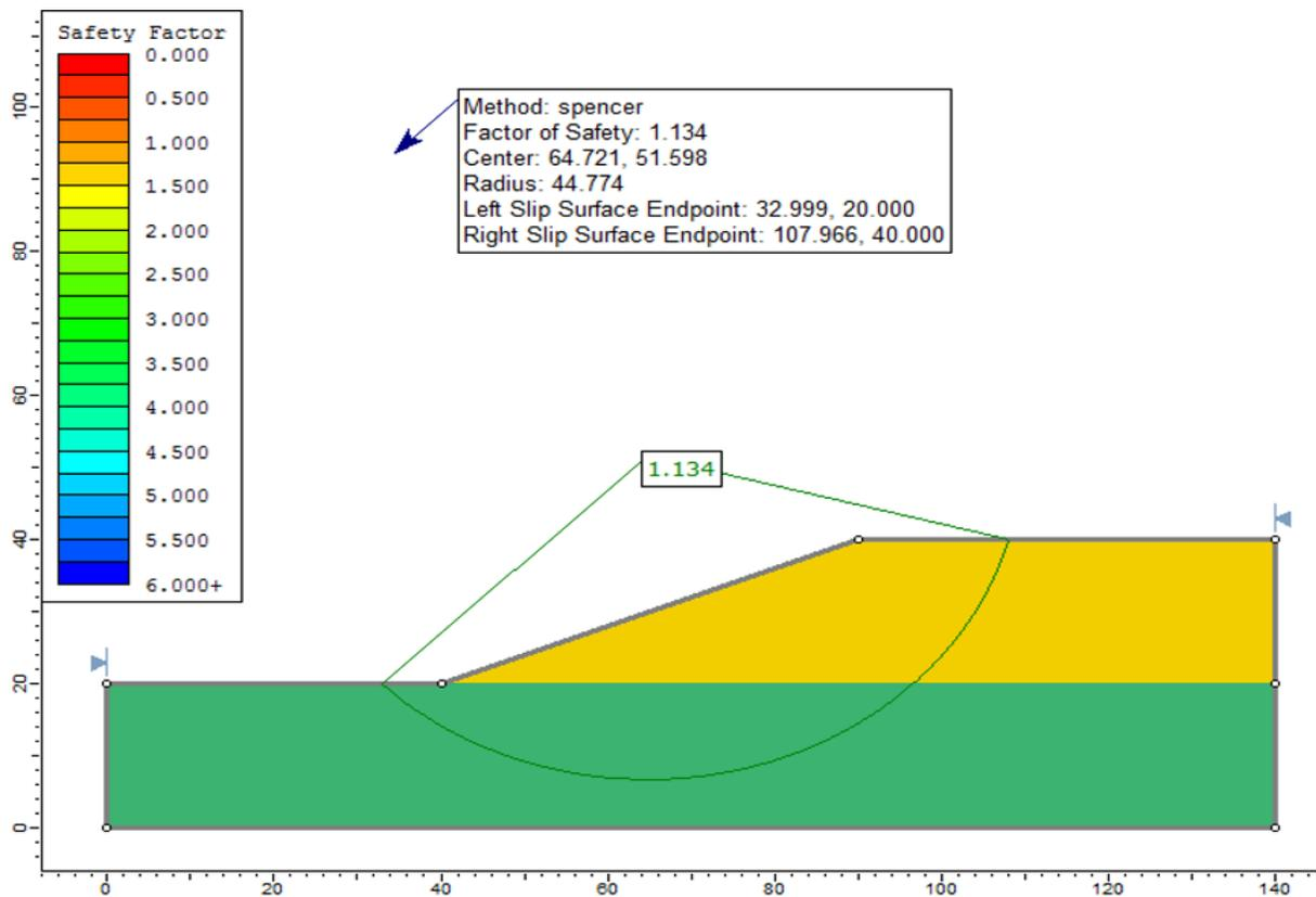
Figure 84.5: Solution to Case 4, using the Spencer method
