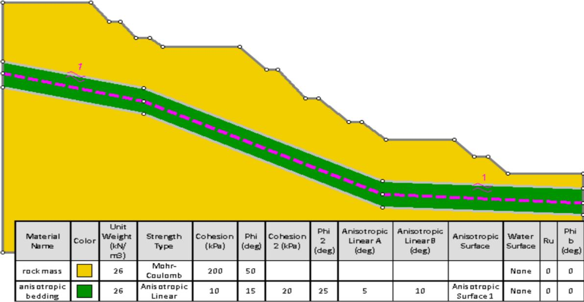
Figure 105.1: Tutorial model used in this example
