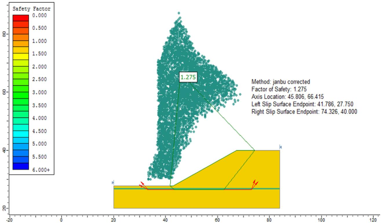
Figure 7.4: Solution, using the Janbu corrected method
