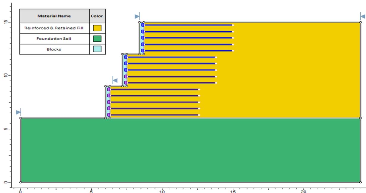
Figure 90.1: A Three-tiered Wall in **Slide**
