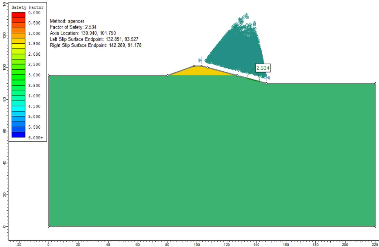
Figure 46.4: Critical failure surface, using the Spencer method
