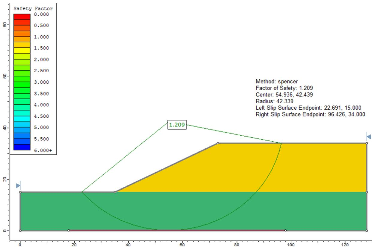
Figure 81.2: Solution for Case 1, using the Spencer method
