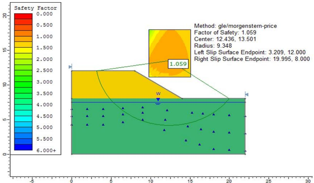
Figure 11.4: Solution, using the GLE method
