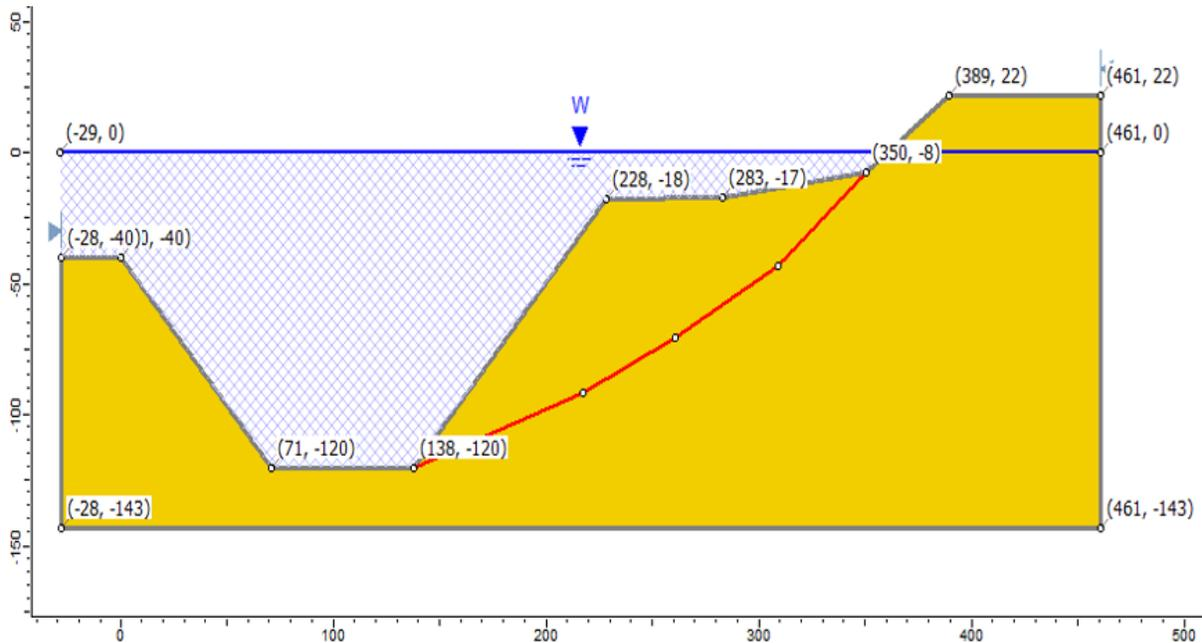
Figure 29.1: Geometry Setup in Slide
