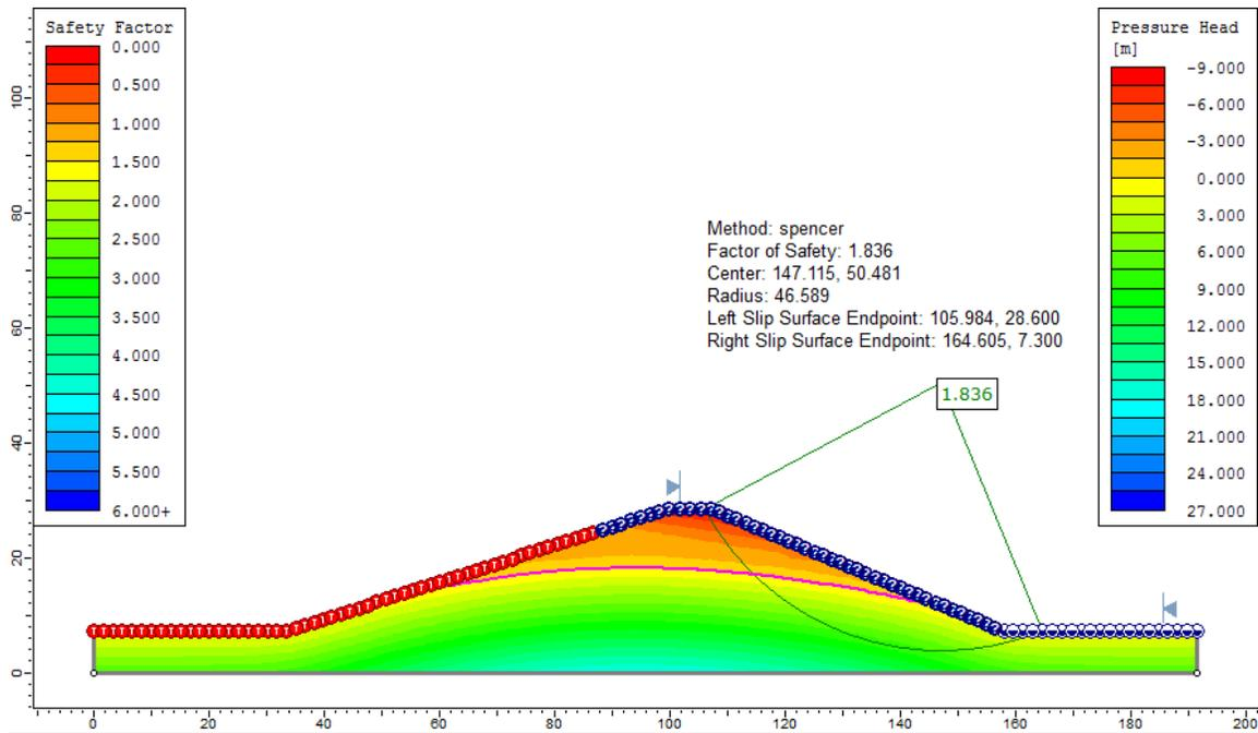
Figure 102.6: **Slide** Results for  $\phi^b = 0^\circ$  at 80 h, using the Spencer method
