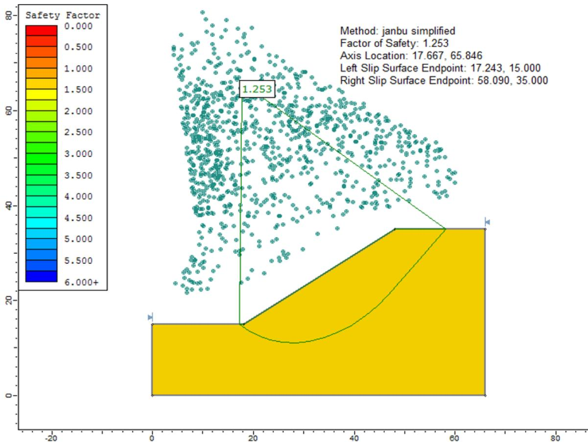
Figure 14.3: Noncircular failure surface, using the janbu simplified method
