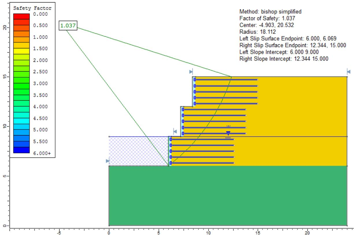
Figure 92.2: Solution, using the Bishop simplified method
