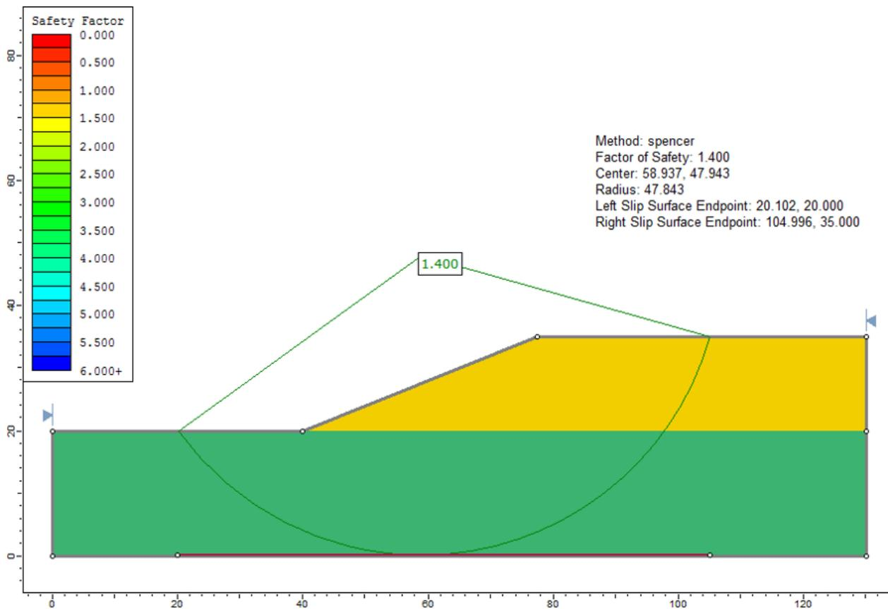
Figure 79.2: Solution to Case 1, using the Spencer method
