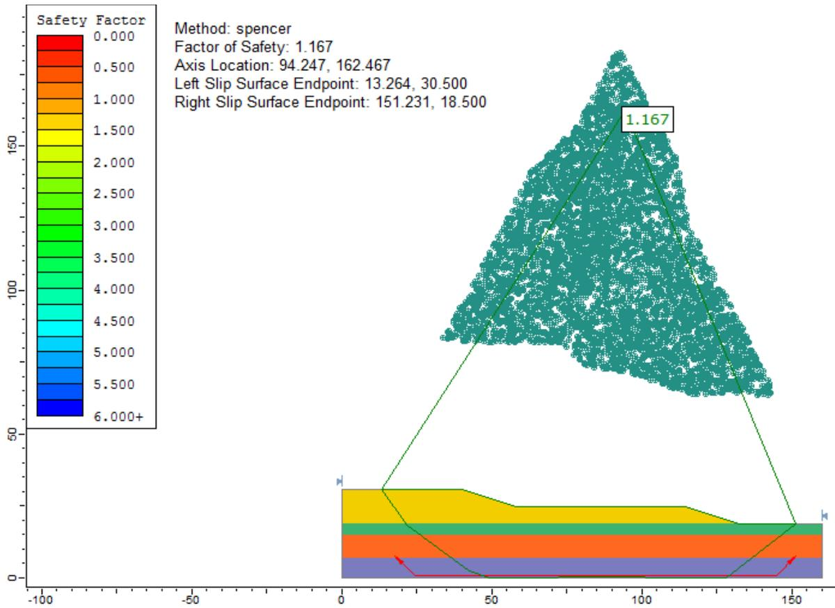
Figure 75.3: Solution to Case 2, using the Spencer method
