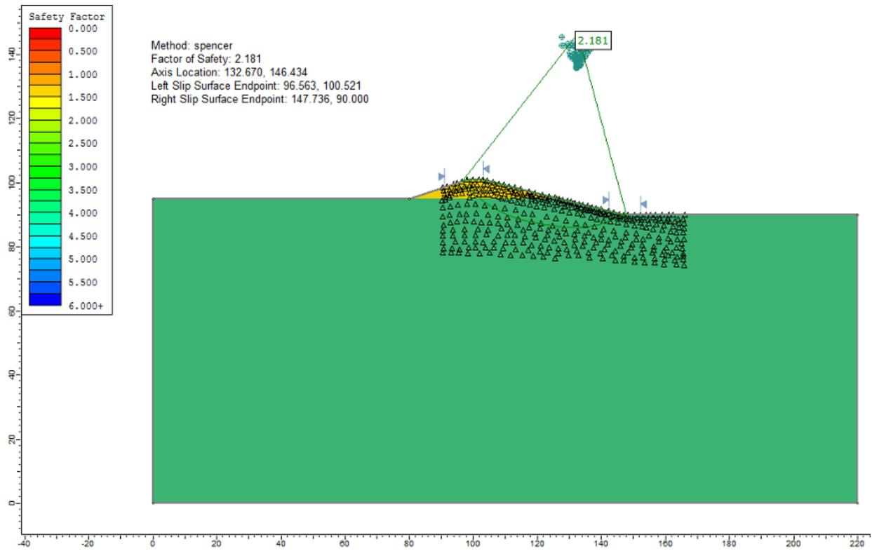
Figure 46.8: Critical failure surface, using the Spencer method
