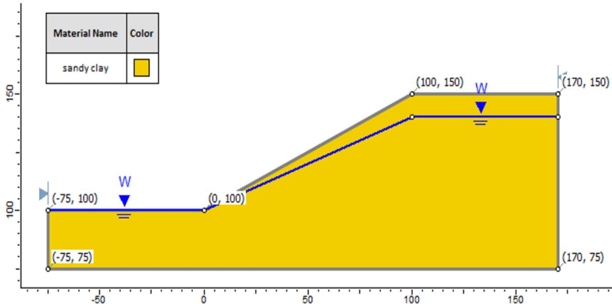
Figure 55.1: Geometry Setup in **Slide**
