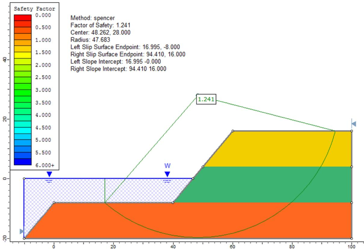
Figure 68.2: Solution, using the Spencer method
