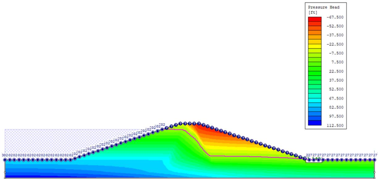
Figure 72.3: Solution to Case 1(a) (Circular), using the Bishop method
