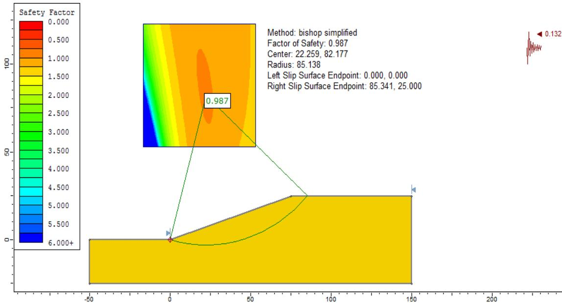
Figure 62.4: Circular slip surface, using the Bishop simplified method
