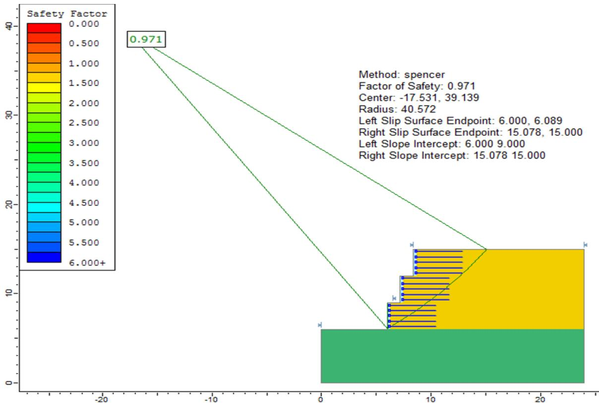
Figure 89.2: Solution, using the Spencer method
