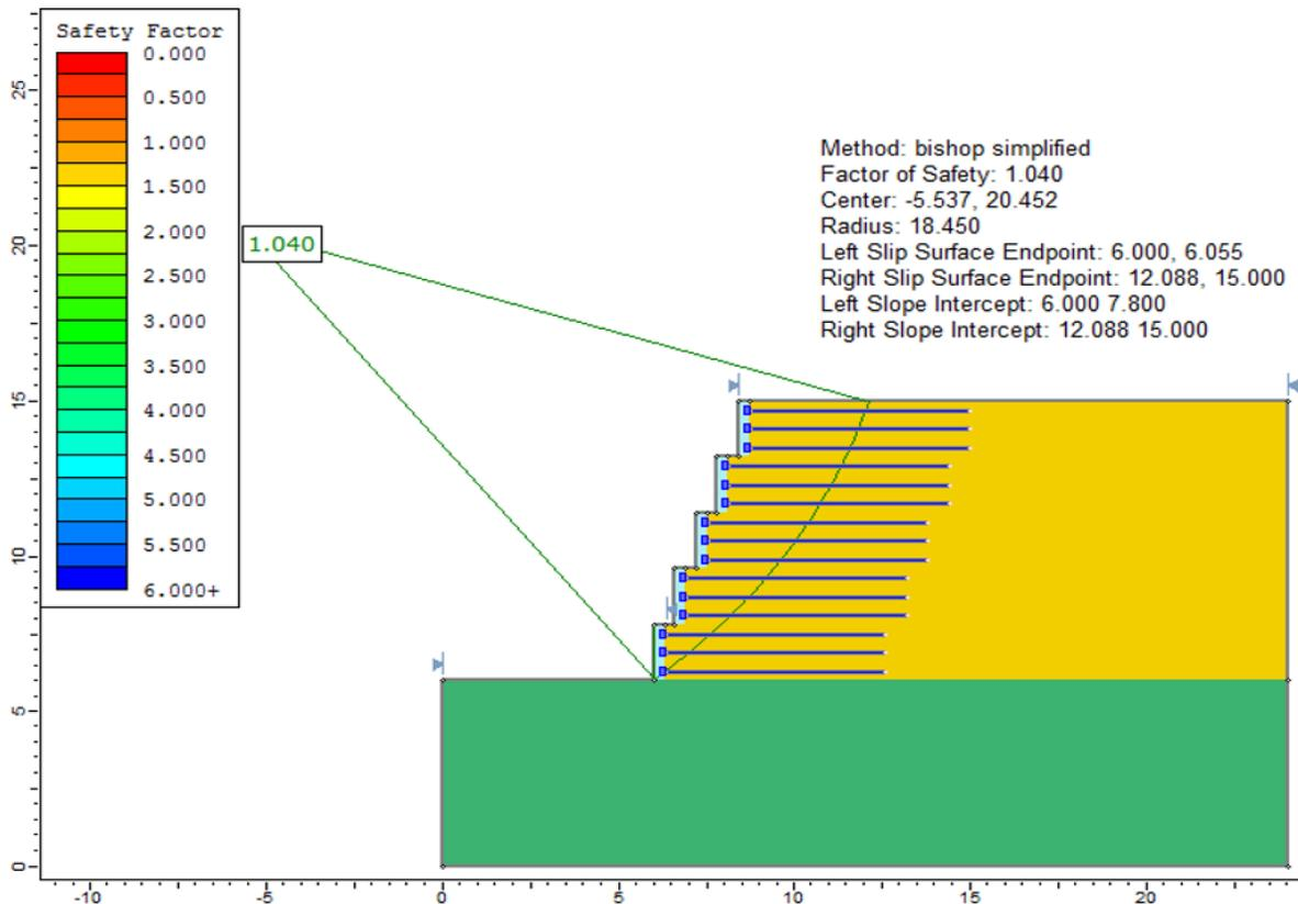
Figure 94.2: Solution, using the Bishop simplified method
