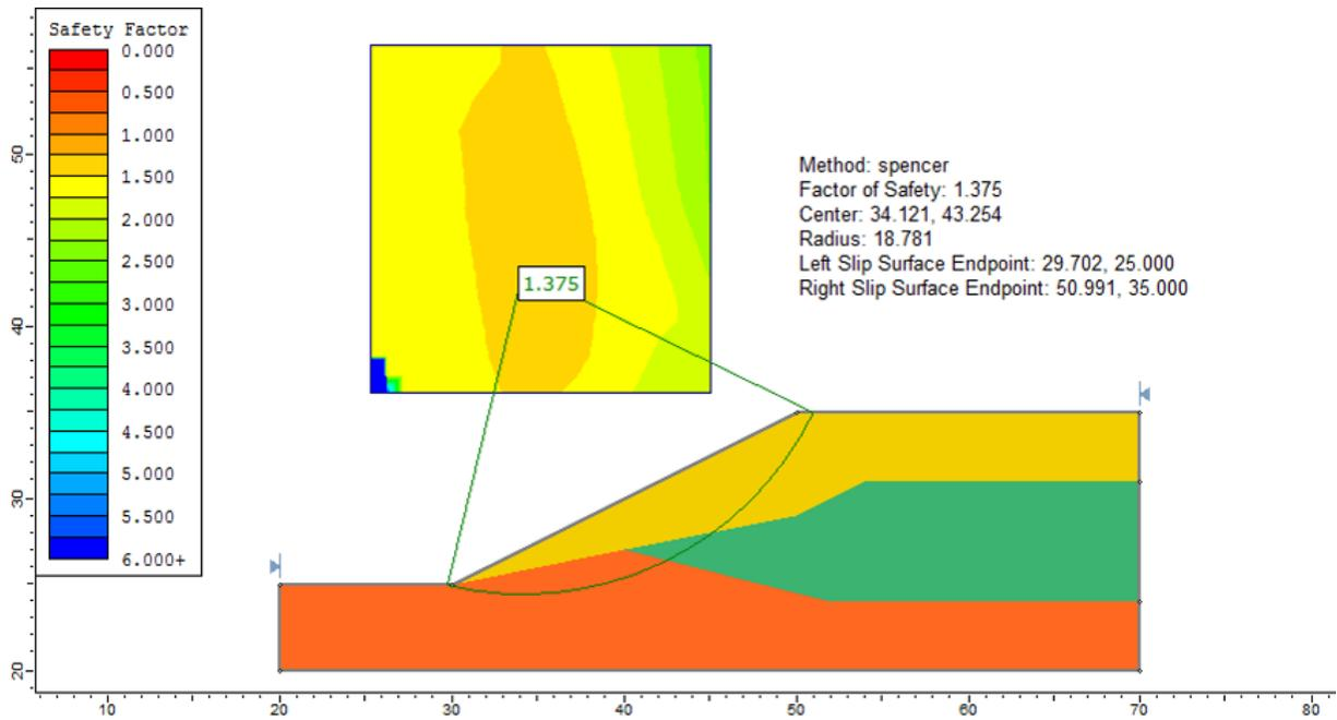
Figure 3.3: Solution, using the Spencer method
