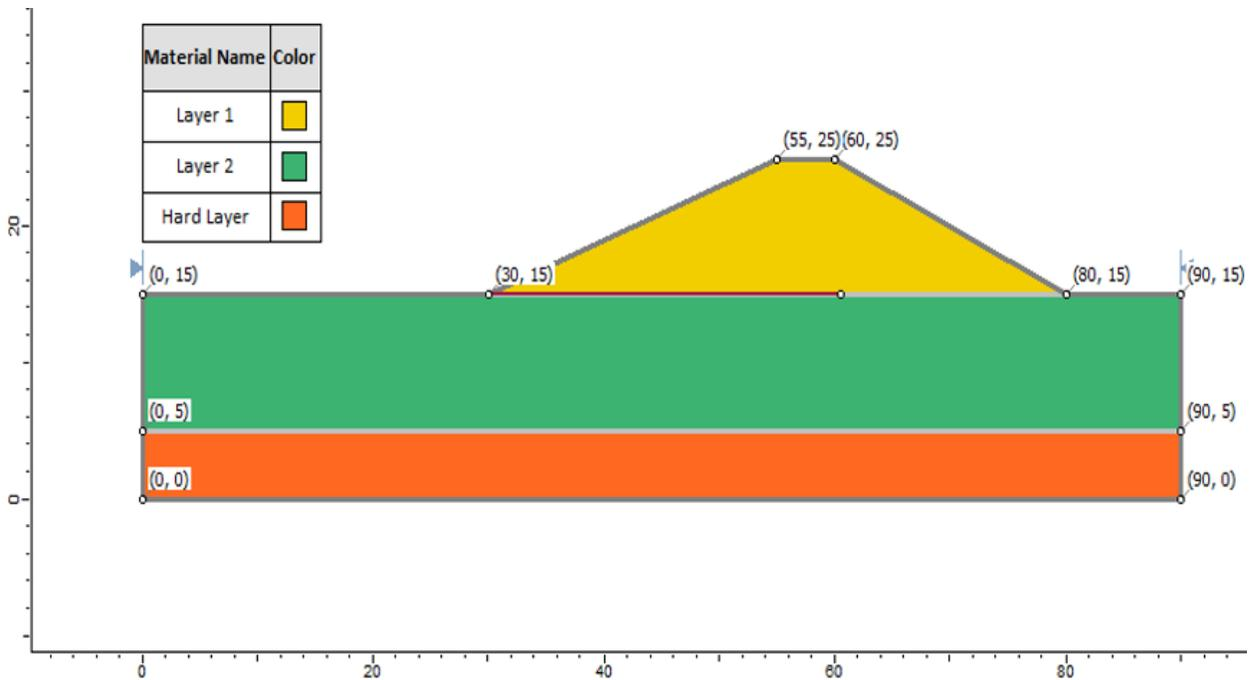
Figure 28.2: Geometry for Example 5 (an embankment on a soft clay foundation)
