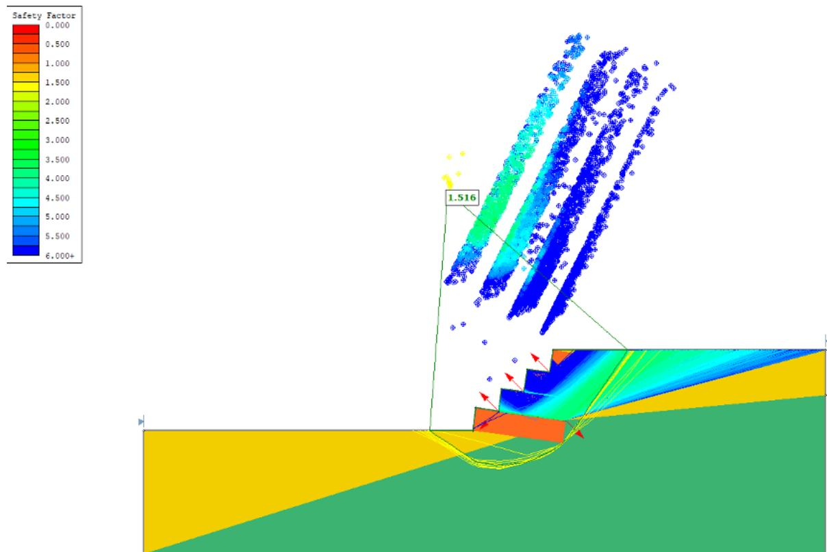
Figure 109.2: Solution, using Block Search and Bishop method
