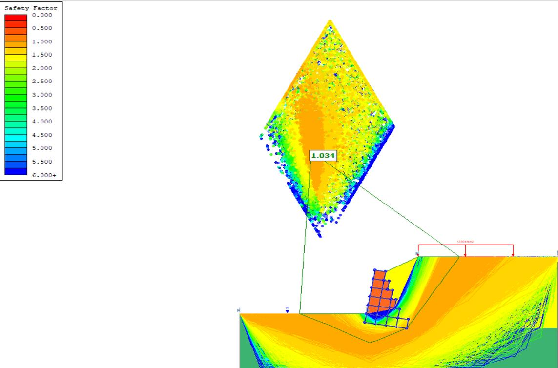
Figure 107.8: Solution for Mesh Method Using Cuckoo Search and Bishop Method
