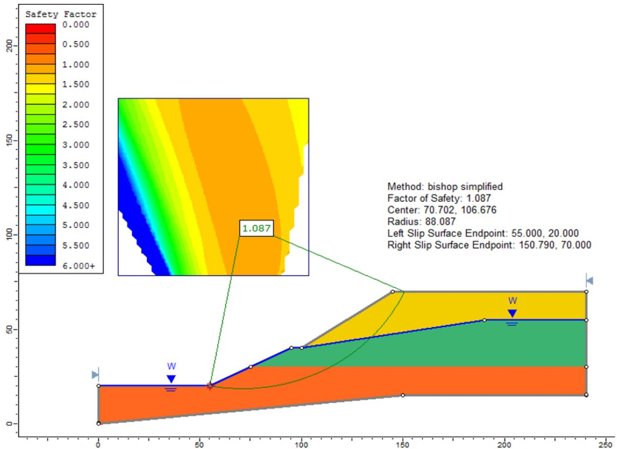
Figure 20.2: Circular failure surface, using the Bishop simplified method
