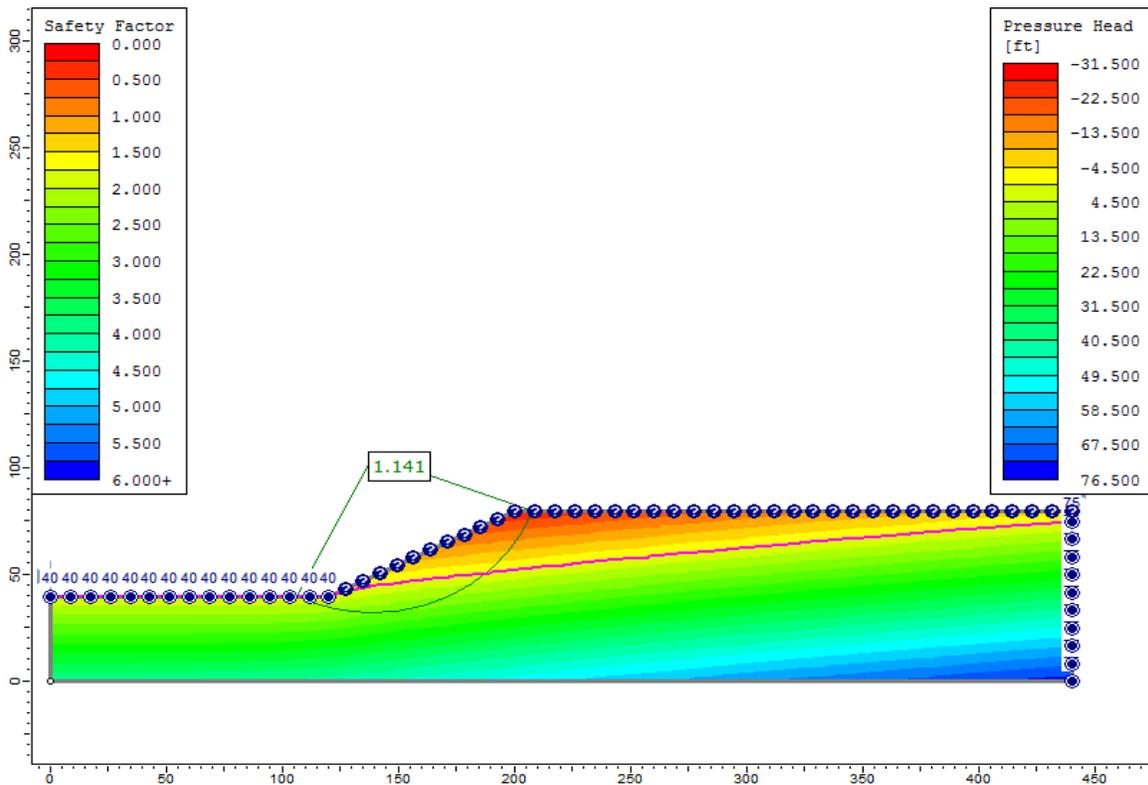
Figure 71.3: Solution to Case 1, using the Spencer method
