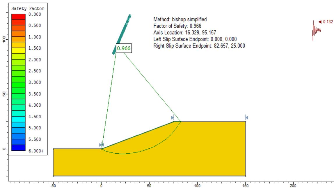
Figure 62.5: Non-circular slip surface, using the Bishop simplified method
