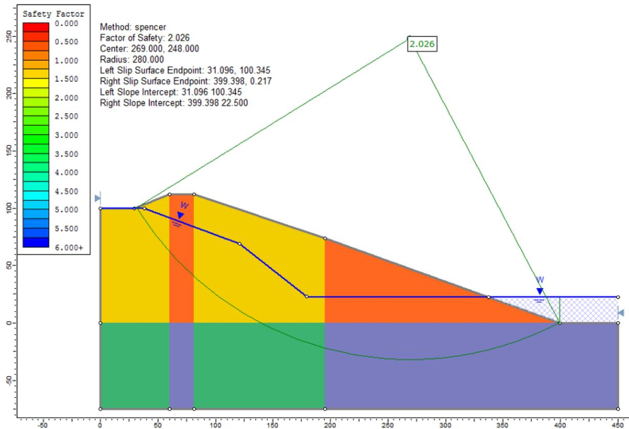
Figure 69.2: Solution, using the Spencer method
