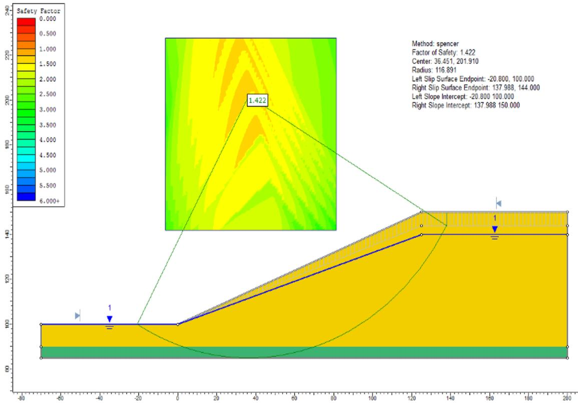
Figure 57.3: Circular failure surface, using Spencer method
