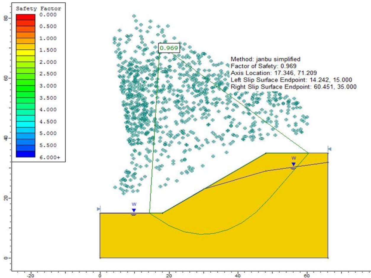
Figure 16.2: Circular failure surface using the Bishop simplified method
