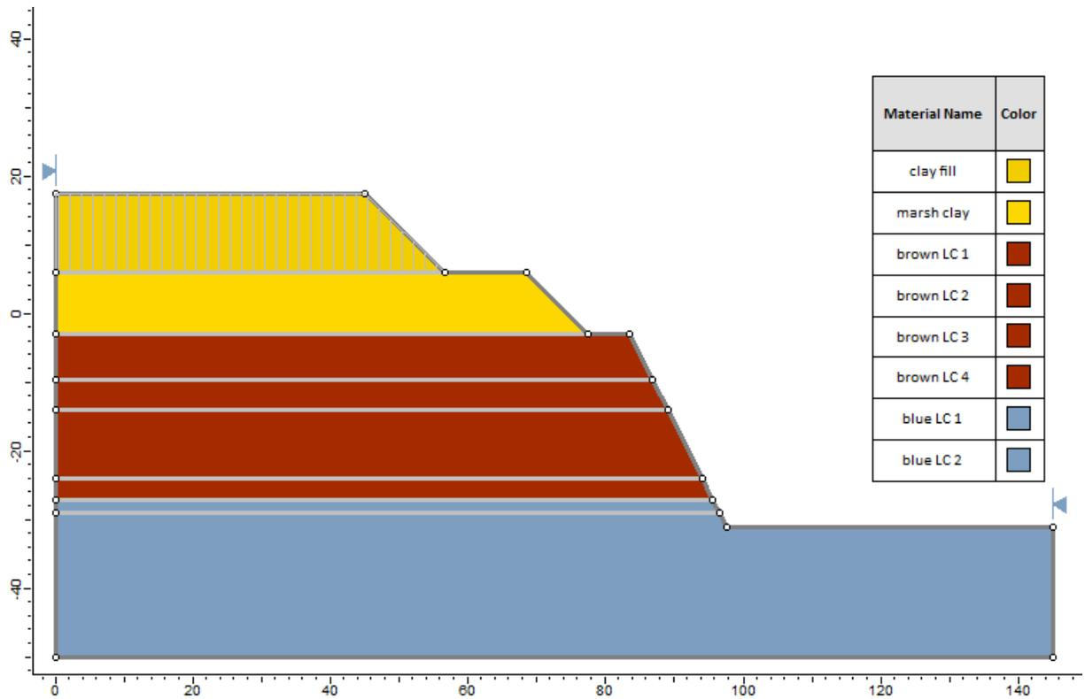
Figure 73.2: Excavated Slope Geometry in **Slide**
