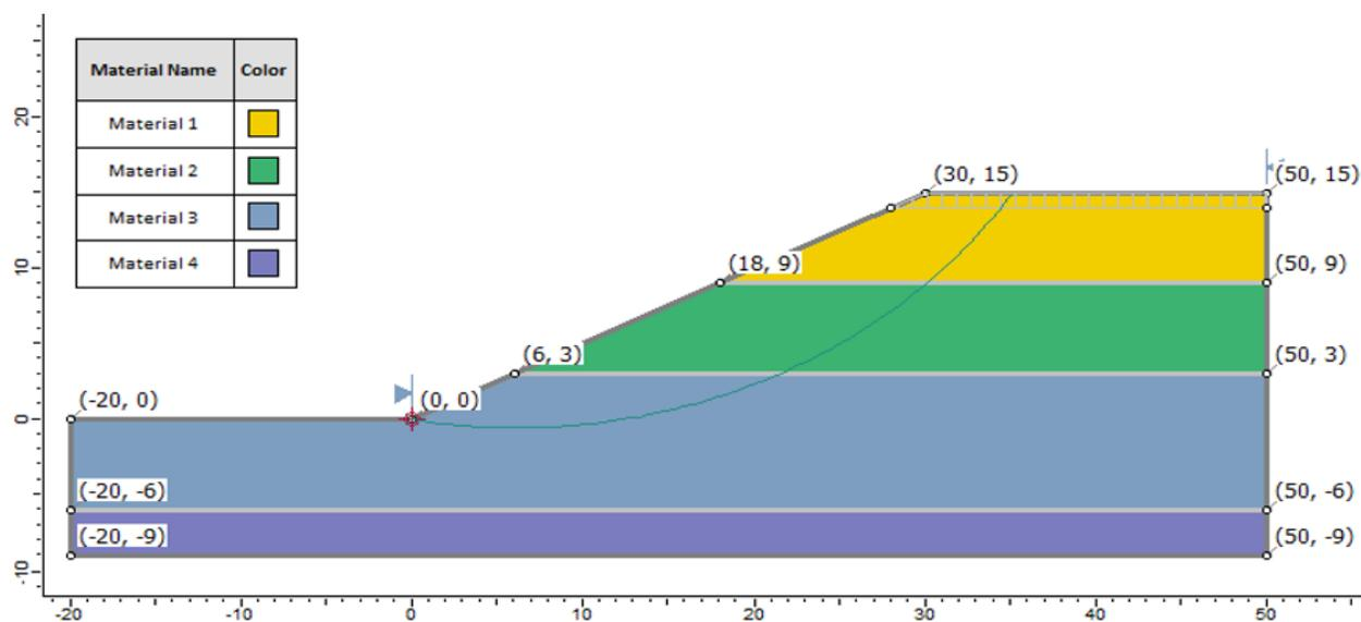
Figure 52.1: Geometry Setup in **Slide** (dry condition)
