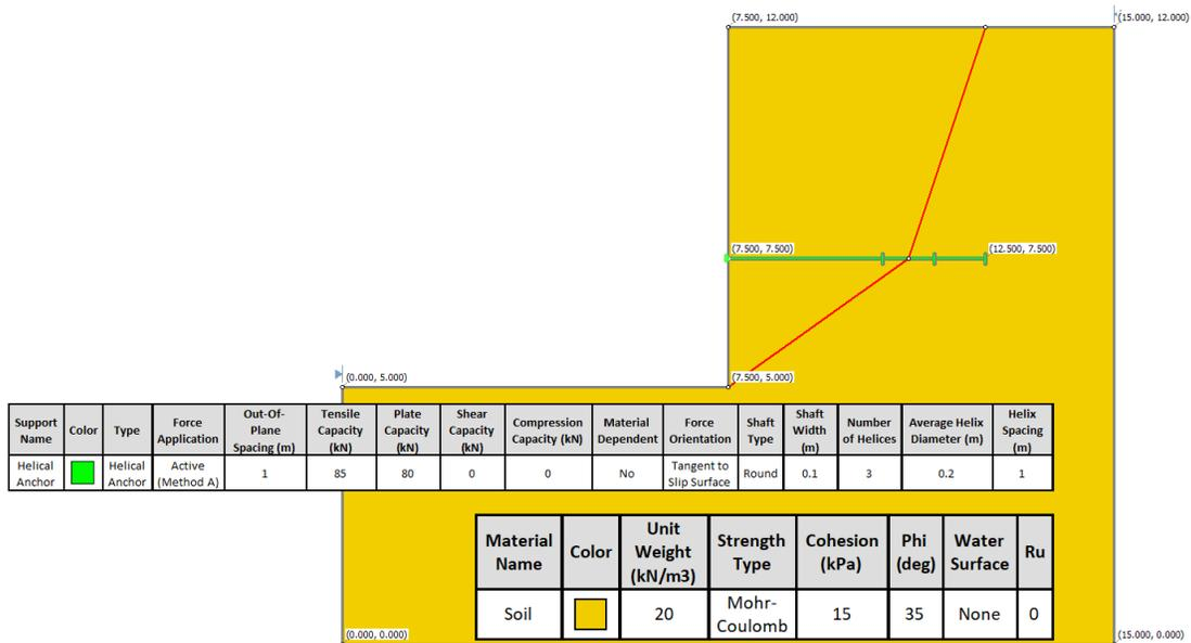
Figure 111.1: Model with single surface and helical anchor
