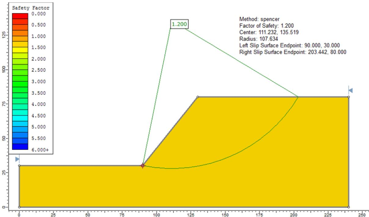
Figure 78.2: Solution to Case 1(a), using the Spencer method
