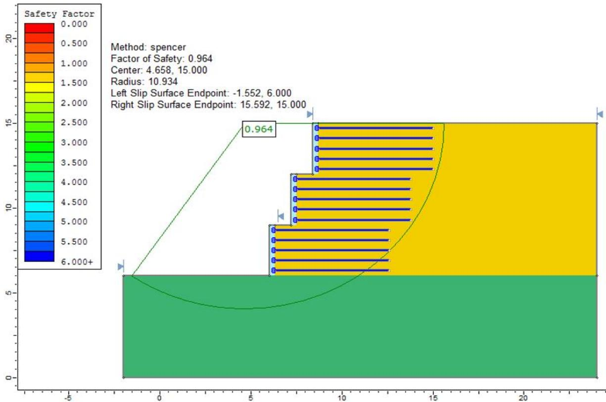
Figure 91.2: Solution, using the Spencer method
