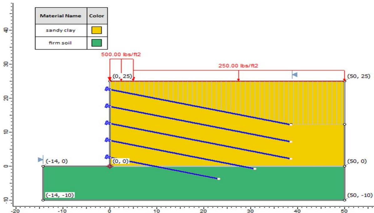
Figure 60.1: Geometry Setup in **Slide**
