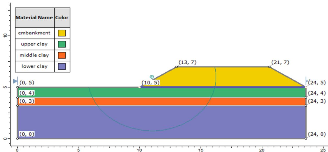
Figure 30.1: Geometry Setup in **Slide**
