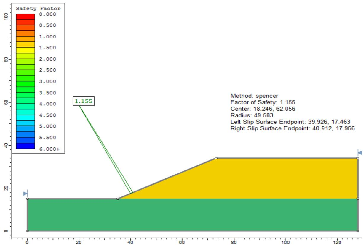
Figure 81.3: Solution for Case 2, using the Spencer method
