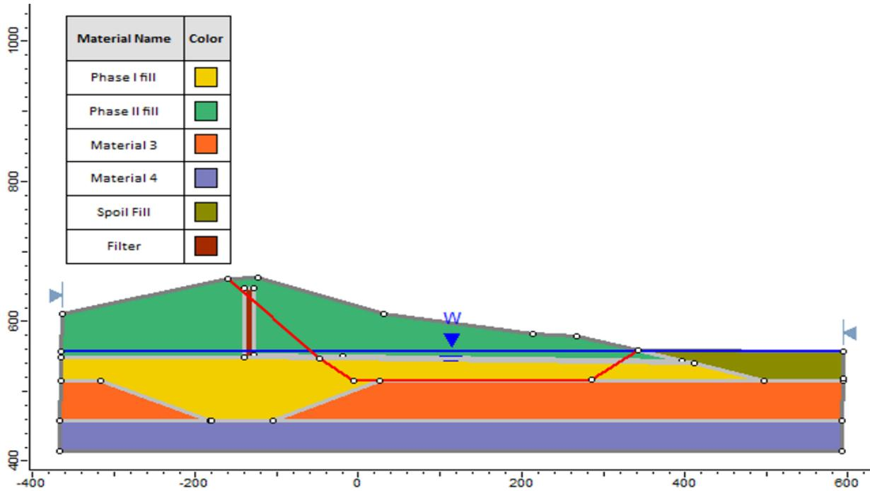
Figure 34.2: Geometry Setup in **Slide**
