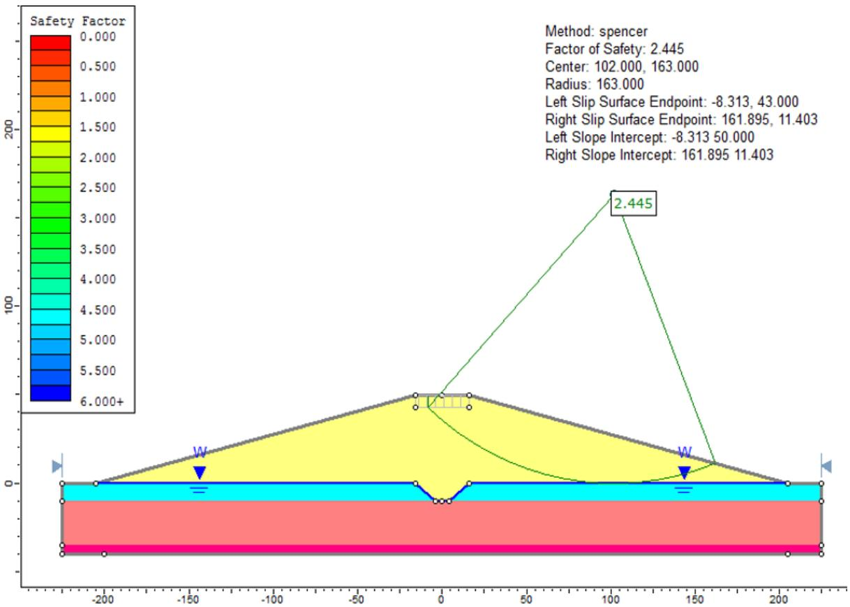
Figure 64.2: Solution, using the Spencer method
