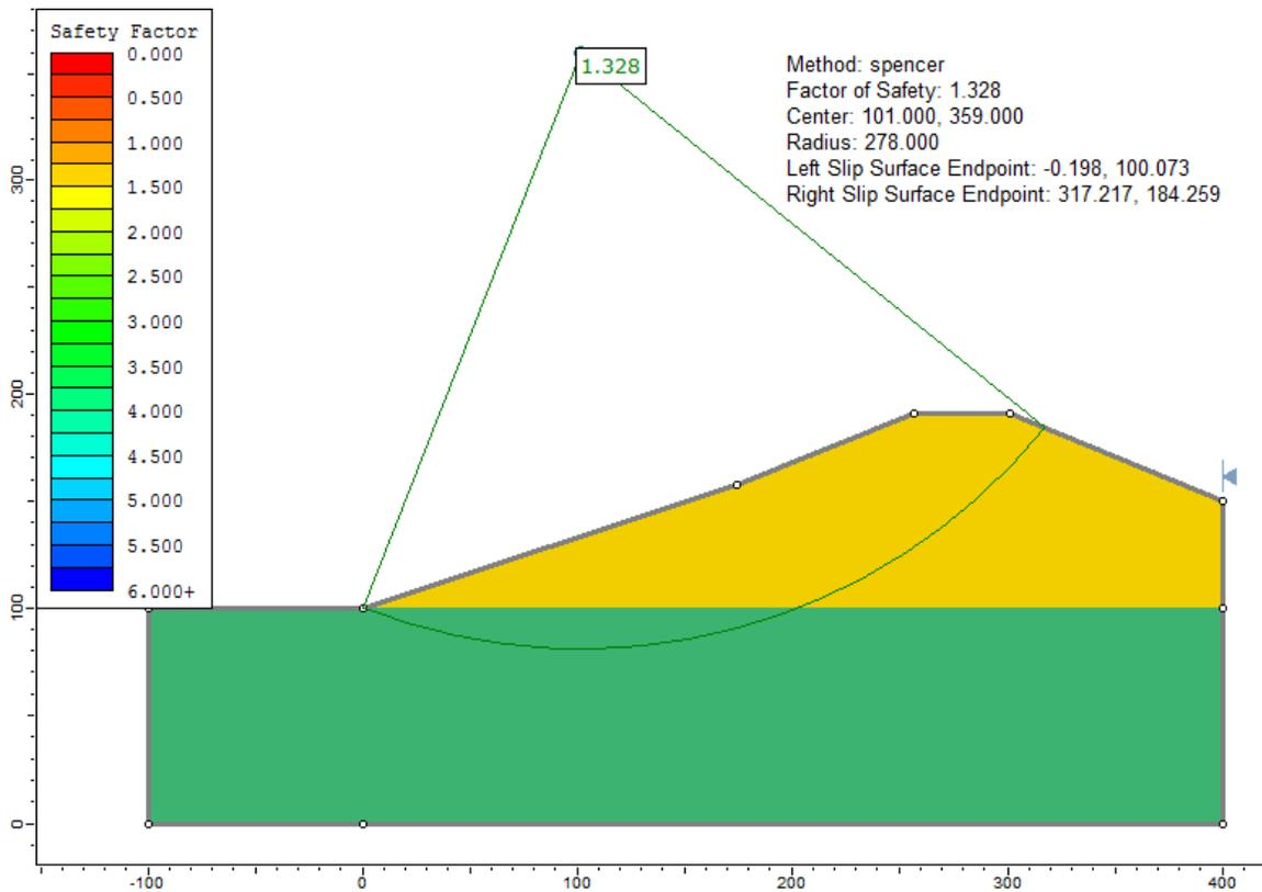
Figure 67.2: Solution, using the Spencer method
