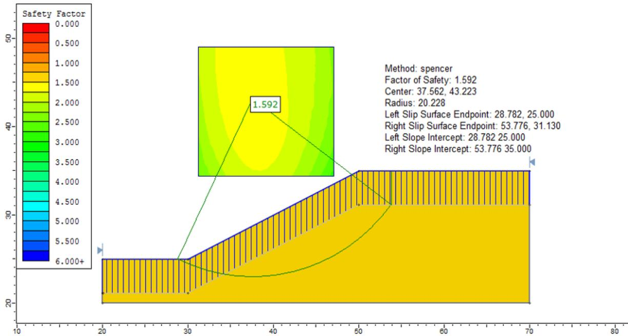
Figure 2.3: Solution, using the Spencer method
