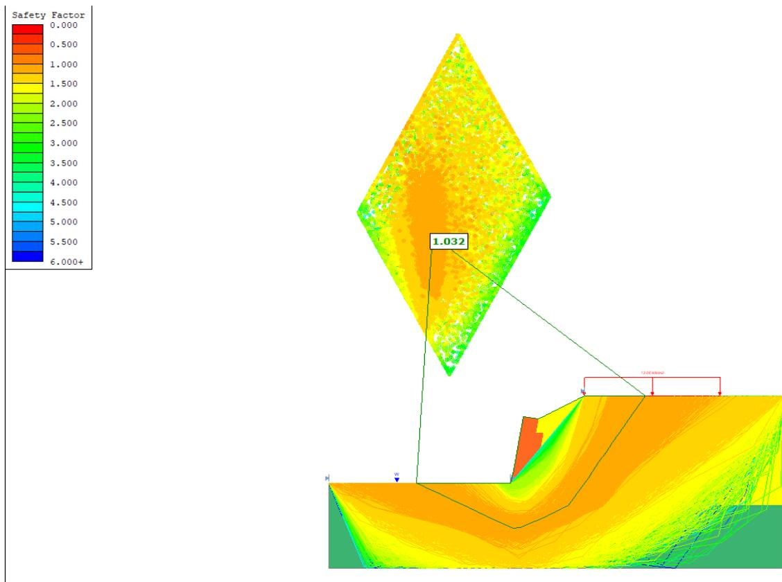
Figure 107.6: Solution for Equivalent Cohesion Method Using Cuckoo Search and Bishop Method
