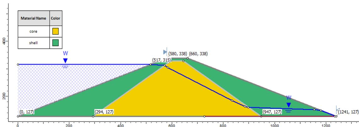
Figure 77.2: Piezometric Line Approximation
