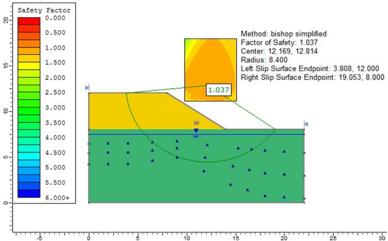
Figure 11.2: Solution, using the Bishop simplified method
