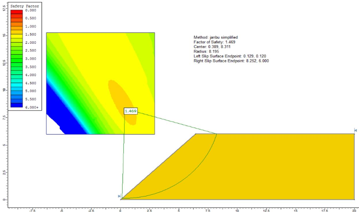
Figure 44.3: Critical failure surface, using the Mohr-Coulomb criterion, Janbu simplified
