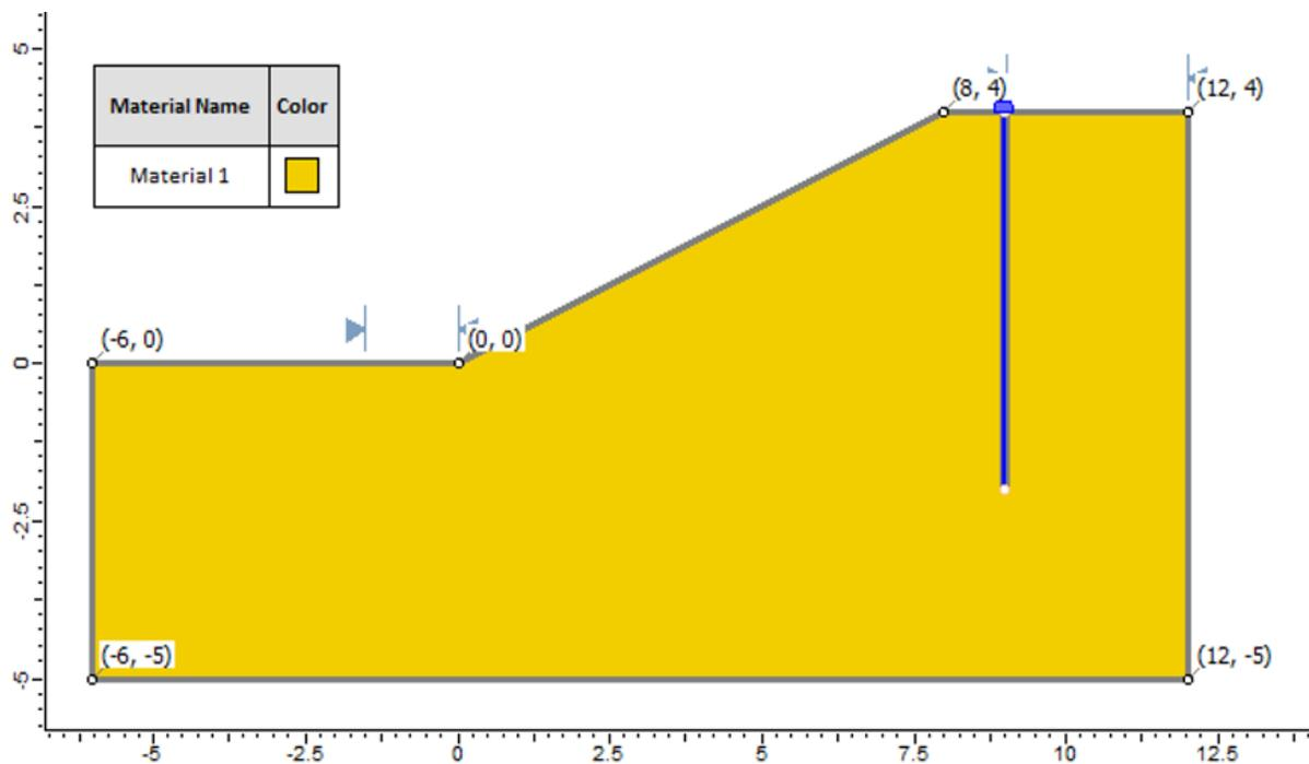
Figure 54.1: Geometry Setup in **Slide**
