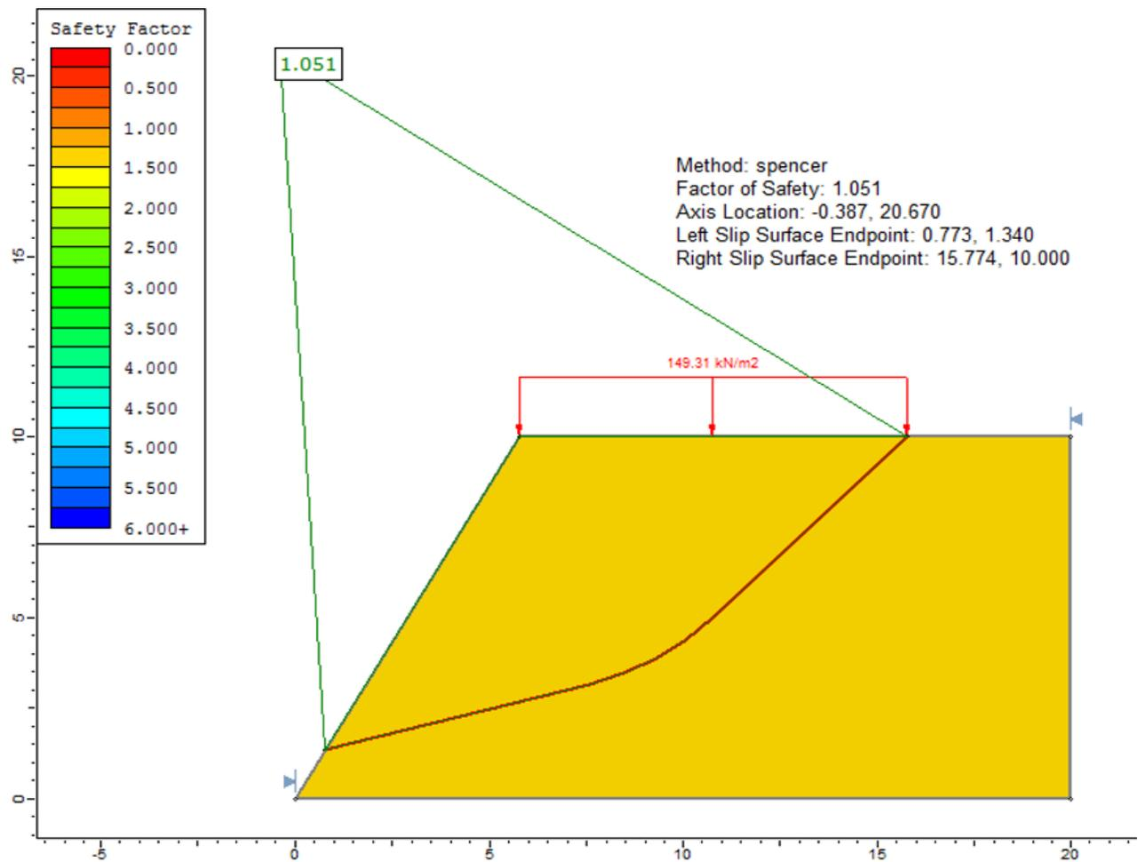
Figure 25.3: Non-Circular failure surface, by using the Spencer method
