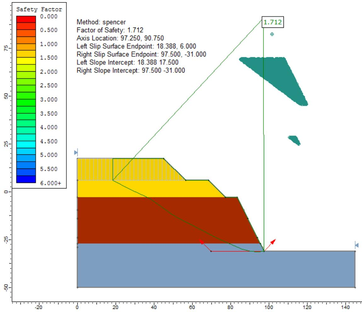
Figure 73.4: Solution, using the Spencer method (Non-circular)
