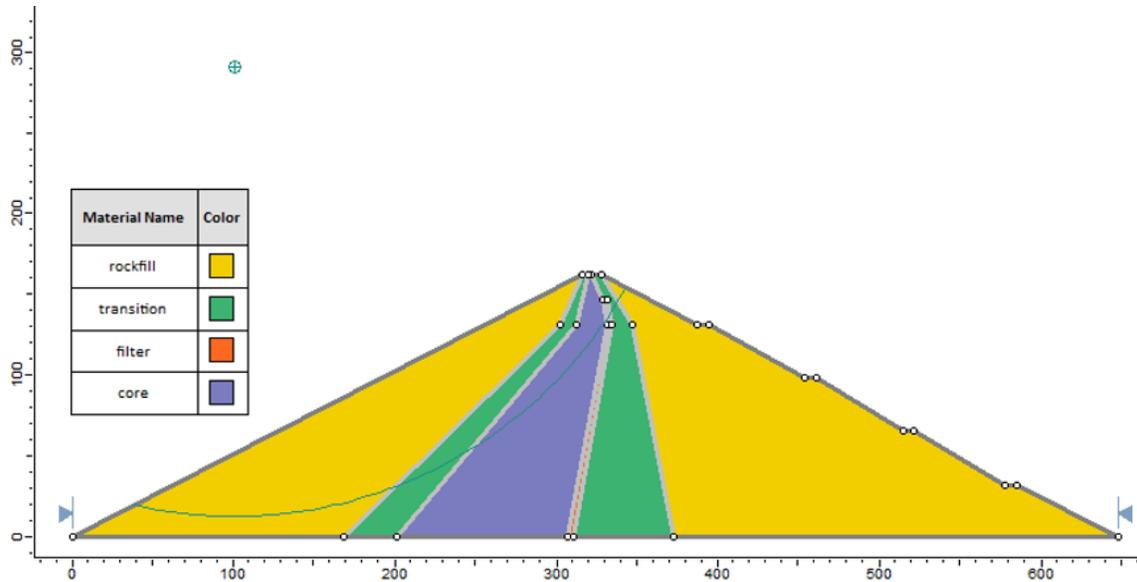
Figure 6.2: Geometry Setup in **Slide**
