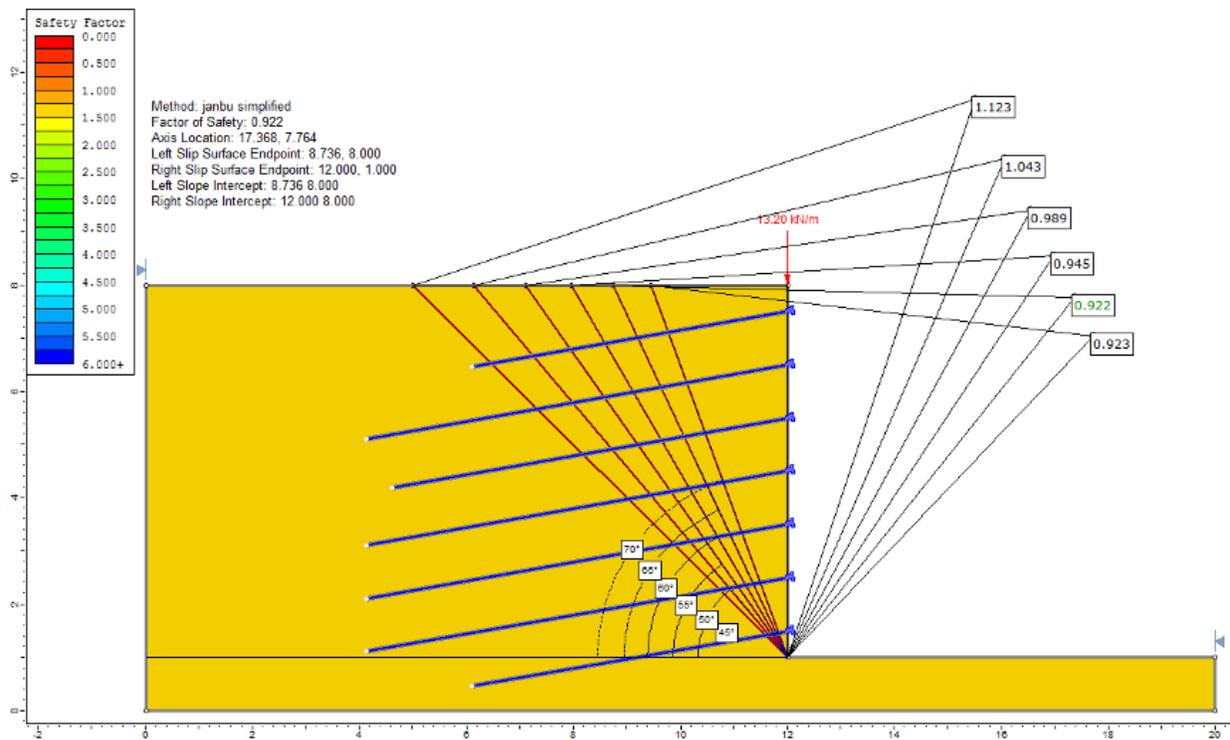
Figure 48.2: Failure planes and corresponding safety factors
