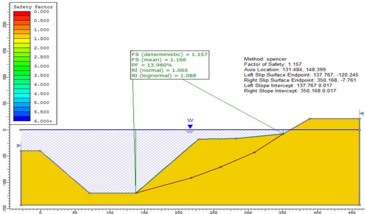
Figure 29.2: Noncircular failure surface, using the Spencer method
