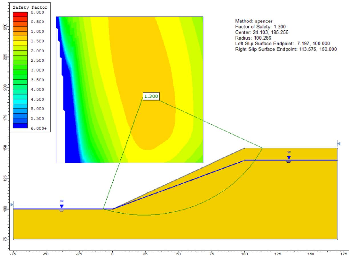
Figure 55.2: Circular failure surface, using Spencer method
