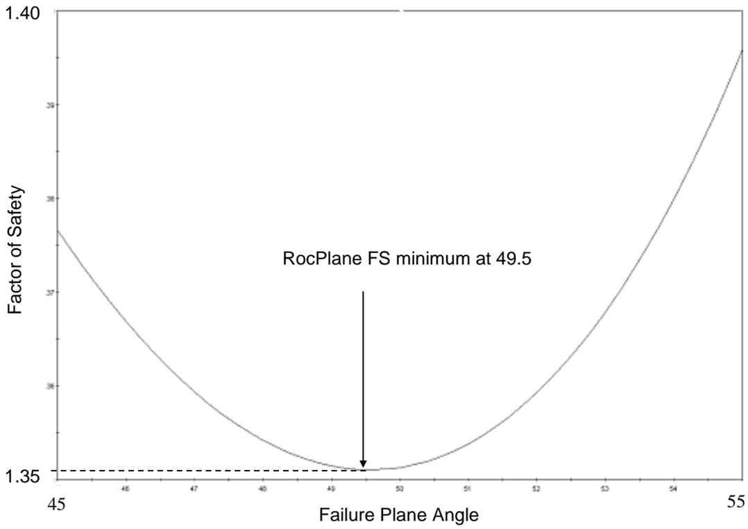
Figure 43.5– Solution using RocPlane 2.0
