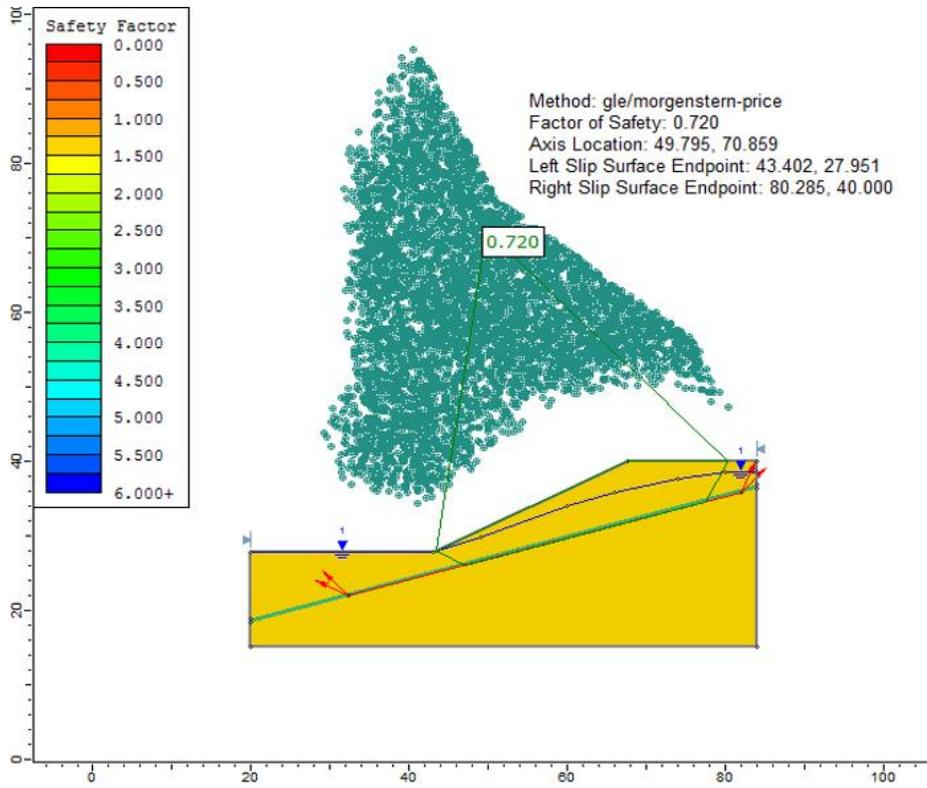
Figure 9.3: Solution, using the GLE method
