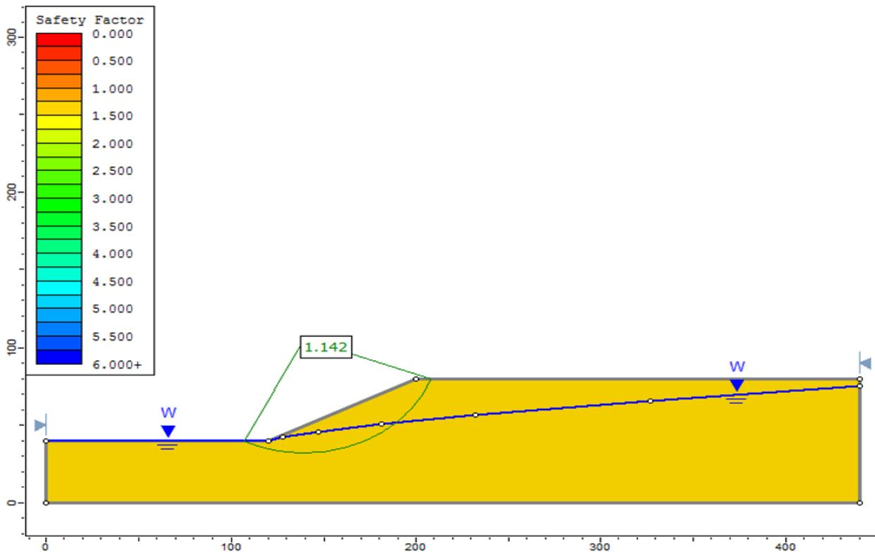
Figure 71.4: Solution to Case 2, using the Spencer method
