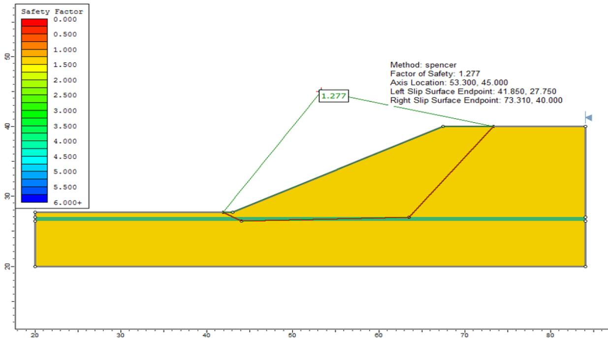
Figure 8.2: Solution, using the Spencer method
