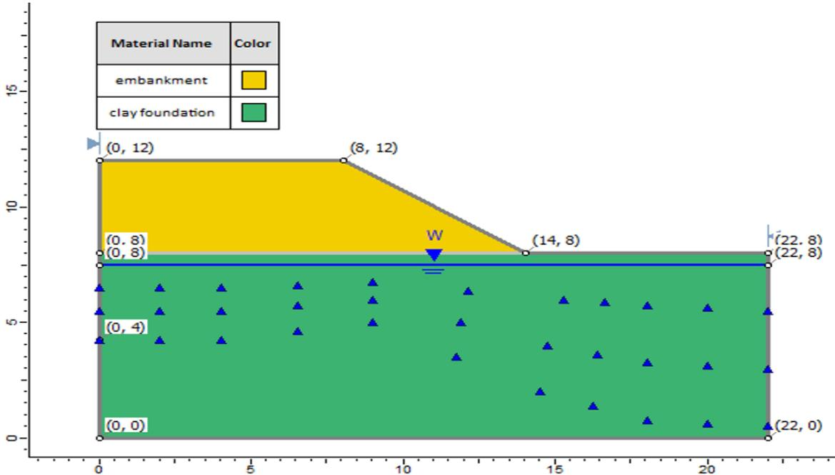
Figure 11.1: Geometry Setup in Slide
