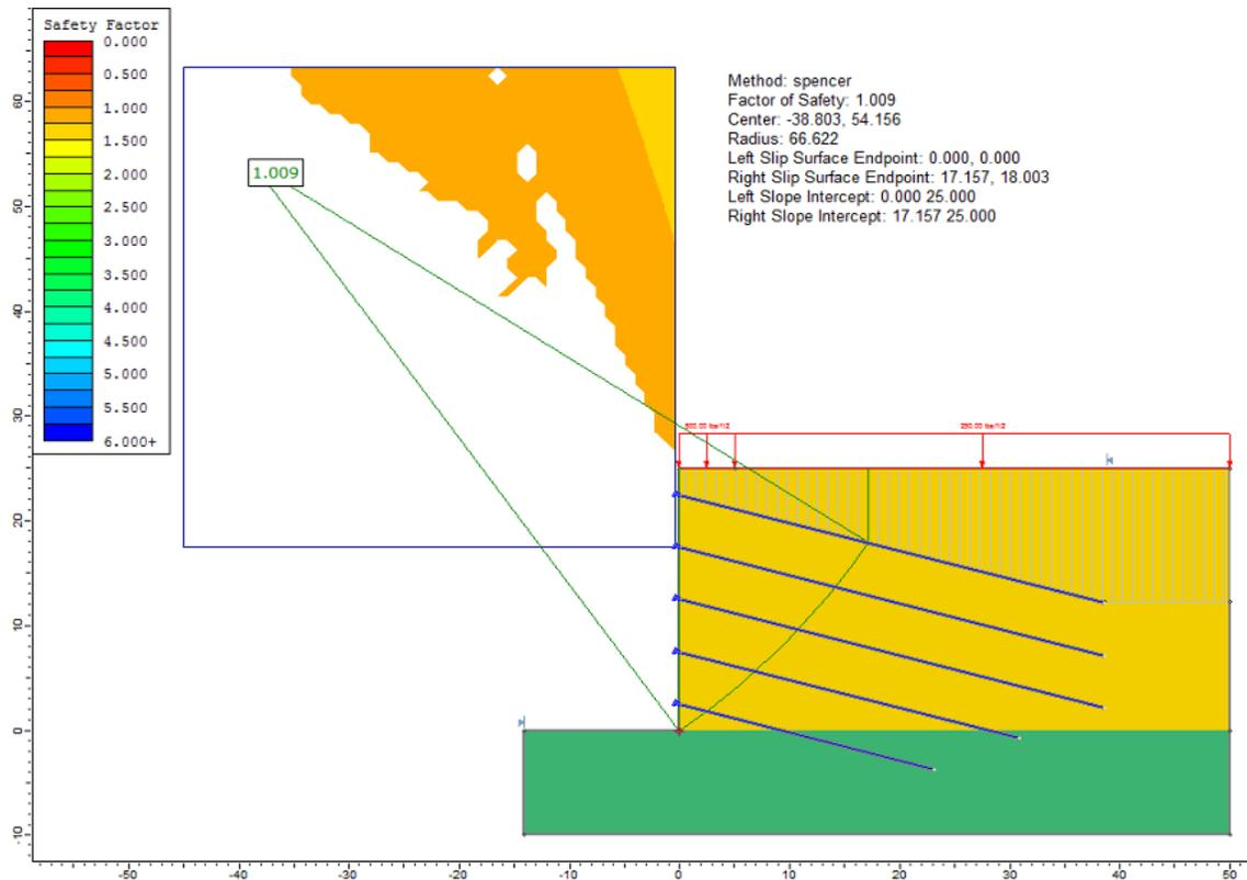
Figure 60.2: Critical failure surface, using Spencer method
