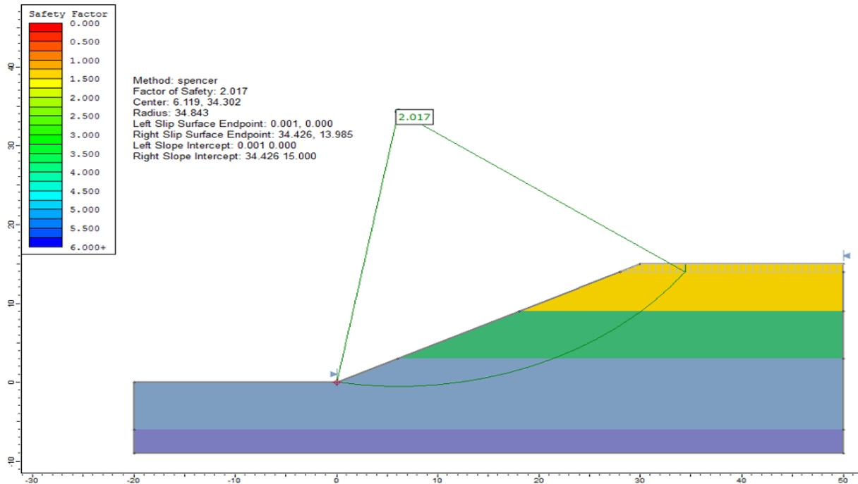
Figure 52.2: Solution, using the Bishop simplified method
