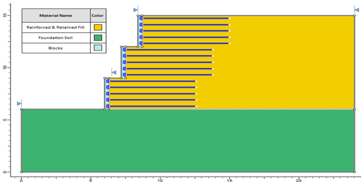
Figure 88.1: A Three-tiered Wall in Slide
