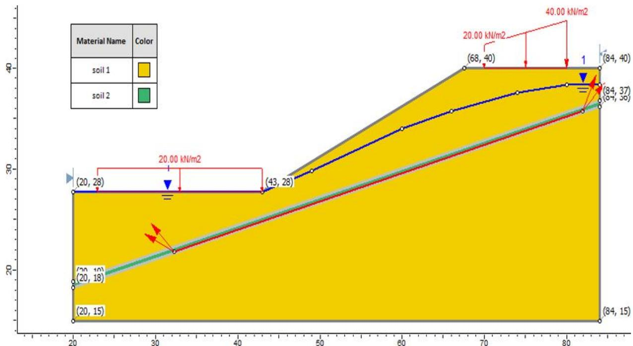
Figure 9.1: Geometry Setup in **Slide**
