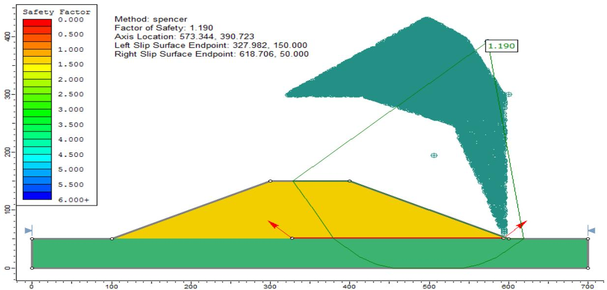
Figure 74.3: Solution, using the Spencer method (Non-circular)
