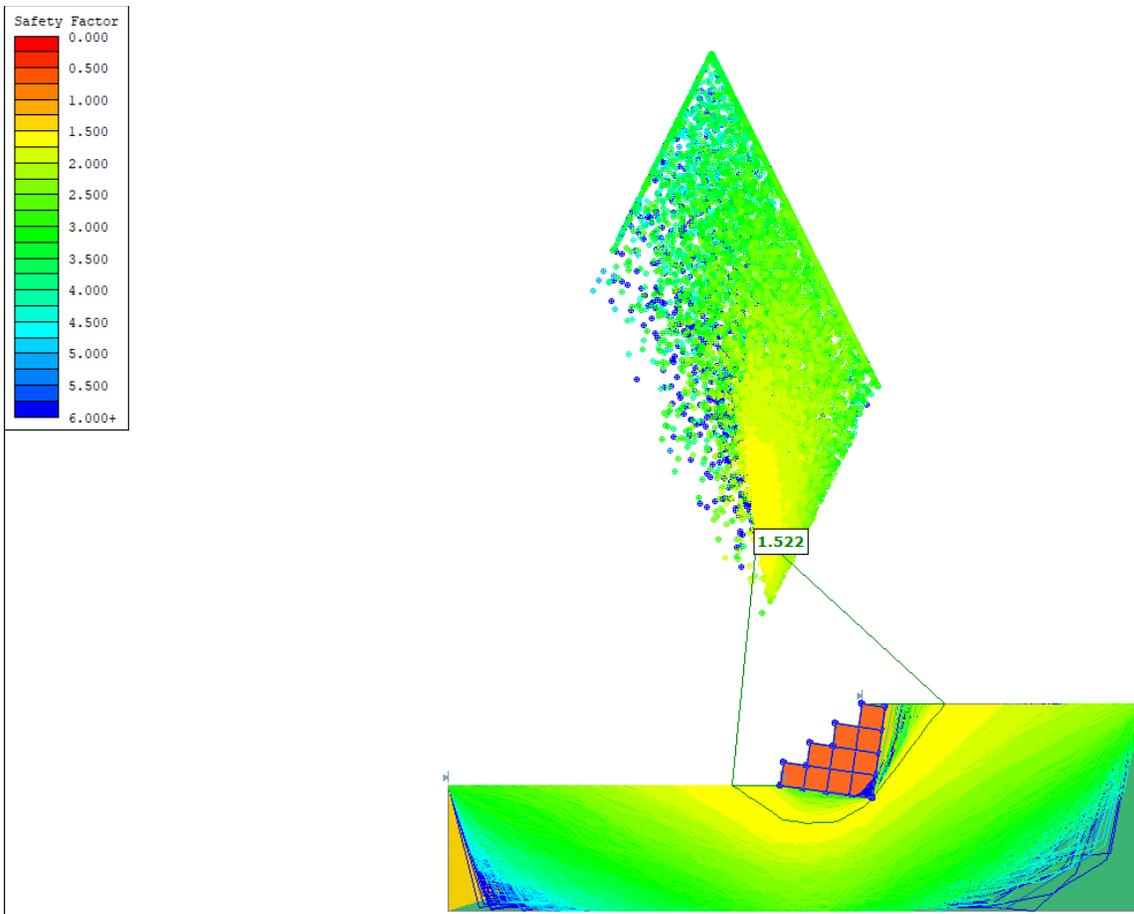
Figure 108.6: Solution for Mesh Method Using Cuckoo Search and Bishop Method
