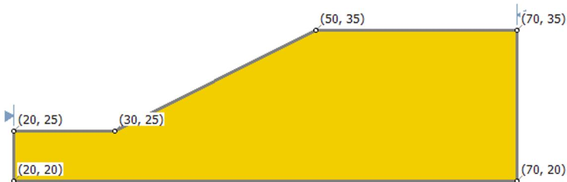
Figure 1.1: Geometry Setup in **Slide**
