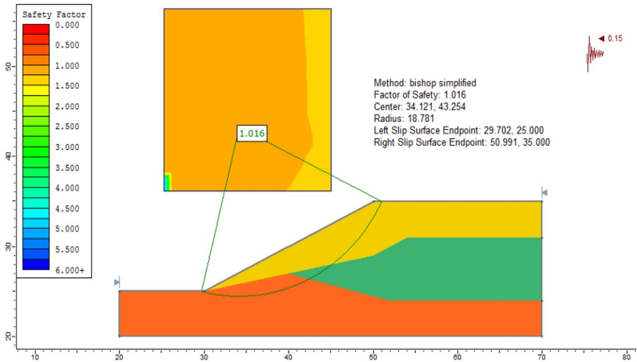
Figure 4.2: Solution, using the Bishop simplified method
