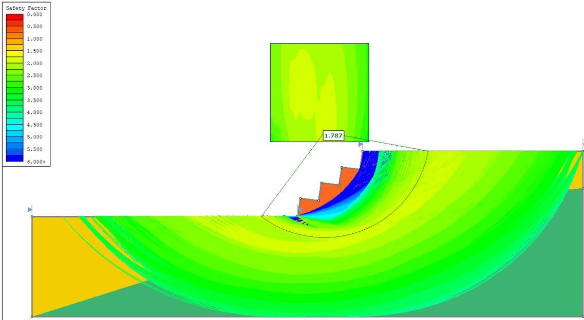
Figure 108.3: Solution for Equivalent Cohesion Method Using Circular Search and Bishop Method
