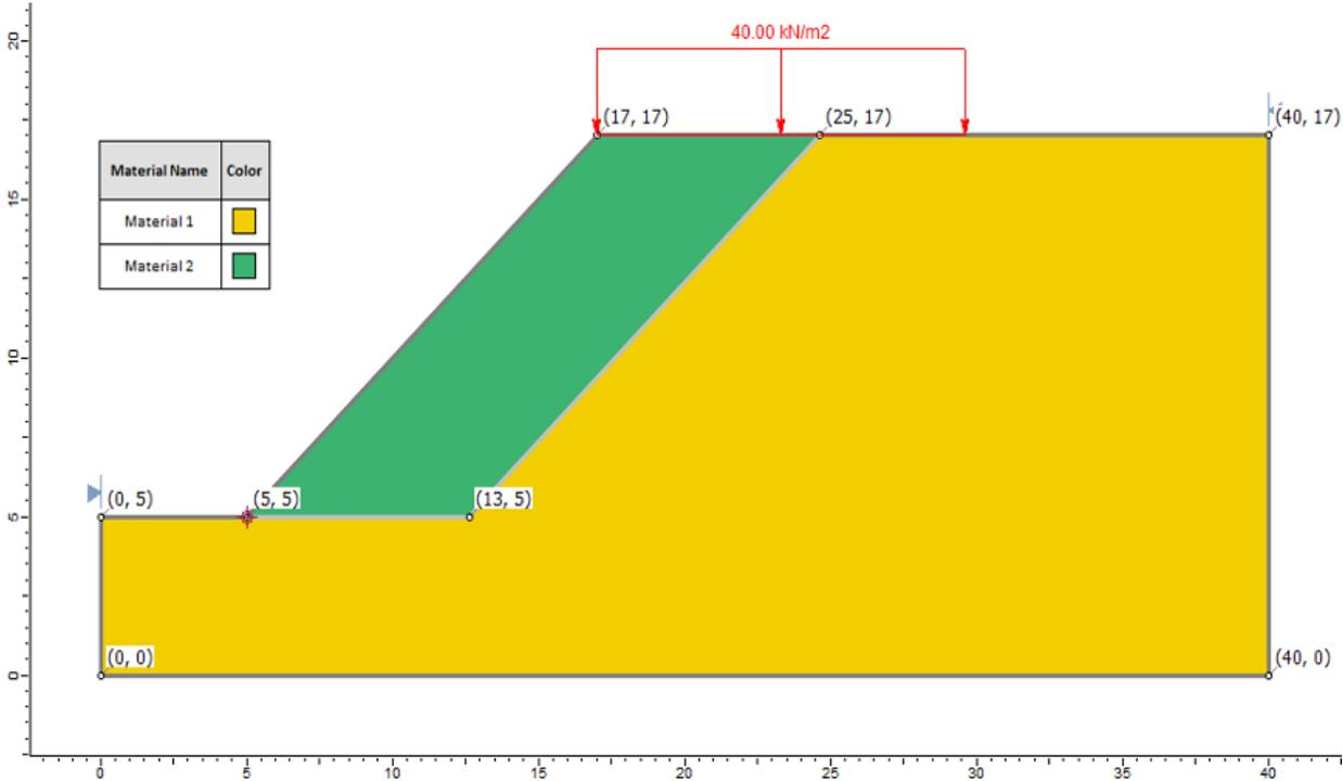
Figure 37.2: Geometry Setup in **Slide** (with reinforced zone)
