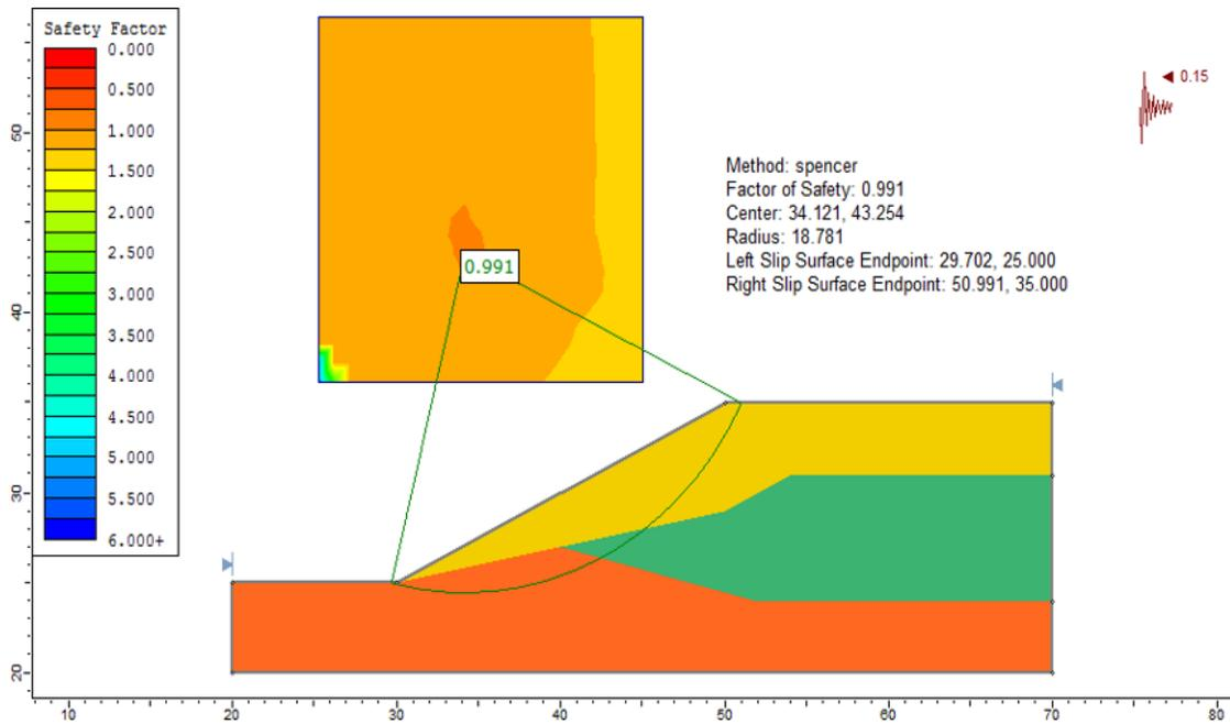
Figure 4.3: Solution, using the Spencer method
