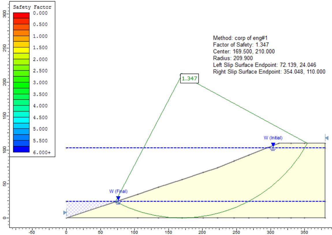
Figure 95.2: Solution, using the Army Corp. Eng. 2-stage rapid drawdown method
