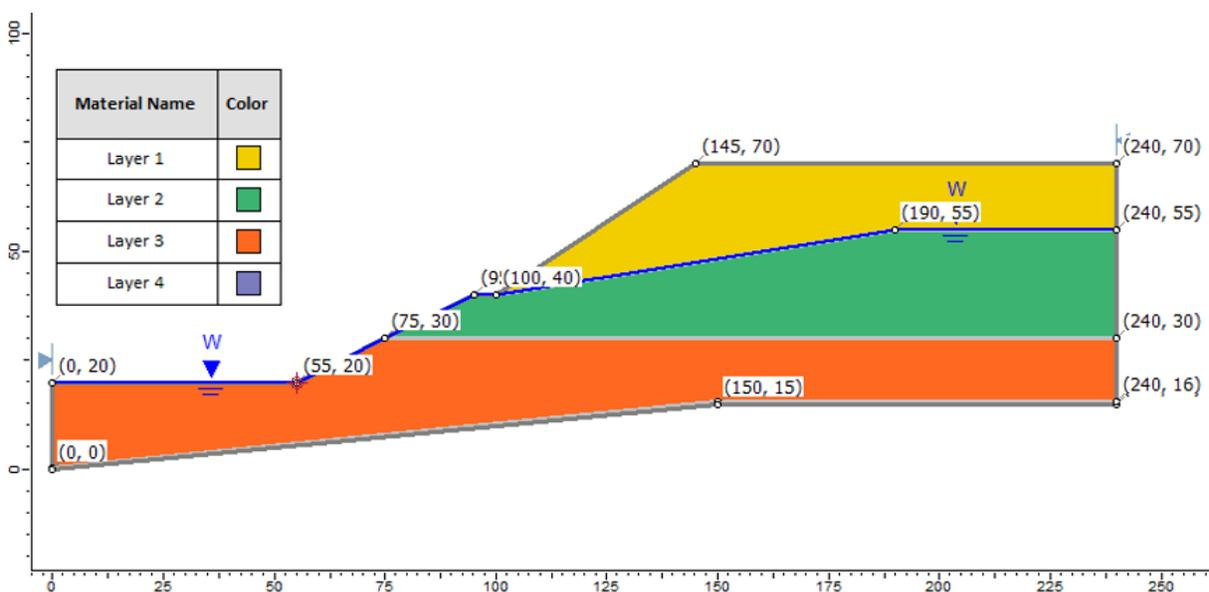
Figure 20.1: Geometry Setup in **Slide**
