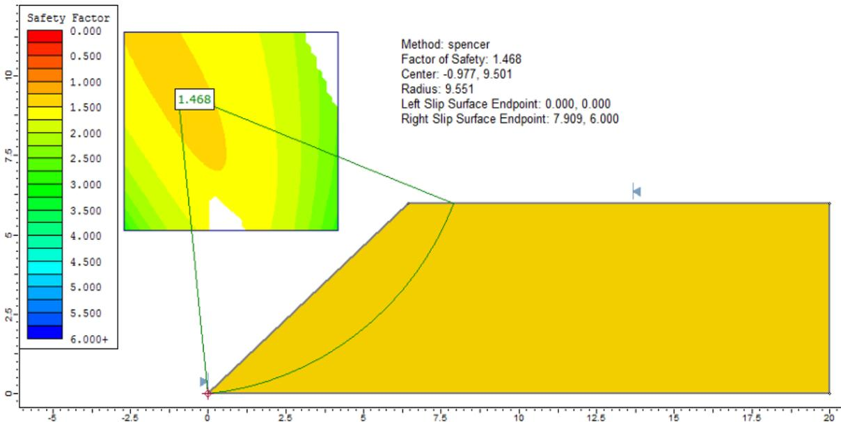
Figure 61.2: Circular critical surface with power curve criteria, Spencer method
