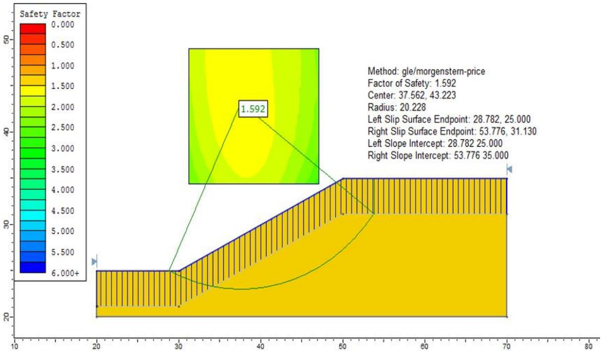
Figure 2.4: Solution, using the GLE method
