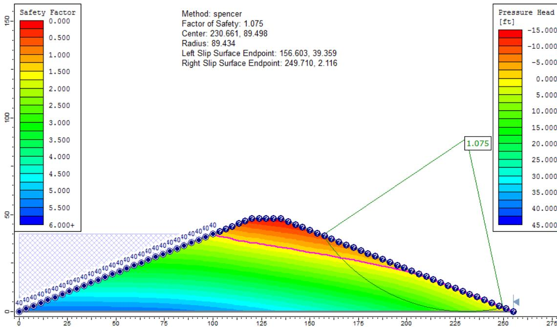
Figure 76.3: Solution to Case 1, using the Spencer method (Circular)
