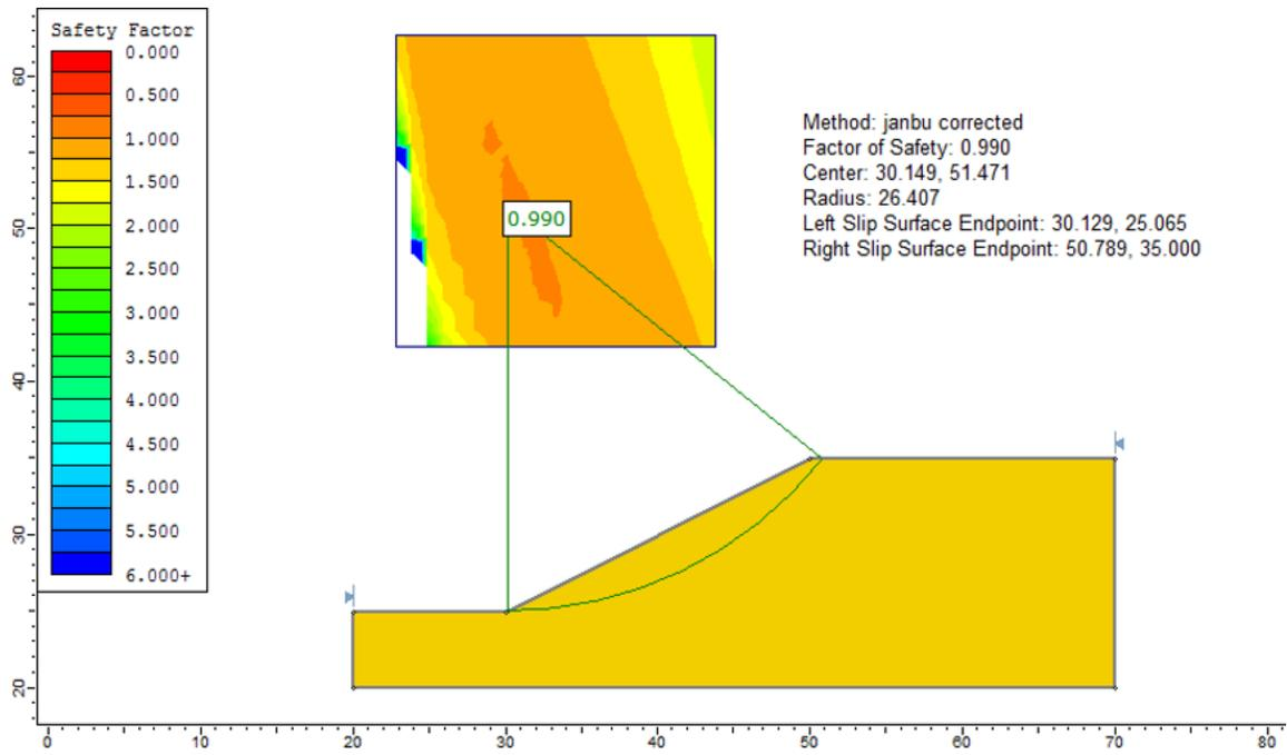
Figure 1.5: Solution, using the Janbu corrected method
