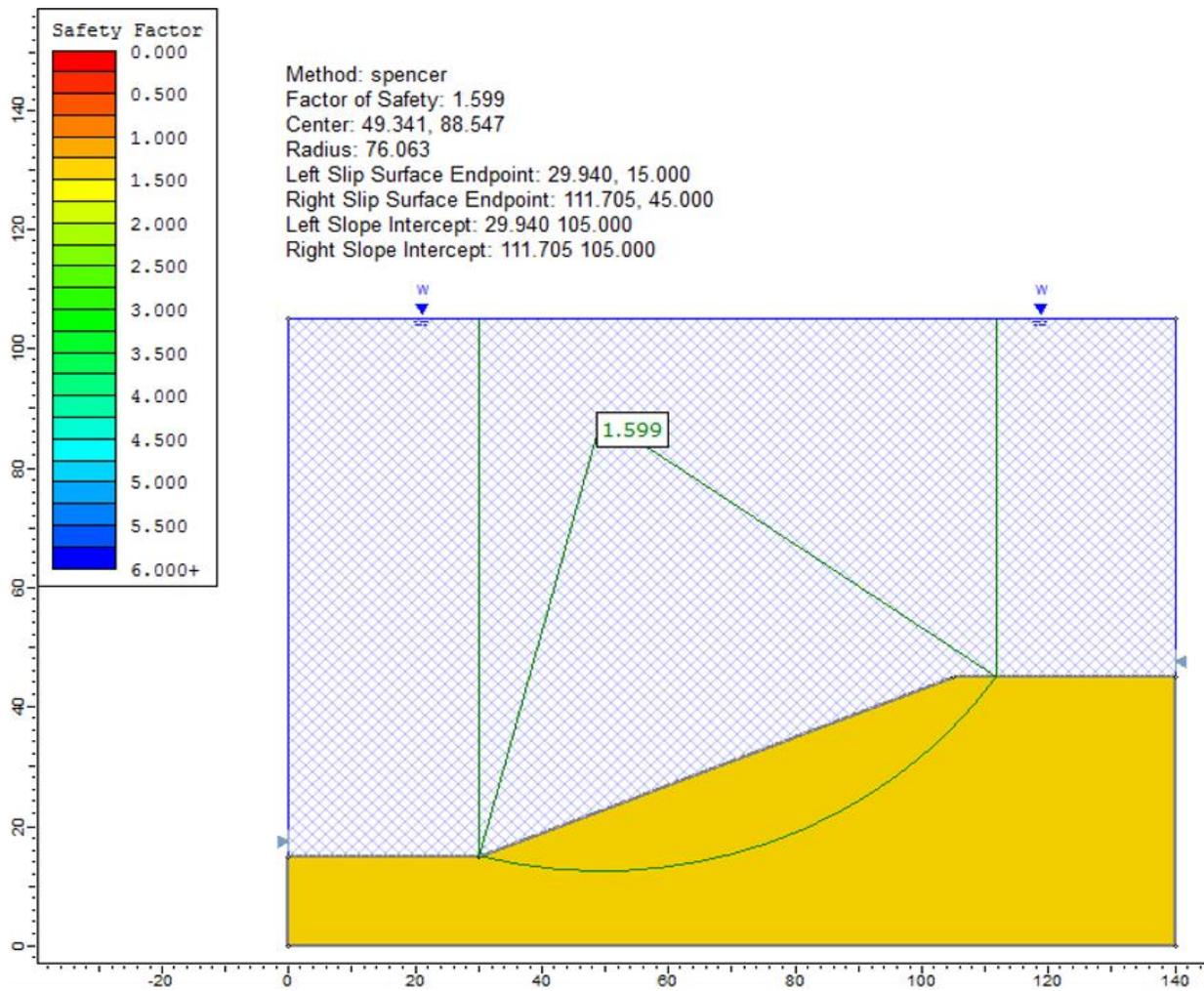
Figure 70.4: Solution to case 2 (circular), using the Spencer method
