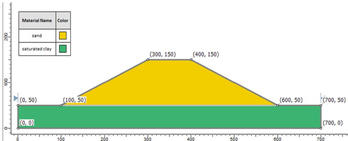
Figure 74.1: Sand Embankment on Saturated Clay Foundation
