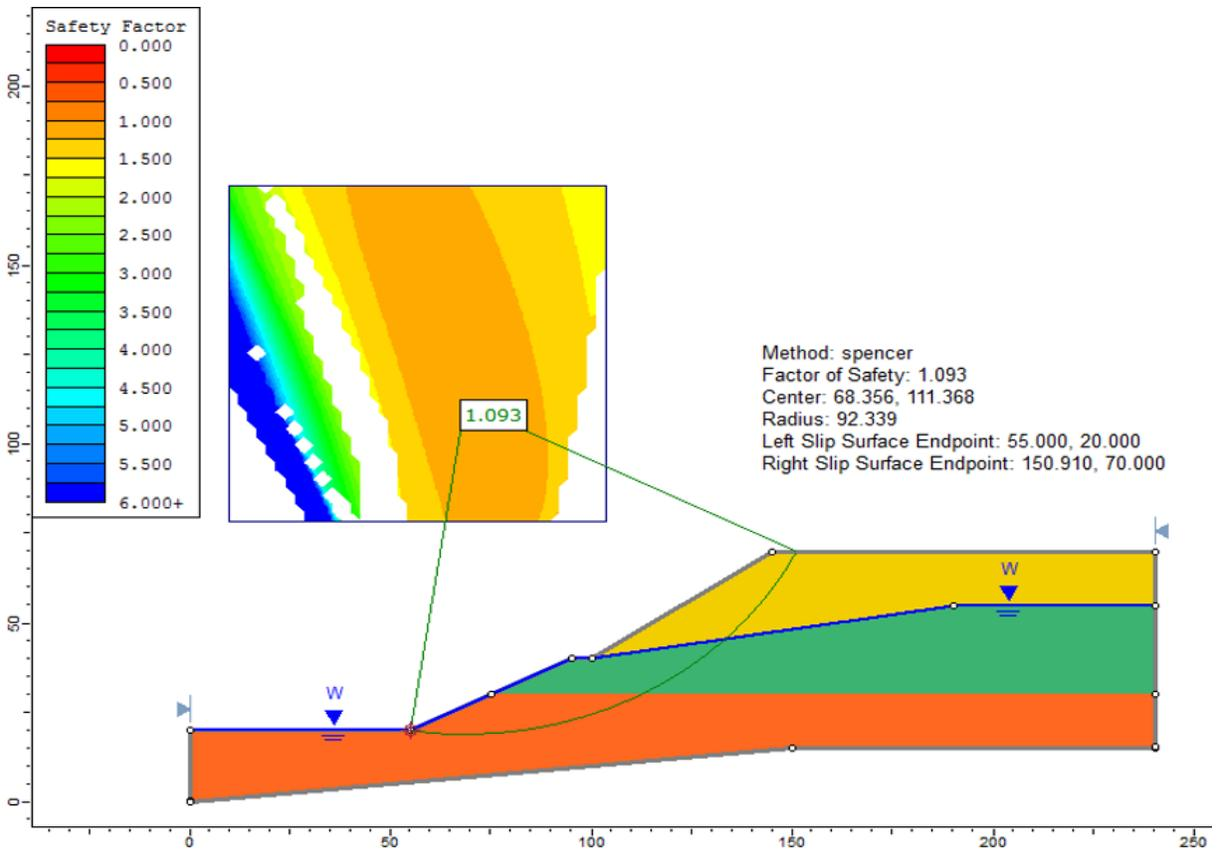
Figure 20.3: Circular failure surface using the Spencer method
