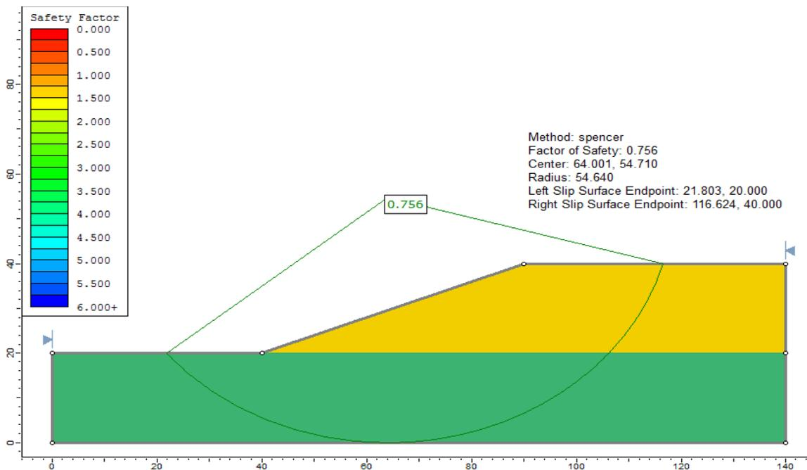
Figure 84.2: Solution to Case 1, using the Spencer method
