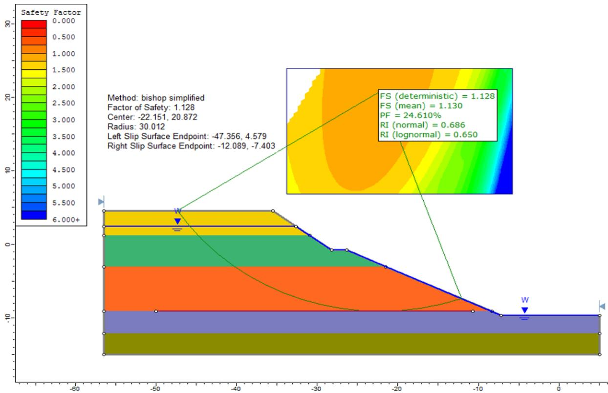
Figure 28.3: Critical slip circle tangential to lower boundary of clay layer 2
