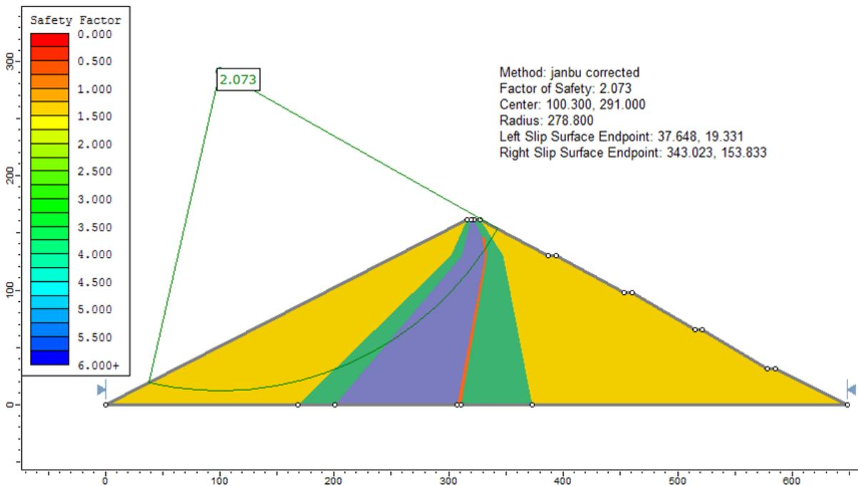
Figure 6.6: Solution, using the Janbu corrected method
