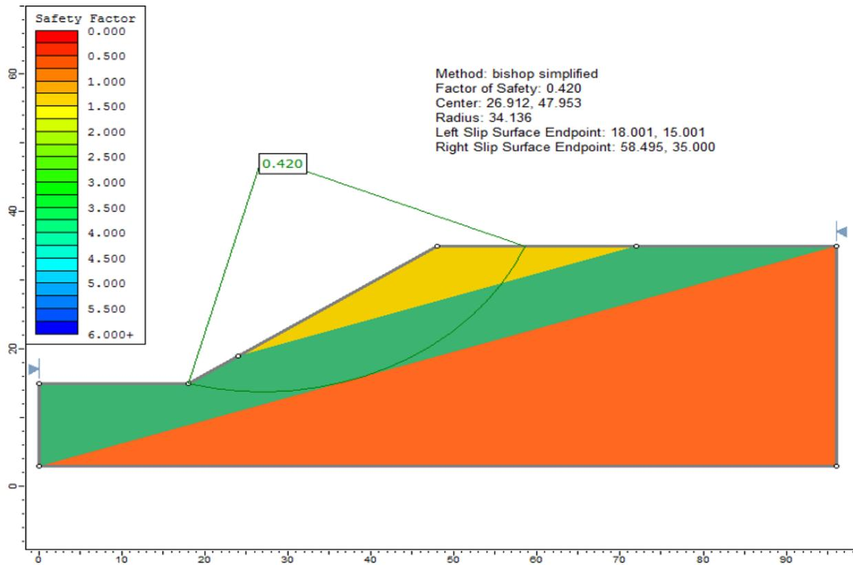
Figure 15.2: Circular failure surface, using the Bishop simplified method
