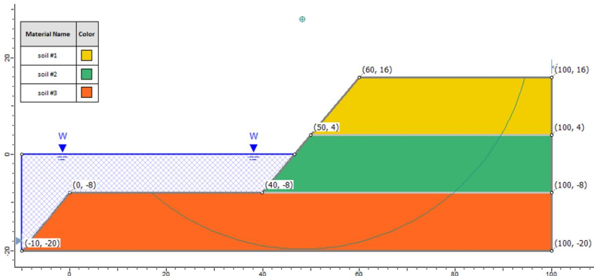
Figure 68.1: Geometry Setup in **Slide**
