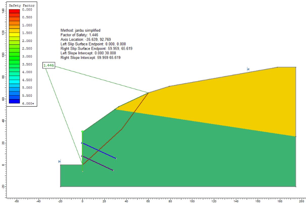
Figure 49.2: Critical failure surface, using the Janbu simplified method
