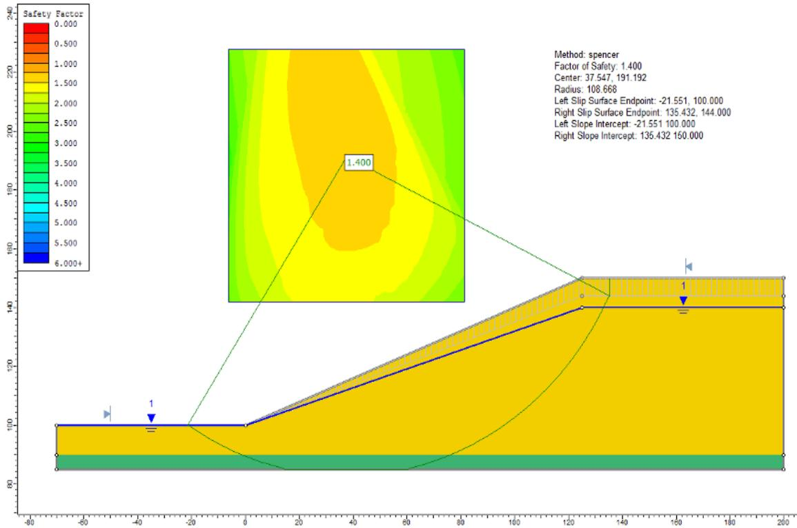
Figure 57.2: Noncircular failure surface, using Spencer method
