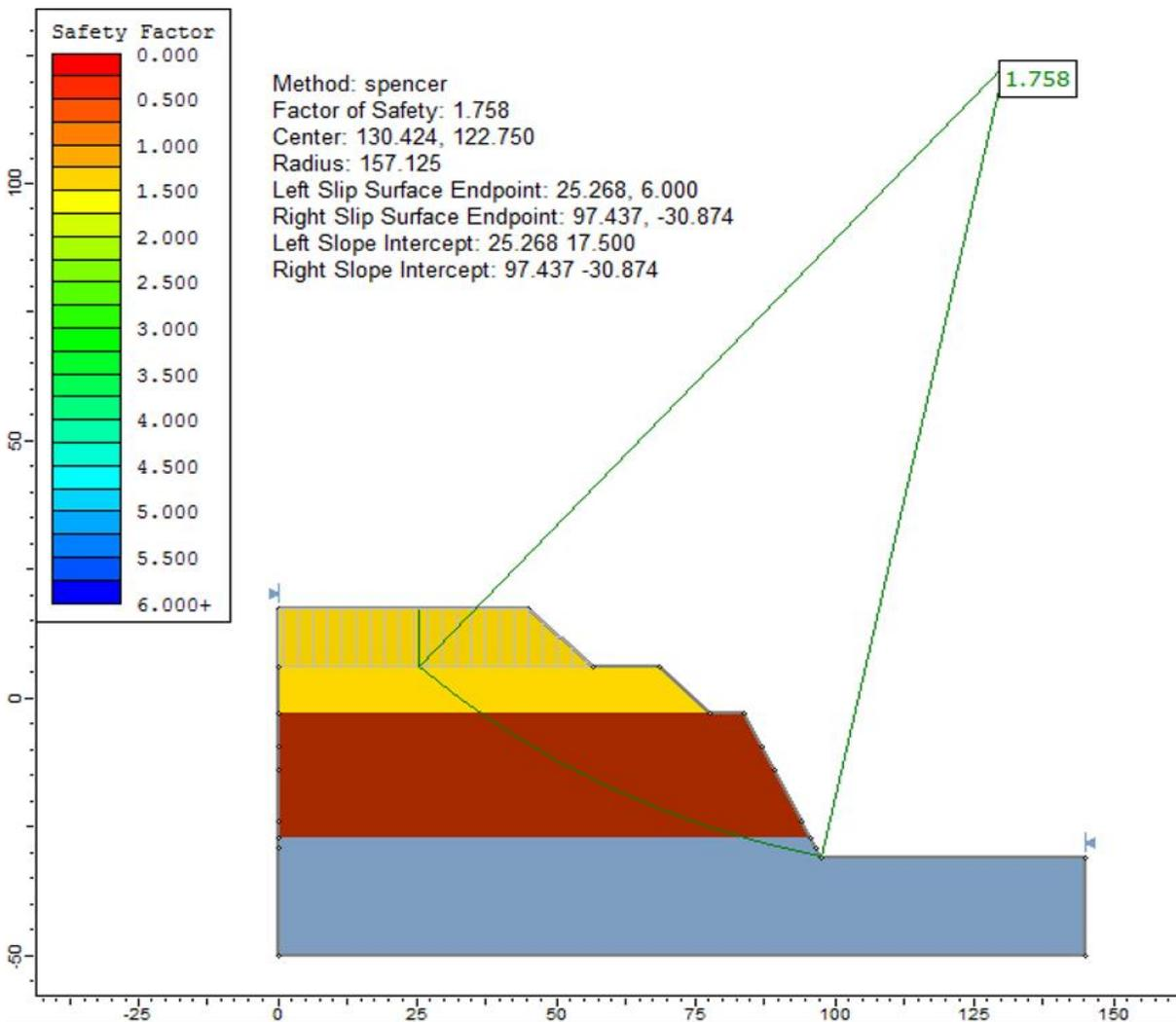
Figure 73.3: Solution, using the Spencer method (Circular)
