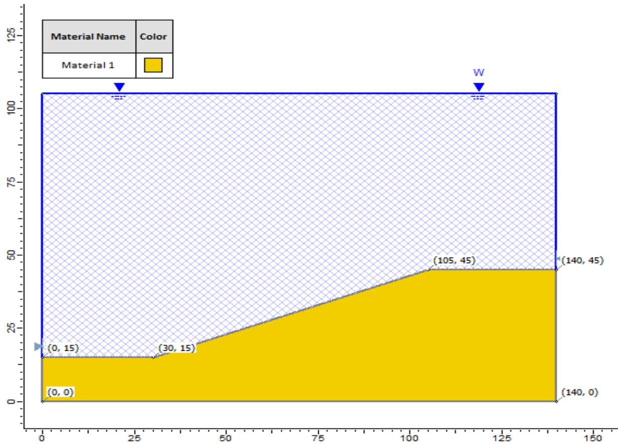
Figure 70.2: Water Table at 60' above the Crest (Case 2)
