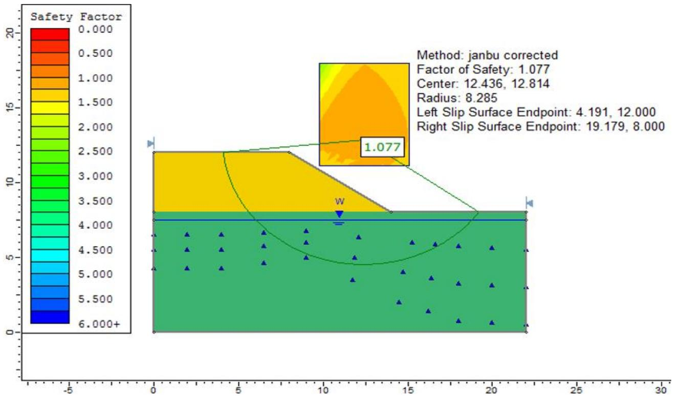
Figure 11.5: Solution, using the Janbu corrected method
