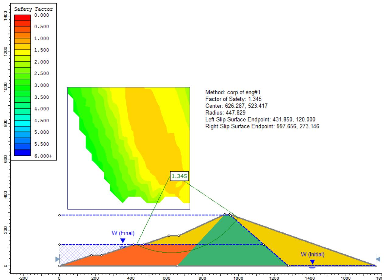
Figure 99.2: Solution Using Army Corp. Eng. 2-stage rapid drawdown method
