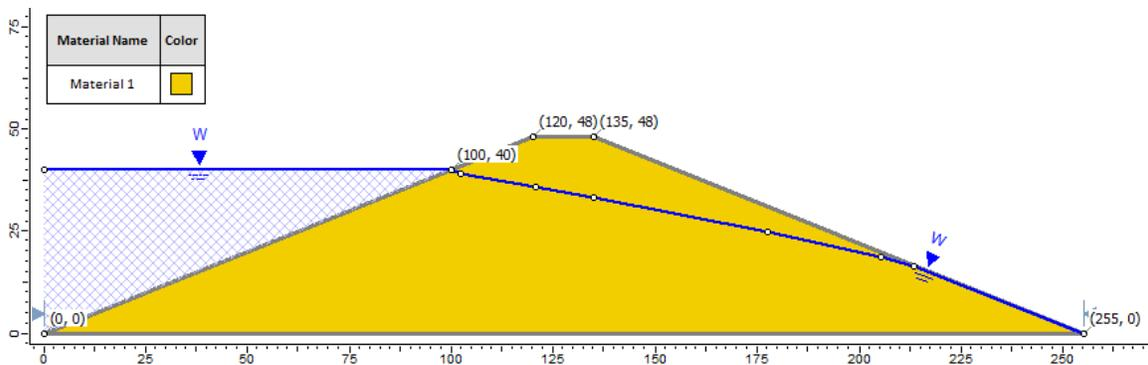
Figure 76.2: Piezometric Line Approximation
