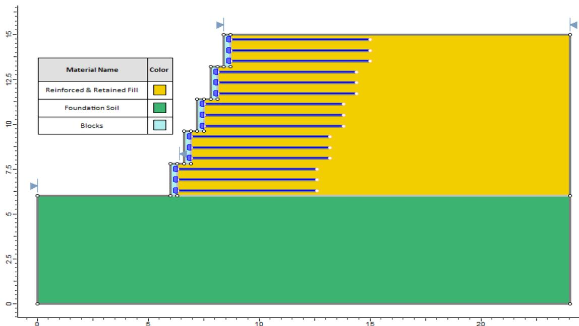
Figure 94.1: A Three-Tiered Wall in **Slide**
