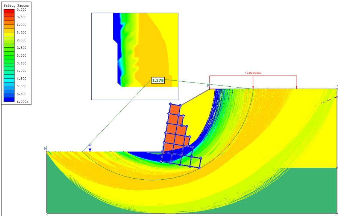
Figure 107.7: Solution for Mesh Method Using Circular Search and Bishop Method
