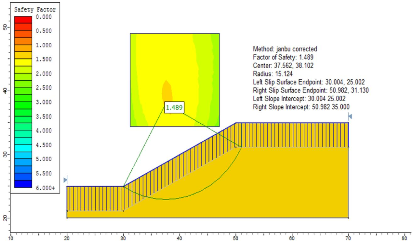
Figure 2.5: Solution, using the Janbu corrected method
