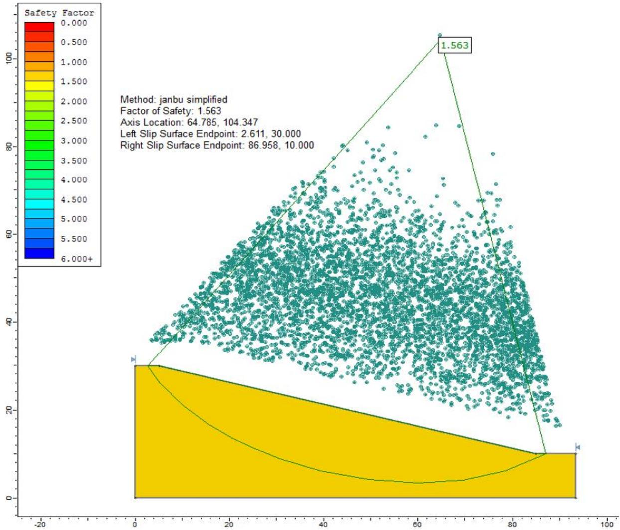
Figure 41.3: Solution, using the Janbu simplified method
