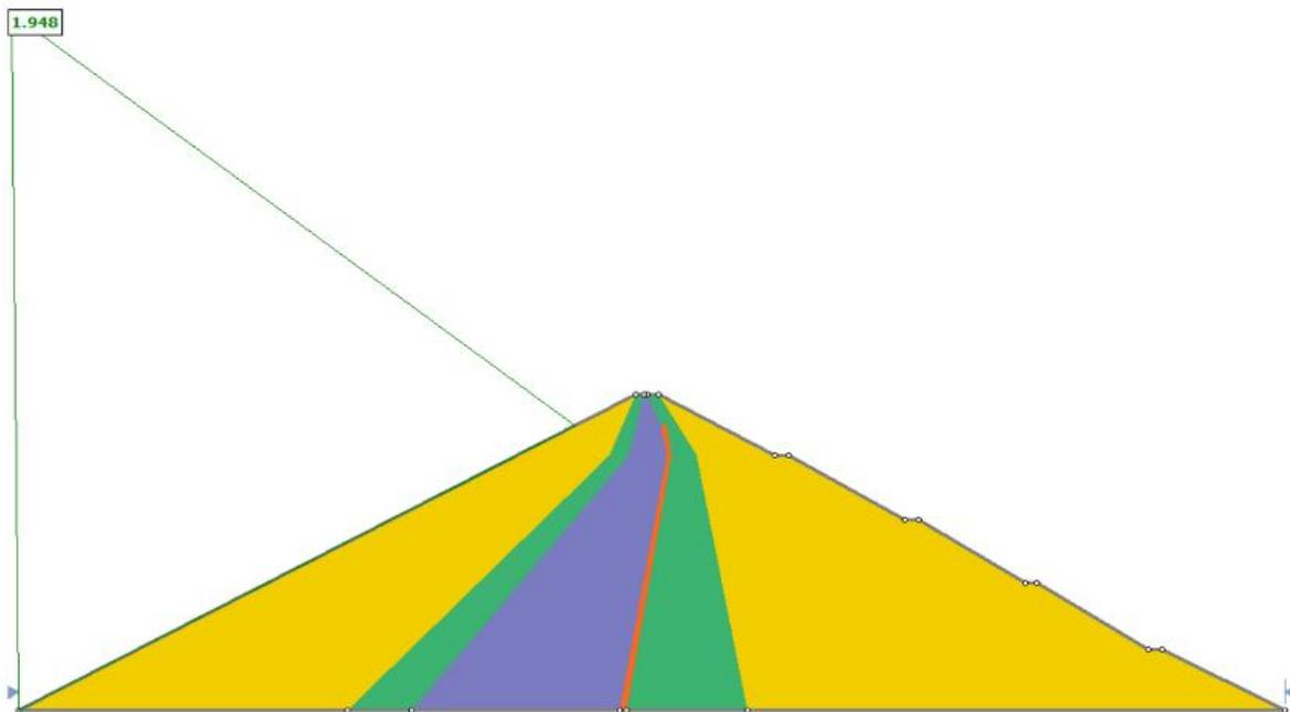
Figure 5.3: Solution, using the Bishop simplified method
