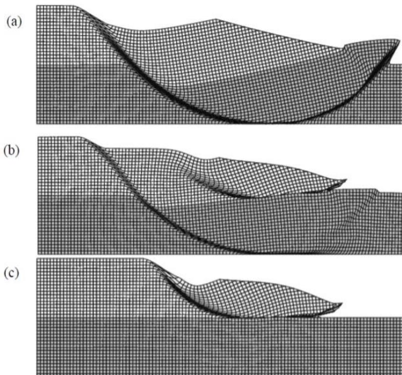
Fig. 5. Deformed meshes at failure for different strength ratios  $c_{u2}/c_{u1}$  ( $D = 2.0$  and  $\cot\beta=2.0$ ):
