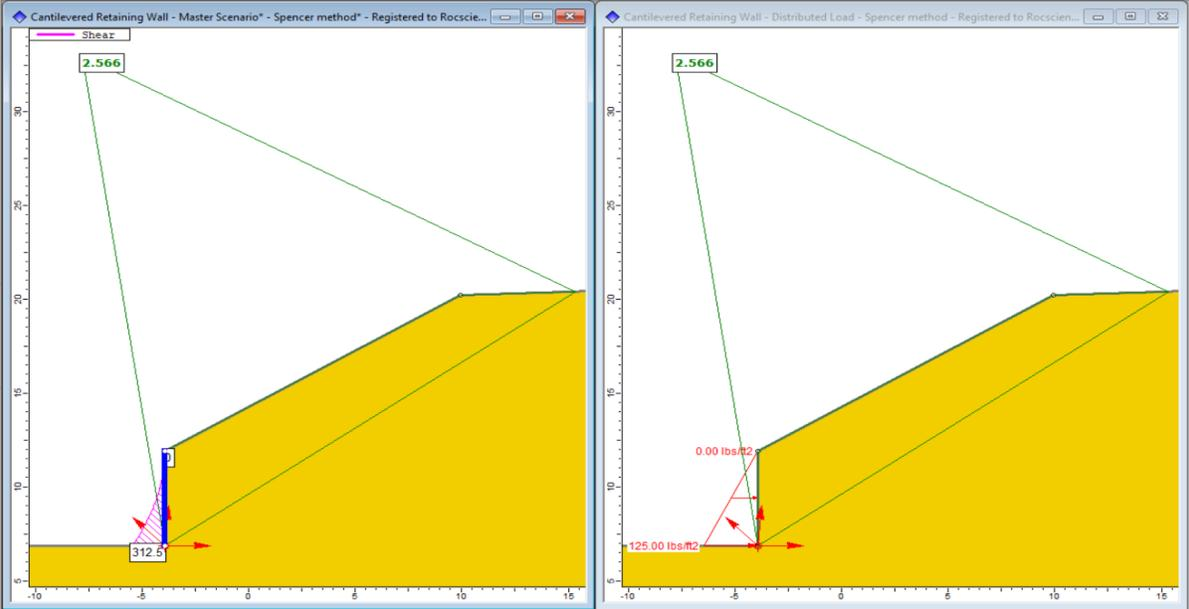
Figure 110.3 – Results using Spencer’s method are matching as expected
