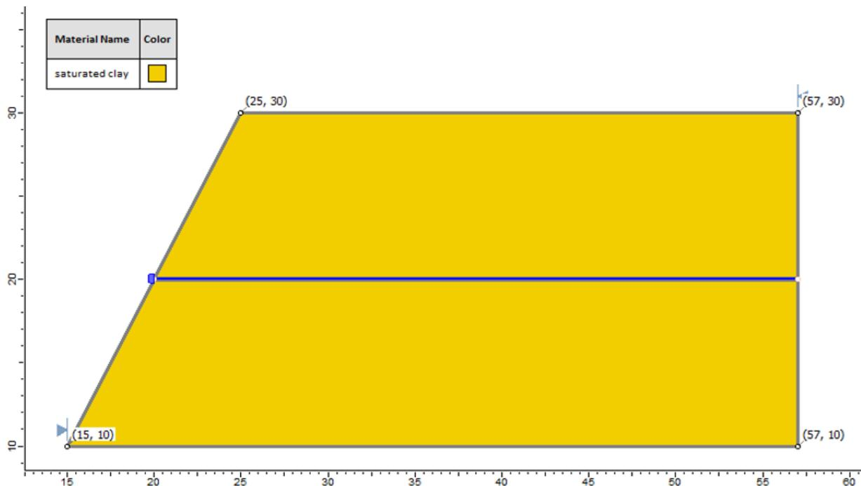
Figure 85.1: A Saturated Clay Slope in **Slide**
