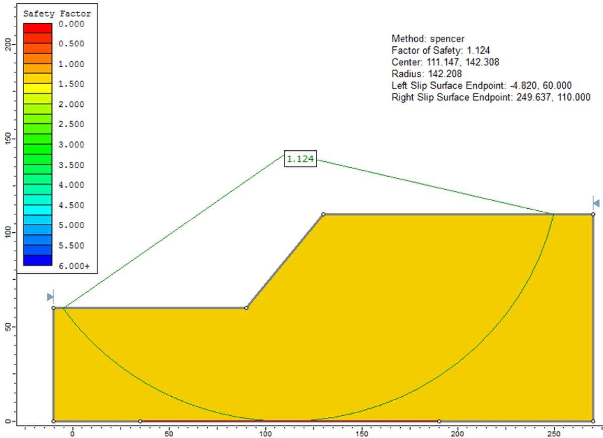
Figure 78.7: Solution to Case 3(b), using the Spencer method
