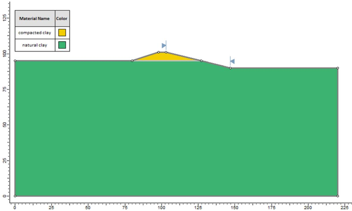
Figure 46.1: Geometry Setup in **Slide** – Stage 1
