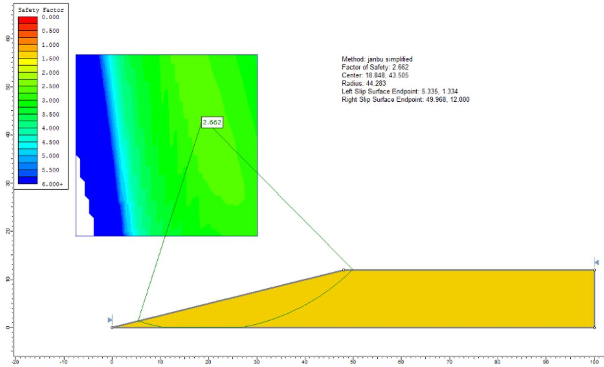
Figure 45.3: Critical failure surface, using the Mohr-Coulomb criterion, Janbu simplified
