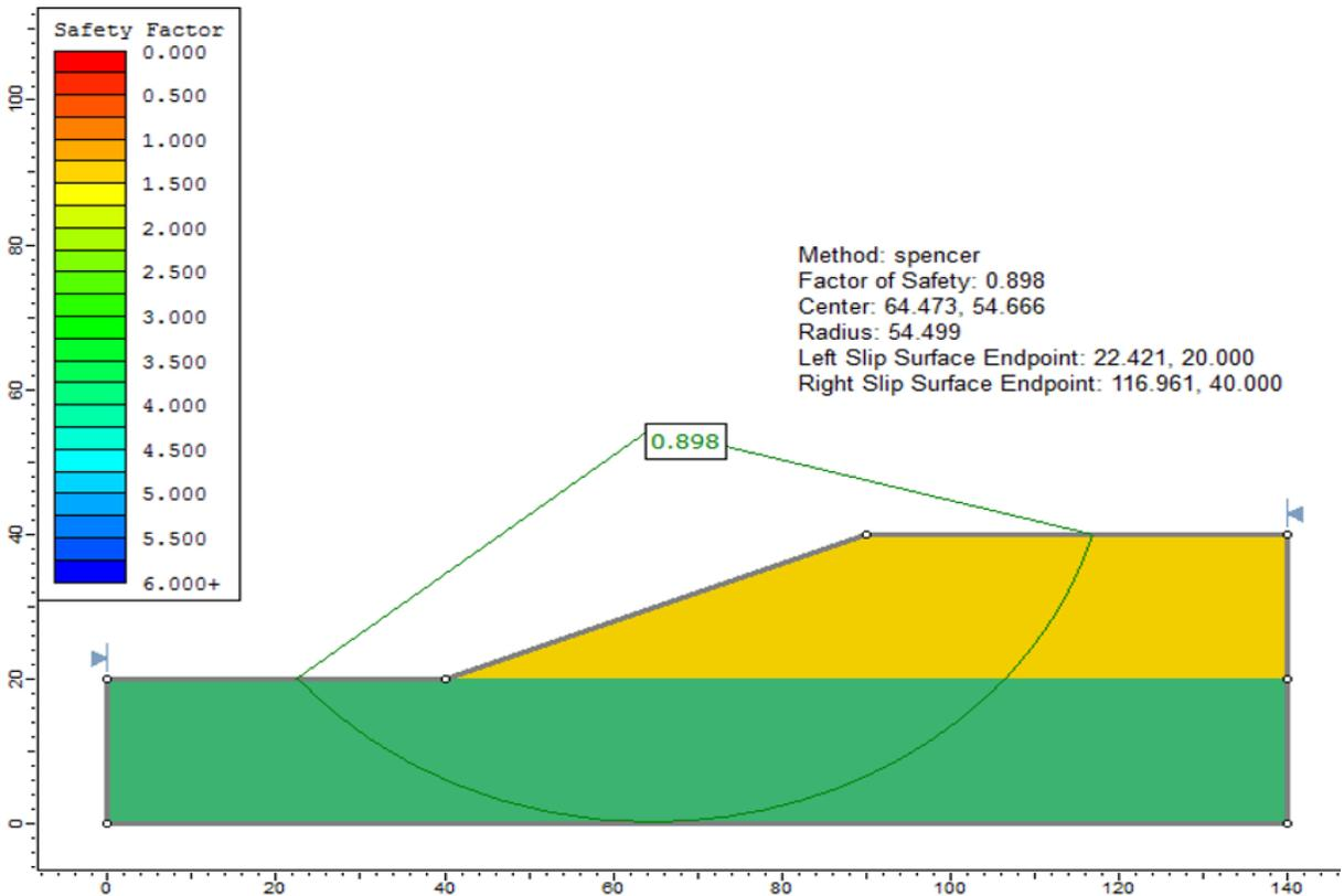
Figure 84.3: Solution to Case 2, using the Spencer method
