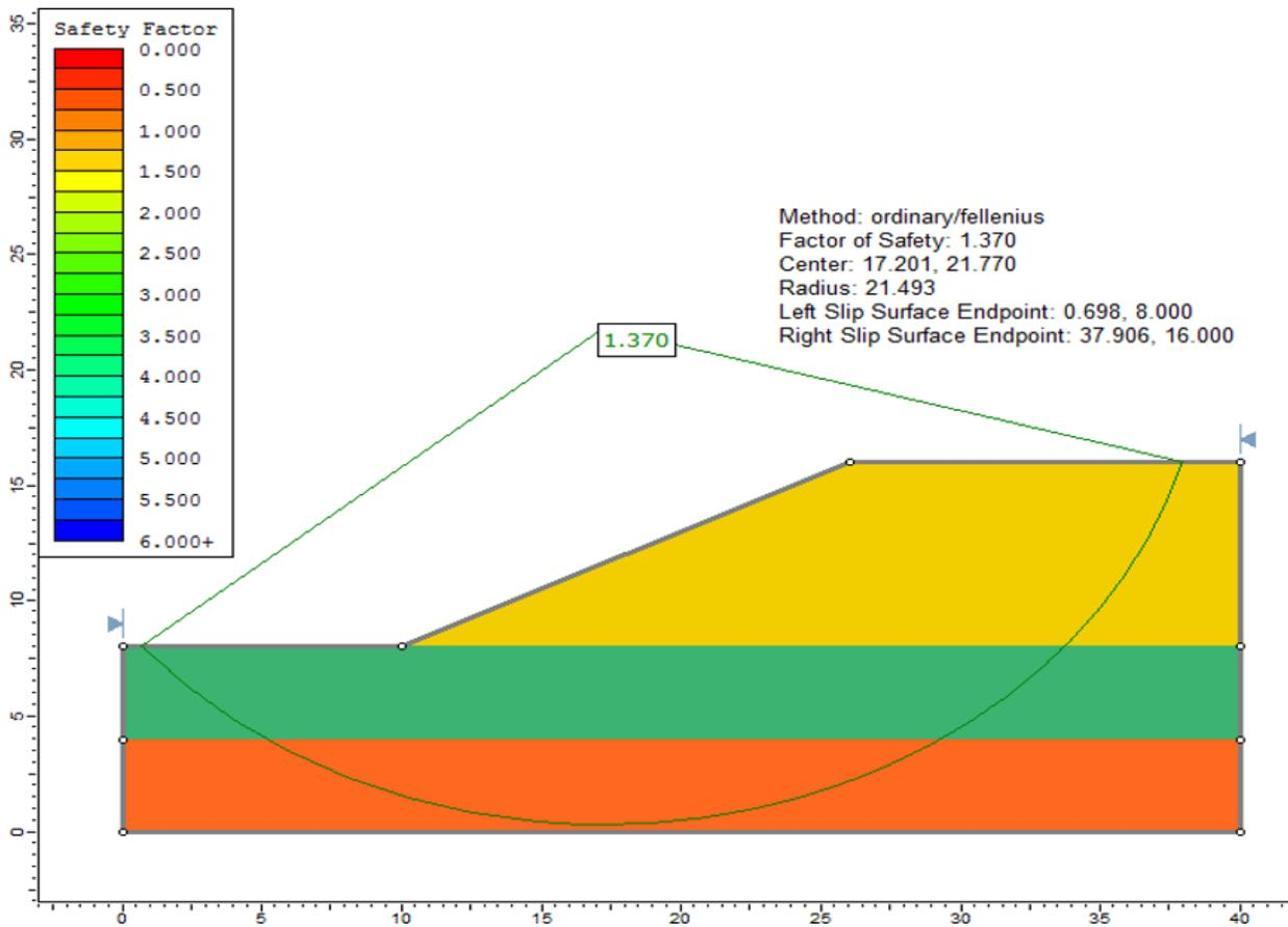
Figure 23.2: Circular failure surface using the Ordinary/Fellenius method
