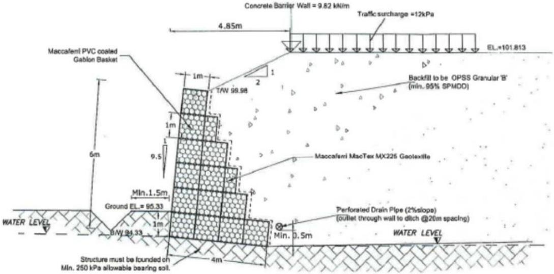
Figure 107.1: Drawing of gabion wall provided by Cao et Al. (2016)
