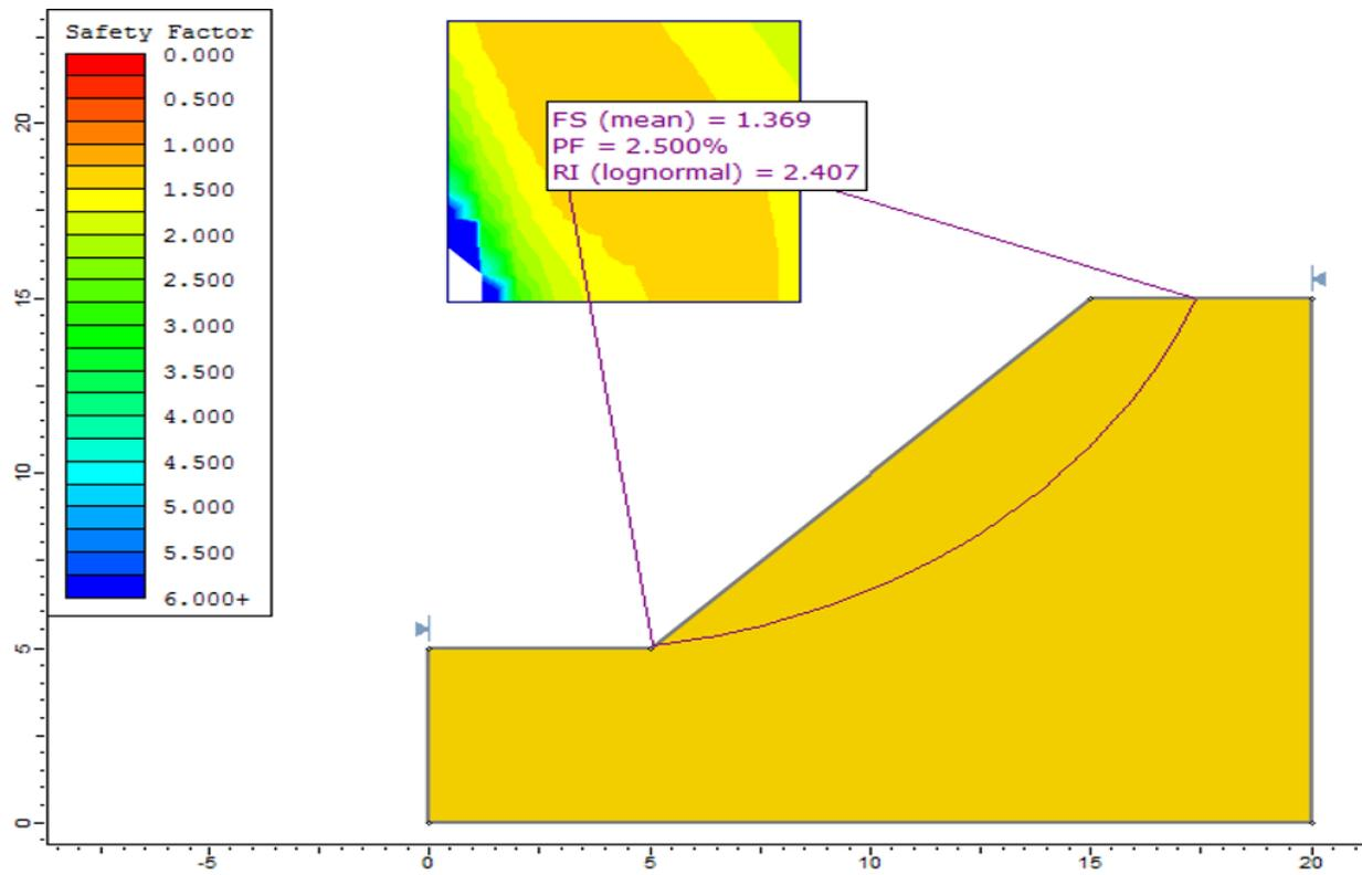
Figure 36.3: Critical probabilistic surface
