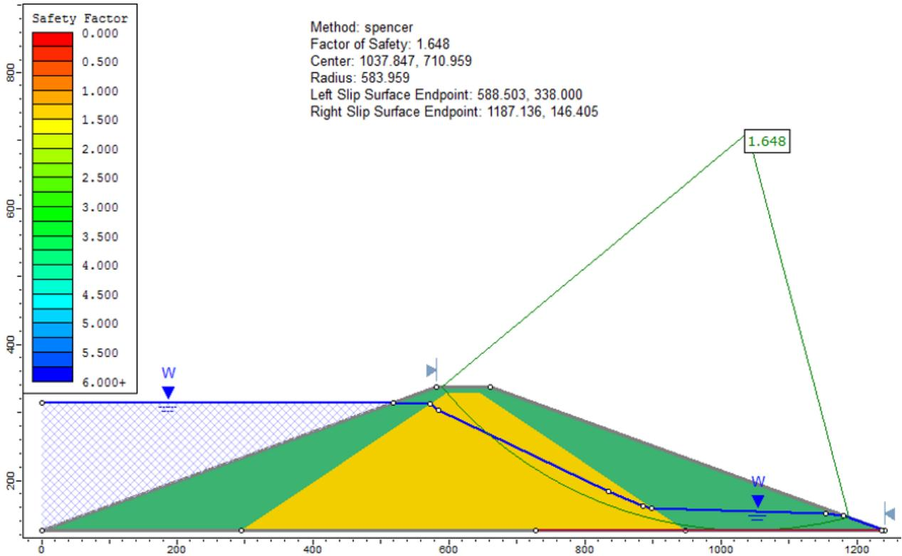
Figure 77.4: Solution to Case 2, using the Spencer method
