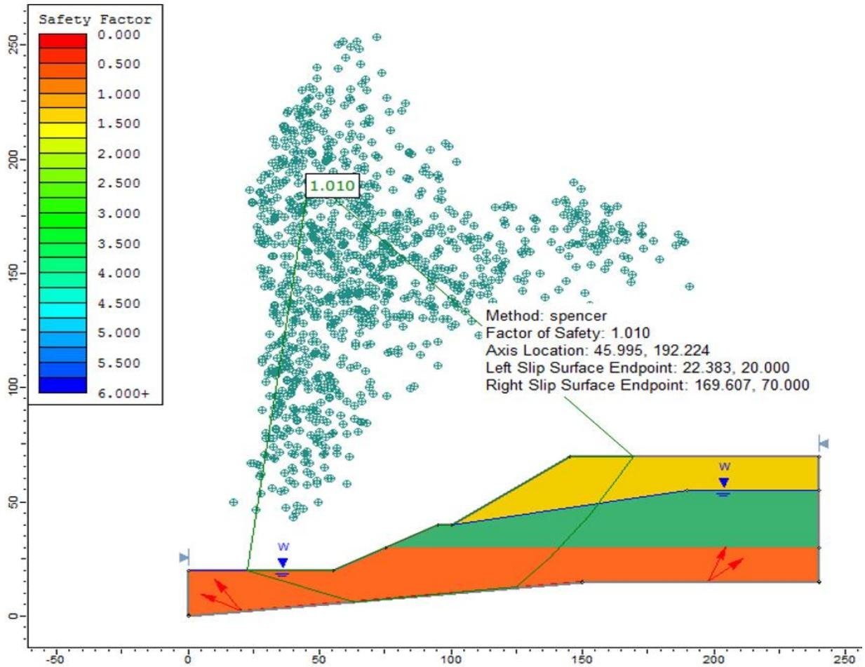
Figure 20.4: Noncircular failure surface using the Spencer method and block search
