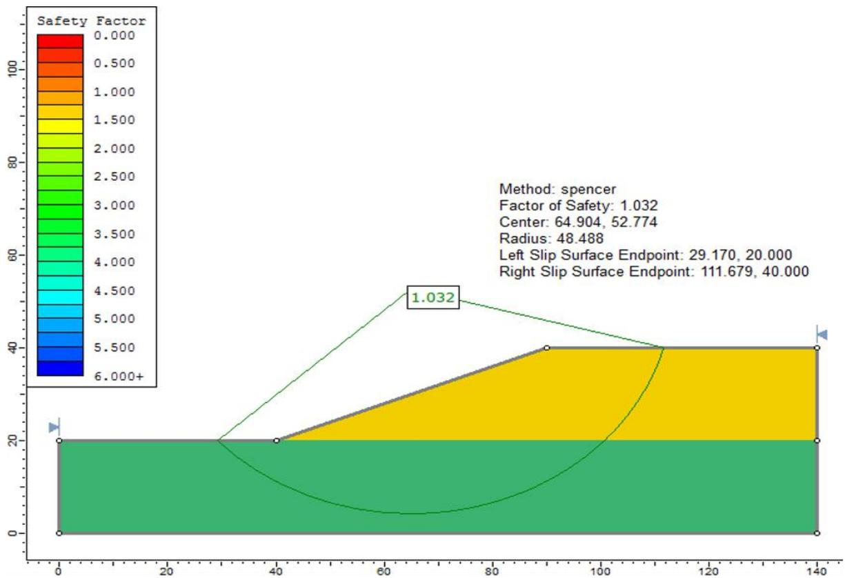
Figure 84.4: Solution to Case 3, using the Spencer method
