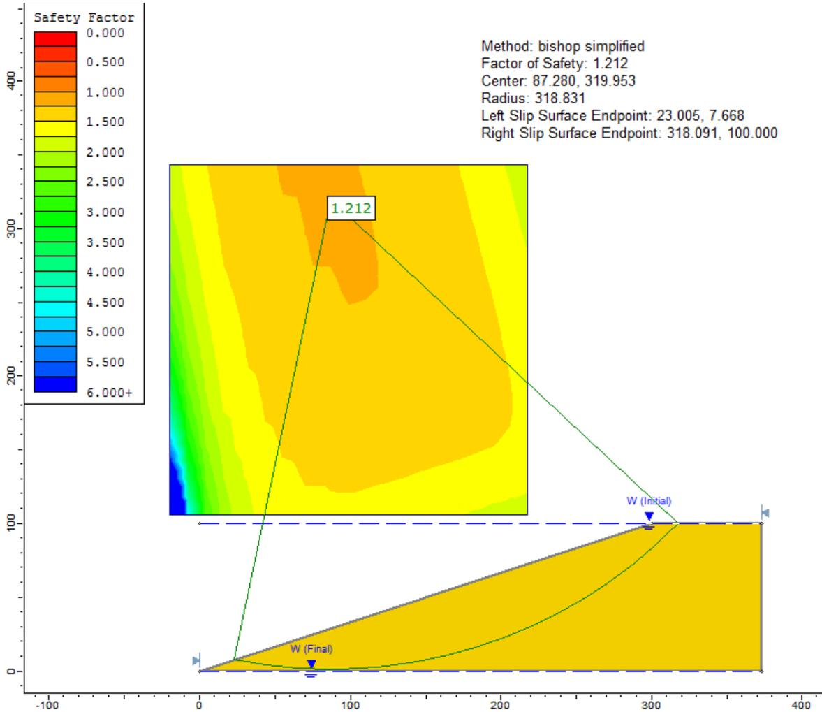
Figure 100.2: Solution, using B-Bar rapid drawdown method
