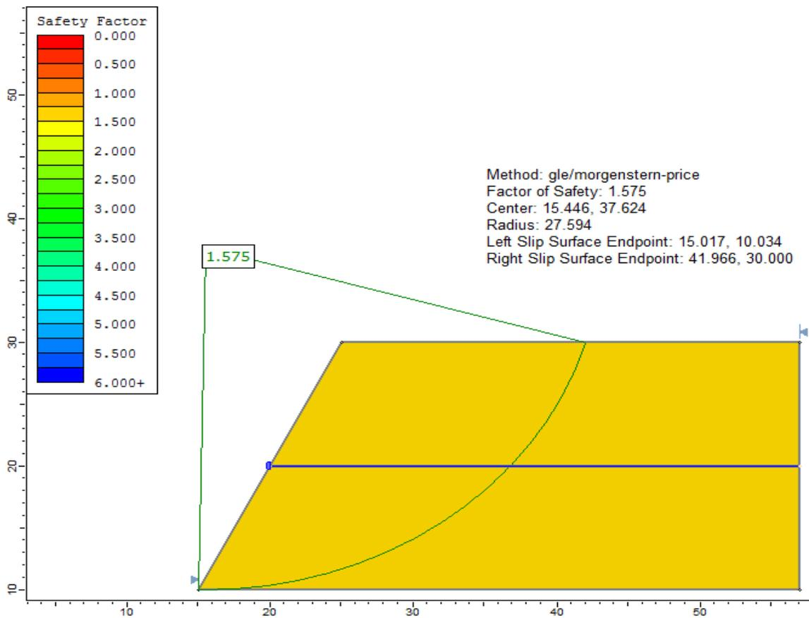
Figure 85.2: Solution to Case 1, using the GLE method
