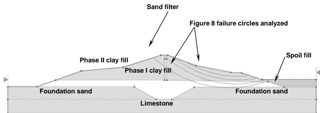
Figure 35.4 Slide Setup for the original Figure 8
