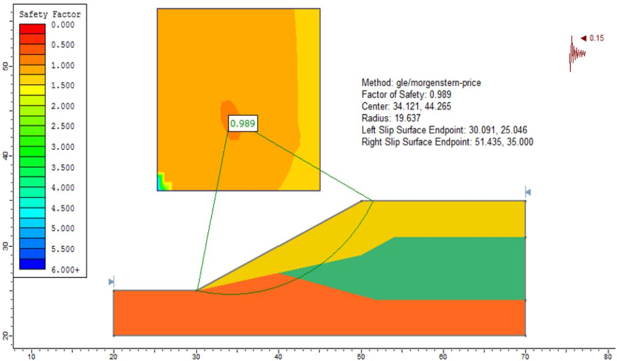
Figure 4.4: Solution, using the GLE method
