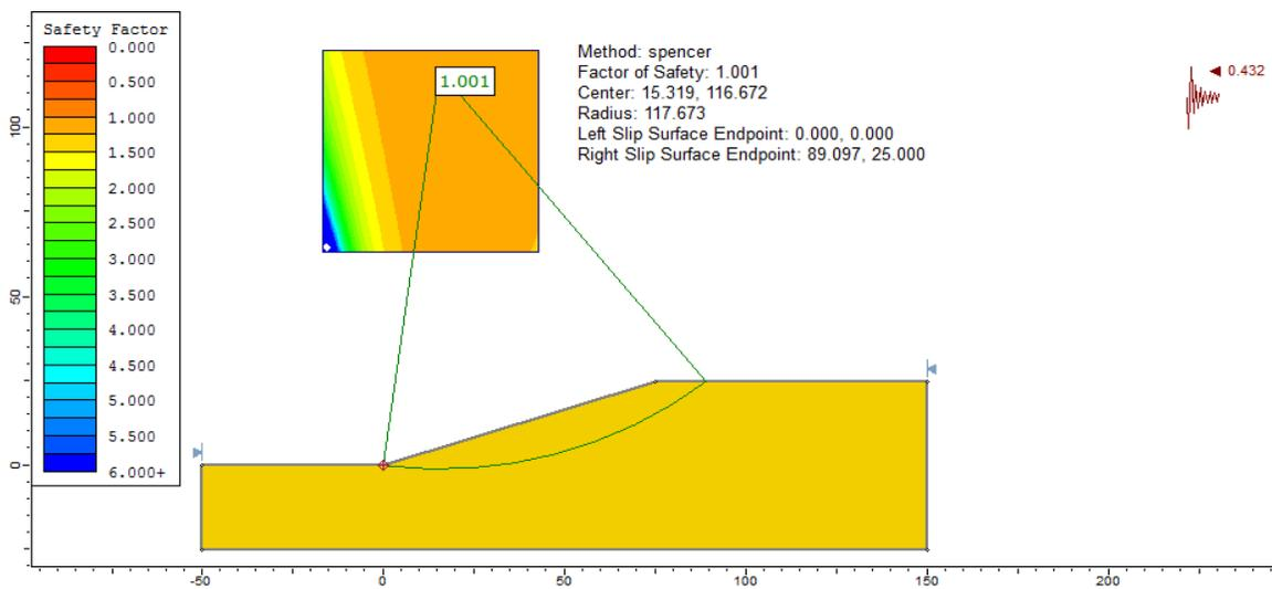
Figure 62.2: Circular slip surface, using the Spencer method
