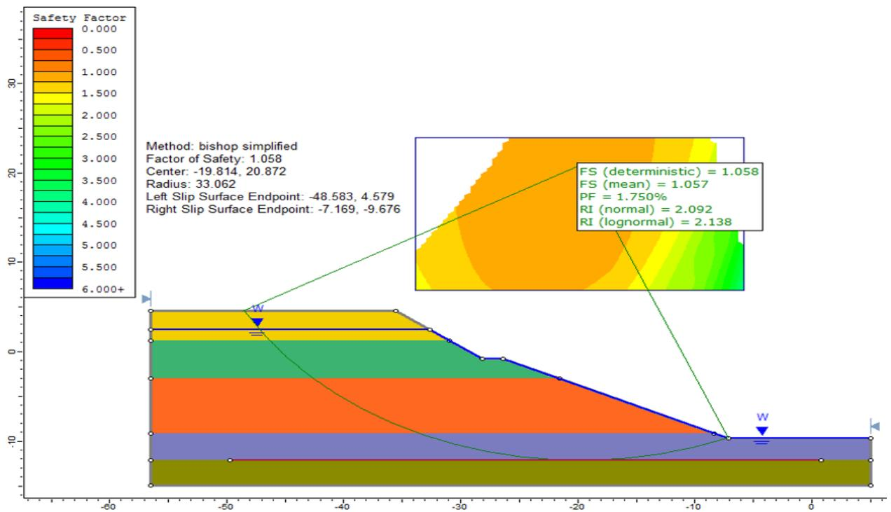
Figure 28.6: Critical slip circle tangential to lower boundary of clay layer 3
