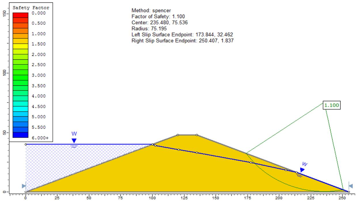
Figure 76.4: Solution to Case 2, using the Spencer method (Circular)
