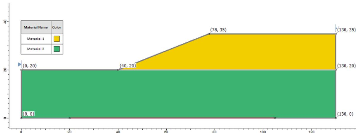
Figure 79.1: A Cohesionless Earth Embankment
