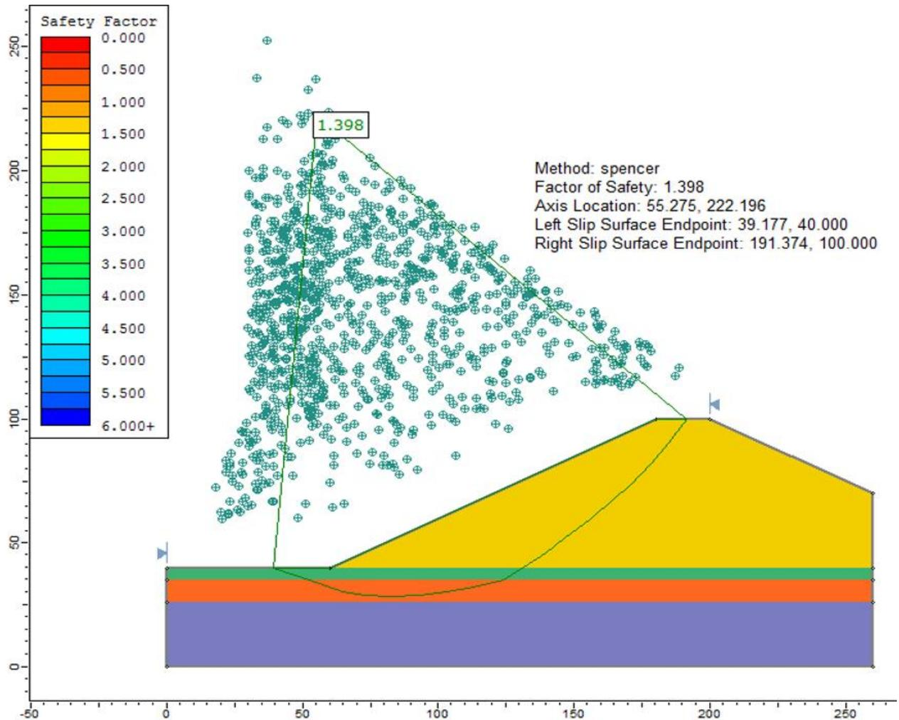
Figure 19.2: Noncircular failure surface, using the Spencer method
