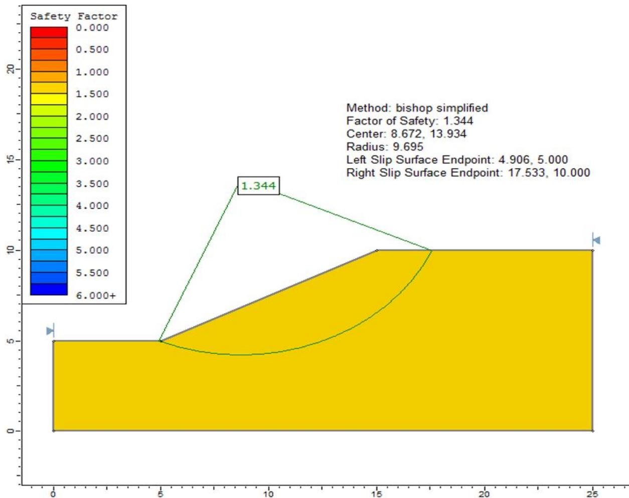
Figure 17.2: Circular failure surface, using the Bishop simplified method
