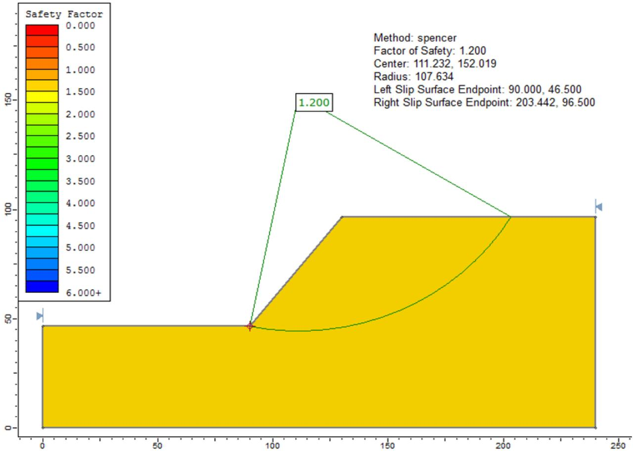
Figure 78.4: Solution to Case 2(a), using the Spencer method
