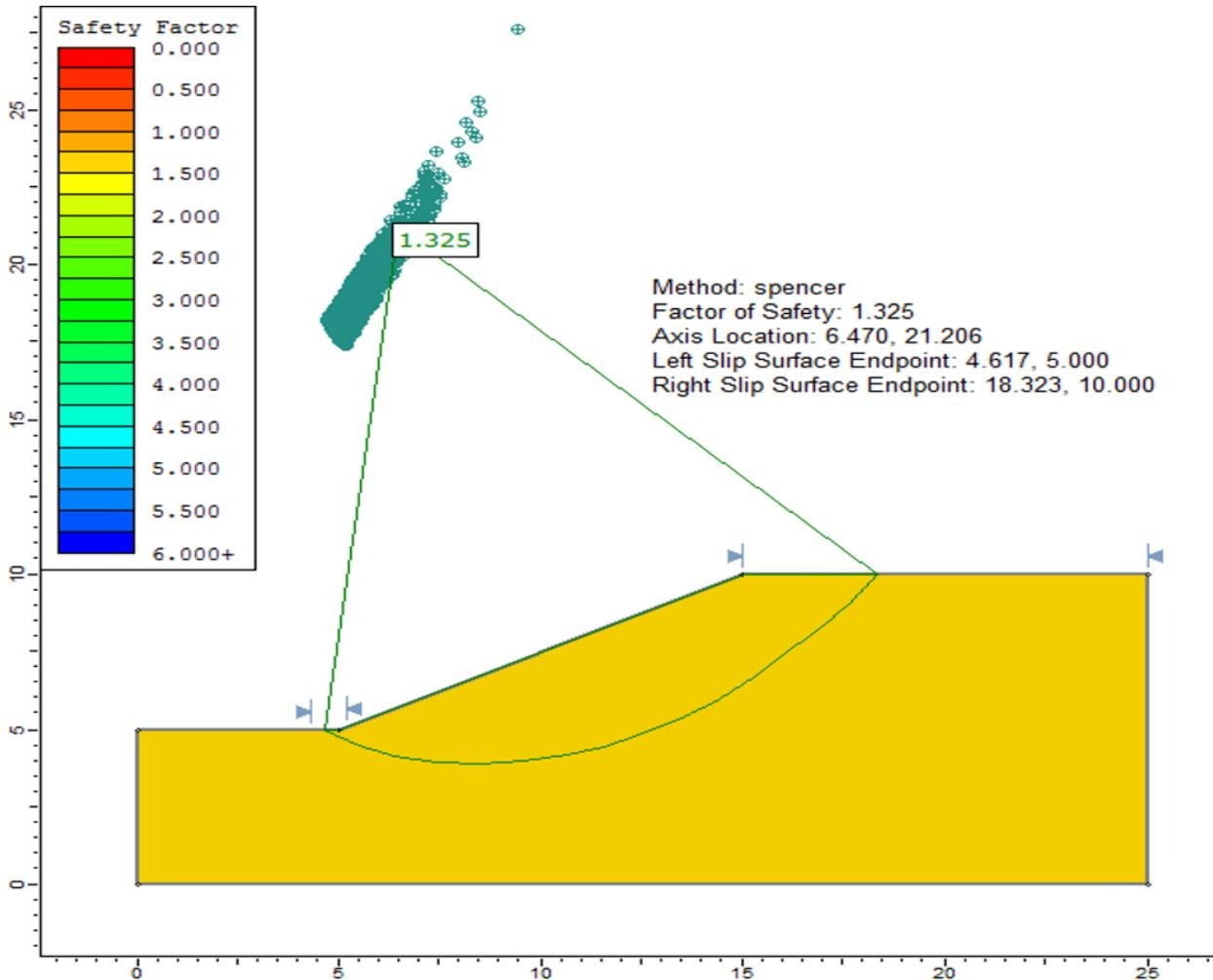
Figure 17.3: Noncircular failure surface, using the Spencer method
