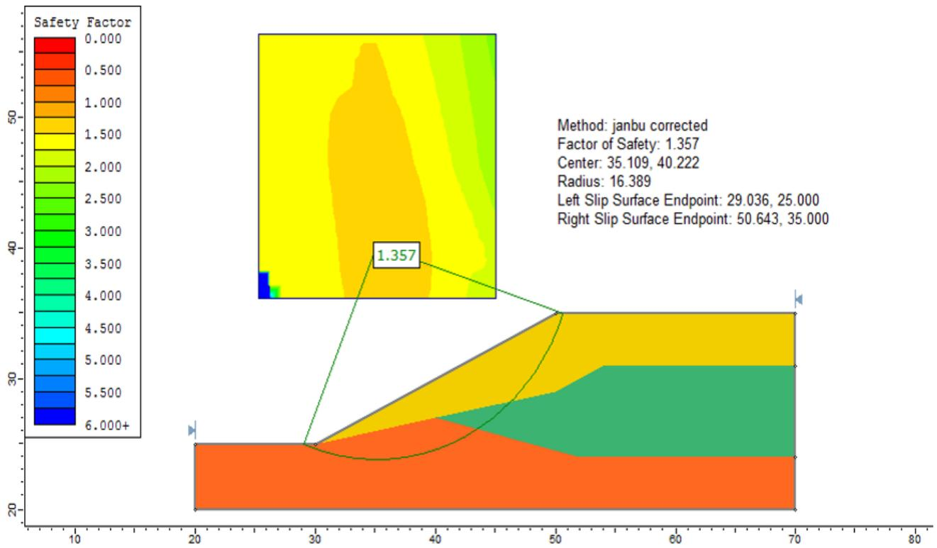
Figure 3.5: Solution, using the Janbu corrected method
