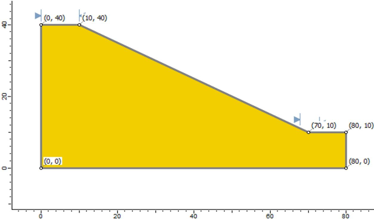
Figure 18.1: Geometry Setup in Slide
