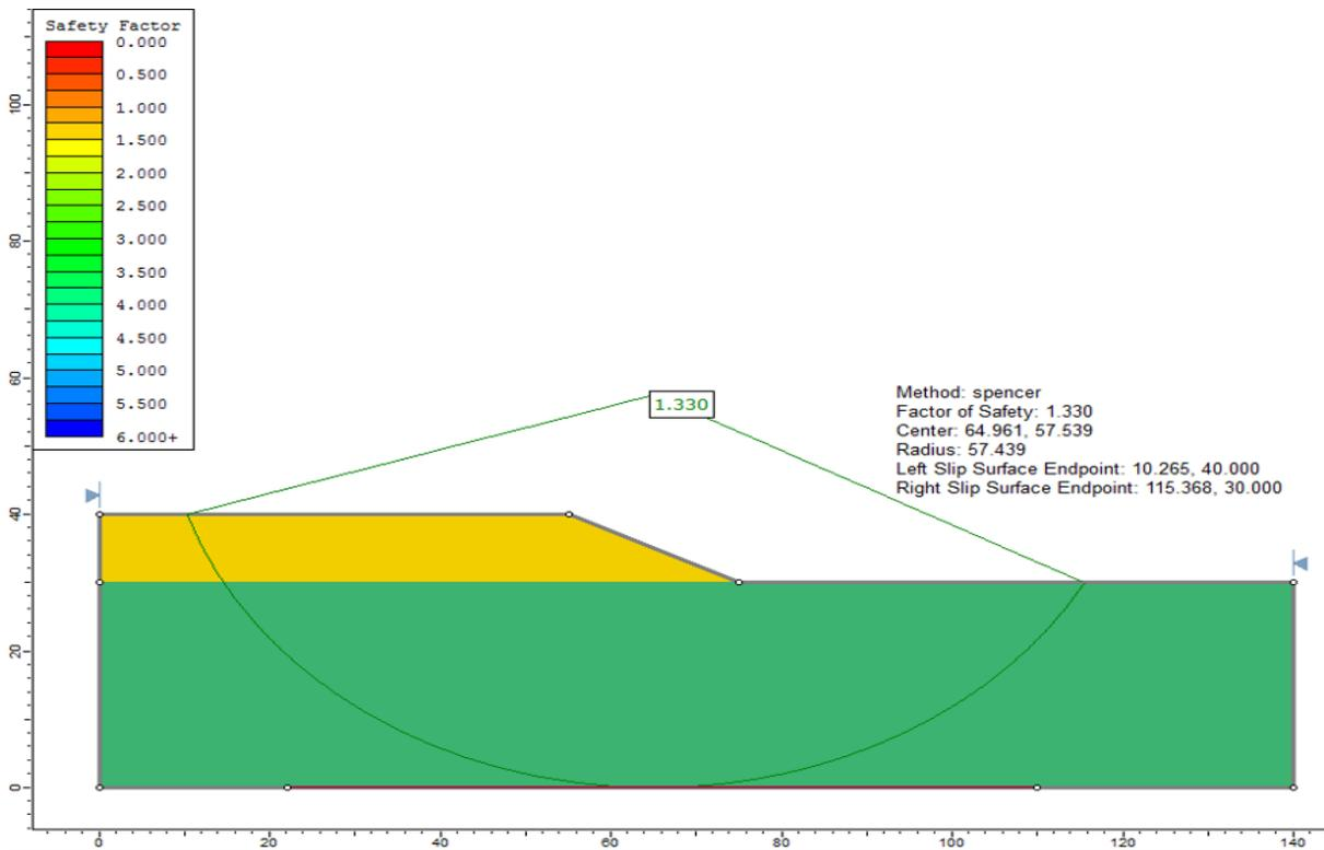
Figure 83.4: Solution to Case 2, using the Spencer method
