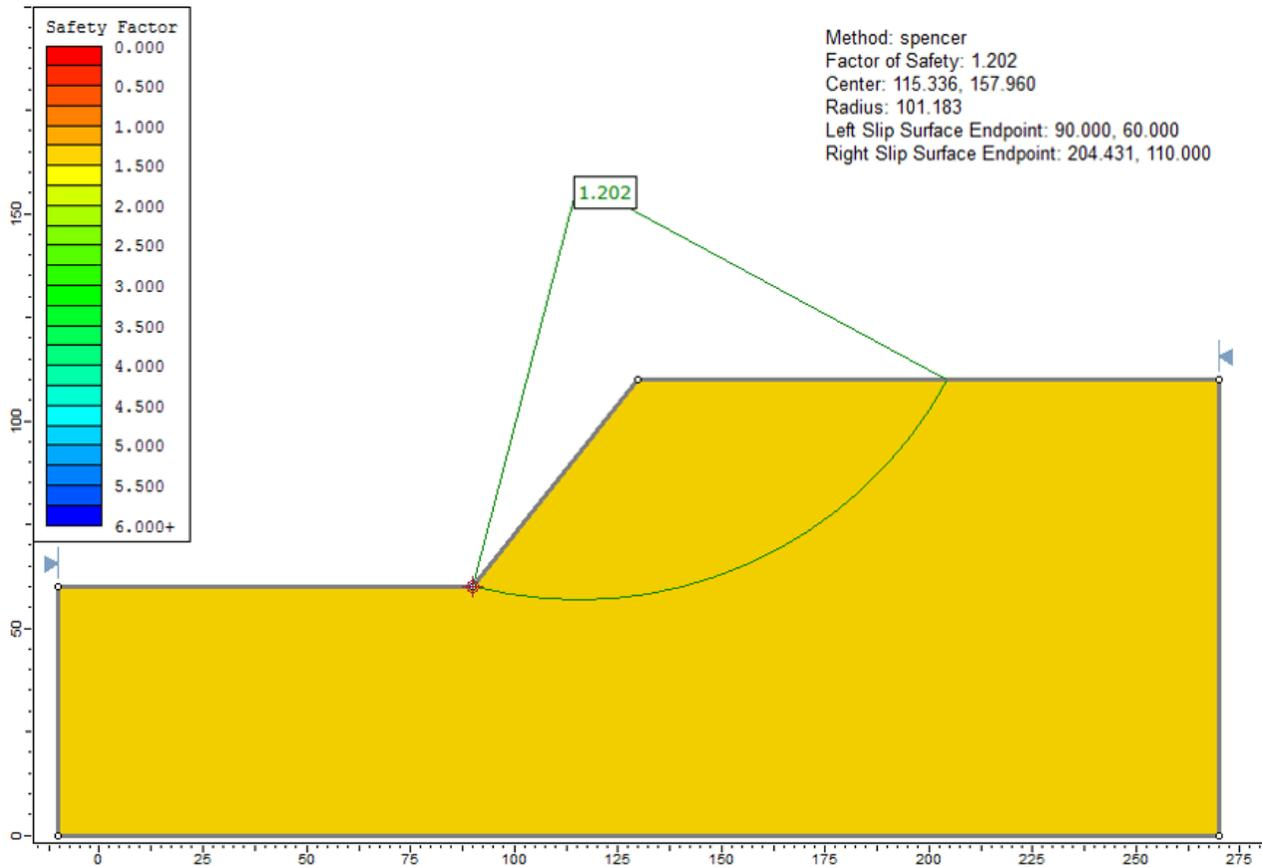
Figure 78.6: Solution to Case 3(a), using the Spencer method
