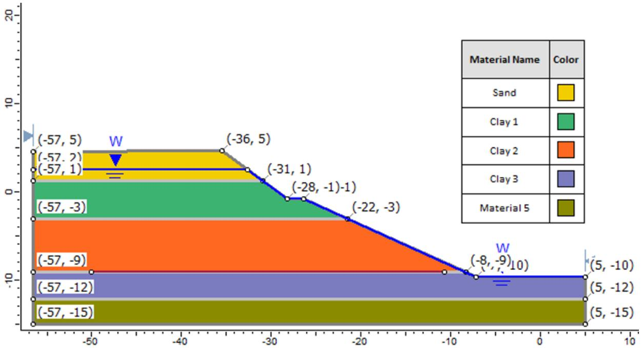
Figure 28.1: Geometry for Example 1 – 4 (excavated slope)
