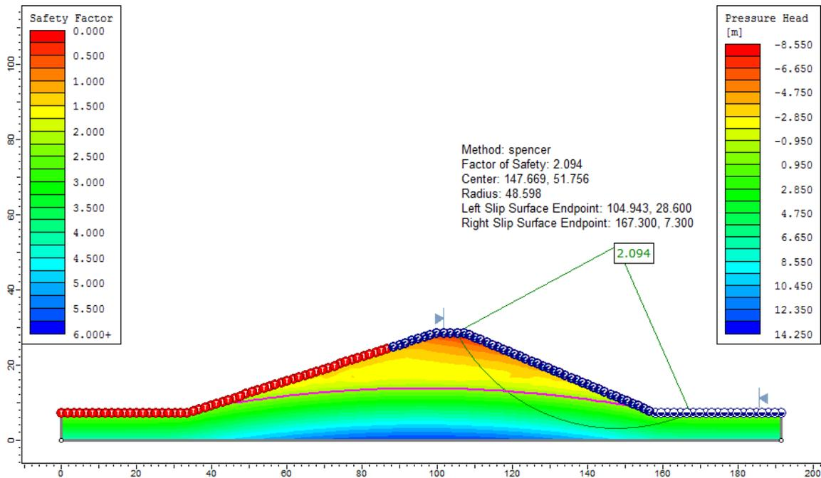
Figure 102.7: **Slide** Results for  $\phi^b = 0^\circ$  at 300 h, using the Spencer method
