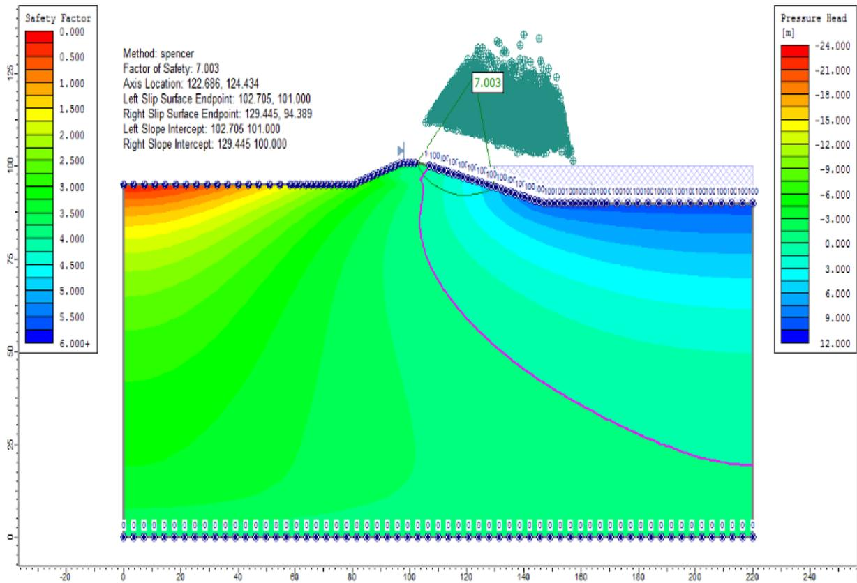
Figure 46.6: Critical failure surface, using the Spencer method
