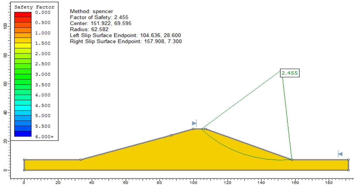
Figure 102.2: **Slide** Results for Dry Conditions, using the Spencer method
