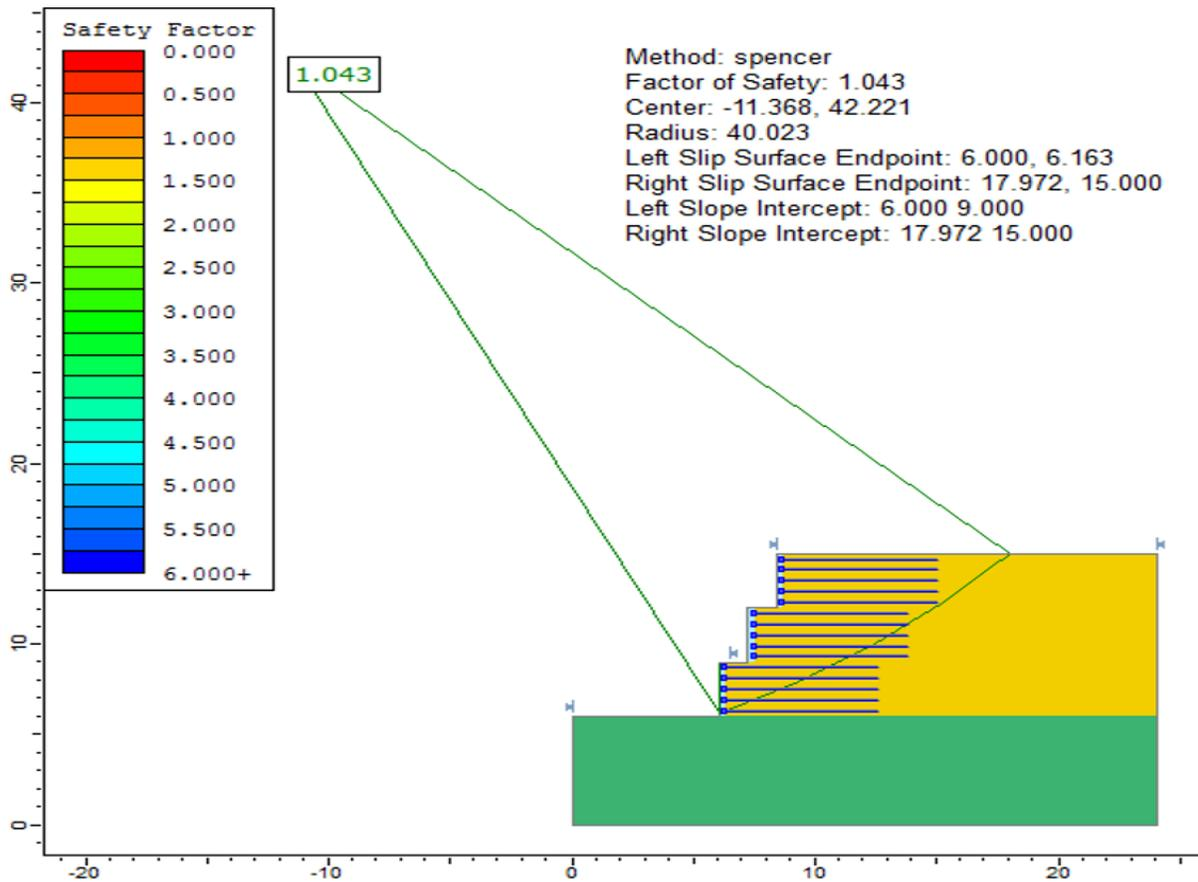
Figure 88.2: Solution, using the Spencer method
