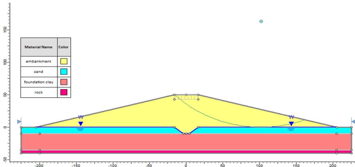
Figure 64.1: Geometry Setup in Slide
