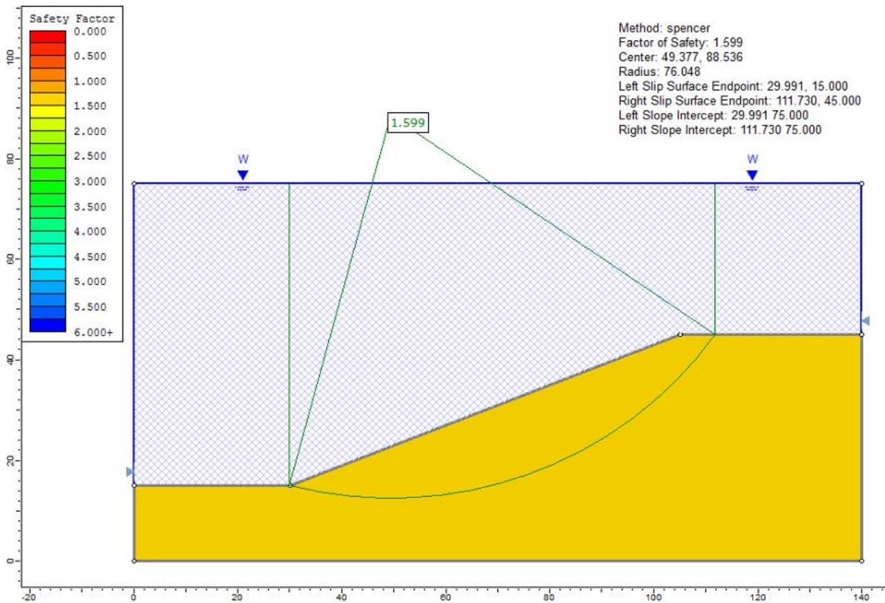
Figure 70.3: Solution to case 1 (circular), using the Spencer Method
