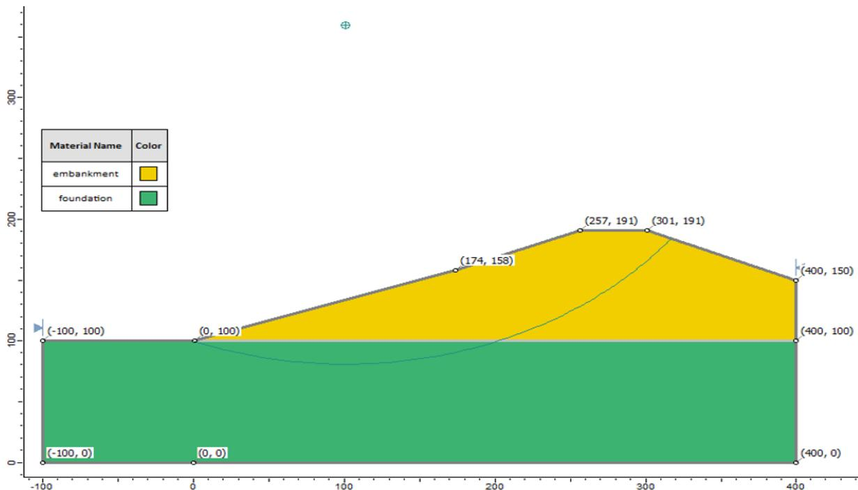
Figure 67.1: Geometry Setup in **Slide**
