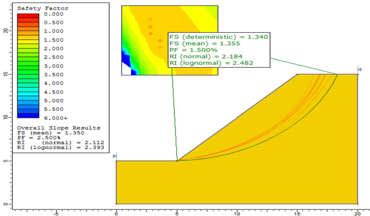
Figure 36.2: Critical deterministic surface and overall result
