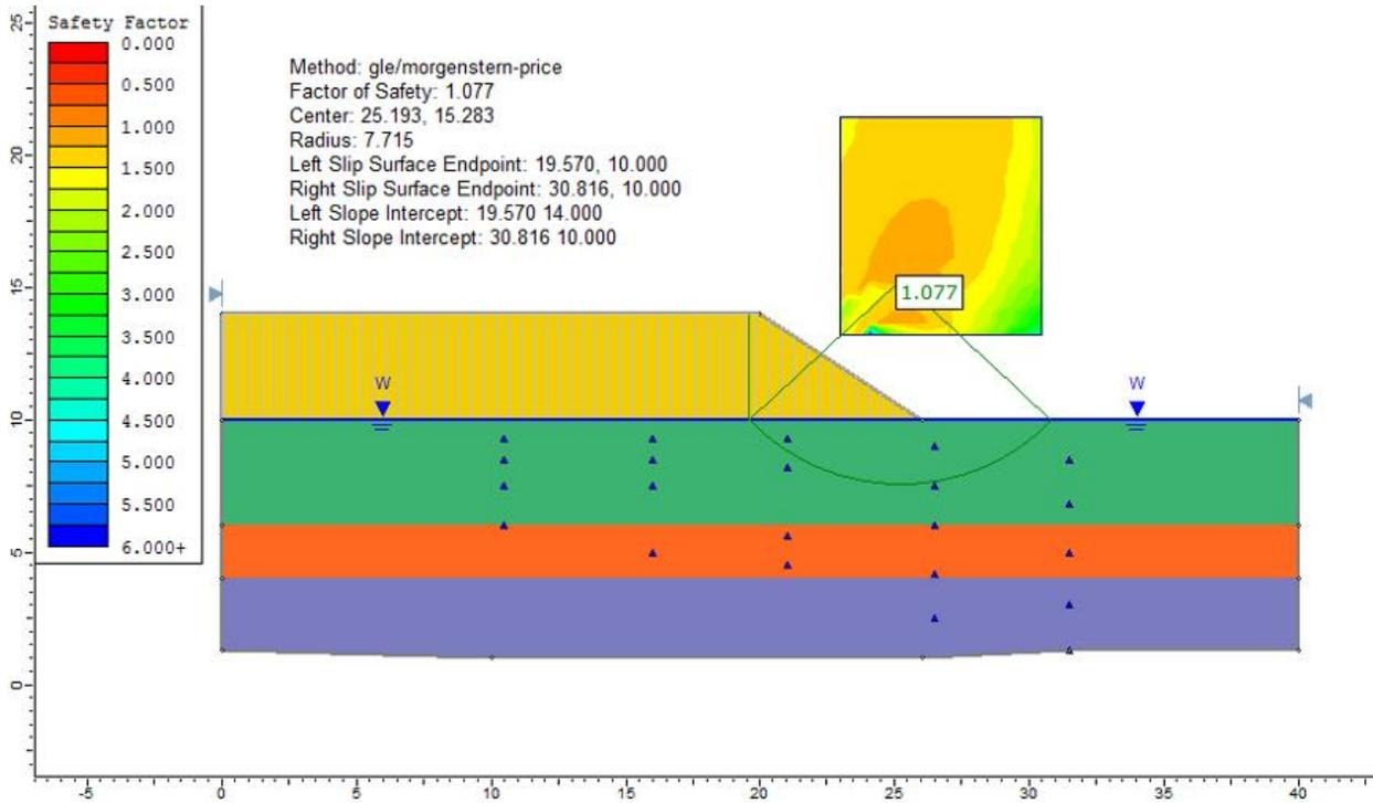
Figure 12.4: Solution, using the GLE method
