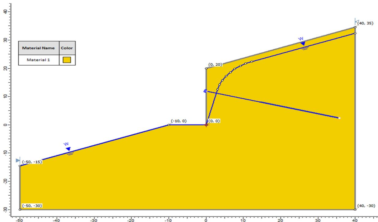
Figure 59.1: Geometry Setup in **Slide**
