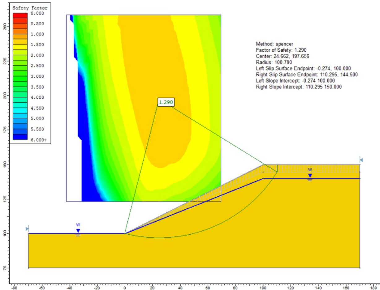
Figure 56.2: Circular failure surface, using the Spencer method
