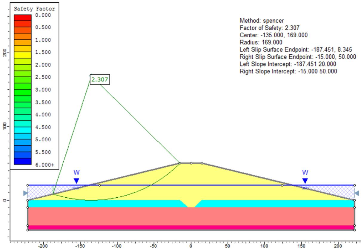
Figure 66.2: Solution, using the Spencer method
