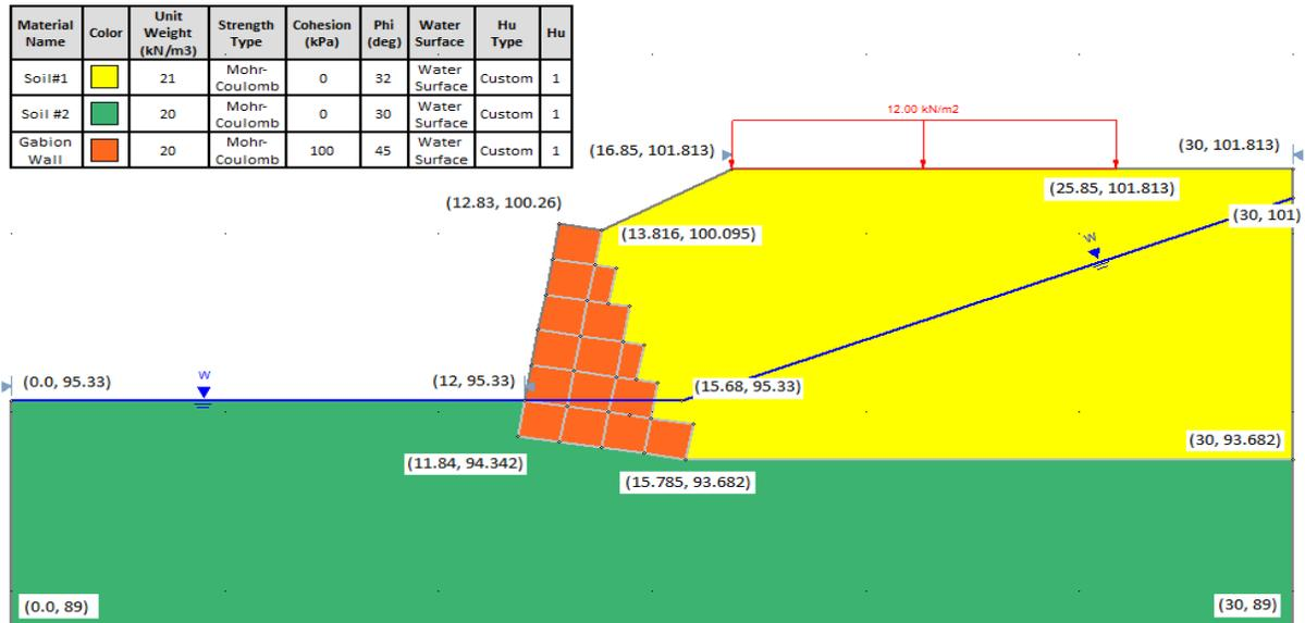
Figure 107.3: Gabion Wall Model in **Slide** (equivalent cohesion method)
