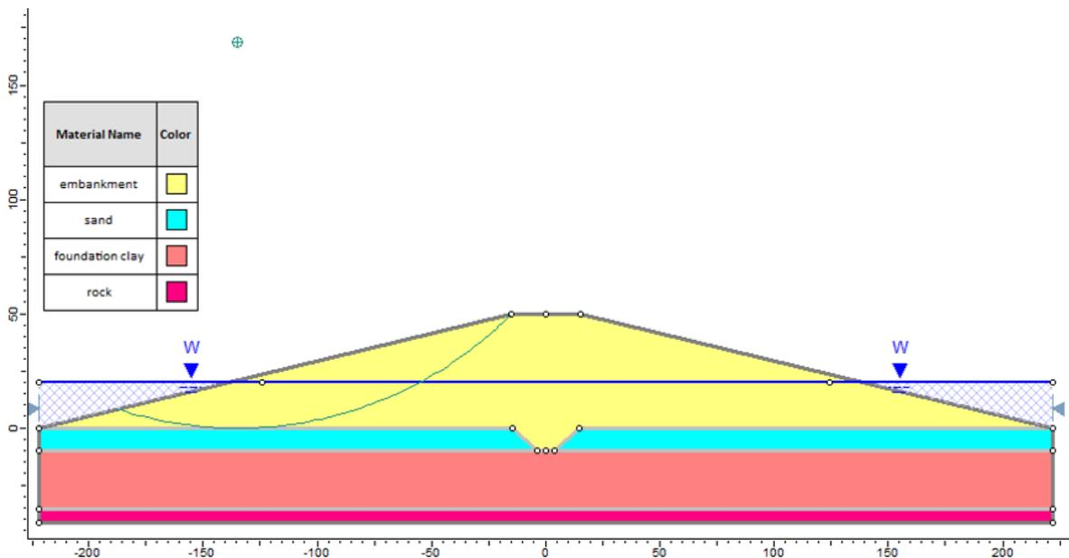
Figure 66.1: Geometry Setup in **Slide**
