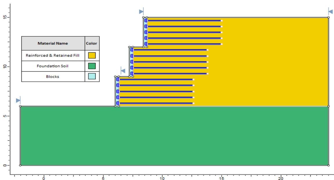
Figure 91.1: A Three-Tiered Wall in **Slide**
