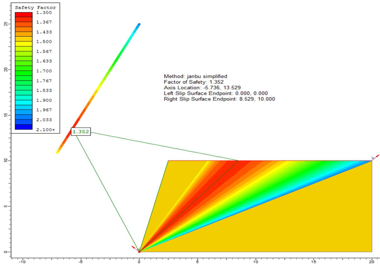
Figure 43.4 – Planar failure surfaces, using Janbu simplified method
