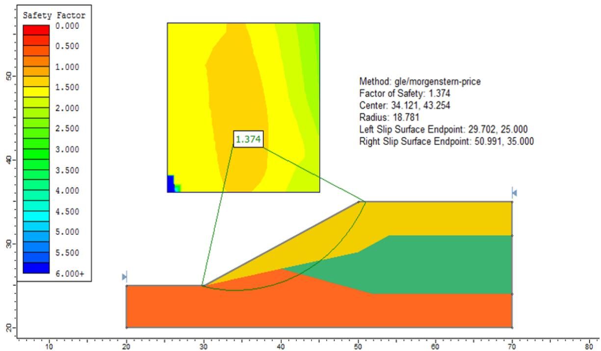
Figure 3.4: Solution, using the GLE method
