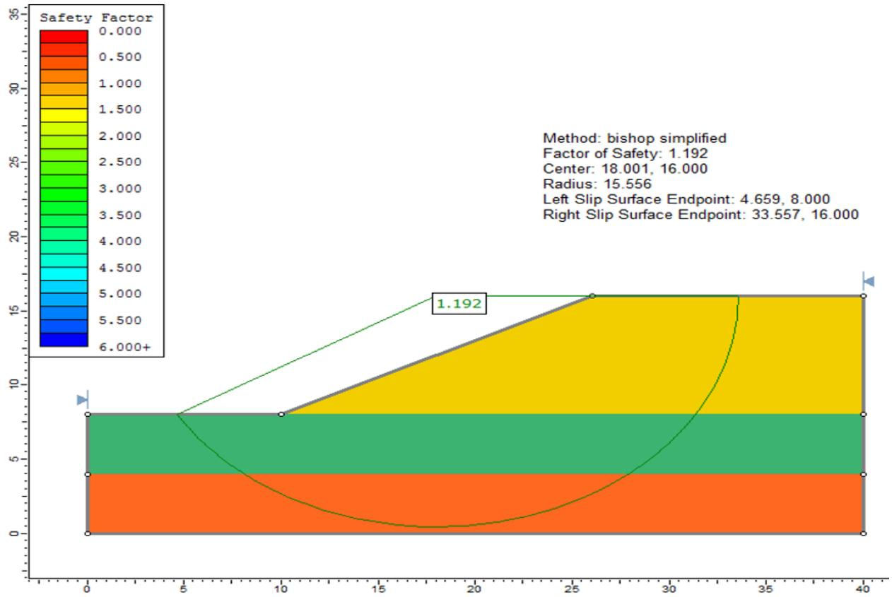
Figure 23.3: Circular failure surface using the Bishop simplified method
