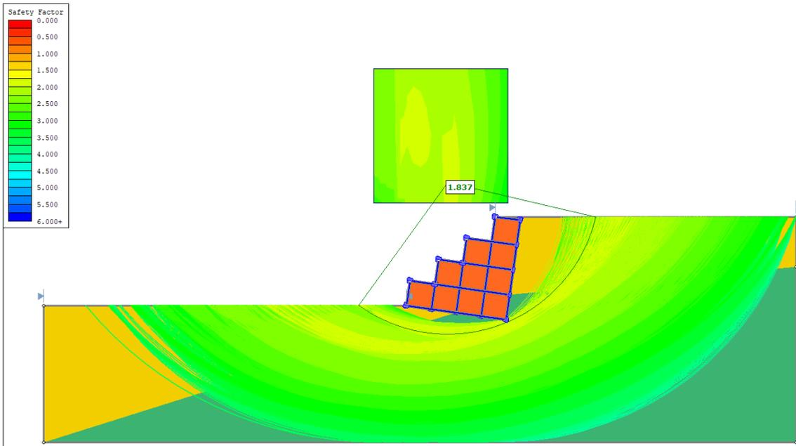
Figure 108.5: Solution for Mesh Method Using Circular Search and Bishop Method
