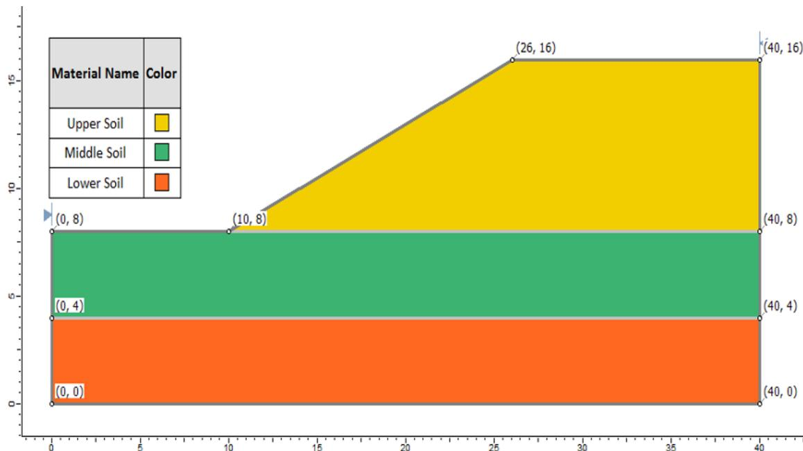
Figure 23.1: Geometry Setup in **Slide**
