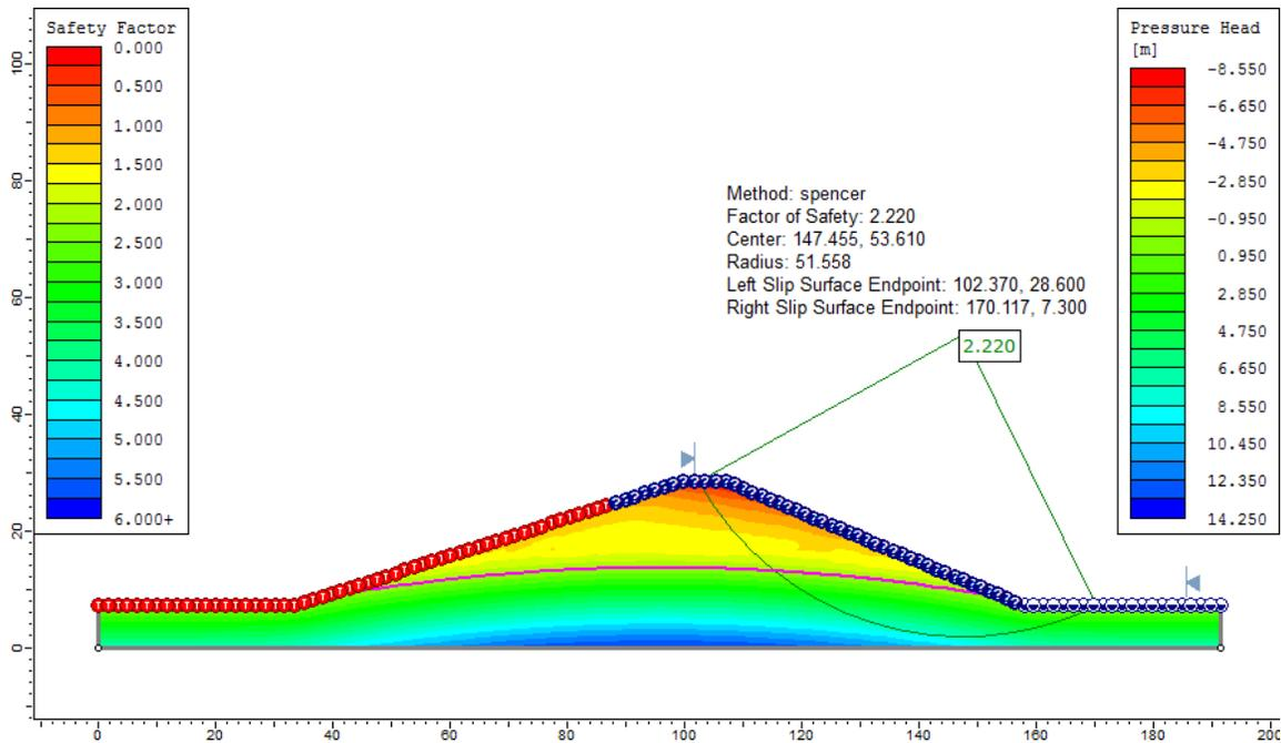
Figure 102.10: **Slide** Results for  $\phi^b = 37^\circ$  at 300 h, using the Spencer method
