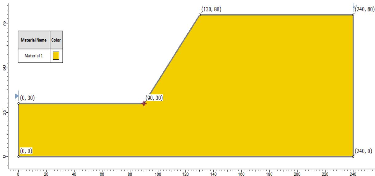
Figure 78.1: A Simple, Pure Cohesive Slope with a Foundation Thickness H
