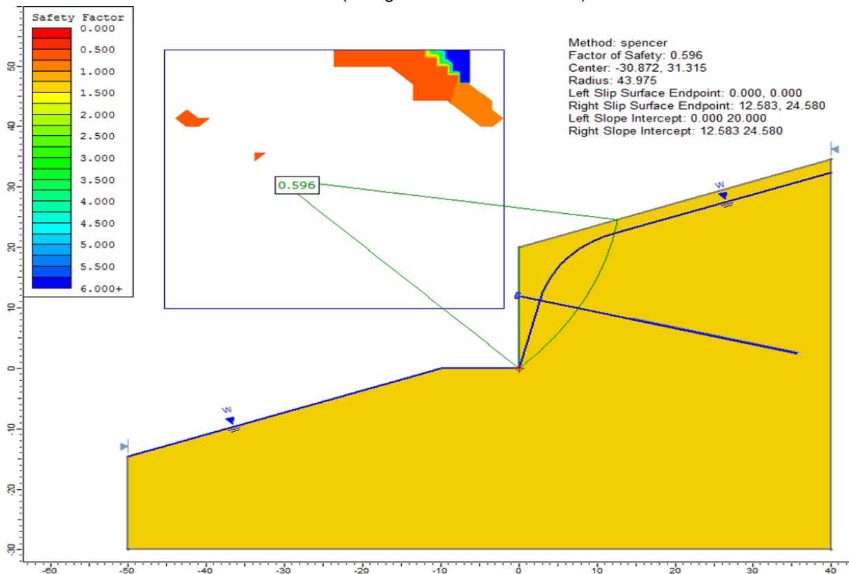
Figure 59.2: Critical failure surface, using the Spencer method
