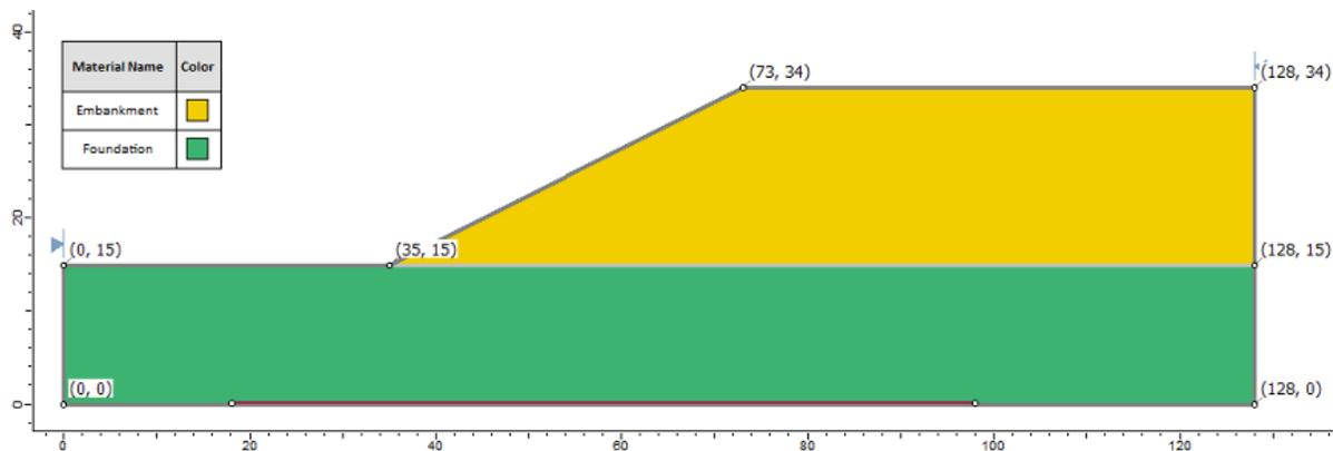
Figure 81.1: Geometry Setup in **Slide**
