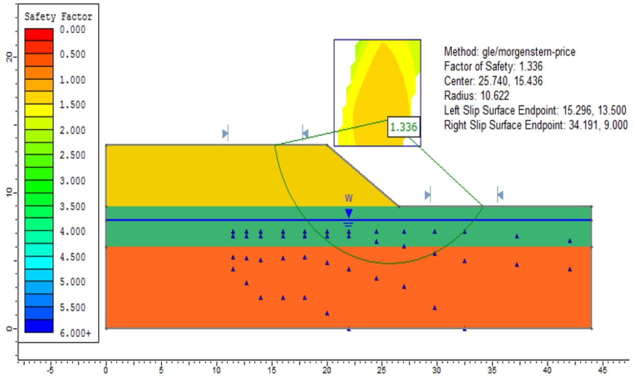
Figure 13.4: Solution, using the GLE method
