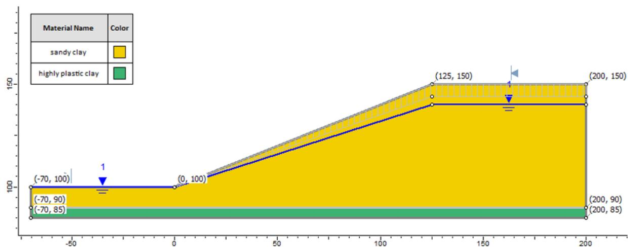
Figure 57.1: Geometry Setup in **Slide**
