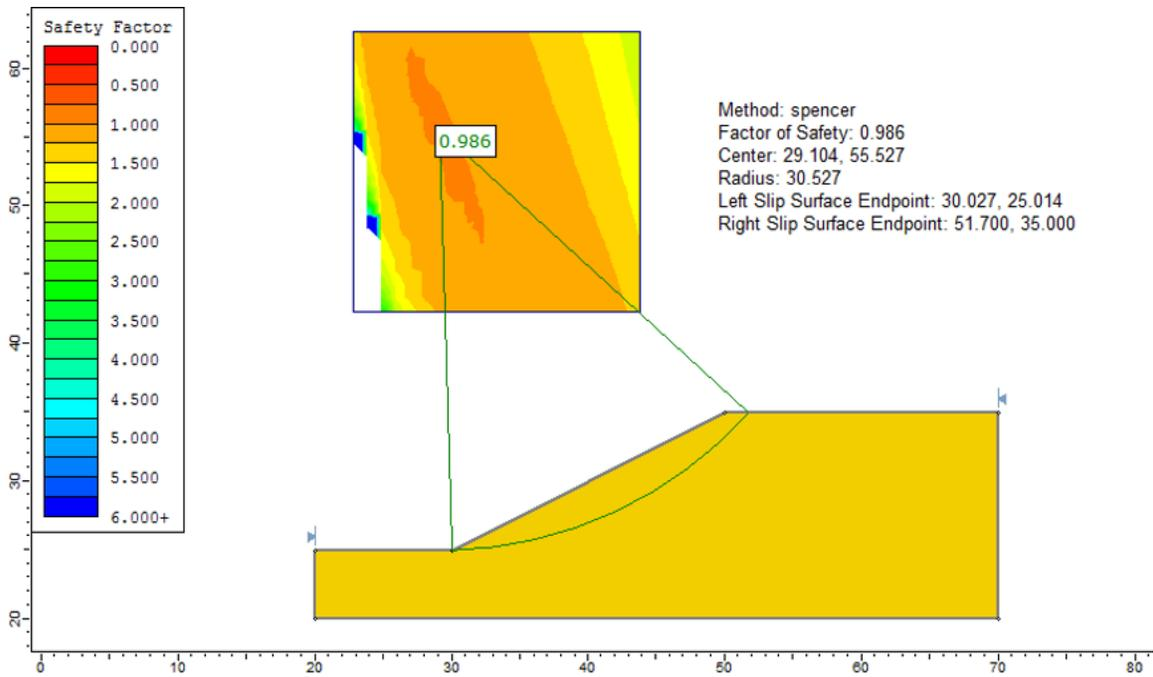
Figure 1.3: Solution, using the Spencer method
