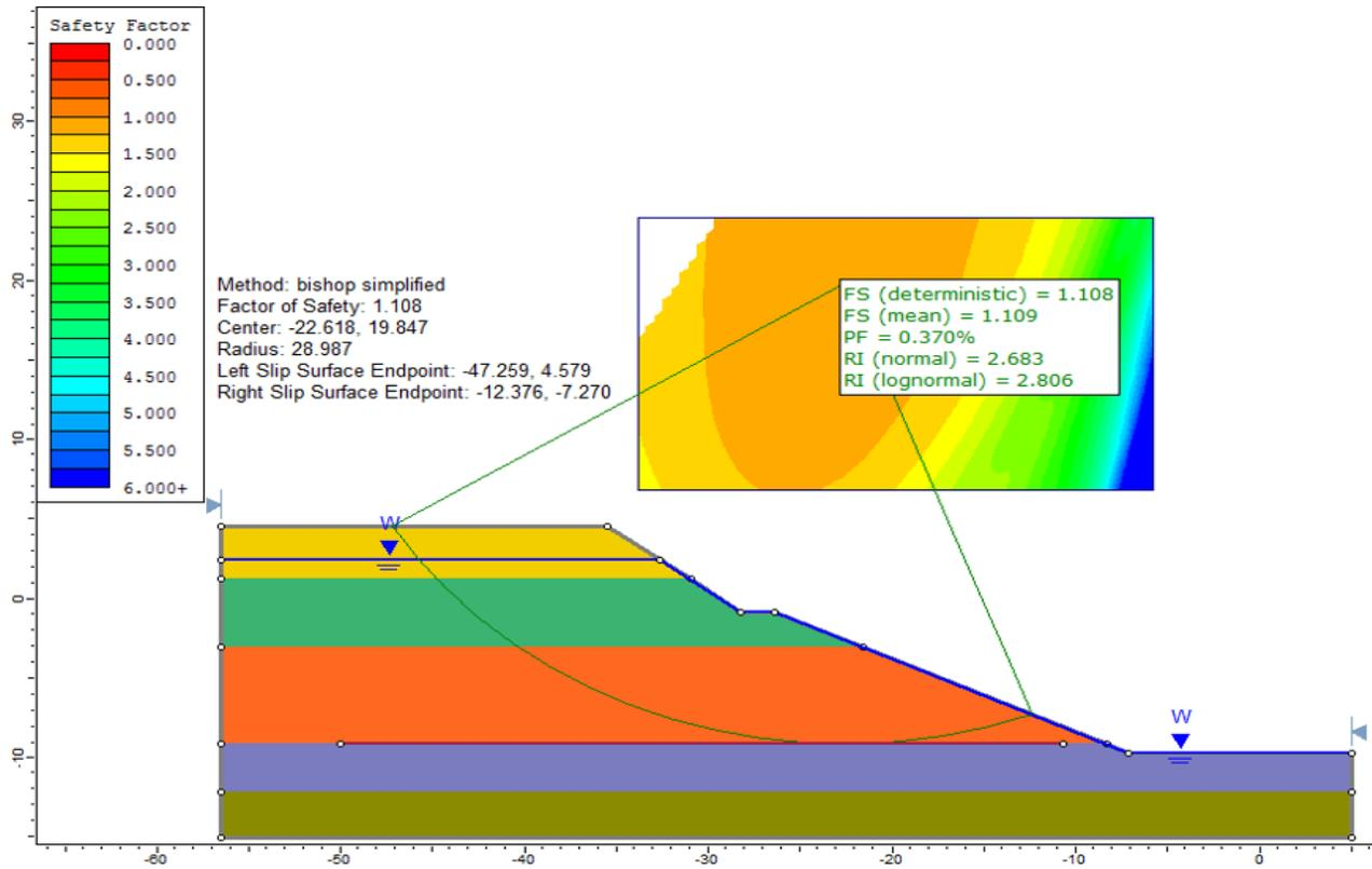
Figure 28.5: Critical slip circle tangential to lower boundary of clay layer
