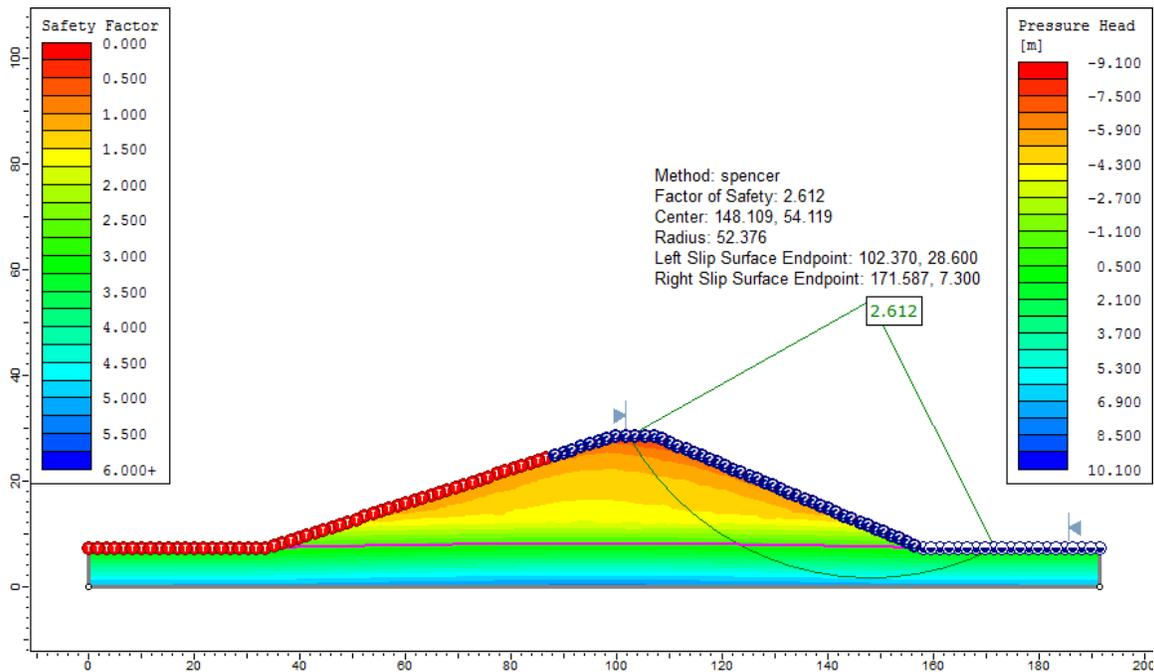
Figure 102.11: **Slide** Results for  $\phi^b = 37^\circ$  at 1500 h, using the Spencer method
