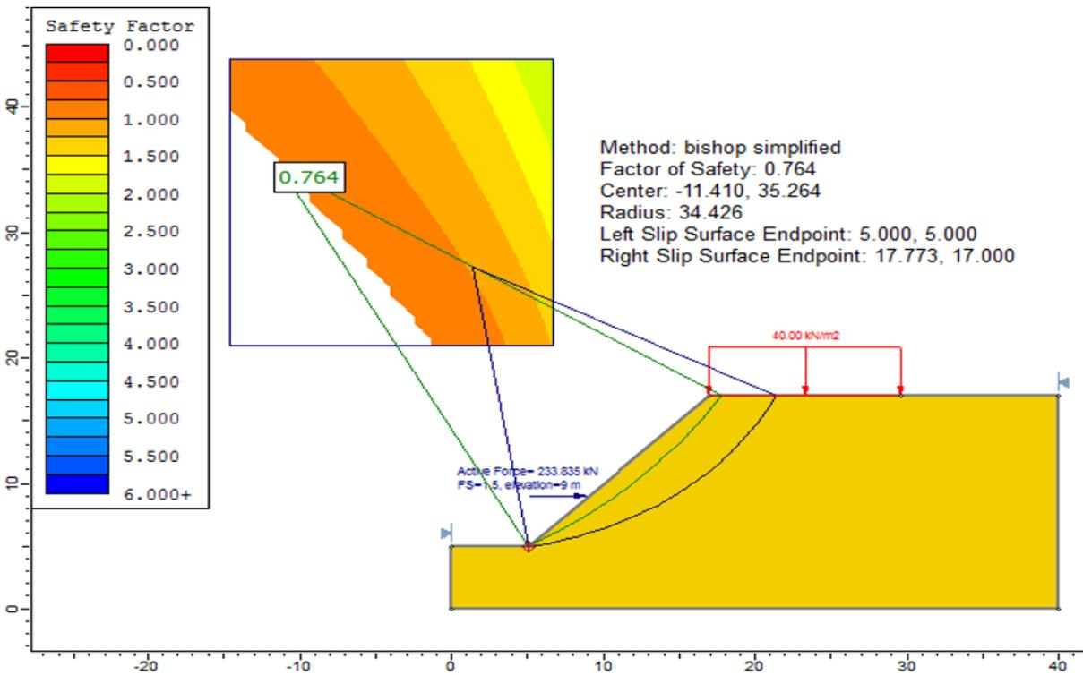
Figure 37.3: Critical Surface (back analysis)
