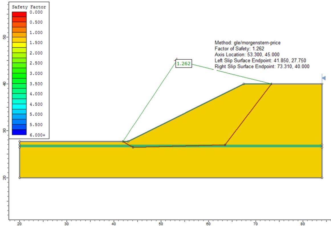
Figure 8.3: Solution, using the GLE method
