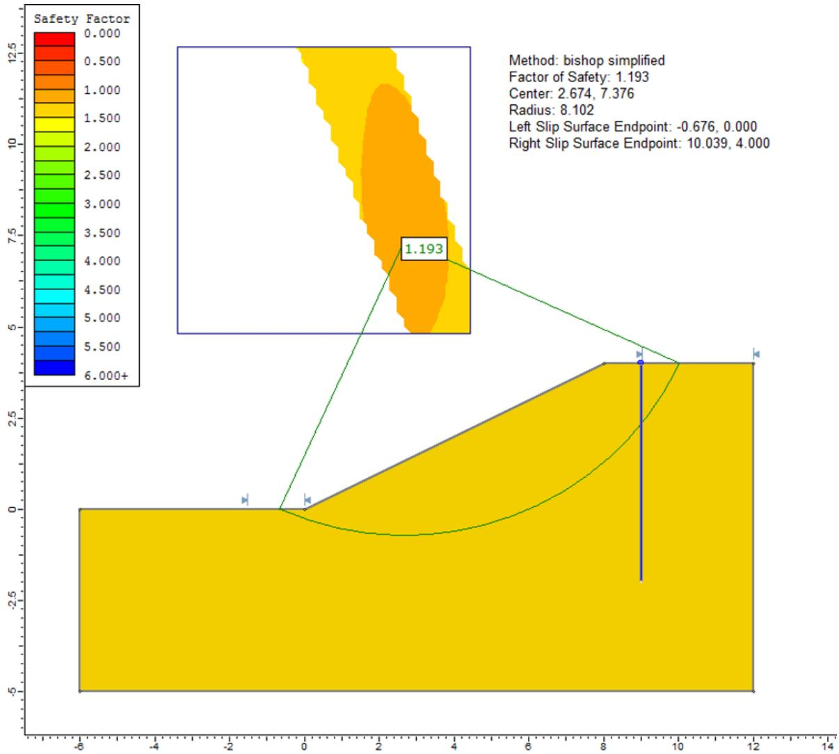
Figure 54.3: Circular failure surface, with reinforcing pile
