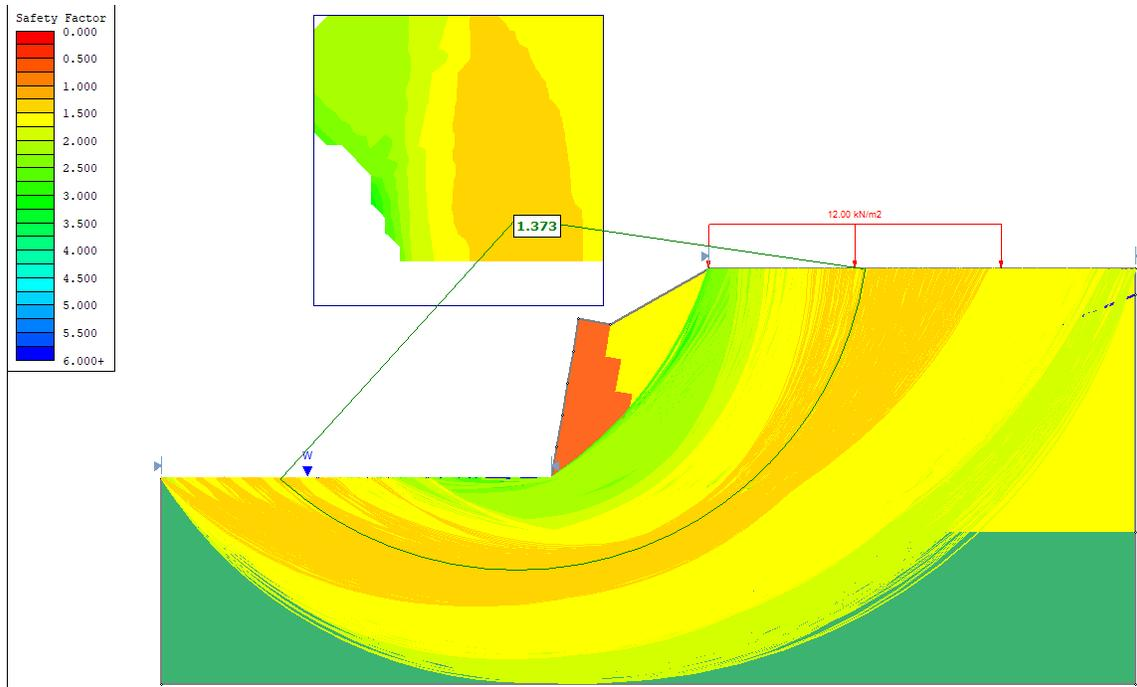
Figure 107.5: Solution for Equivalent Cohesion Method Using Circular Search and Bishop Method
