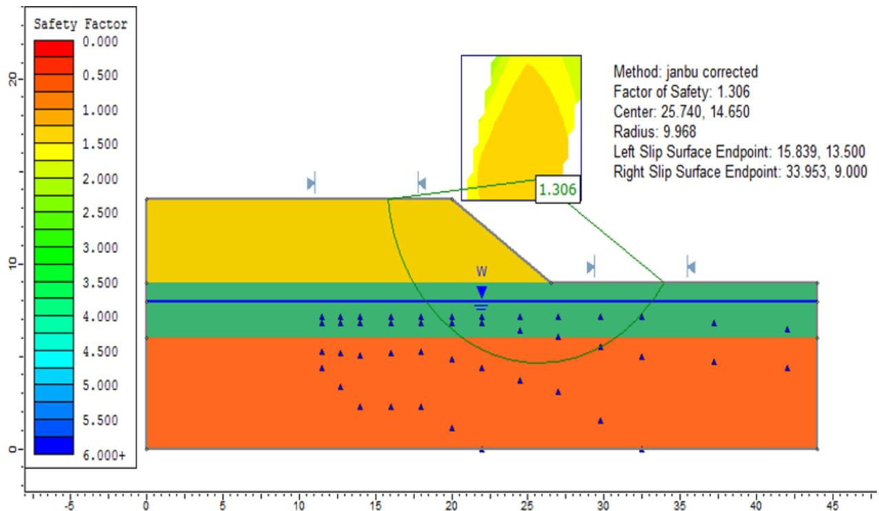
Figure 13.5: Solution, using the Janbu corrected method
