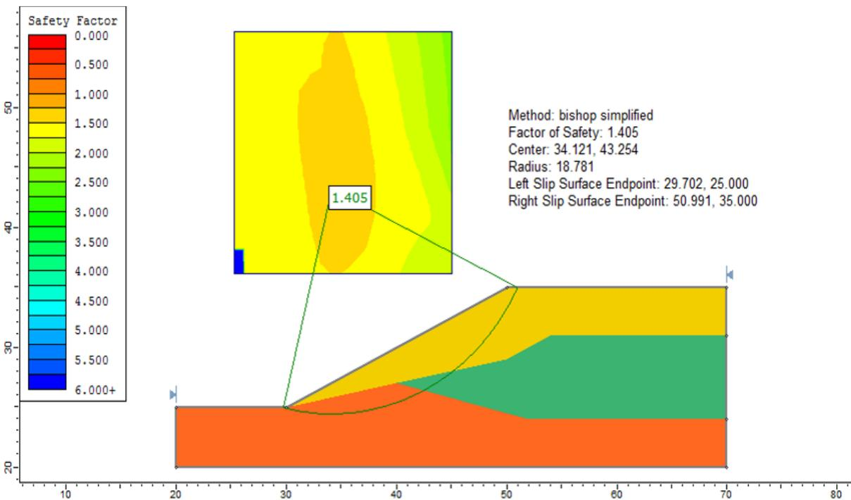
Figure 3.2: Solution, using the Bishop simplified method
