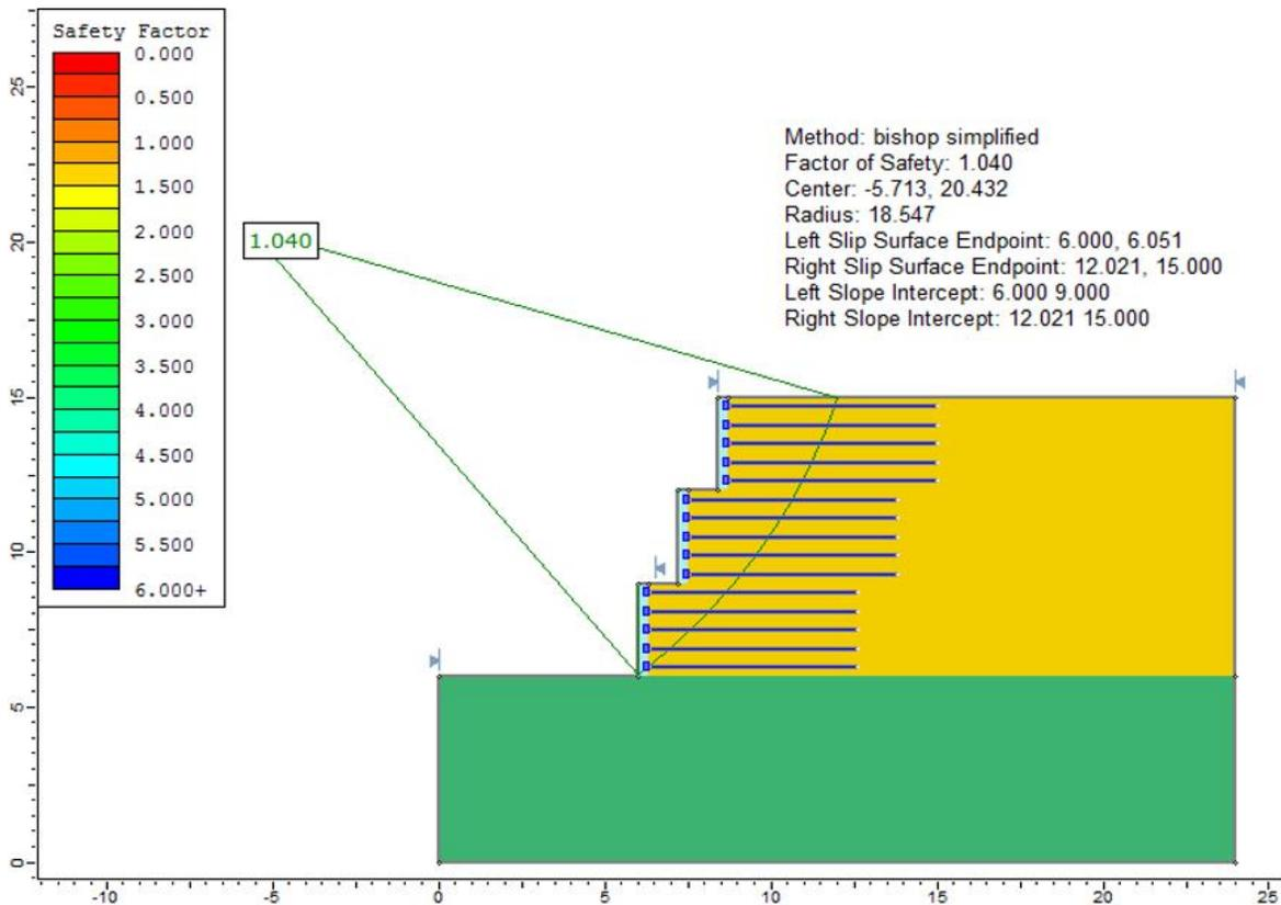
Figure 87.2: Solution, using the Bishop simplified method
