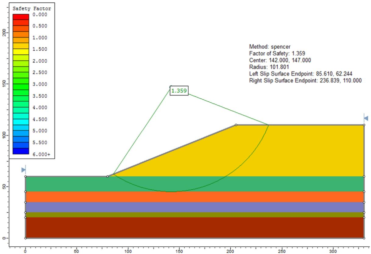
Figure 80.3: Solution to Case 2, using the Spencer method
