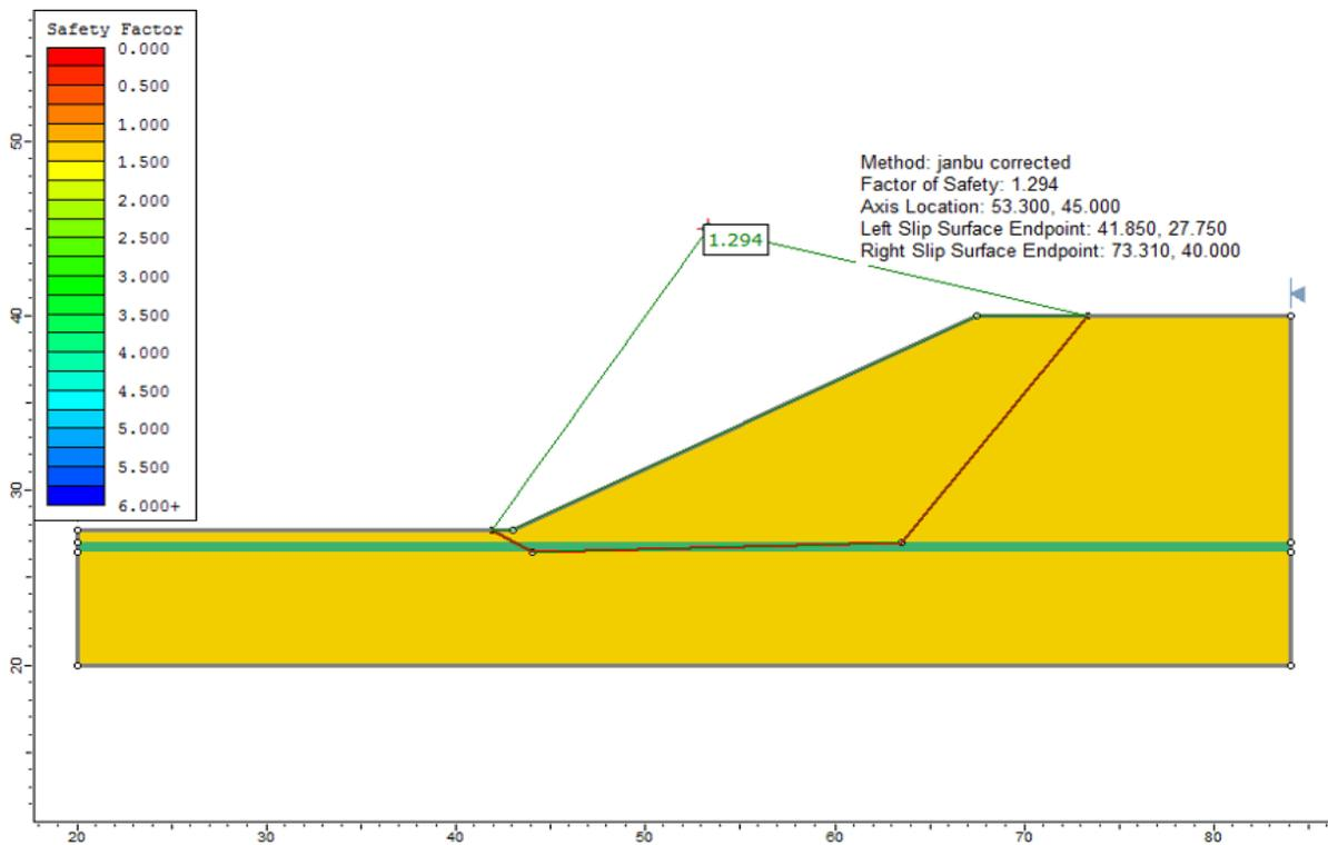
Figure 8.4: Solution, using the Janbu corrected method
