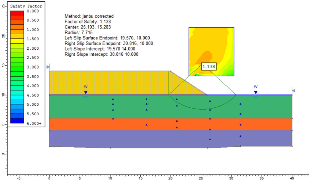
Figure 12.5: Solution, using the Janbu corrected method
