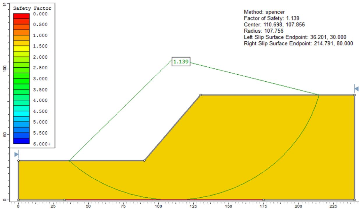
Figure 78.3: Solution to Case 1(b), using the Spencer method
