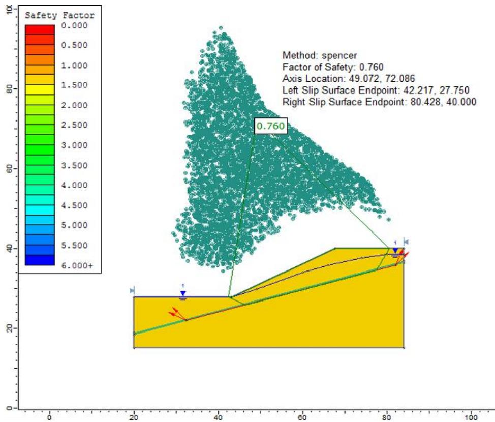
Figure 9.2: Solution, using the Spencer method
