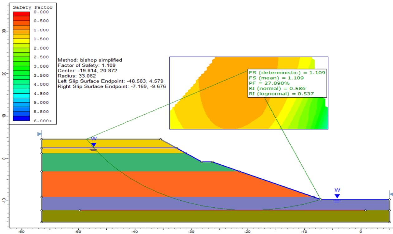
Figure 28.4: Critical slip circle tangential to lower boundary of clay layer 3
