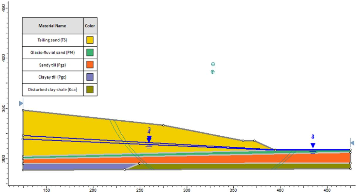
Figure 33.2: Geometry Setup in Slide
