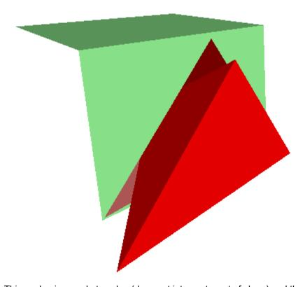
This wedge is a socket wedge (does not intersect crest of slope) and there is no tension crack.
