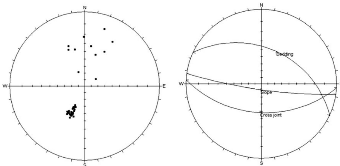
**Fig. 13** Stereonet diagrams of discontinuities and face slope of Galandroud mine rock mass
