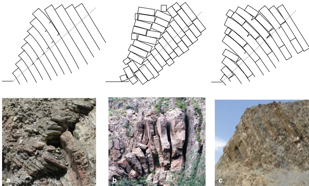
**Fig. 1** Possible main toppling failures in rock slopes. **a** Flexural. **b** Blocky. **c** Block-flexure
