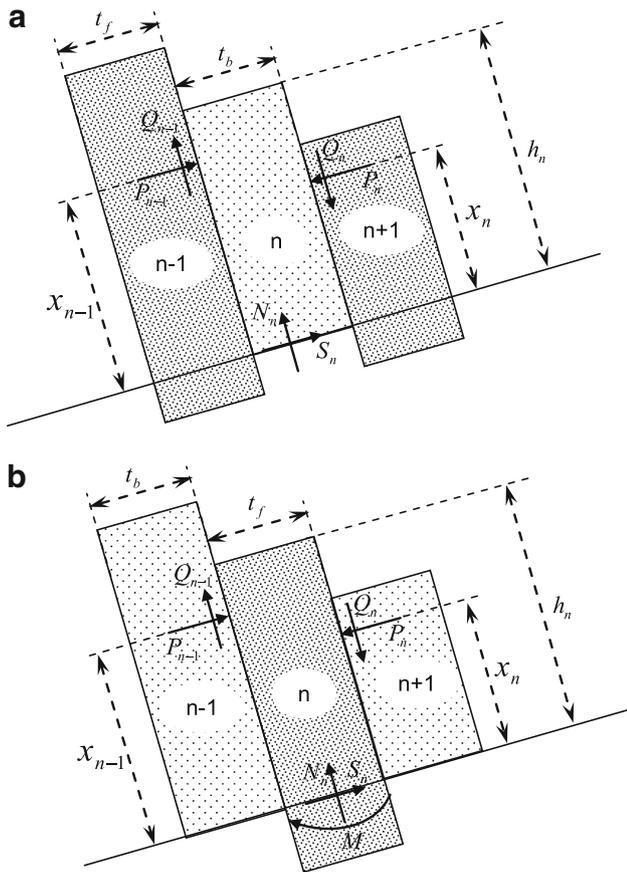
**Fig. 3** Two separate parts of a rock slope having the potential for block-flexure toppling failure
