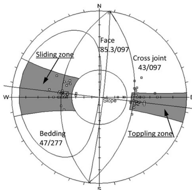
**Fig. 11** Kinematic stability analysis of the rock slope facing Chalus Road
