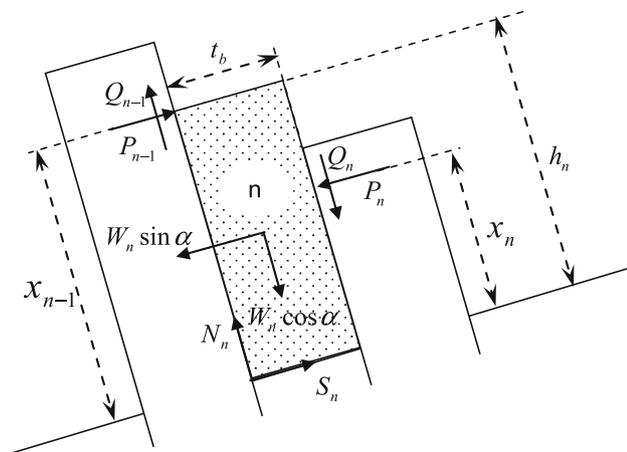
**Fig. 4** Analysis of three blocks having the potential for flexural and blocky toppling failures
