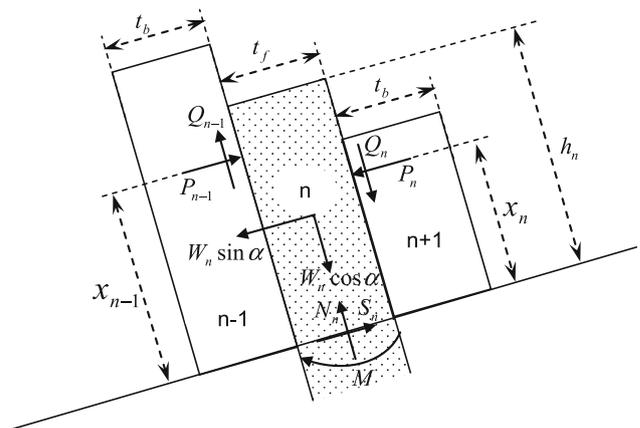
Fig. 7 Analysis of three blocks having potential for block-flexure toppling failures
