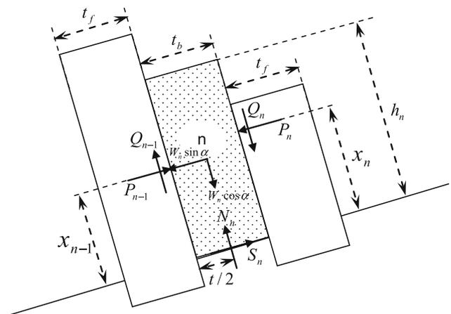
**Fig. 5** Analysis of three blocks having the potential for flexural toppling and sliding failures
