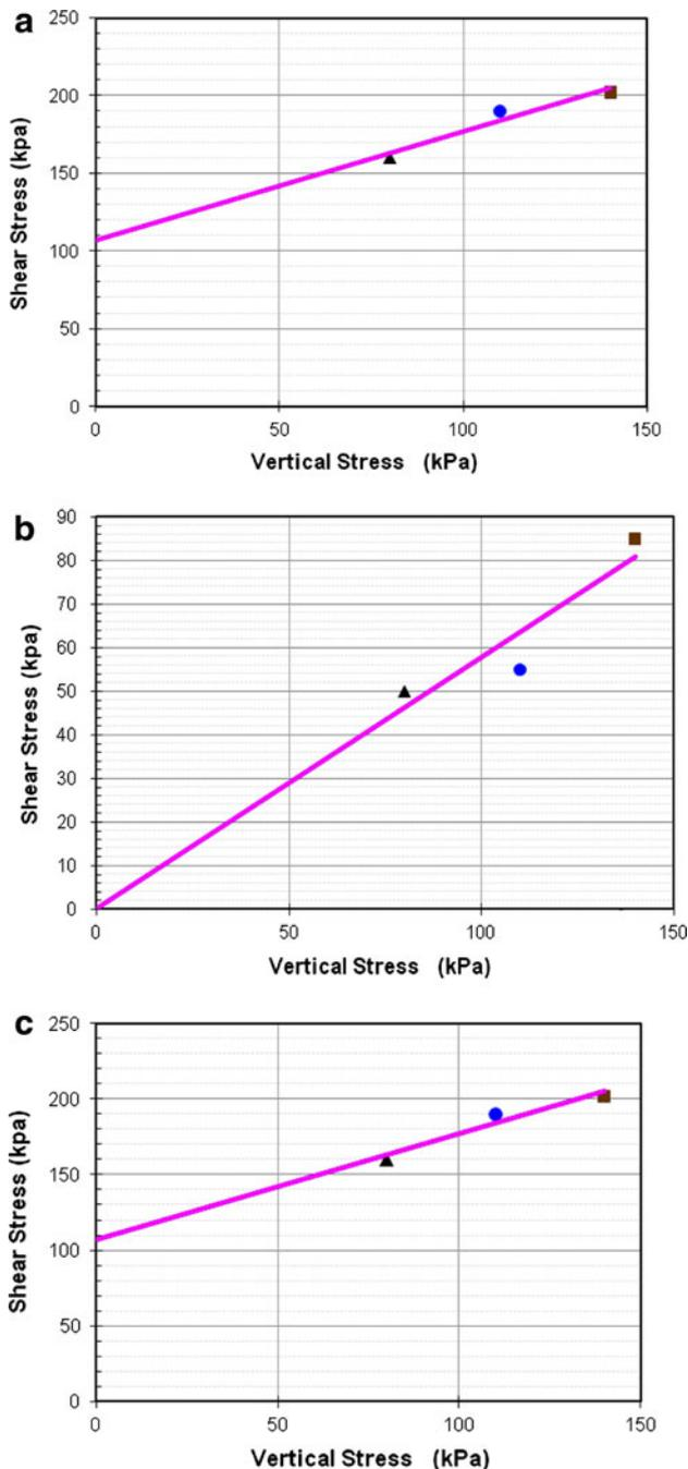
**Fig. 10** Direct shear test results of the samples taken from the rock mass facing Chalus Road. **a** Sandstone joints. **b** Shale. **c** Intact rock
