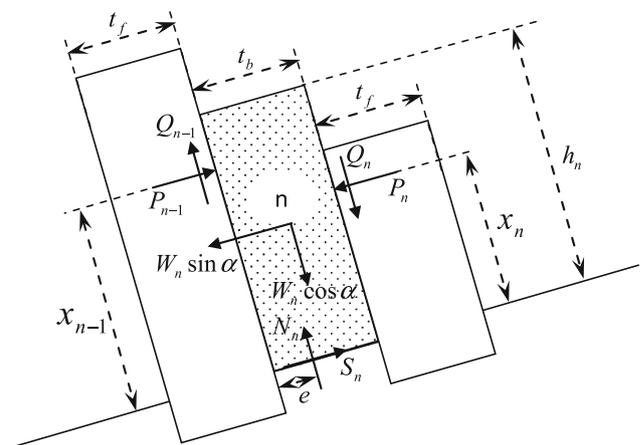
**Fig. 6** Analysis of three blocks having the potential for flexural toppling and blocky toppling-sliding failures
