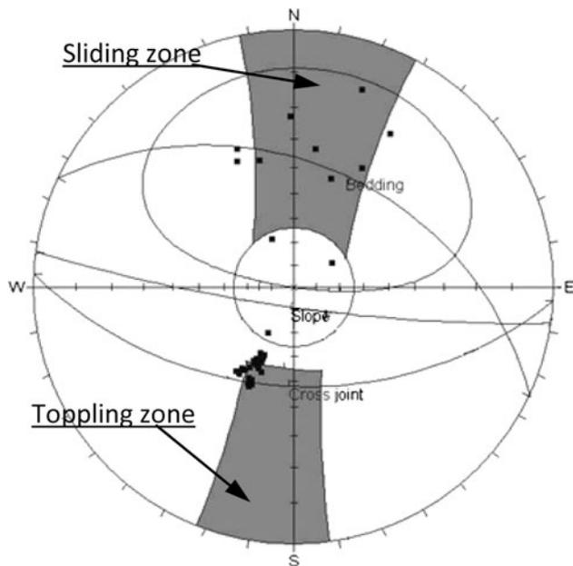
**Fig. 14** Kinematic stability analysis of the Galandrood mine slope
