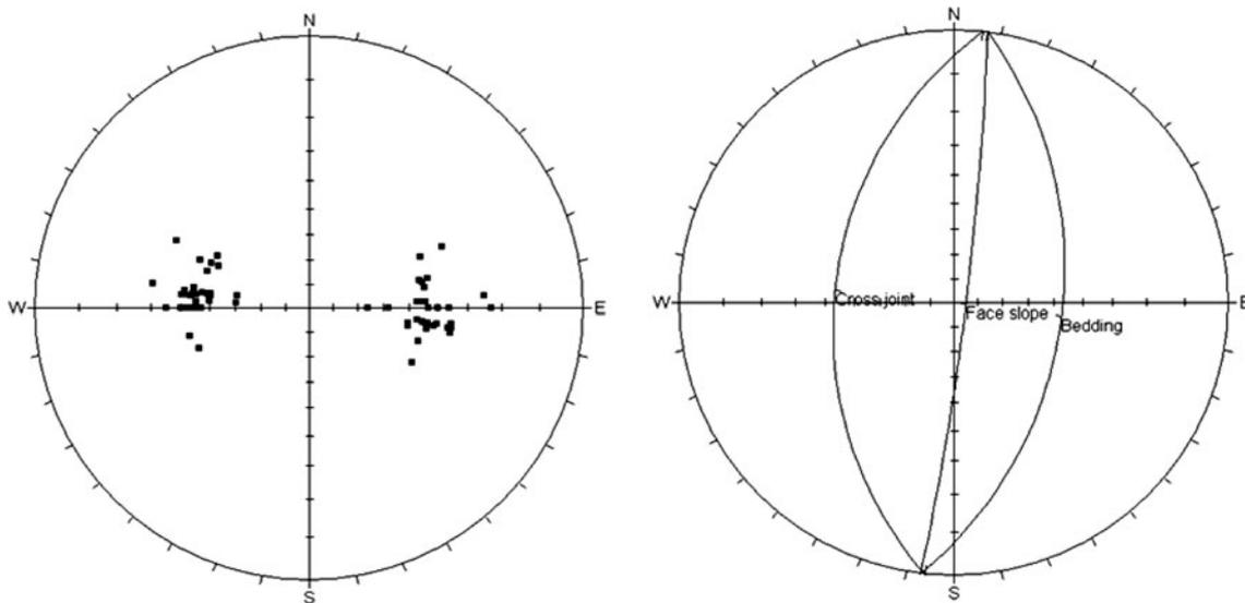
Fig. 9 Stereonet diagrams of discontinuities and face slope of the Chalus Road rock mass
