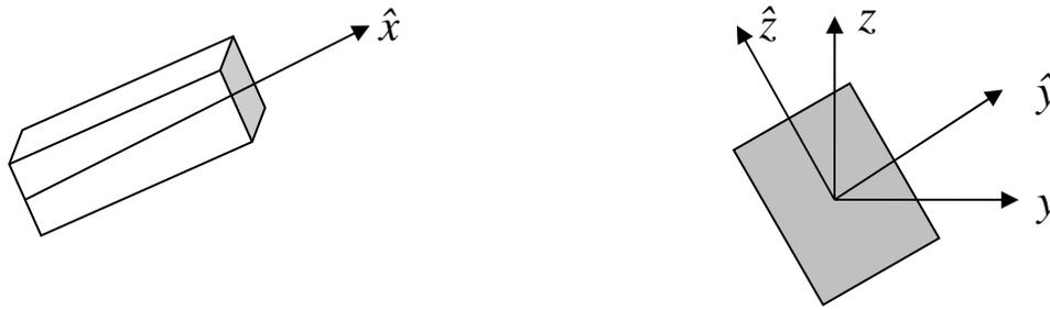
Figure 2 - Geometry of a 3D beam element.
