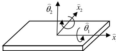
**Figure 5 - geometric representation of a plate component.**
