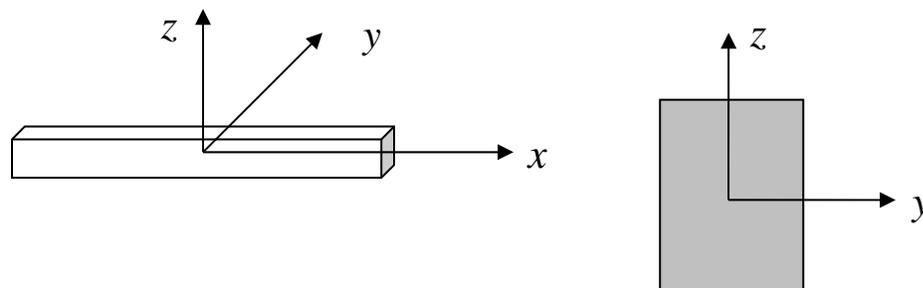
**Figure 1 - Geometry of a 3D beam element.**
