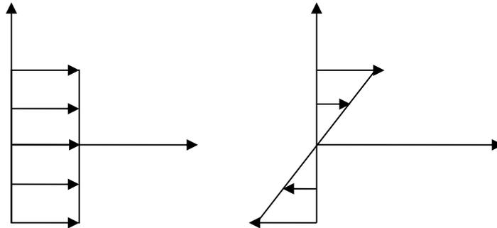
**Figure 6 - Distribution of axial stress distribution due to (a) membrane mechanism, (b) bending mechanism through the thickness of plate.**
