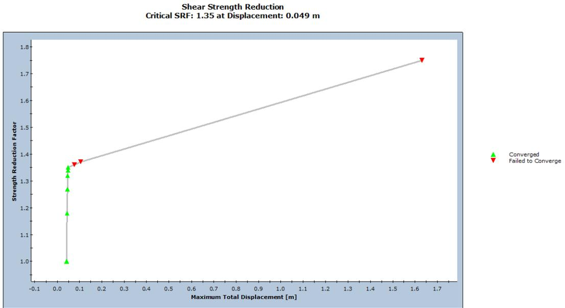
**Figure 3 – Graph of Shear Strength Reduction for Case 1**
