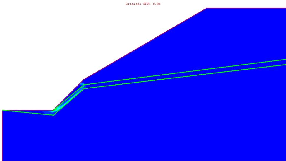
Figure 5 - Maximum Shear Strain Plot of Analysis I Case 2
