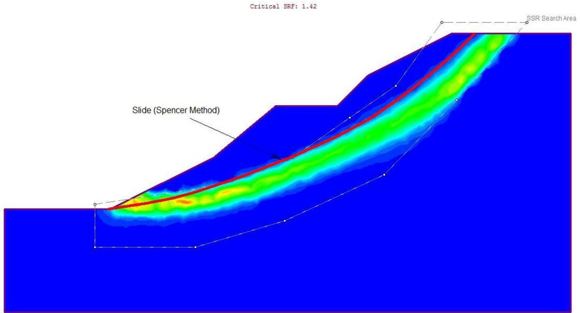
**Figure 5 – Maximum Shear Strain Plot of Case 3**
