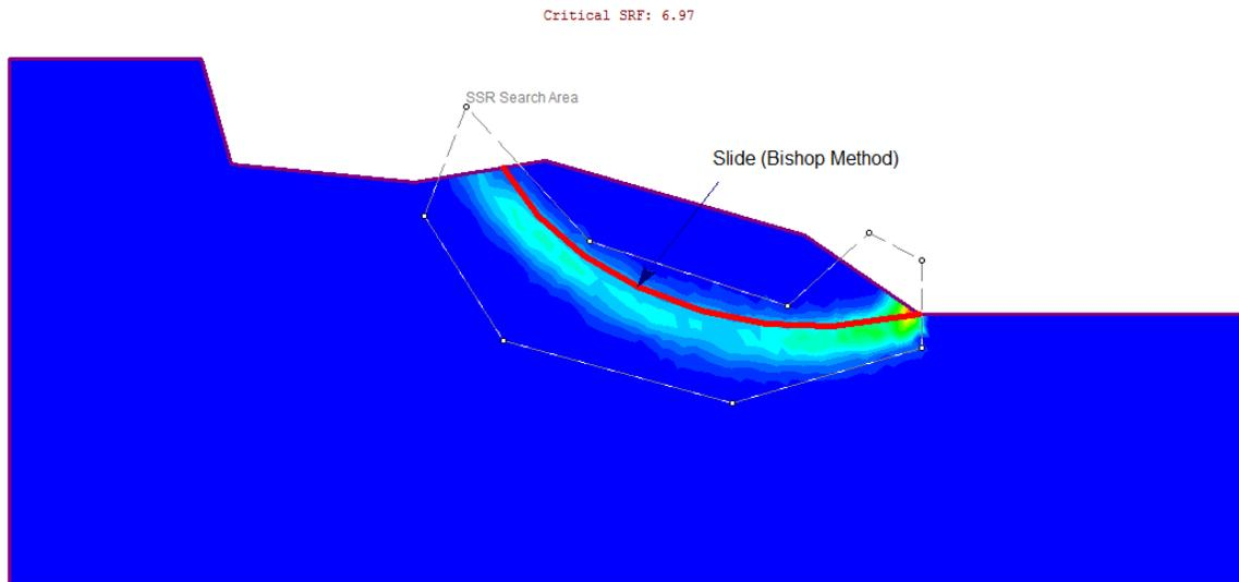
**Figure 10 – Maximum Shear Strain Plot of Case 6**
