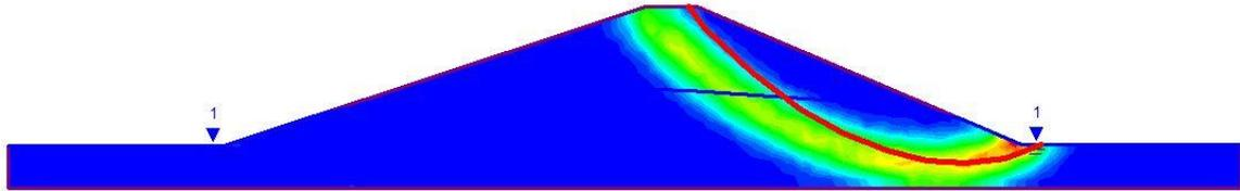
**Figure 4 - Dam (downstream) with free surface 90 h after rapid drawdown**
