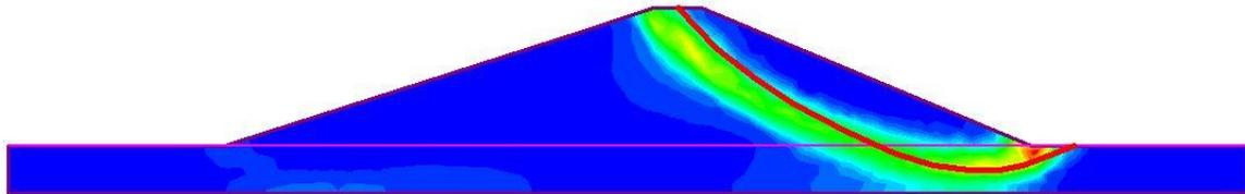
**Figure 6 - Dam (downstream) with free surface 1500 h after rapid drawdown**
