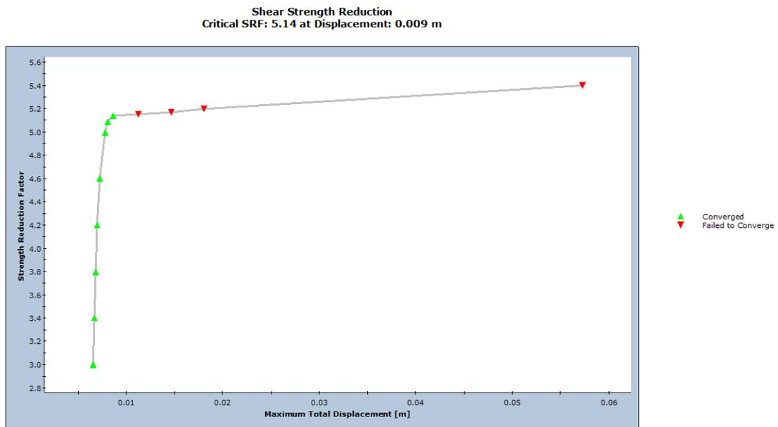
**Figure 5 – Graph of Shear Strength Reduction for Case 1**
