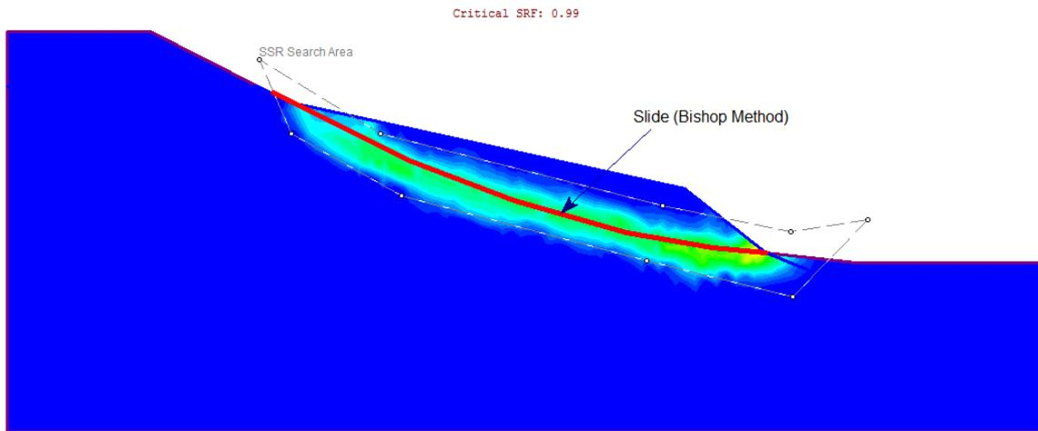
**Figure 13 – Maximum Shear Strain Plot of Case 8**
