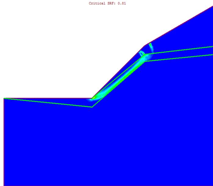
Figure 12 - Maximum Shear Strain Plot of Analysis III Case 1
