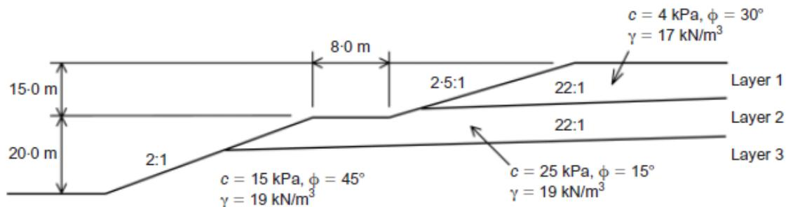
Figure 2 - Non-homogeneous slope geometry
