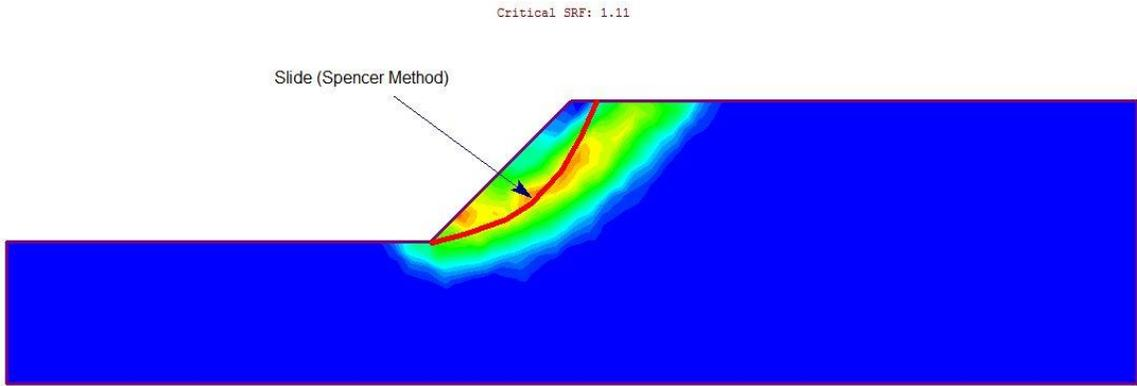
**Figure 6 – Maximum Shear Strain Plot of Case 3**
