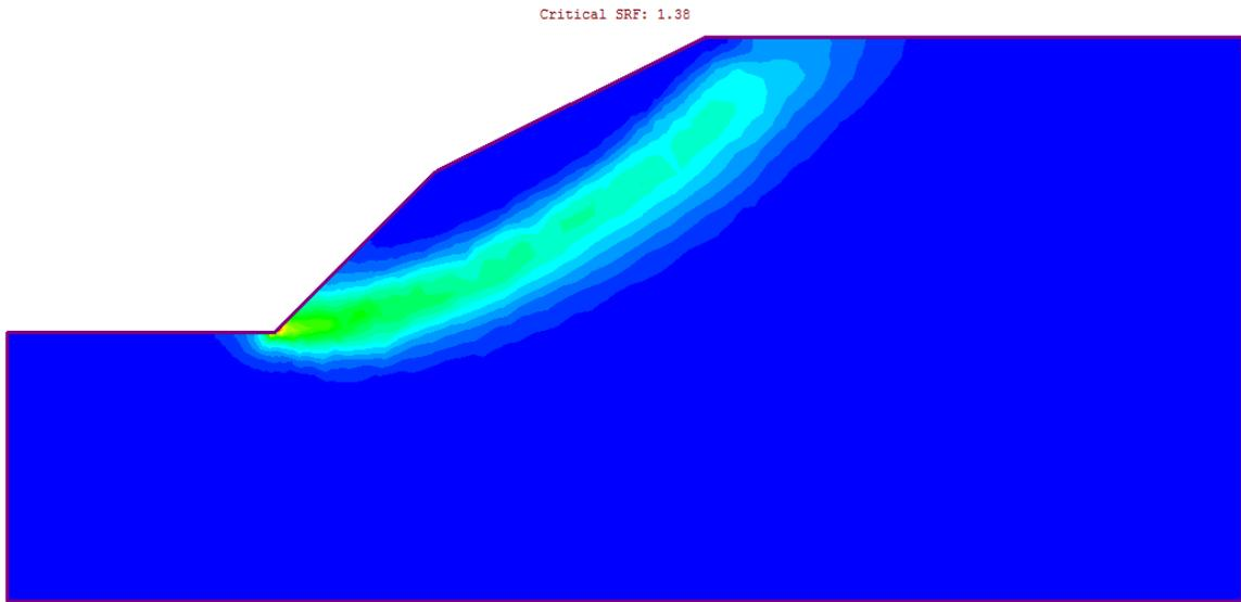
**Figure 2 – Maximum Shear Strain Plot of Case 1**
