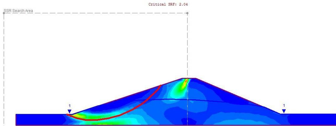
**Figure 5 - Dam (upstream) with free surface 90 h after rapid drawdown**
