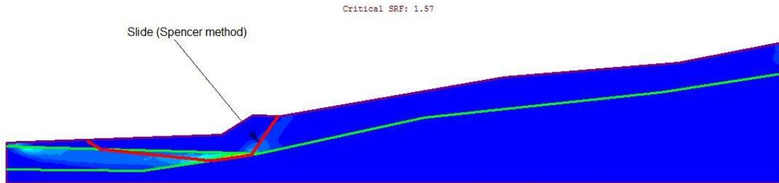
**Figure 2 - Maximum Shear Strain Plot of Case 1**
