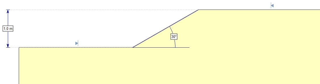
**Figure 2 - Case 2, Geometry  $\beta = 30^\circ$**
