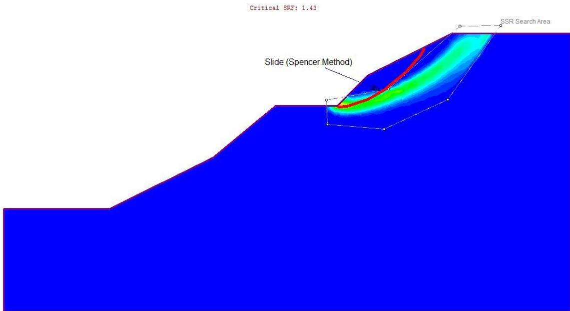
**Figure 6 – Maximum Shear Strain Plot of Case 4**
