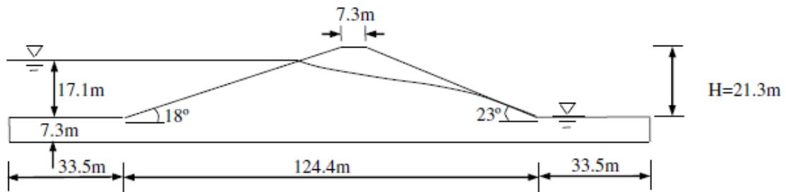
**Figure 1 - Dam Geometry**
