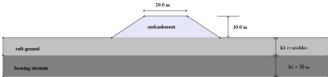
Figure 1 - Embankment geometry
