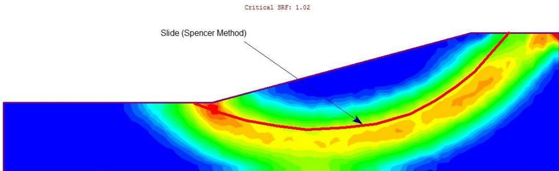
**Figure 4 – Maximum Shear Strain Plot of Case 1**
