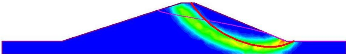
**Figure 3 - Dam (downstream) with steady free surface (steady seepage)**
