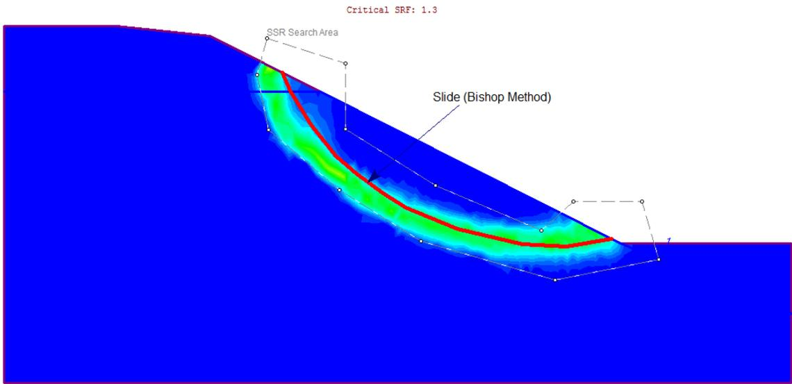
**Figure 14 – Maximum Shear Strain Plot of Case 9**
