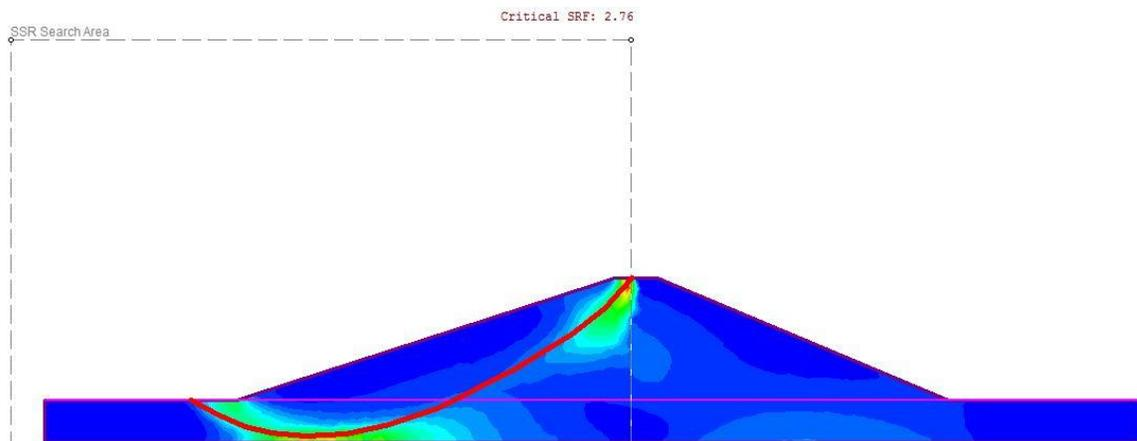
**Figure 7 - Dam (upstream) with free surface 1500 h after rapid drawdown**
