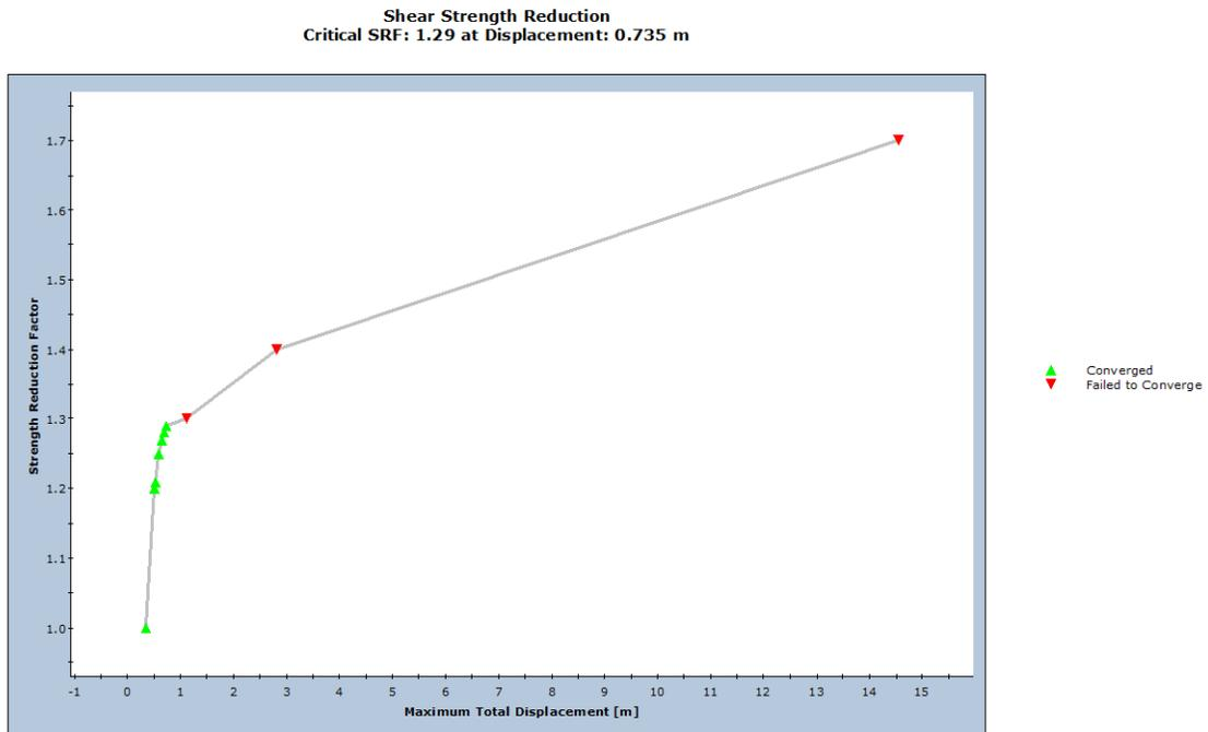
**Figure 3 – Graph of Shear Strength Reduction**
