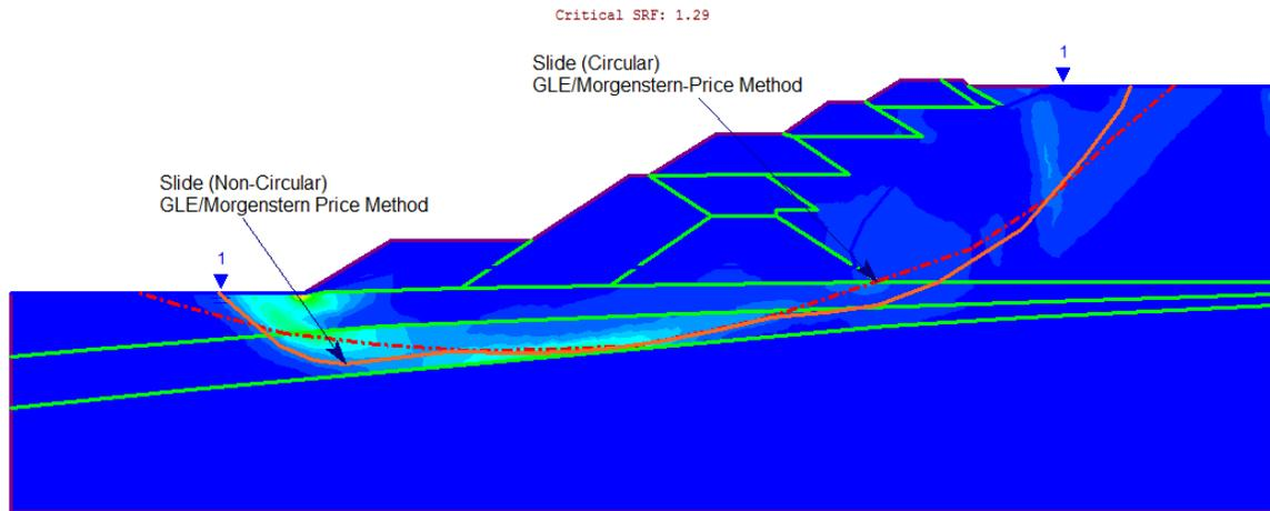
**Figure 2 – Maximum Shear Strain Plot**
