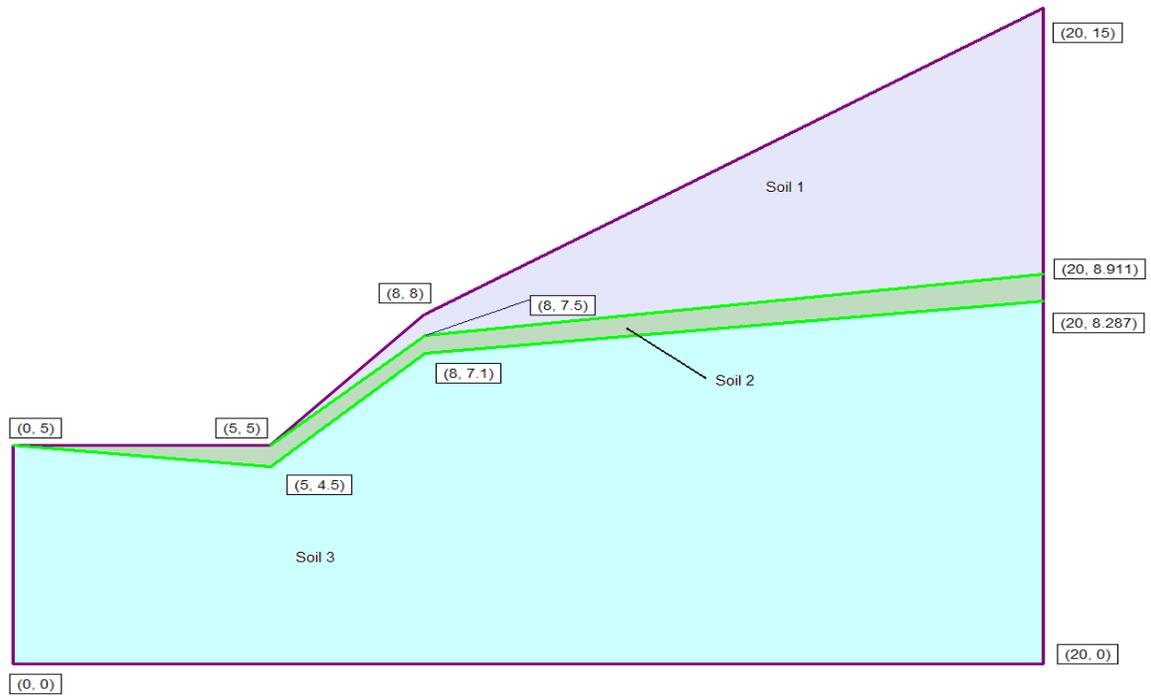
**Figure 2 - Geometry II (20 m Domain)**
