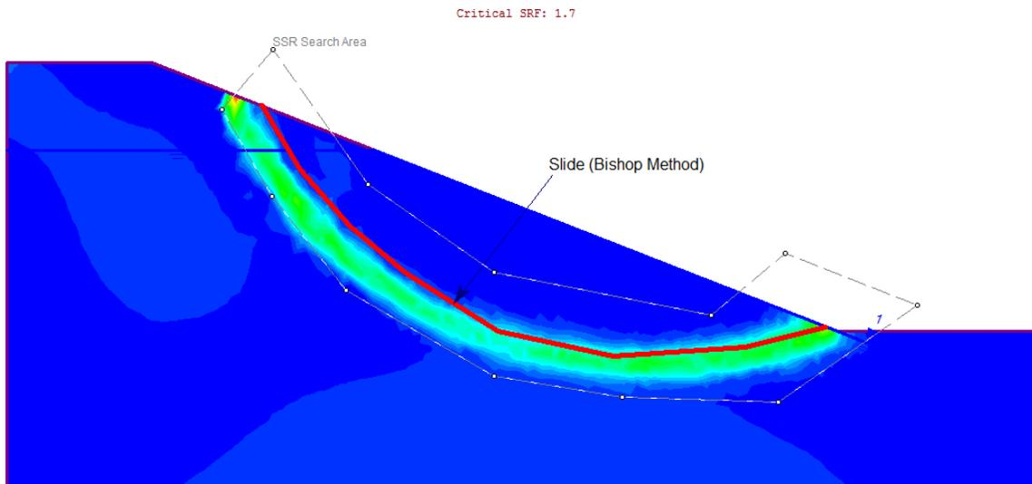
**Figure 11 – Maximum Shear Strain Plot of Case 7**
