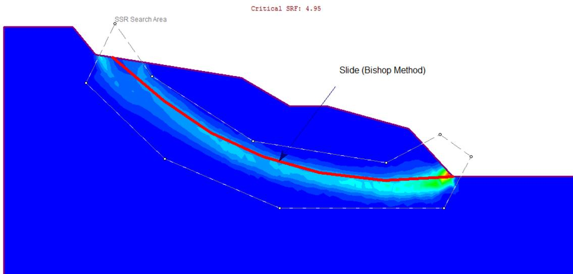
**Figure 8 – Maximum Shear Strain Plot of Case 4**
