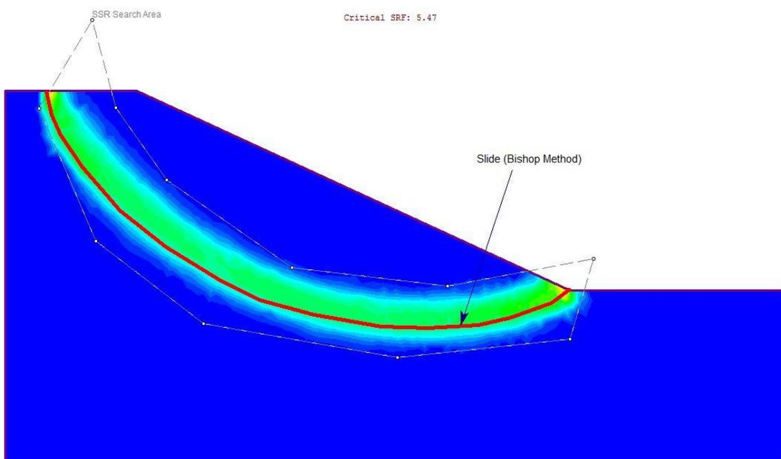
**Figure 9 – Maximum Shear Strain Plot of Case 5**
