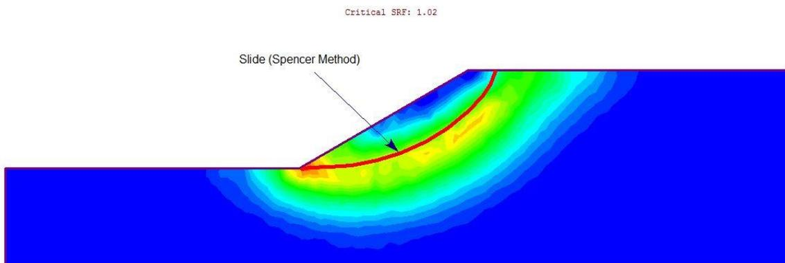
**Figure 5 – Maximum Shear Strain Plot of Case 2**
