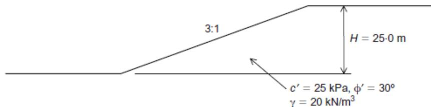
Figure 1 - Homogeneous slope geometry
