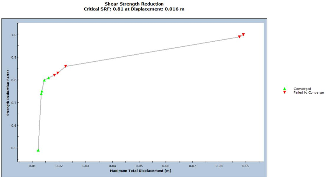
**Figure 14 - SSR Convergence Graph of Analysis III Case 1**
