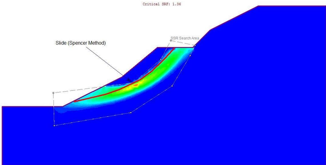
**Figure 4 – Maximum Shear Strain Plot of Case 2**
