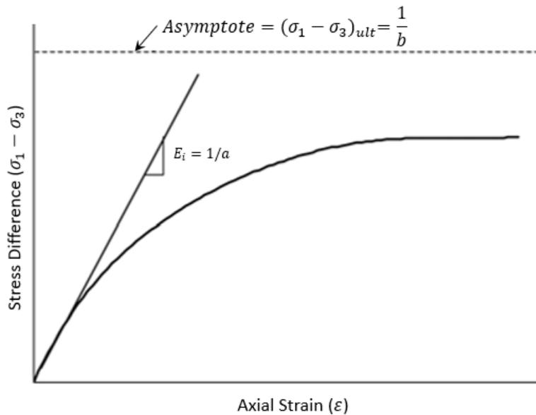
Figure 7.0. Hyperbolic stress-strain curve
