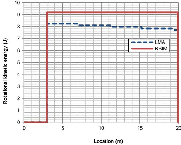
Figure 6. Rotational kinetic energy versus rock path location.
