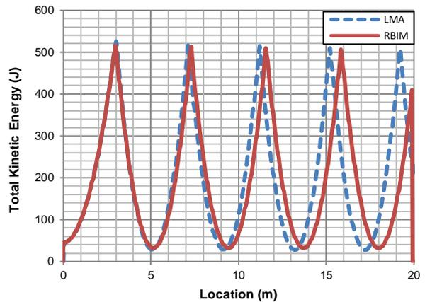
Figure 5. Total kinetic energy versus rock path location.
