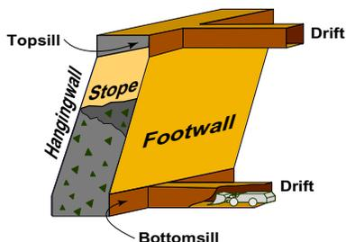
Figure 1: Illustration of a typical bulk-mining stope
