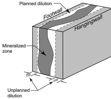
Figure 4: Illustration of planned and unplanned dilution.
