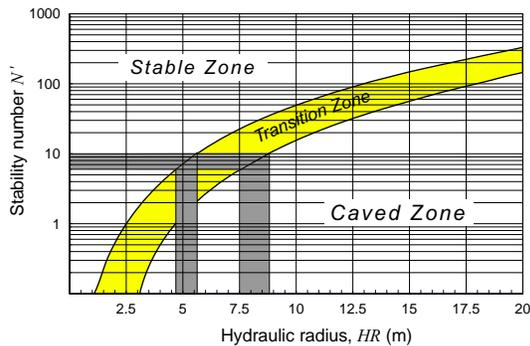
Figure 5: Stability graph showing the zones of stable ground and caving ground, i.e., dilution.
