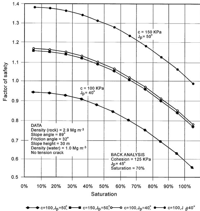
Fig. 11. Sensitivity analysis for planar failure (relationship between factor of safety on the one hand and rock mass saturation, cohesion,  $c$ , and joint angle,  $j_p$  on the other). The term saturation refers to the height of the water table in the slope as a percentage of the slope height. For example, 100% saturation indicates a water table that is at the surface.
