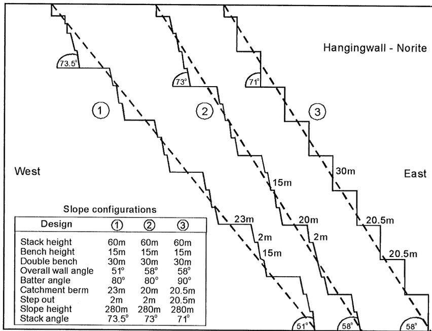
Fig. 19. Stack configuration for the hangingwall.
