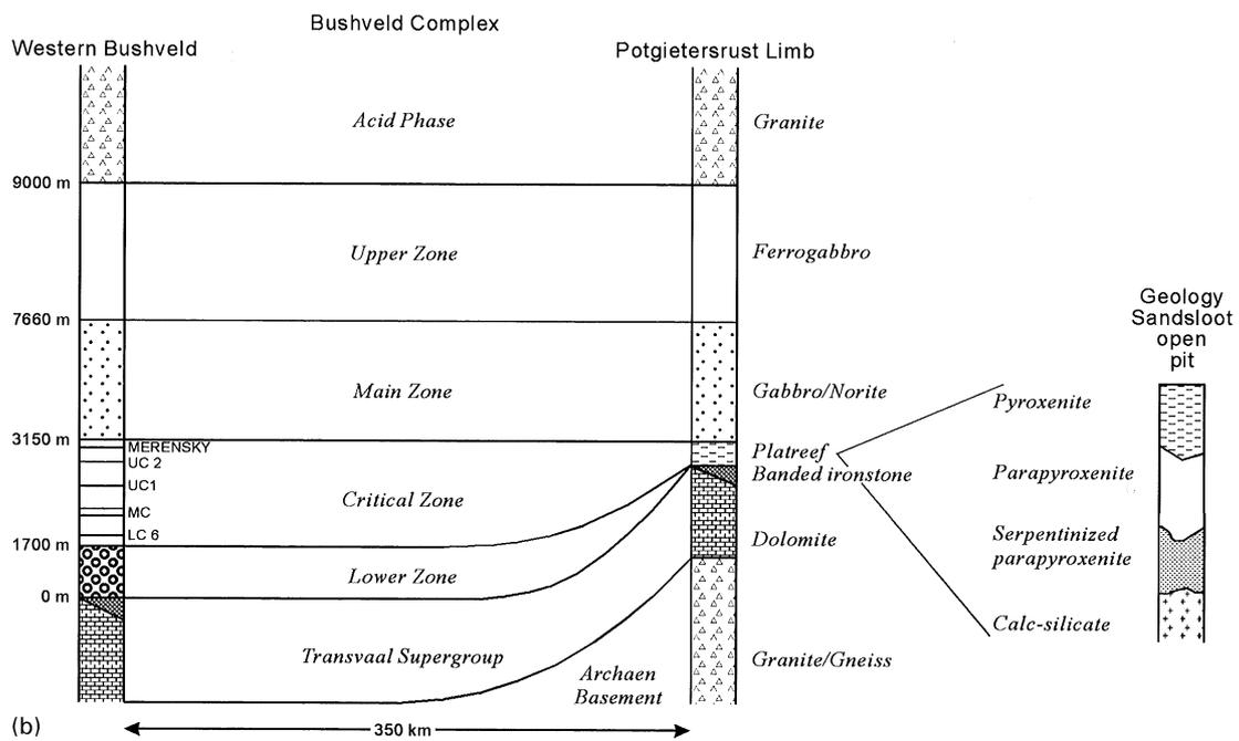
Fig. 3. (a) Geology of the Sandsloot locality. (b) Order of stratigraphic occurrence of the rocks in the Sandsloot locality.
