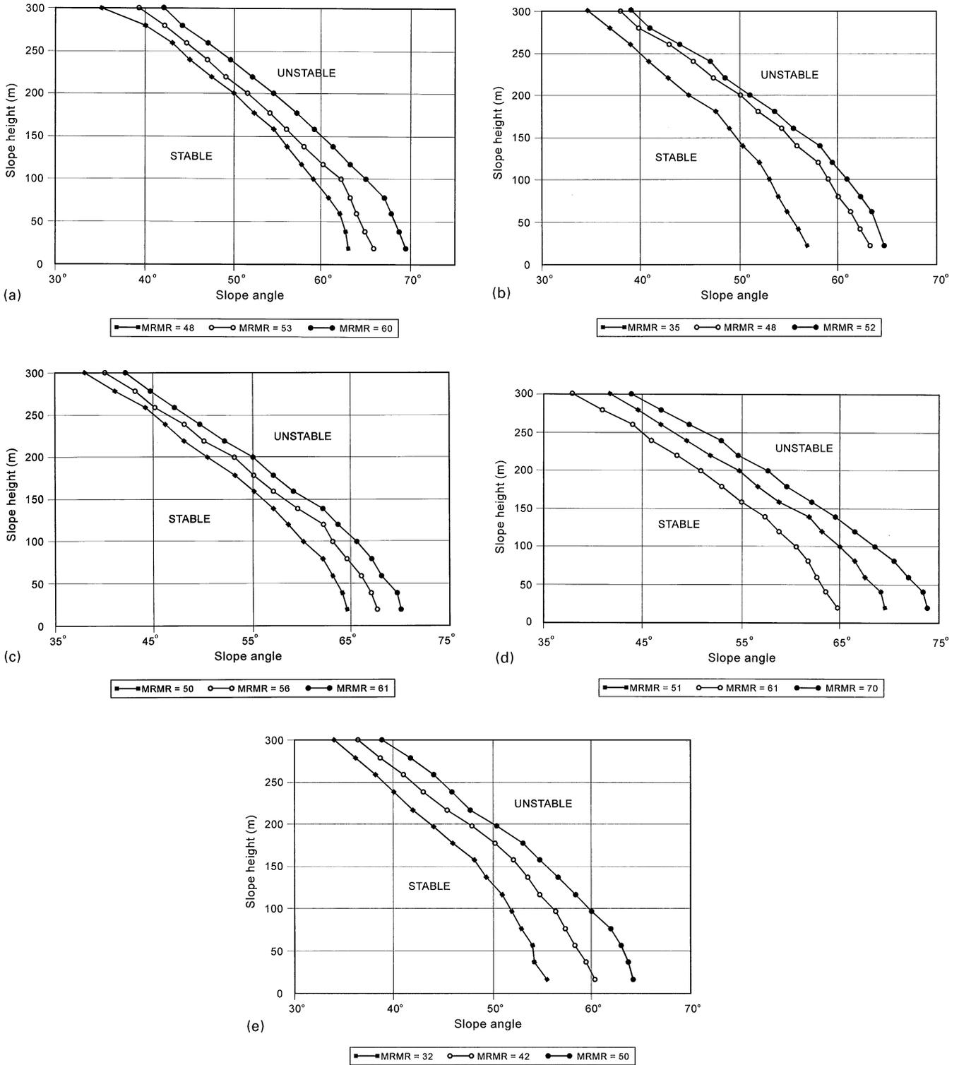
Fig. 21. Range of slope design based on MRMR, slope height and slope angle for (a) norite, (b) pyroxenite, (c) parapyroxenite, (d) serpentinized pyroxenite and (e) calc-silicate.
