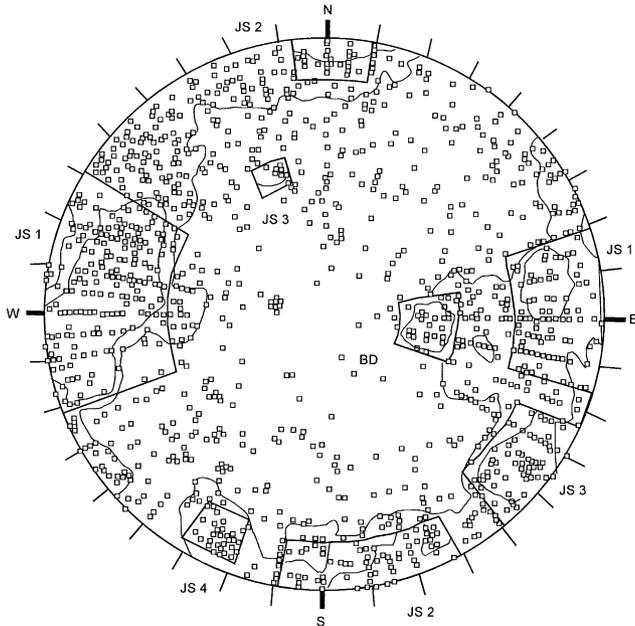
Fig. 6. Stereonet showing the families of joint sets at Sandsloot open pit.
