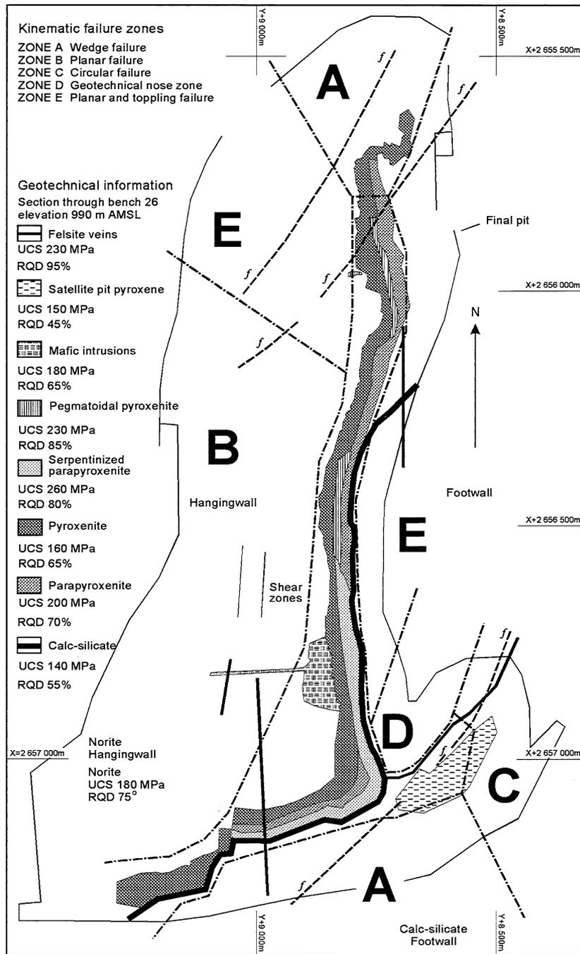
Fig. 8. Failure zones identified at Sandsloot of pit.
