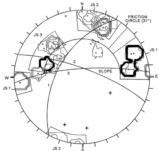
Fig. 13. Stereonet indicating potential wedge failure. Joints 1 and 2 intersect within the friction circle (joint intersection dip angle > friction dip angle) and will daylight within the slope face, resulting in a high probability of wedge failure.
