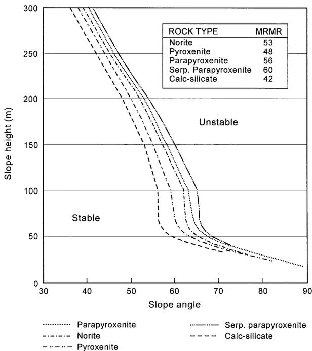
Fig. 20. An example of a slope design chart for rock types at Sandsloot.
