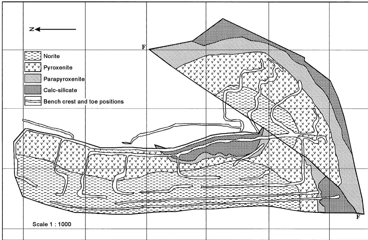
Fig. 4. Plan view showing the geology of Sandsloot open pit. The double lines reflect the crest and toe positions of the active mining benches.
