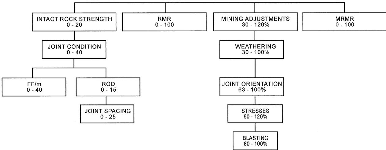
Fig. 16. Flow diagram illustrating the MRMR system of Laubscher [8].
