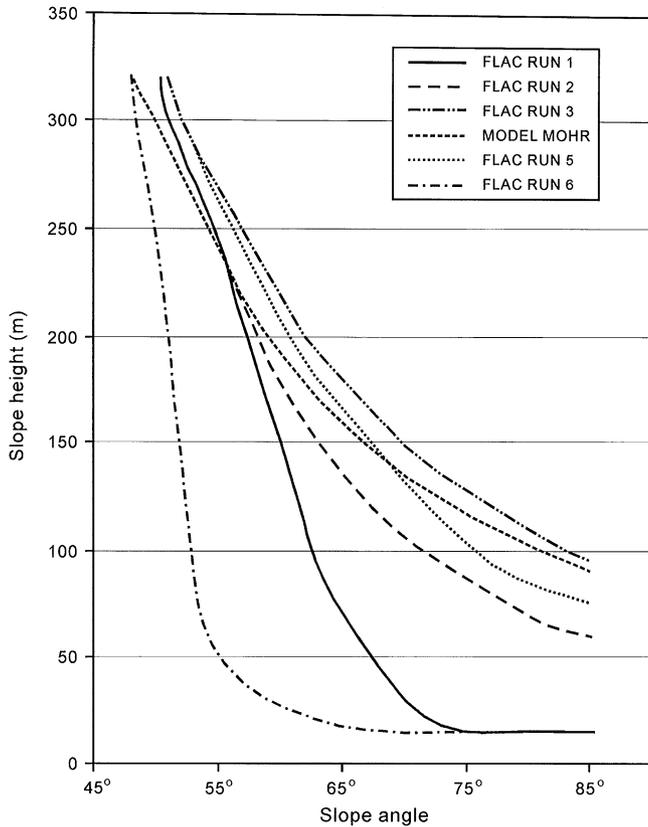
Fig. 18. Stability envelopes for norite of the hangingwall developed by FLAC analyses.
