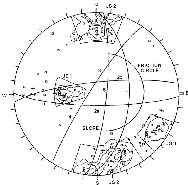
Fig. 10. Stereonet depicting plane failure on the western highwall.
