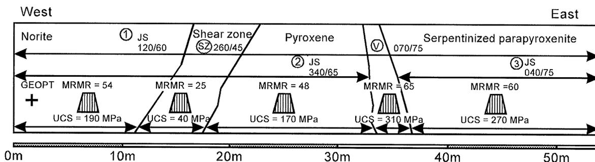
Fig. 17. An example of a geotechnical face map.
