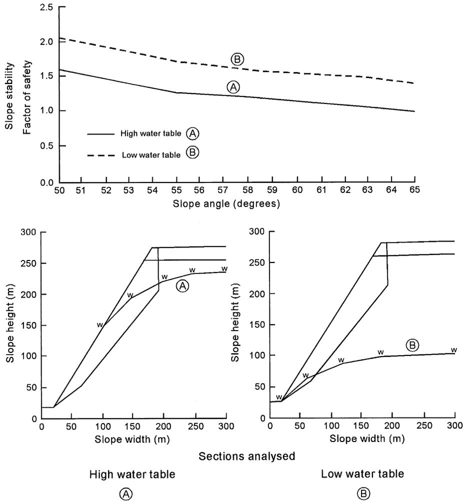
Fig. 5. The effect of dry and wet conditions on the factor of safety of the design of slopes. Line A indicates a lower FOS/less stable slope than line B, for an equivalent slope height and angle, due to the higher level of the water table within the slope. For example a dry slope at 50° will have a FOIS of 2.1 while a wet slope will have a lower FOS of 1.6.
