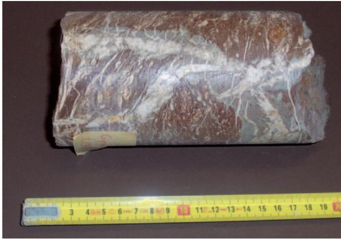
Fig. 1. Core with slickensides in anhydrite-bearing claystone (gypsum keuper) from a boring in western side wall of the Hauenstein Base Tunnel (1988)
