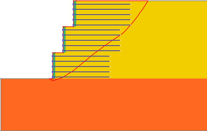
**Figure 2. Deterministic critical composite failure surface with  $F_s = 1.28$ .**
