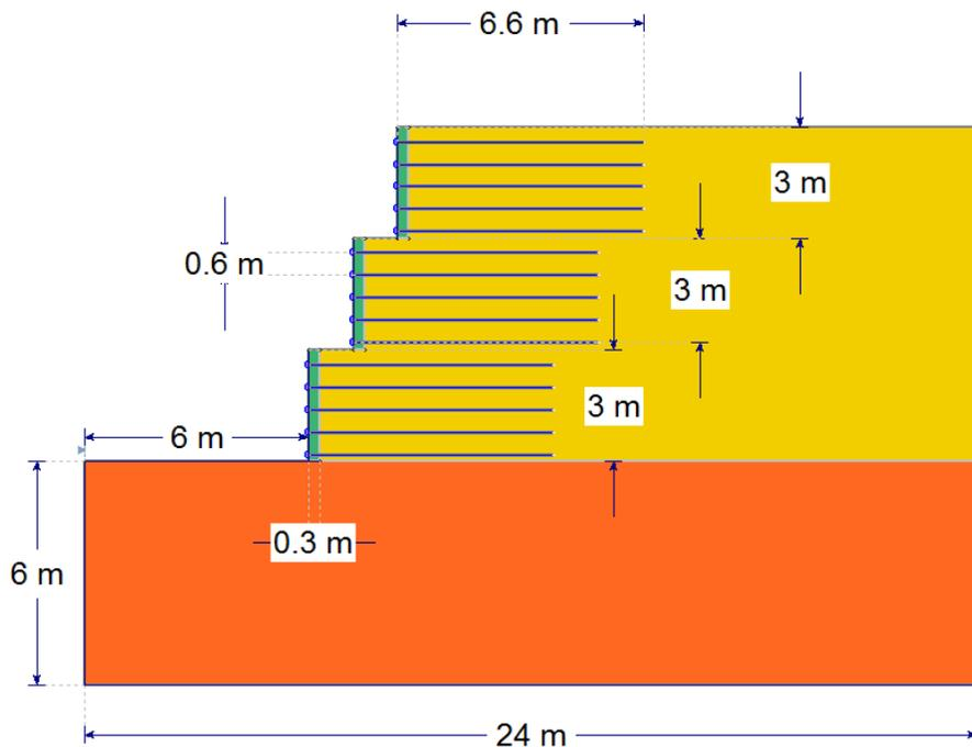
**Figure 1. Geosynthetic reinforced MSE wall model.**
