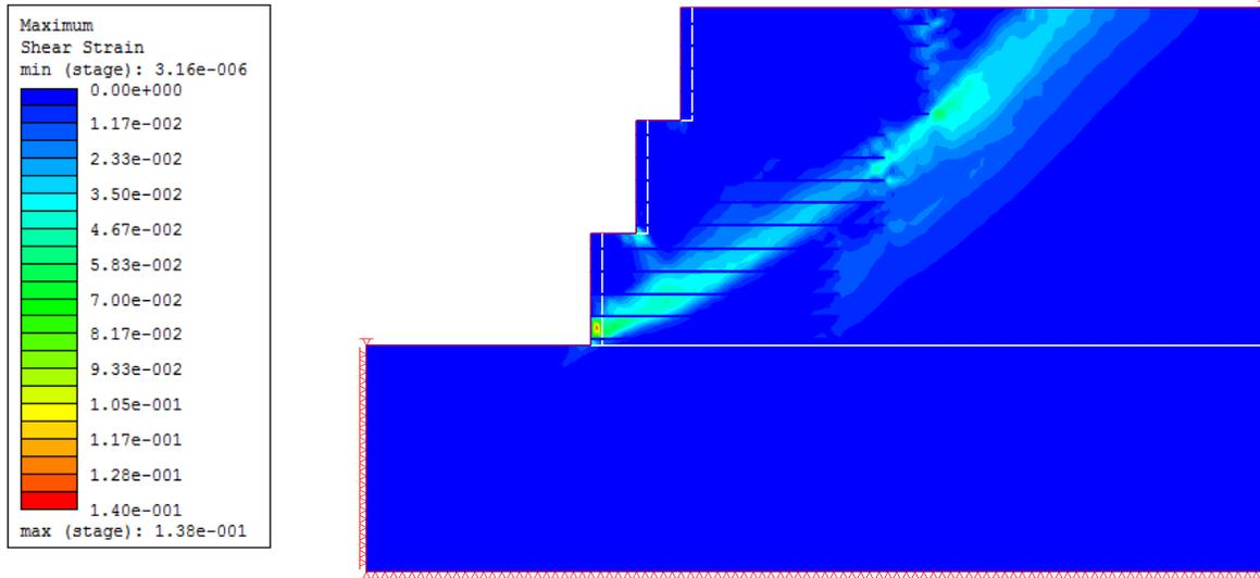
**Figure 3. Shear strength reduction method: contours of maximum shear strain. Critical shear strength reduction factor = 1.35. Computed with RS2 (Rocscience, 2014).**
