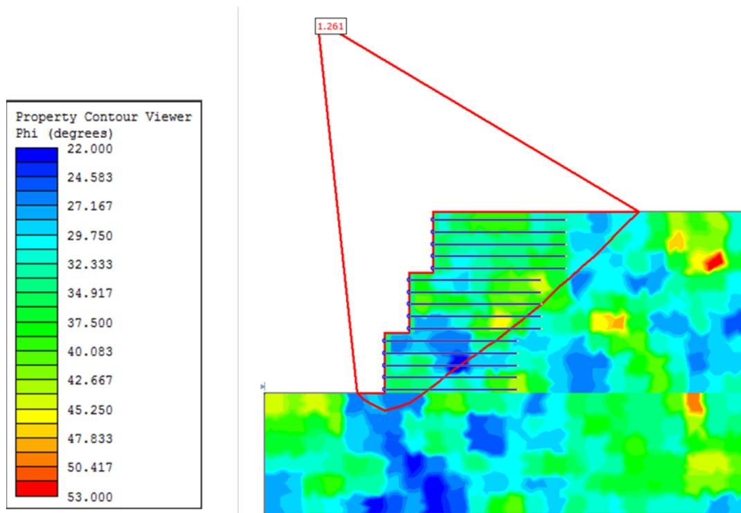
**Figure 7. Random field and corresponding failure surface and factor of safety.**
