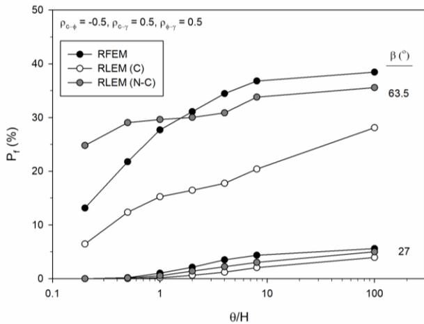
Figure 12. Comparison between the results of RLEM (circular and non-circular) and RFEM for different values of Spatial correlation length and for  $\beta = 27^\circ$  and  $\beta = 63.5^\circ$  (considering cross-correlation between soil properties).
