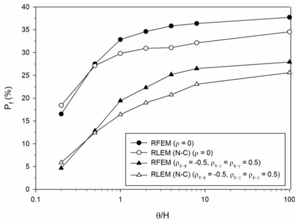
Figure 10. Comparison between the results of non-circular RLEM and RFEM for the case of  $COV_c = 0.2$  and  $COV_\phi = 0.2$  and  $COV_\gamma = 0.1$  with and without cross-correlation between soil properties.
