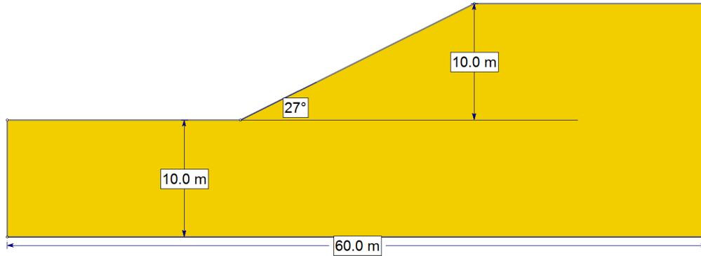
**Figure 1. Slope model used in the study.**
