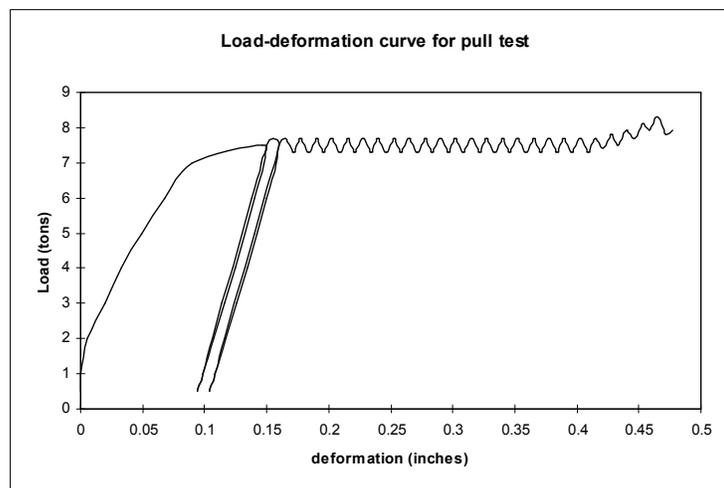
**Figure 2-10. Load-deformation curve for a pull test carried out on a 5 ft. SS39 immediately after installation. The bolt was loaded until initial slippage, unloaded and reloaded twice and then pulled out of the hole for a full 0.5 inches. Note that an approximately constant load of 7.5 tons was reached. From Scott, 1977.**
