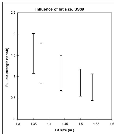
**Figure 2-7. Relationship between bit size and pull-out strength for all SS39 test results (numbering over 450). The results are plotted in error bar form for the five most common bit sizes (1.35, 1.375, 1.438, 1.5 and 1.538 in. sizes). Each bar represents the distribution of test results for its particular bit size. The bars are centred on the mean, with each extremity positioned one standard deviation on either side of the mean.**
