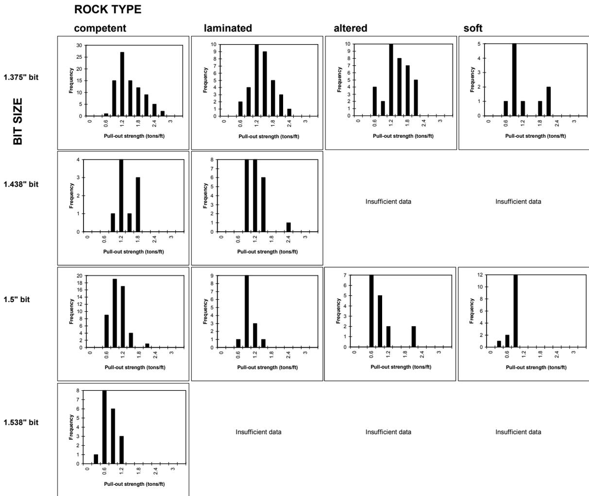
**Figure 2-20. Histograms showing the distribution of immediate pull-out strength for different rock types and bit sizes. Note that the sample sizes are not all the same and that there was not enough data in some circumstances to produce histograms. All histograms are for SS39 bolts.**
