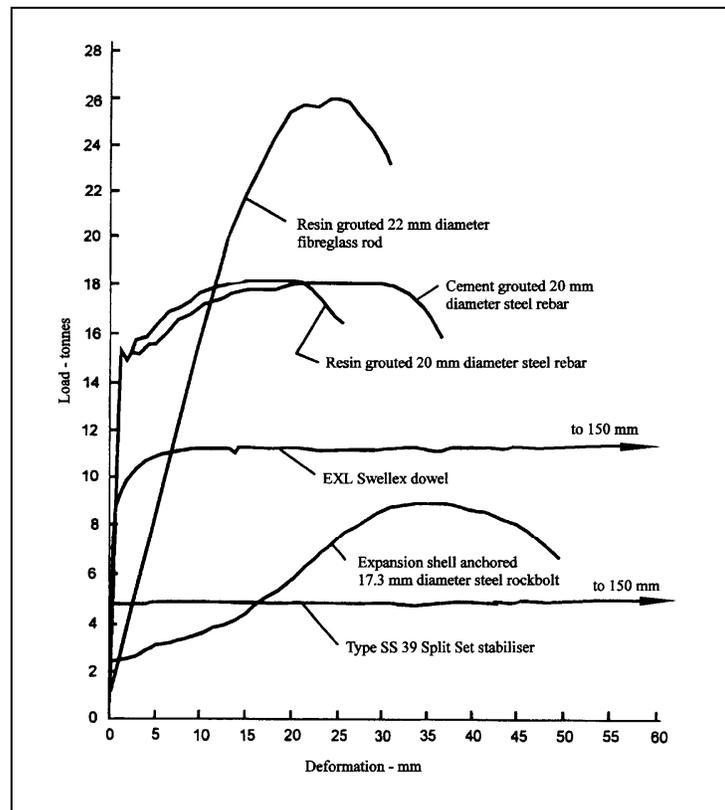
**Figure 2-11. Load-deformation curves obtained in tests carried on various support elements. High strength reinforced concrete with a uniaxial compressive strength of 60 Mpa was used for the test blocks and holes were drilled with a percussion rig to simulate in-situ rock conditions. From Stillborg, 1994**
