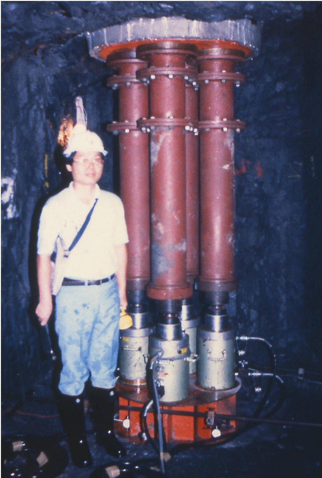
In situ jacking test in an exploration adit for the New Tienlun hydroelectric project in Taiwan
