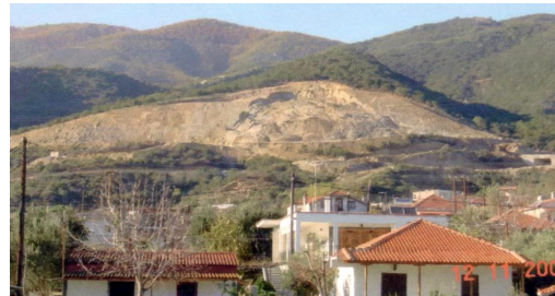
Figure 21. The landslide of figure 20. the rotational failure is clear
