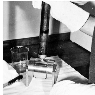
(f) Rubber forced into mould with hand piston.
