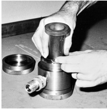
(a) Insertion of sleeve into cell body.
