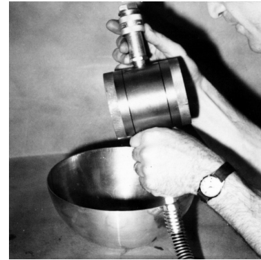
(c) Cell filled with oil by hand pump with air bled through second coupling.
