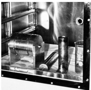
(g) Full mould and utensils cured at 100°C for 3 hours.
