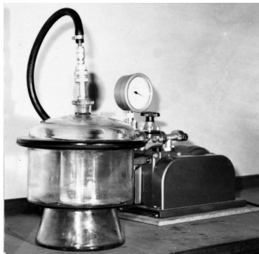
(d) Adiprene subjected to vacuum of 2 mm Hg for 5 min and then reheated before mixing.
