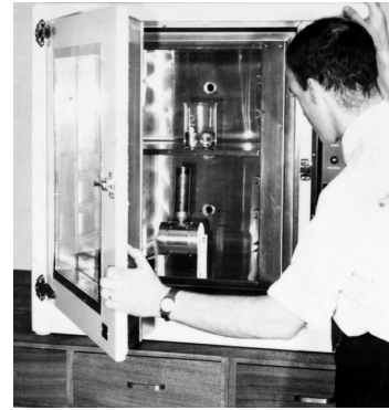
(c) Mould and rubber heated 30 min. Mould and Adiprene at 100°C, MOCA at 120°C.
