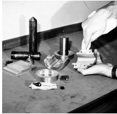
(b) Mould greased with release agent and assembled.
