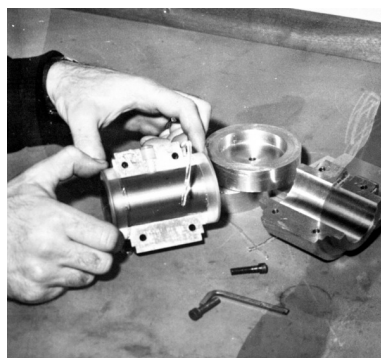
(h) Mould struck and cured rubber sleeve removed.
