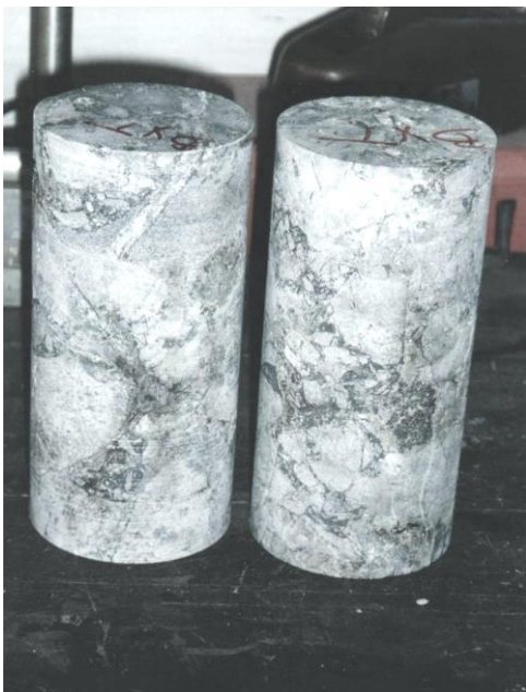
Fig. 20. 100 mm diameter by 200 mm long specimens of Braden Breccia from the El Teniente mine in Chile
