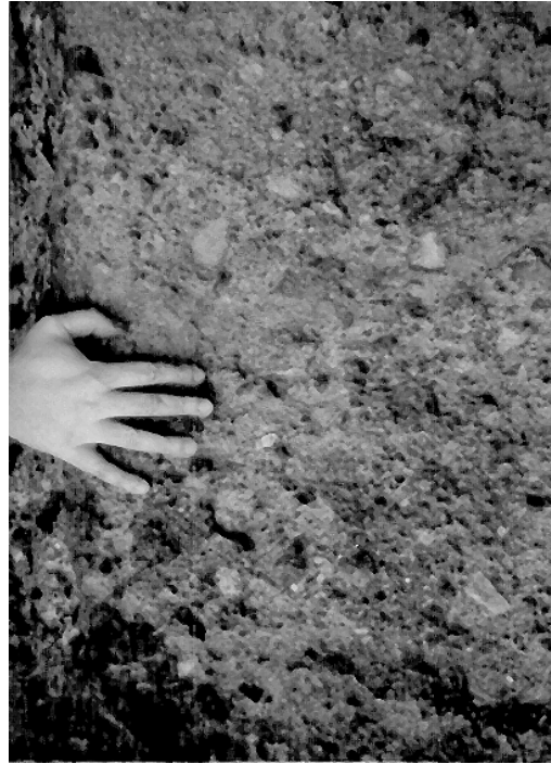
Fig. 10. Braden Breccia at El Teniente Mine in Chile. This rock is a cemented breccia with practically no joints. It was dealt with in a manner similar to weak concrete and tests were carried out on 100 mm diameter specimens illustrated in Fig. 11.
