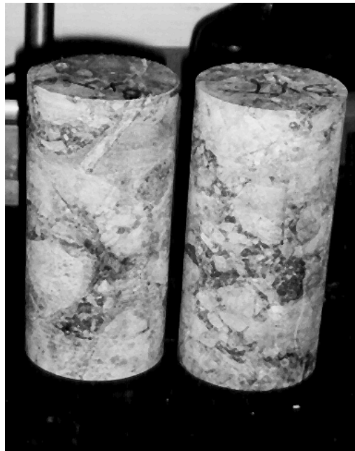
Fig. 11. 100 mm diameter by 200 mm long specimens of Braden Breccia from the El Teniente mine in Chile.
