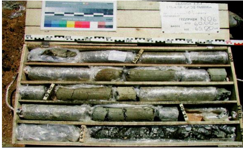
Figure 24 Core of weak ophiolites recovered from borehole NO6 behind the Big Cut at depths from 60 to 65 m below surface. Pieces of clayey like transformed serpentine are present.
