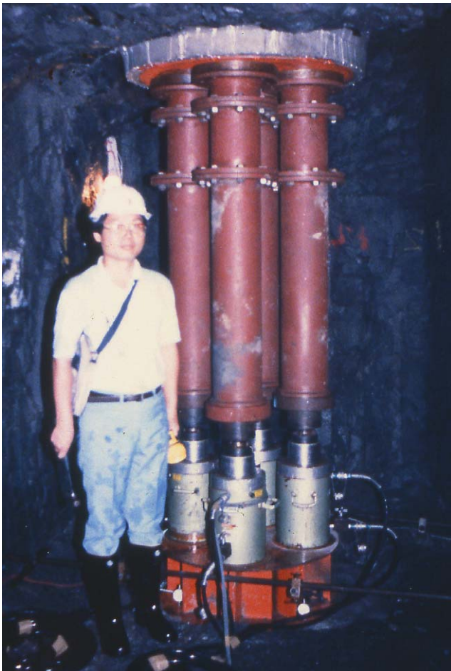
Fig. 3. In situ jacking test in an exploration adit for the New Tienlun hydroelectric project in Taiwan.
