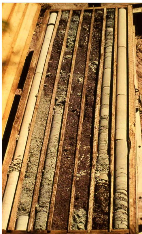
Figure 7: Similar core to that shown in Figure 6 but after storage for 6 months.
