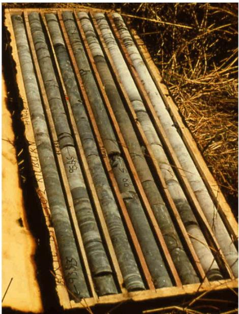
Figure 6: Freshly drilled sandstones and siltstones from the Drakensberg Pumped Storage Project in South Africa (1972).
