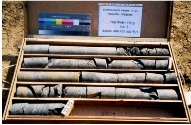
Figure 4: Appearance of molassic rock core immediately after drilling. Sandstones and siltstones are present but the bedding planes (mainly of the siltstone) do not appear as defined discontinuity surfaces.
