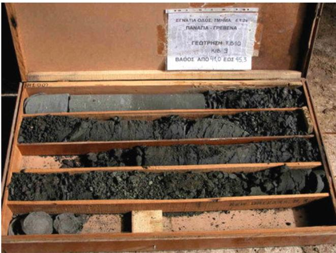
Figure 5: Appearance of the same core as shown in Figure 4 but after storage in a core shed for six months. The sandstone remains intact but the siltstones exhibit fissility followed by collapse.
