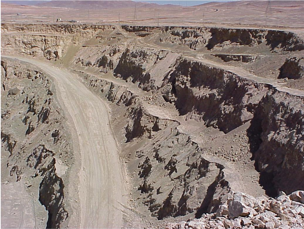
Figure 9: Bench faces created by normal production blasting.
