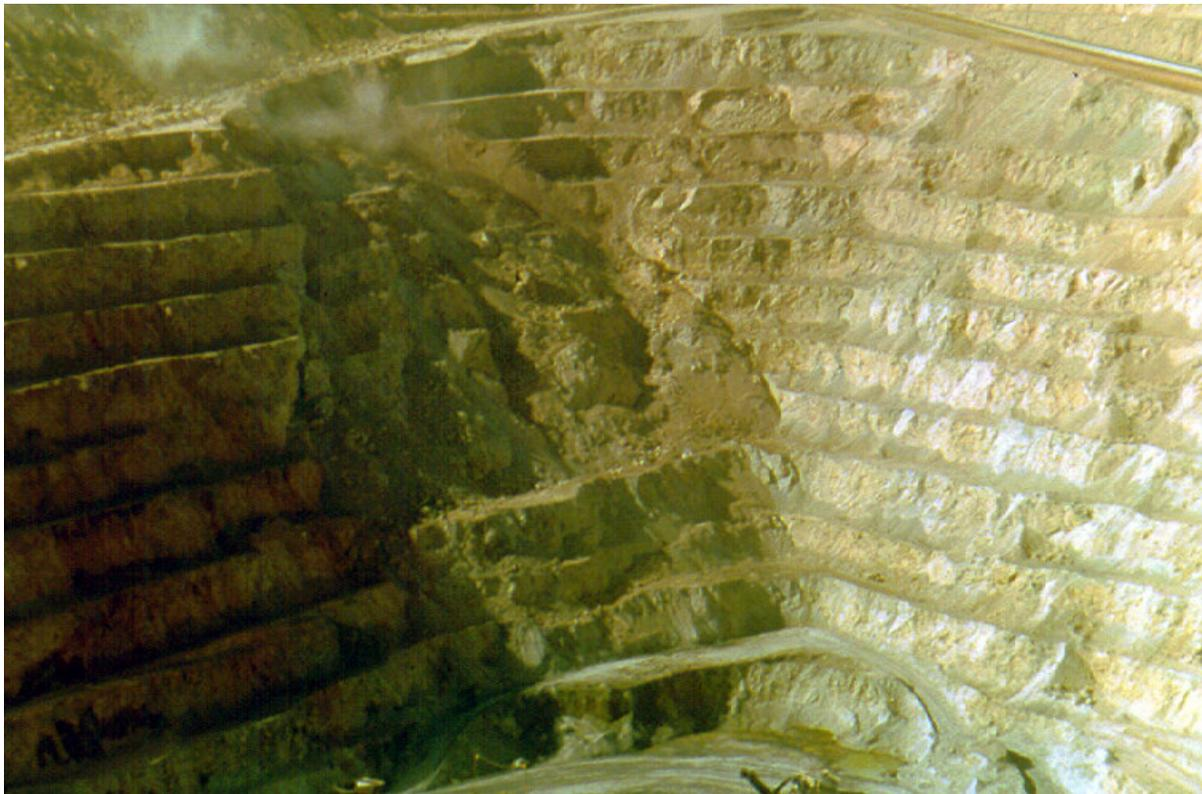
Figure 1: Slope failure in which some structural control by faults is evident at the top of the failure but where the mechanisms involved in the lower part of the failure are unclear.
