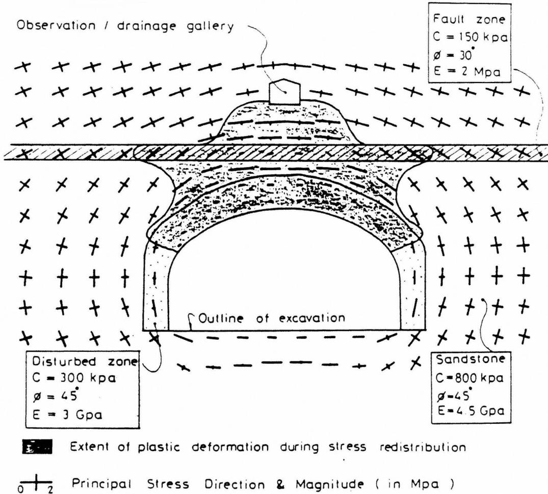
Figure 9. Input/output data for FLAC analysis
