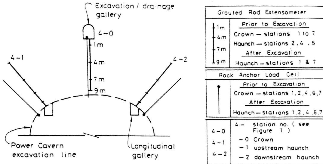
Figure 5. Instrumentation layout
