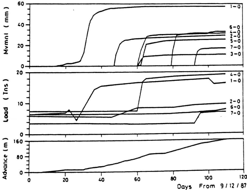
Figure 6. Instrumentation data, top heading excavation
