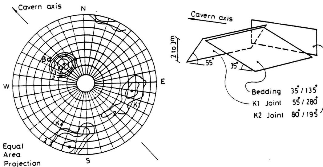
Figure 2. Jointing and wedge formation in cavern roof.
