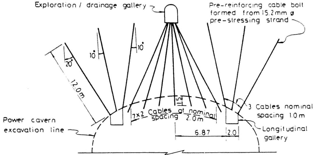
Figure 4. Typical arrangement of pre-reinforcement cables
