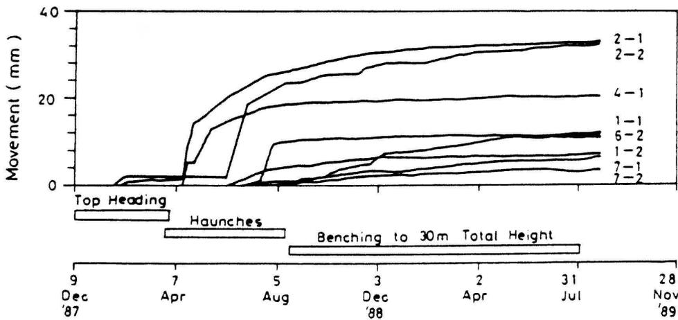
Figure 8. Haunch extensometer data to August 1989
