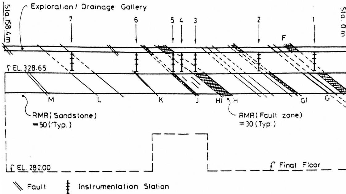
Figure 1. Longitudinal section of power cavern showing encountered geology.
