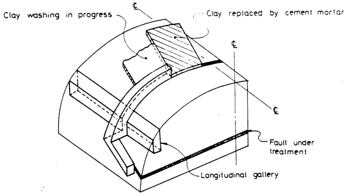
Figure 3. Schematic layout of fault treatment works
