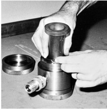
(a) Insertion of sleeve into cell body.
