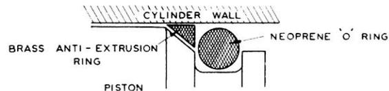
Figure 9. Detail of high pressure moving seal.
