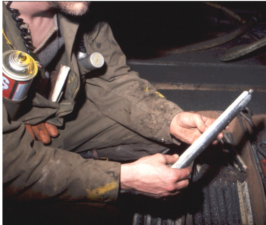
Figure 3: Typical two-component resin cartridge used for anchoring and grouting rockbolts
